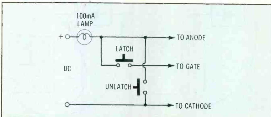
Figure 9 Any supply between 6V and 28V can be used as a test voltage for higher-power SCRs, provided the lamp has the same rating and draws about 100mA.
