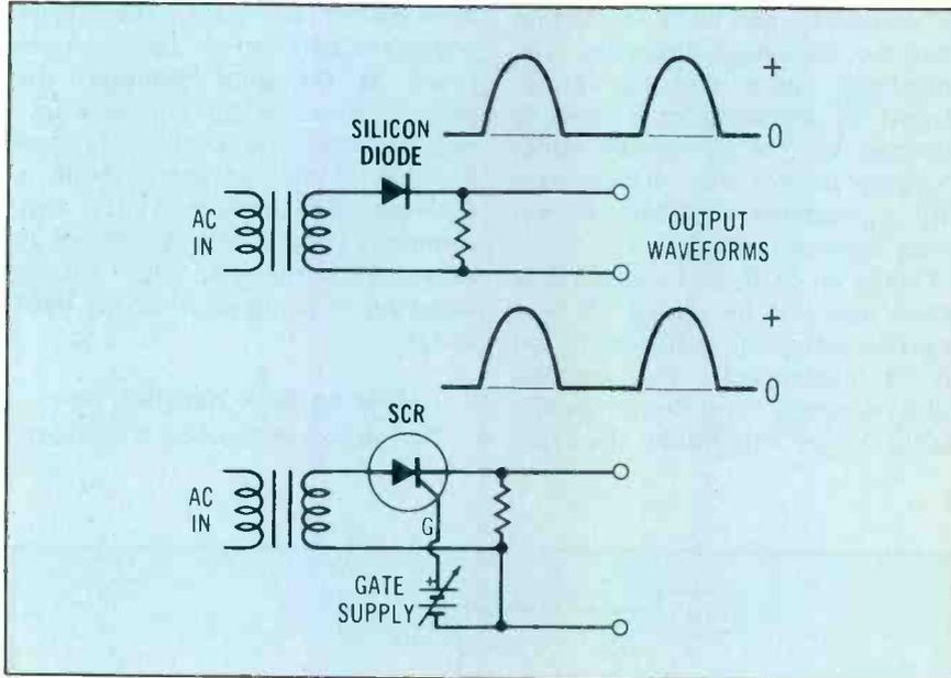
Figure 4 An SCR that is gated on steadily produces the same output waveform from ac as a regular silicon diode.
