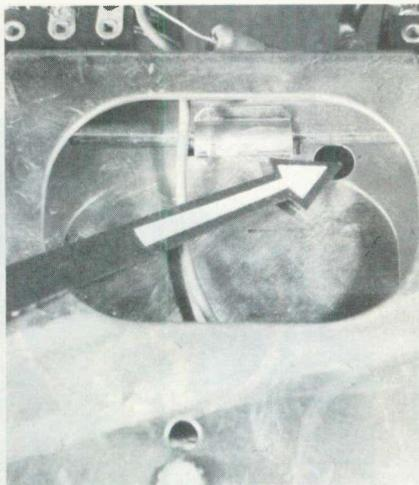
Many of the older tuners with Nuvistor RF amplifiers by now have had tuner cleaners sprayed accidentally into the neutralization trimmers. This gives the effect of wrong neutralization and produces oscillation on some high-band channels. The trimmers must be thoroughly cleaned out with a solvent and allowed to dry before they are adjusted.
