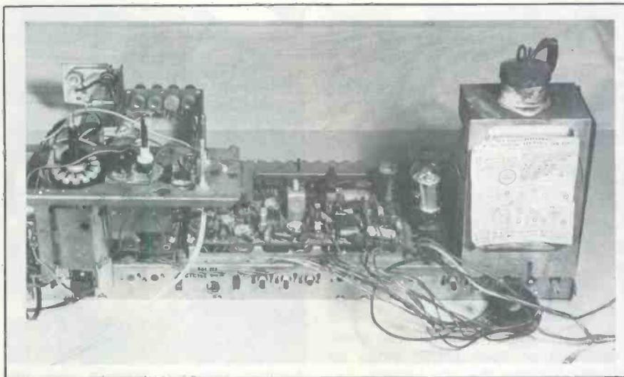
An old RCA CTC16 chassis was selected as an example. Notice that the tuner assembly is mounted correctly on the chassis for servicing or transportation. Two chassis screws and matching slots in the tuner bracket hold the assembly. (If the tuner is placed on top of chassis wiring severe damage can occur to unshielded coils and other fragile components.)
