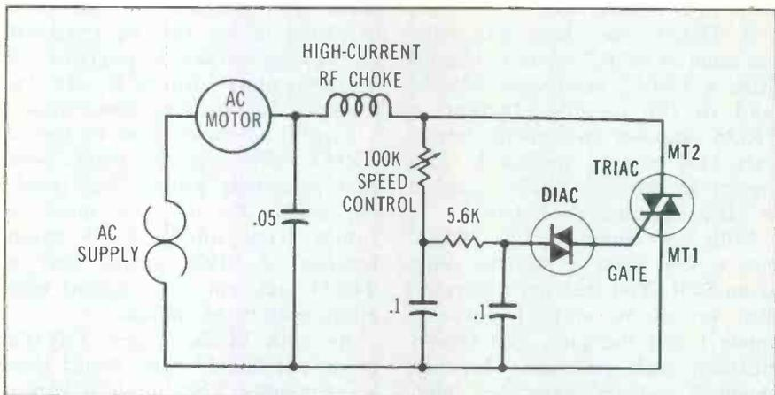
Figure 14 A practical TRIAC-type motor speed control should have a choke and capacitors to suppress RFI.
