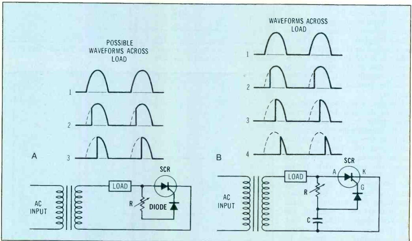
Figure 5 (A) An SCR that's gated by ac controls power to load. Waveform 1 is half-cycle, 2 is less than half-cycle, 3 is quarter-cycle of applied current. This circuit is limited to a control range between  $\frac{1}{2}$  and  $\frac{1}{4}$  ( $90^\circ$ ) of cycle. In B, adding a capacitor allows control over the entire half-cycle ( $180^\circ$ ).
