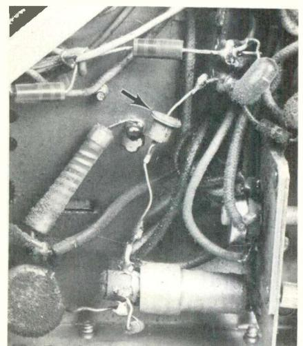
Another servicing mistake was the conventional *top-hat* diode used as a boosted-boost diode. This one was not shorted, but it should have been, for these are called on to supply about 300V of extra dc voltage—far above the ratings of the wrong replacement.
