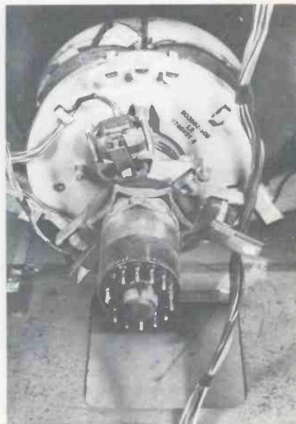
The convergence-yoke assembly was crooked on the picture-tube neck, evidence of previous poor servicing.
