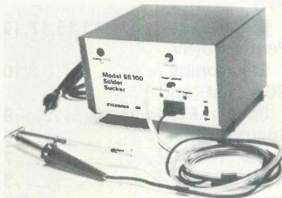
for removal of solid-state devices from circuit boards. An internal pump provides vacuum controlled by a switch on the handle of the soldering iron. A switch selects either 40- or 20-W iron power. Two iron tips are included and six others are available.
