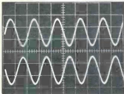
Figure 1 The graticule has full-size 8cmX10cm calibrations. Here is a typical waveform and graticule when the illumination is adjusted for maximum.
