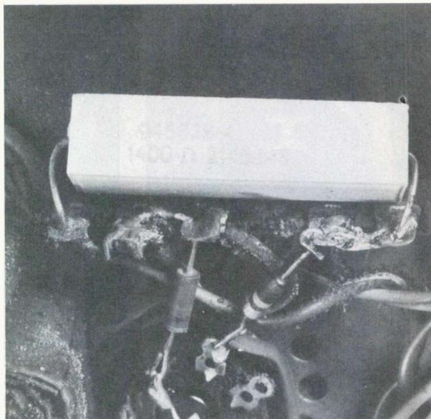
Heat from the large 20W 1400  $\Omega$  wire-wound resistor deteriorated all soldering joints on the terminal strip and carbonized the insulation. None of the joints were open, but would have gotten worse with time.
