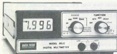
and current, resistance to .1 Ω resolution and a diode test feature. The list price for the basic instrument including one set of batteries is \$159.
