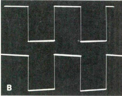
**Figure 2** (A) Each channel has a lever-type ac/dc coupling switch that is convenient to operate. (B) Square waves of 20Hz had no tilt during dc-coupling operation. With the low-capacitance probe and ac coupling, the tilt at 20Hz is barely noticeable (bottom trace, indicating good low frequency response).
