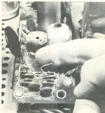
The degaussing thermistor was missing. Such an open circuit stops all operation except the tube heaters. For a temporary test, short across the thermistor leads. The thermistor also functions as a surge resistor, so it's advisable to replace any bad ones rather than jumpering them permanently.
