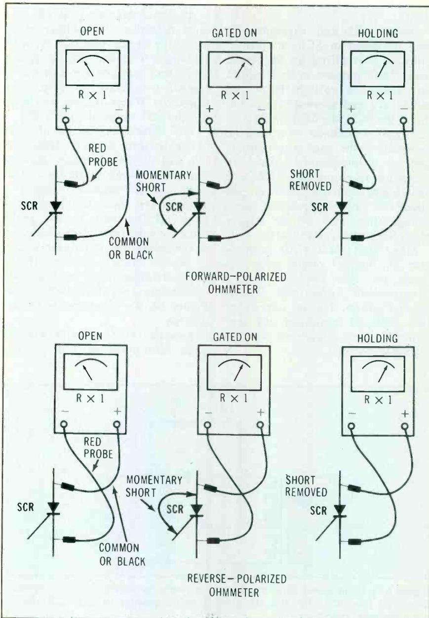
Figure 8 Testing SCR with ohmmeter of either polarity. Clue: Always gate SCR from anode voltage.
