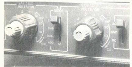
**Figure 4** Six types of dual-trace operation can be selected by this mode switch and other control settings.
