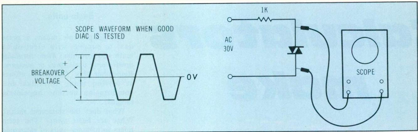
Figure 15 DIAC testing with ac and oscilloscope may not reveal imbalances, unless dc scope coupling is used.
