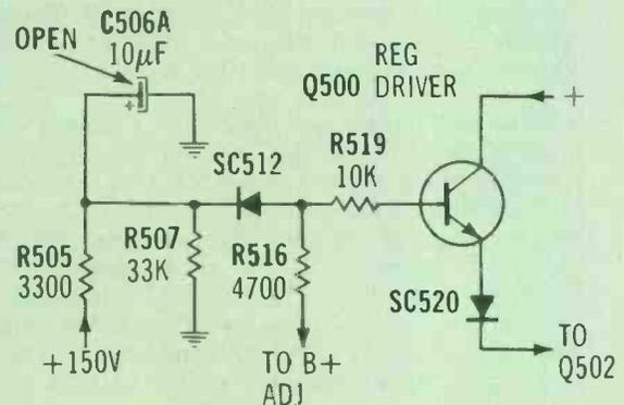
**Symptom**—Excessive B+ and HV causing shut-down
