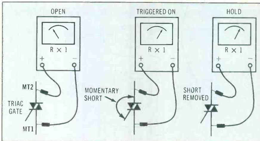
Figure 12 After testing a TRIAC with the procedure above, reverse the ohmmeter leads and perform the same tests again, to check operation in both polarities. The ohmmeter Rx1 scale must be used, to provide sufficient holding current.
