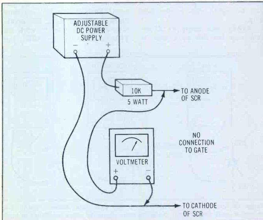
Figure 10 Testing SCR breakover voltage. For testing reverse breakover, connect positive lead of supply to SCR cathode and the negative lead to anode.
