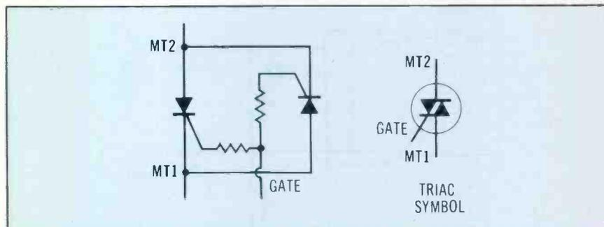
Figure 11 A TRIAC operates like two SCRs in parallel-opposing.
