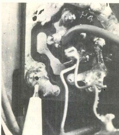
A pen points to the hole in a ground joint of the IF board where a ground lance had pulled loose. Erratic color level often results from opens at auxiliary grounds.
