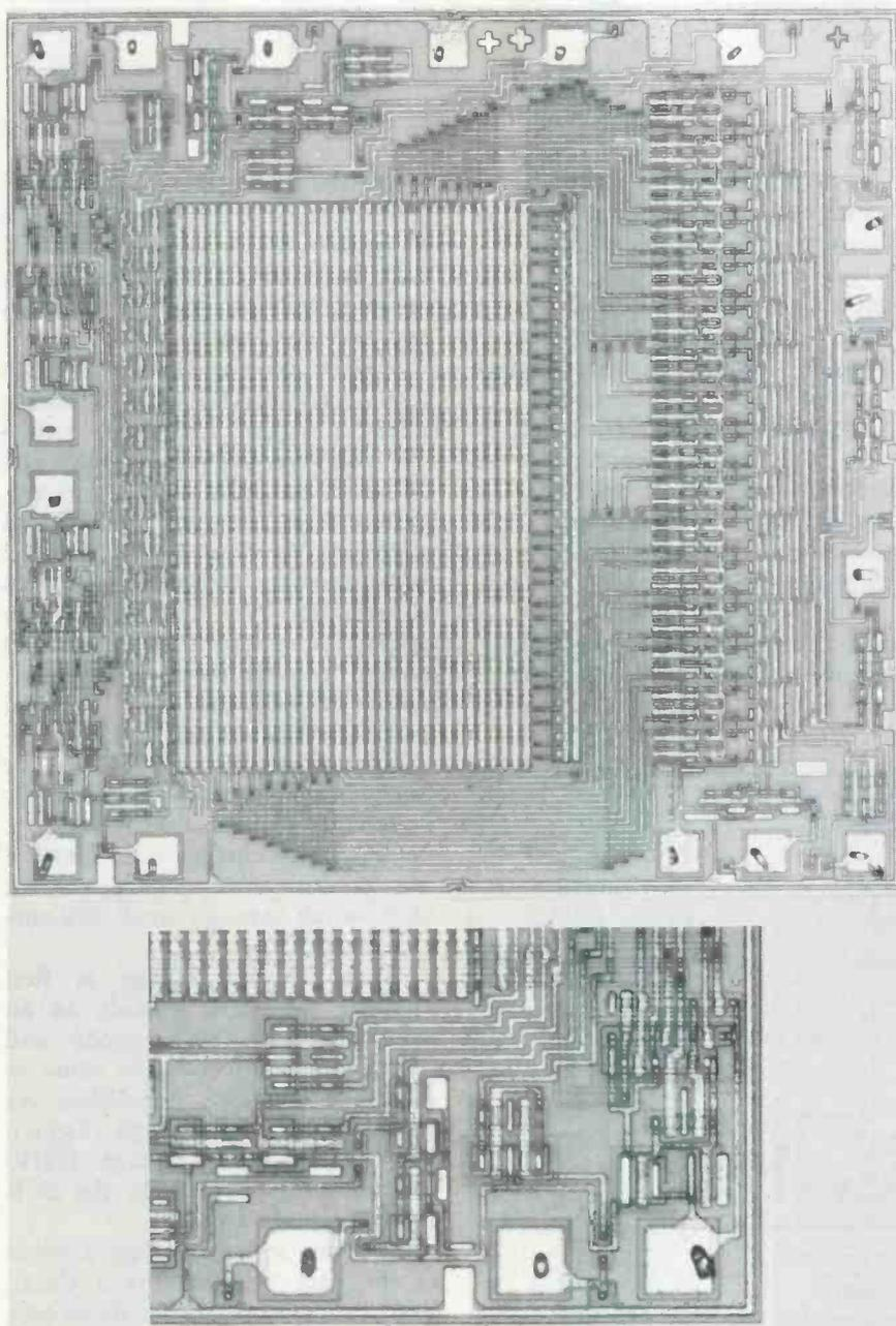
For the Motorola model MCM1452 1024-bit Read-Only Memory (ROM), one picture shows the entire IC chip, which is about a quarter-inch square. The other is a 27-times enlargement of one corner of the same chip. (Courtesy of Motorola)
