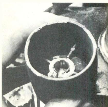
Plate caps on regulator and horizontal-output tubes can be sources of mysterious noise patterns in the TV picture. One common defect is a broken weld where the lead wire is fastened to the metal cap. Such a cap should be replaced since the high heat would melt solder. This 6BK4 cap was crumbling but the weld was alright.
