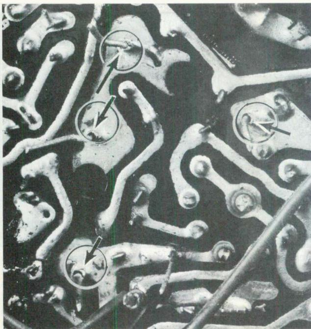
More than eight bad solder joints were found. This closeup picture has arrows added to mark four joints ruined by resistor heat. These resistor leads were loose in the solder.
