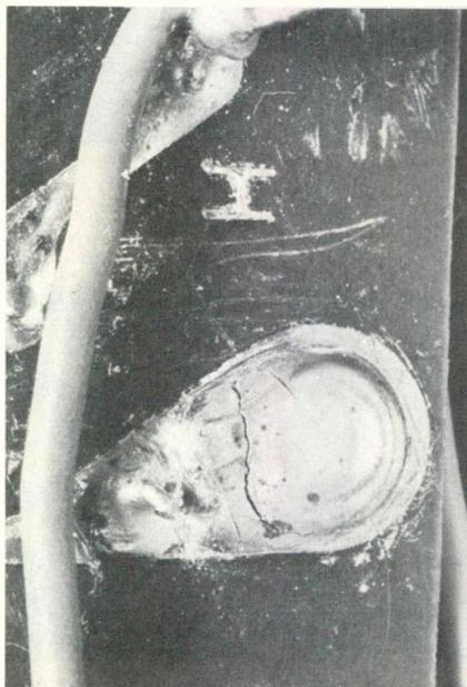
This crack at a ground in the oscillator circuit extended around the rivet completely. It caused intermittent operation of the horizontal oscillator. Flexing of the board made the crack more visible.
