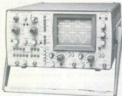
MHz. The OS3500 display modes are flexible and include CH1 or CH2 alone, CH1 and CH2 alternate or chopped, CH1 and CH2 added algebraically and X-Y.
