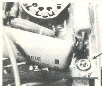
Many RCA chassis develop intermittently open connections at one of the chroma board grounds (see arrow). An open produces extreme brightness and loss of HV. This pictured joint was not bad yet, but both lead wires of the metal-film resistor in front of it were loose in the solder.
