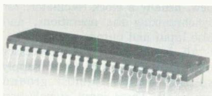
Shown approximately life-size is an 8080 N-channel 40-pin 8-bit microprocessor. The chip inside is even smaller.
