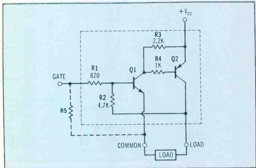
Figure 3 A transistor regenerative switch bears many similarities to an SCR. Resistors' values are typical for  $V_{cc}$  of 6V to 12V.
