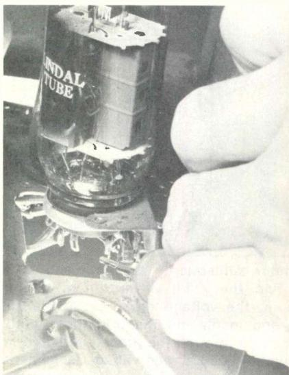
The 6JE6 or 6LQ6 screen grid often can be reached for voltage tests through the ventilation space below the tube-socket shelf.
