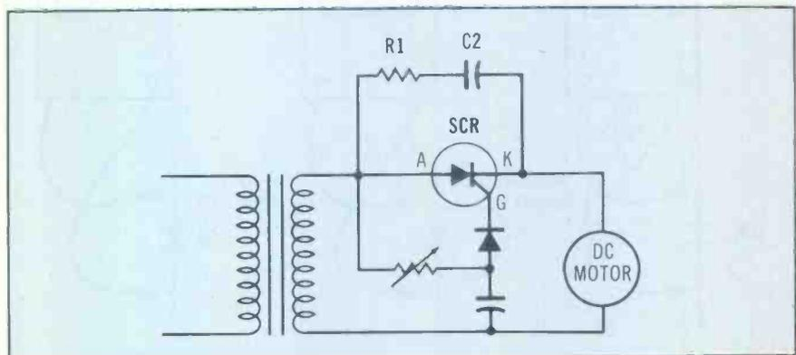
Figure 6 In some speed controls, the motor might be connected in the cathode circuit of the SCR. R1 and C1 prevent self-triggering of the SCR due to inductive-load kickbacks.
