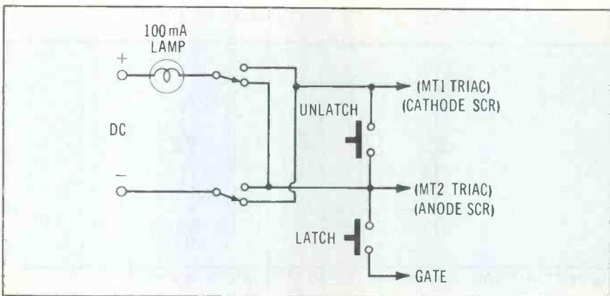
Figure 13 For checking both TRIACs and SCRs, add a DPDT switch. Test all TRIACs in both positions.
