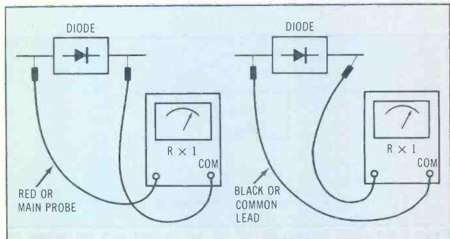
Figure 7 Use a diode to reveal polarity of voltage coming from the leads of your ohmmeter.
