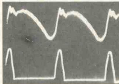
Top trace shows the +123V regulated supply's 6VPP ripple, while the horizontal-sweep waveform is included below to show timing of the ripple.
