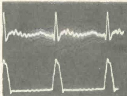
**Figure 7** Narrow 0.25VPP pulses (top trace) are found at the U400 pin-1 correction voltage that locks the master oscillator. Lower trace shows normal flyback pulses for comparison.
