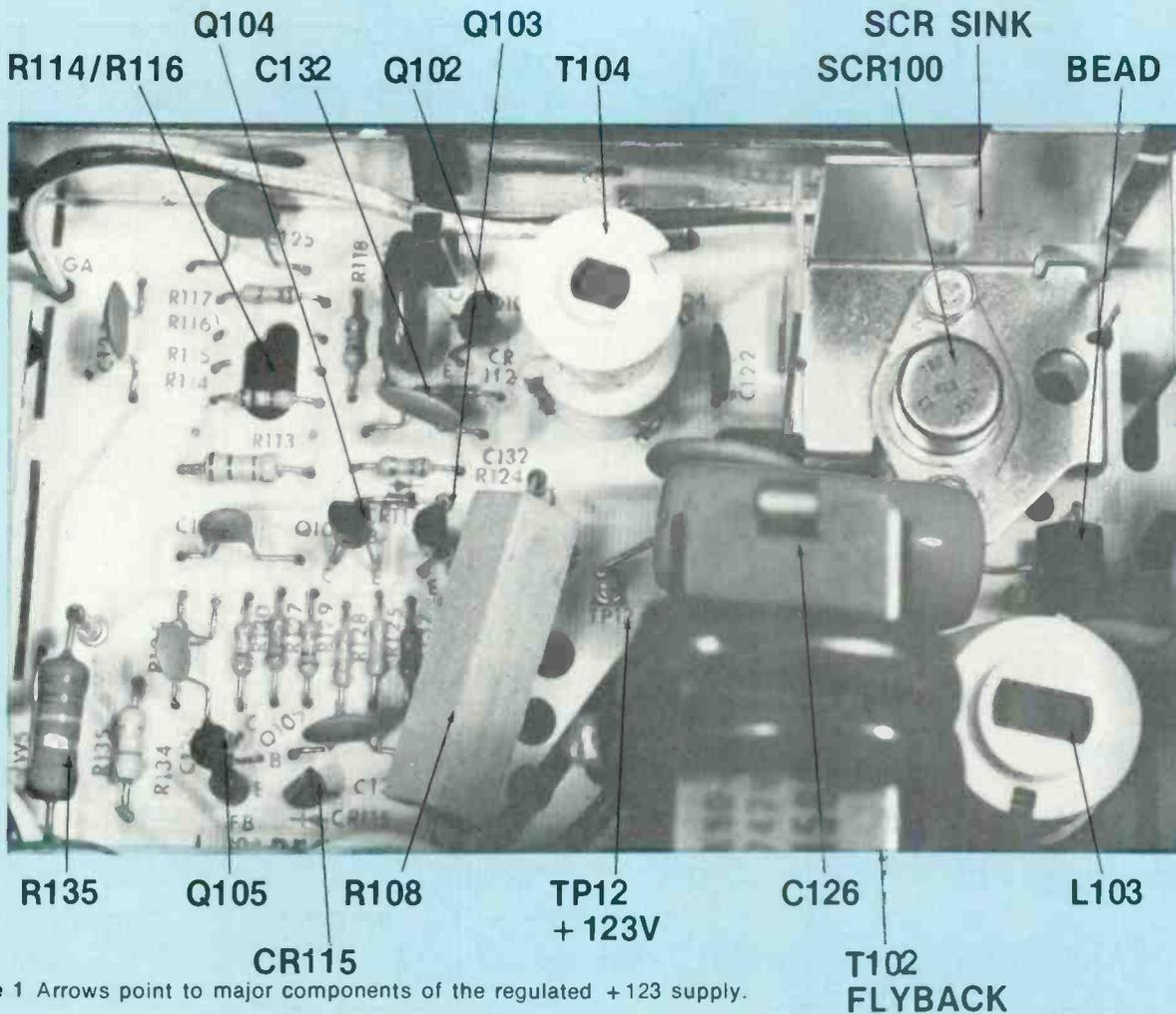
Figure 1 Arrows point to major components of the regulated +123 supply.
