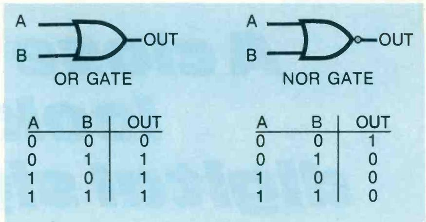
Figure 1 Truth tables show, in tabular form, the functions of logic symbols and devices, and are clues to what you can expect from digital signals of the steady-state variety.
