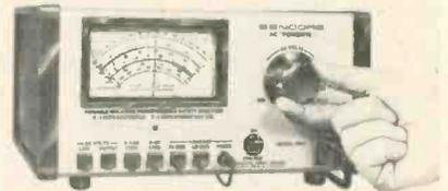
leakage check. Ac voltage is variable from 0 to 140V. A 2% recessed 6-inch meter is used to monitor ac volts, current and watts.
