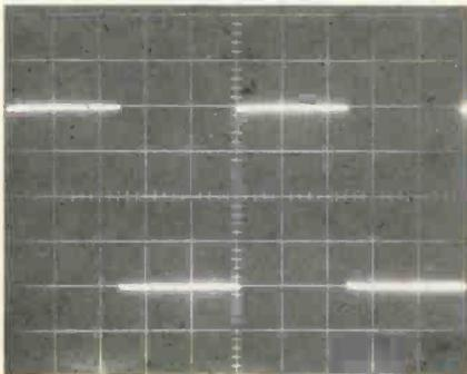
**Figure 3** Looks like a square wave, but it's not. This signal is digital, with a duty cycle that leaves it on half the time and off the other half.
