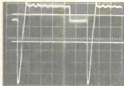
L103, and during conduction, no pulse is there because filter C126 has removed it. Therefore, the SCR current continues after the start of the flyback pulse (although at a decreasing rate) until the input pulse drops to the zero line. There the SCR unlatches, and all conduction current (both +155V and pulse) ceases. This explains the rectification of pulses that appear to be too negative to allow rectification.
