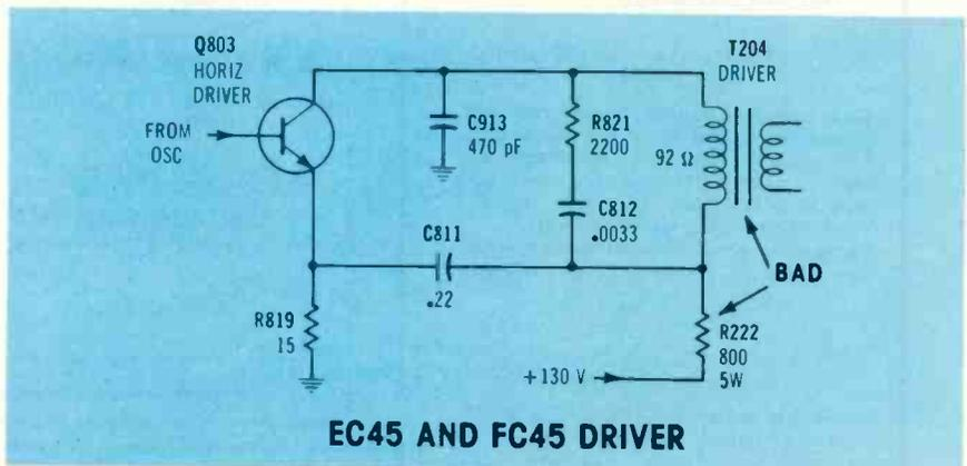
Figure 1 T204 driver transformer and B+ resistor R222 are two horizontal components that occasionally fail in the 19EC45 and 19FC45 Zenith chassis.
