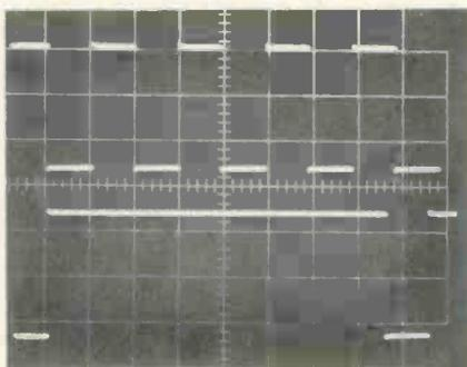
**Figure 3** CW rotation of T1 or T2 controls *increases* duration of that pulse. (A) The top trace (20mS/div) showed T1 9.95mS and T2 10mS durations for a rep rate of about 50Hz. For the lower trace, T1 setting remained the same and T2 was turned fully CW. This increased T2 to about 80ms for a new rep rate of about 12Hz. (B) These conditions started the same with 9.95mS and 10mS but T1 control was turned fully CW, thus lengthening the T1 duration by almost eight times the original.
