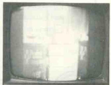
Figure 3 A bad solder joint at the base return of the horizontal-output transistor narrowed the picture as shown.
