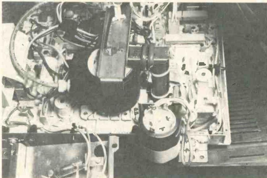
All 123V regulator components are located in front of the flyback; at the right in this picture taken from the high-voltage side.
