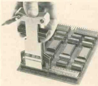
applied simultaneously at both ends of the IC. Designed one-hand operation, the EX-2 features chrome plating for static dissipation, and a terminal lug for attaching a ground strip (strap not included).
