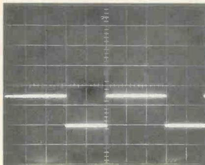
**Figure 4** Examples of various duty cycles; you can recognize these rather easily just by inspection. Text explains calculations involved in more critical duty-cycle measurements.
