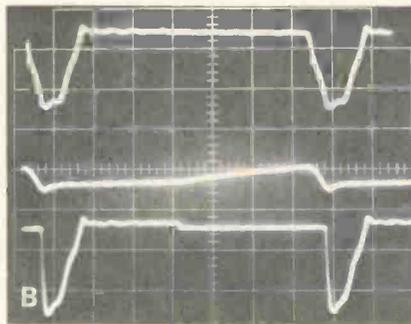
**Figure 4 (A)** These are the normal flyback pulses (top trace), SCR anode current (center), and SCR-anode waveform (bottom trace) when the raster was black and the line voltage was 120Vac. The scope controls were not adjusted, but line-voltage reduction to 60Vac produced the changed waveforms of (B).
