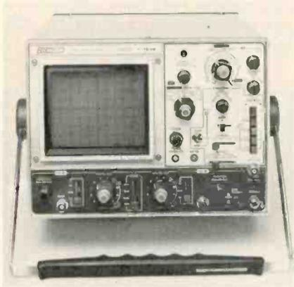
operation, differential measurement capability, and algebraic addition and subtraction of two vertical input signals. The unit operates on 115 or 230 Vac.
