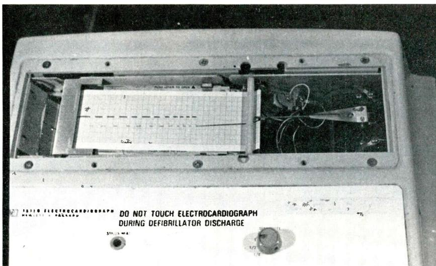
Figure 6 The stylus and galvanometer are exposed for convenient voltage tests and stylus-pressure adjustments after the access cover is removed.
