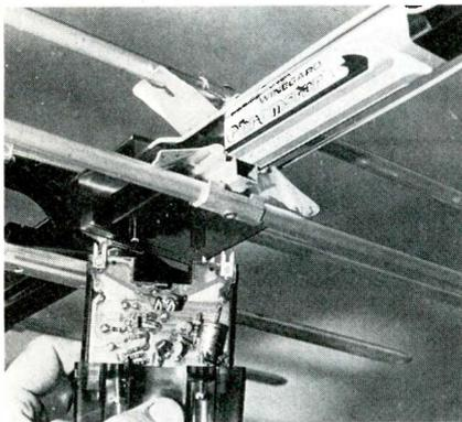
A mast-mounted or antenna-mounted preamplifier produces the best signal-to-noise ratio. This preamplification should occur *before* the downlead attenuates the signal. Either a pre-amplifier or a balun is necessary at the antenna when it is to be connected with coaxial cable downlead. *Courtesy of the Winegard Company.*
