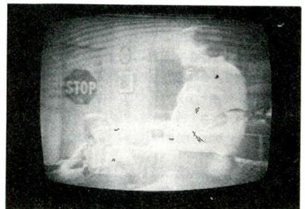
Figure 3 An intermittent tube socket of the AGC keyer in a Sylvania caused erratic losses of contrast. Any moderate increase of *both* RF and IF AGC voltages reduces the contrast.
