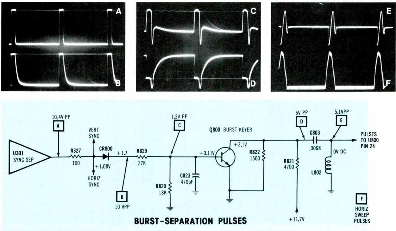
**Figure 4** Horizontal-sweep pulses are not used for burst keying. Instead, horizontal sync pulses are processed and used to ring the C803/L802 series-tuned circuit. The important waveforms are shown in the pictures. Waveform D is the driving signal for the C803/L802 ringing circuit. The positive peak of waveform E ringing signal at U800 pin 24 keys-on the burst separation. Figures E and F are dual-trace waveforms that show the ringing-pulse delay (E) relative to horizontal-sweep pulses (F).
