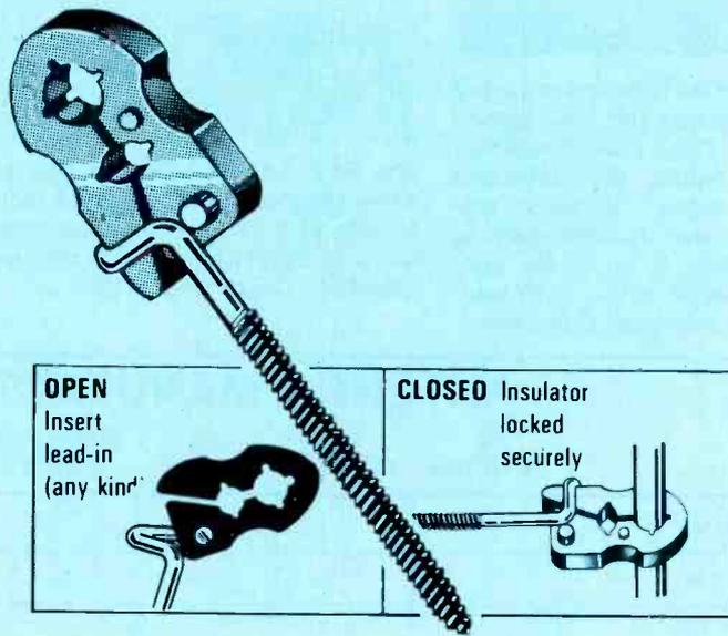
GC Electronics lists many items of hardware for TV-antenna installations. One unique product is E-Z Swing-In standoffs which swing open for insertion of the downlead and then can be locked in the closed position. *Courtesy of GC Electronics.*
