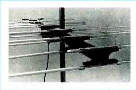
**Girder-type** construction illustrates the strength and durability of new antennas.
