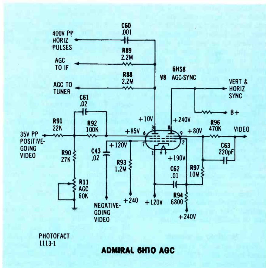
**Figure 7** Many variations of this combination AGC, sync separator, and noise canceller were used in older TVs. The clipped negative-going video pulses at the pin 7 grid allowed strong noise pulses to cancel the positive noise pulses at pin 6. The pin 6 suppressor grid operates similarly to the control grid in a triode AGC keyer; it controls the plate rectification.
