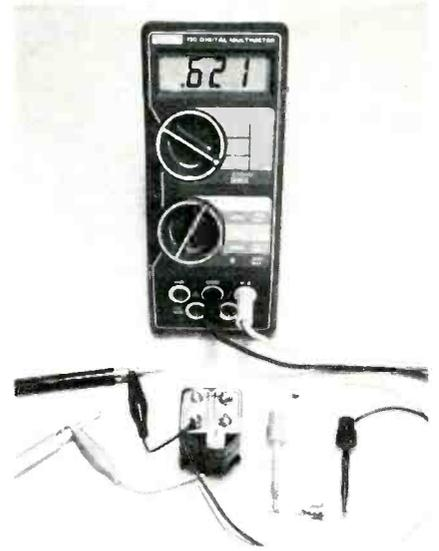
During electronic troubleshooting in the field, most suspected diodes are checked for their resistances during alternate applications of forward-bias and reverse-bias polarities of voltage. The reverse-biased resistance of a good diode should be much higher than the forward-biased resistance.
