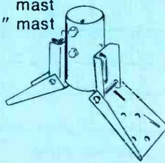
RCA's TV Antennas and Accessories catalog lists many matching baluns and hardware for antenna installation, such as this mounting bracket. *Courtesy of RCA.*
