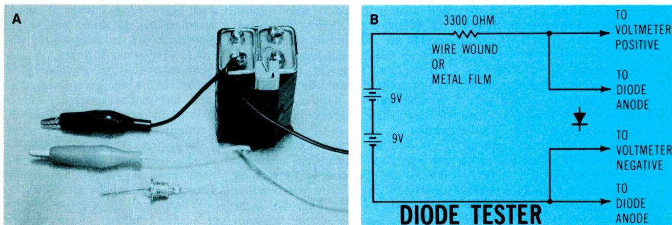
**Figure 1** (A) All components are visible in this photograph of the constant-current voltage-drop diode test adapter. A large wire-wound resistor was used for stability, not because high wattage is required. (B) The schematic is equally simple. Convenience features could be added. An on-off switch and an LED power indicator would remind technicians to shut off the power. A spring-return polarity-reversing switch would save time if many diode junctions are to be tested quickly.
