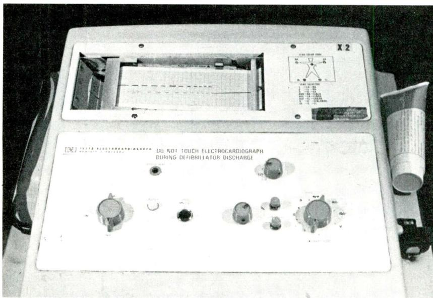
**Figure 5** A typical electrocardiograph is this Hewlett-Packard model 1511. At the right is a tube of conductive paste that is used on the electrodes to give better traces without hum or artifacts.
