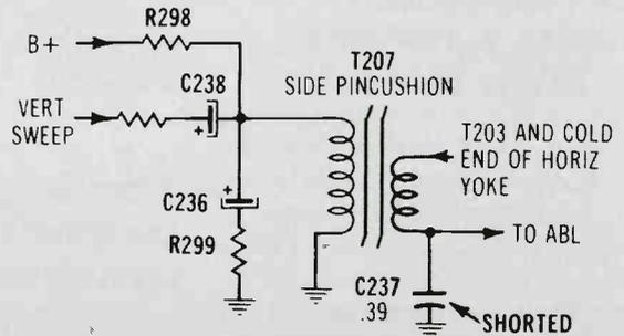
**Symptom**—No picture, no sound, and breaker is tripped. Reset breaker gives loud hum for 5-seconds before trips again.
