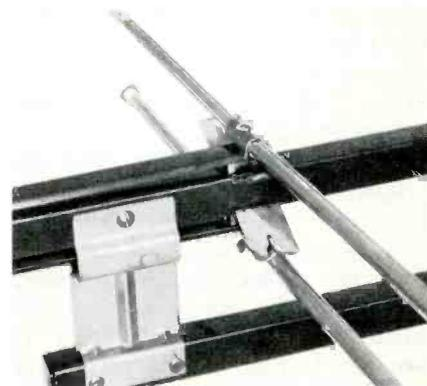
No tools are needed to assemble most new antennas. During shipping, the elements are placed parallel to the boom. Then each is rotated perpendicular to the boom where it is held by flat springs. This reduces the time required for installation. *Courtesy of the Winegard Company.*
