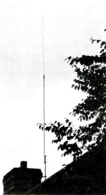
Super Big Stick fiberglass-insulated CB base antenna, by Shakespeare, is 18-foot long and has an ethylene/propylene/rubber insulating boot that insulates the antenna for voltages up to 13kV. Shakespeare is the manufacturer. *Courtesy of Shakespeare.*
