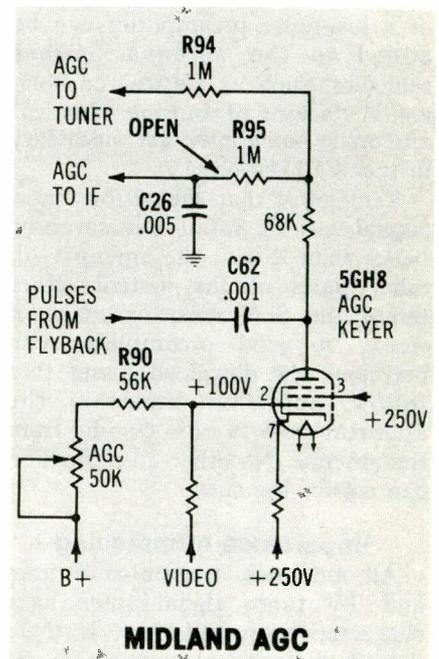
Figure 2 An open R95 in Midland model 15-214 eliminated the IF AGC. Therefore, the AGC keyer plate voltage became more negative. This applied excessive negative AGC to the RF tube and caused snow.
