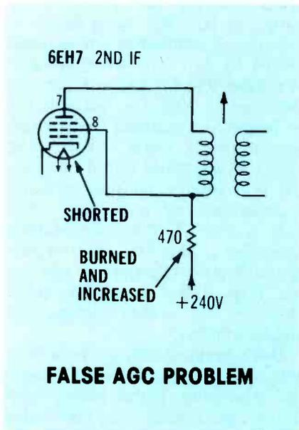
**Figure 6** Defects in tuner or IF stages can imitate AGC symptoms. Low gain in the second IF stage of a Zenith caused a low contrast picture and noisy sound.
