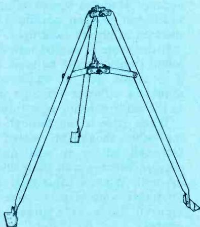
**Tripods** are very popular for rooftop mounting of antenna masts. Another tripod that includes the mast is designed for installation at the side of a roof peak.
