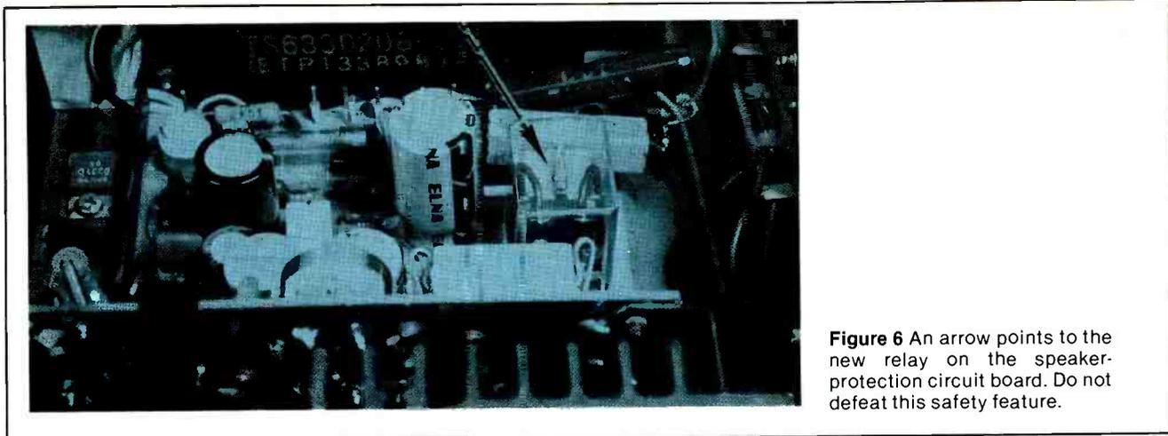
**Figure 6** An arrow points to the new relay on the speaker-protection circuit board. Do not defeat this safety feature.
