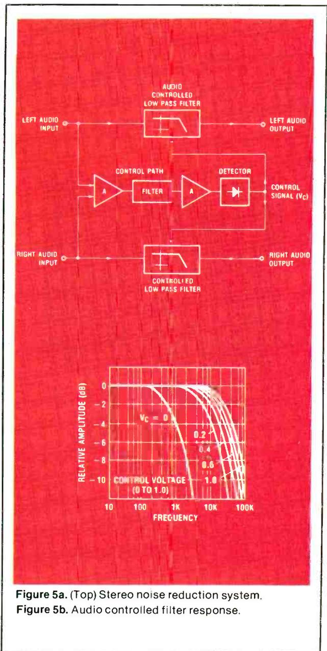
Figure 5a. (Top) Stereo noise reduction system.
