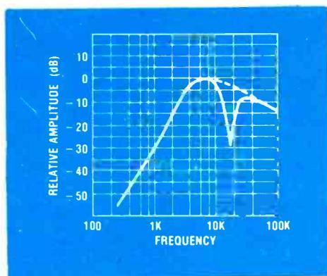
Figure 6. Frequency/amplitude response of DNR control path.
