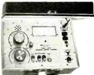
strength meter for professional installers and technicians. Designated FSM-8, the meter operates on any of three different battery combinations. The battery pack is located in the cover and batteries can be changed without removing the meter. The FSM-8 reads directly in dBmV and has a digital delay circuit to automatically shut off the meter at a preset interval.
