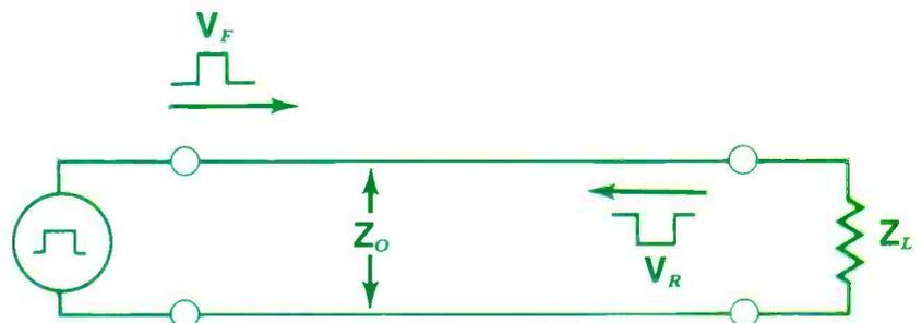
Figure 2. If the load impedance ( $Z_L$ ) does not match the characteristic impedance of transmission line ( $Z_0$ ), a portion of a transmitted signal will be reflected back to the source.
