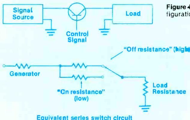
Figure 4. Analog switches may be used in either series (A), or shunt (B) configuration.
