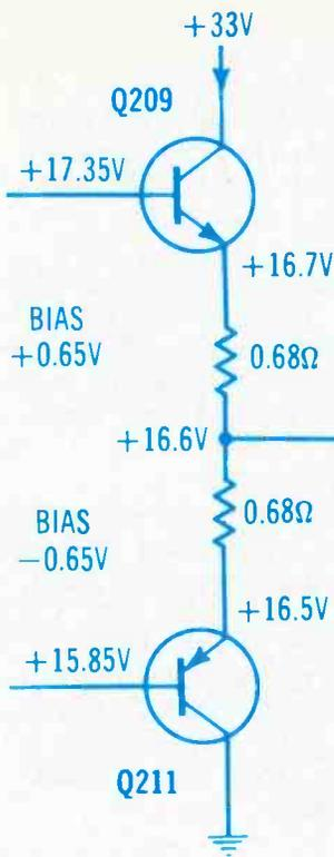
**Figure 6** The base-to-emitter bias of a Q209 NPN output transistor should equal the B/E bias of a Q211 PNP output transistor. Also, dc voltage at the output emitter resistors should be about half of the supply voltage. Always check resistances of the emitter resistors after any overload.
