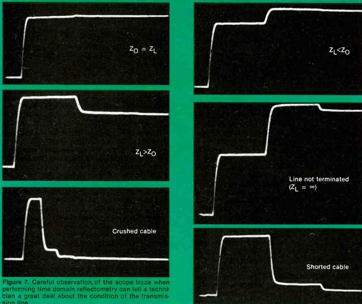
Figure 7. Careful observation of the scope trace when performing time domain reflectometry can tell a technician a great deal about the condition of the transmission line.
