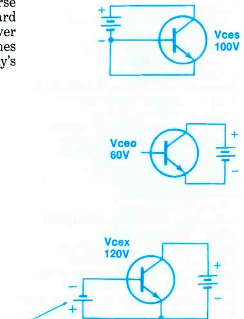
Figure 1. Transistor voltage ratings are established by connecting the transistor in a number of different configurations. It is important to exercise care in interpreting these values in light of the intended application.
