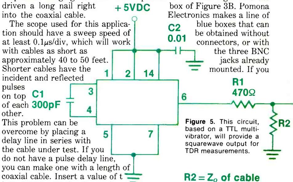
Figure 5. This circuit, based on a TTL multivibrator, will provide a squarewave output for TDR measurements.
