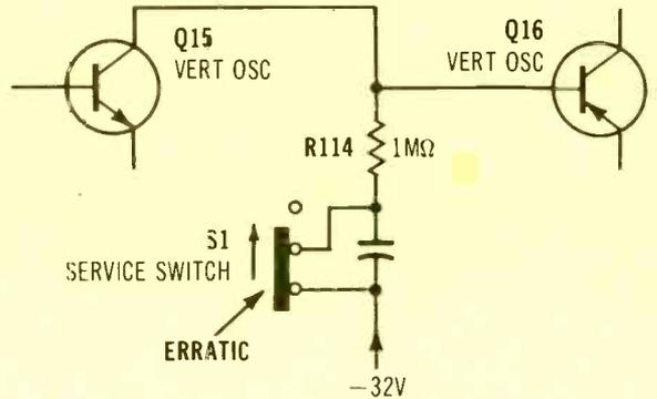
**Symptom –** Erratic vertical roll or loss of height
