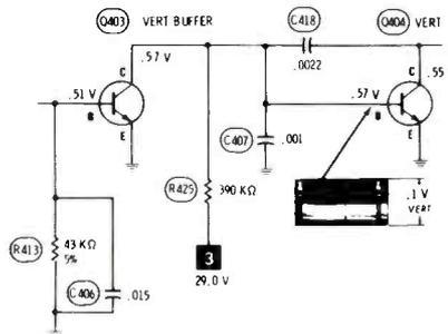
infinity. Even after I removed R425 from the circuit, it tested completely open.
