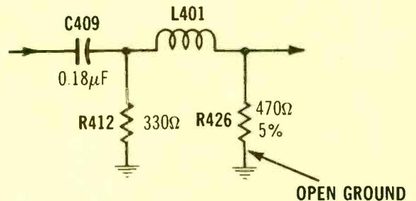
**Symptom –** Intermittent narrowing of picture with flashing lines
