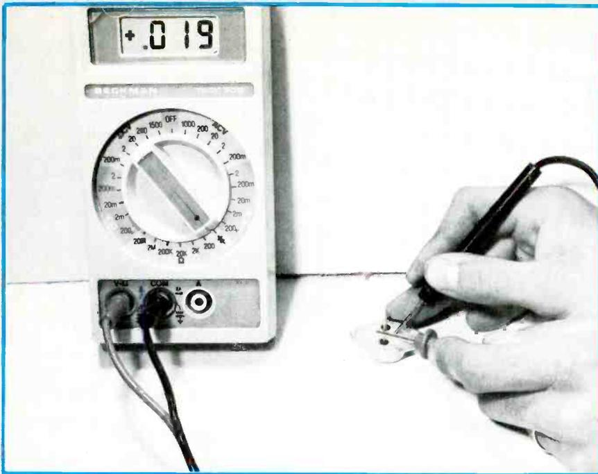
Silicon power transistors should not produce a conductive reading regardless of the polarity of the meter probes with respect to collector and emitter. Some large germanium transistors might show some conduction with one polarity. However, when a low reading (as shown) is obtained with both polarities, the transistor has a collector-to-emitter short.
