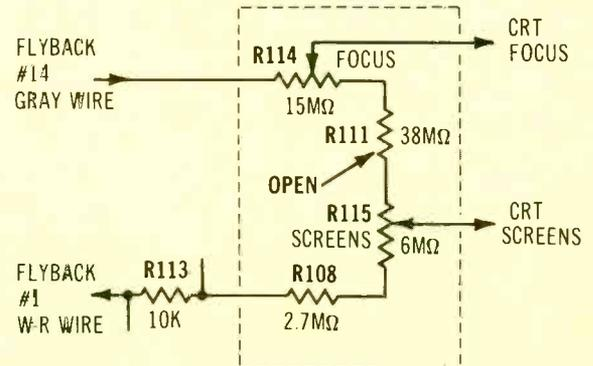
**Symptom –** Dark picture, with no control over focus or screen adjustments
