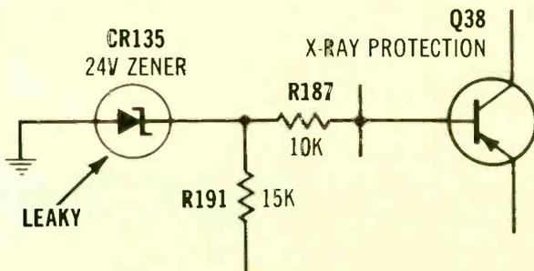
**Symptom –** Shutdown at 120V line voltage, but not at 100Vac
