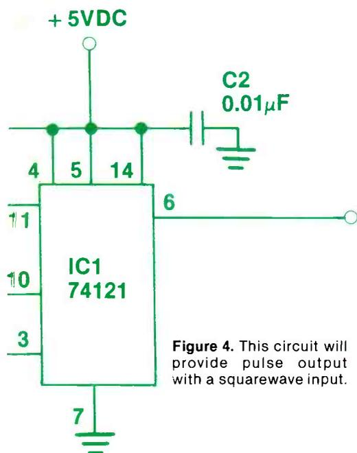
**Figure 4.** This circuit will provide pulse output with a squarewave input.
