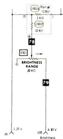
near the kitchen, and I theorize that vapors from cooking settled on the carbon element of the trim pot, eventually causing an open circuit between the wiper and the element.
