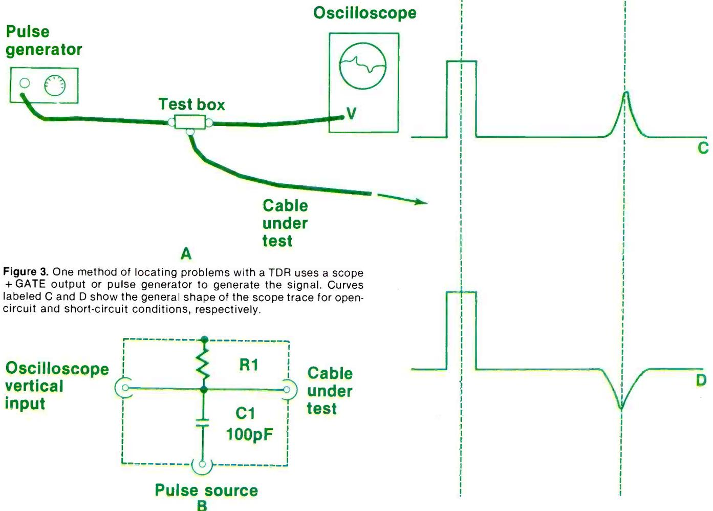
Figure 3. One method of locating problems with a TDR uses a scope + GATE output or pulse generator to generate the signal. Curves labeled C and D show the general shape of the scope trace for open-circuit and short-circuit conditions, respectively.
