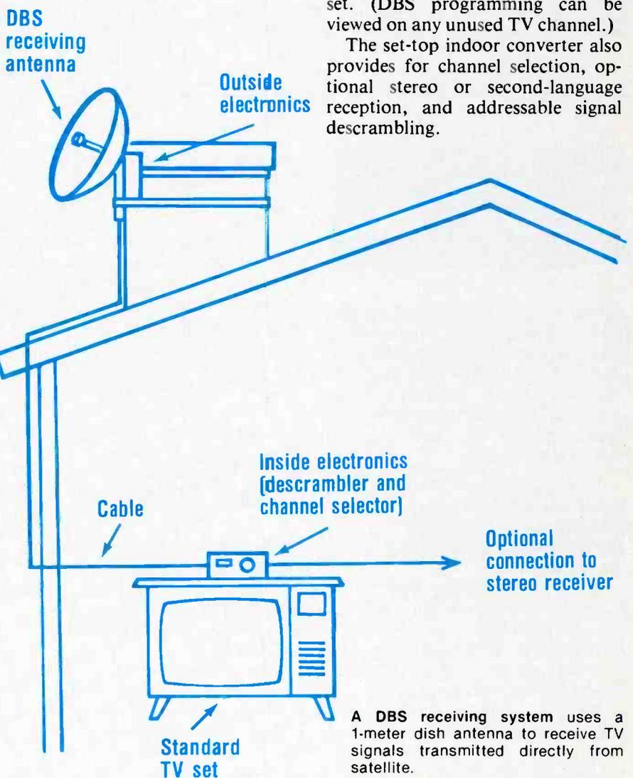
A DBS receiving system uses a 1-meter dish antenna to receive TV signals transmitted directly from satellite.
