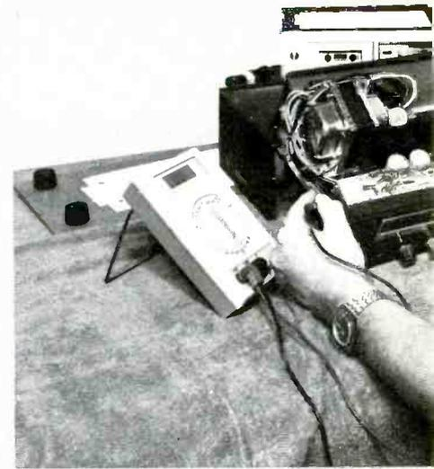
DMMs are recommended for testing the audio stages in AM/FM/stereo radio receivers, especially those meters that have a constant-current voltage-drop type of diode test.
