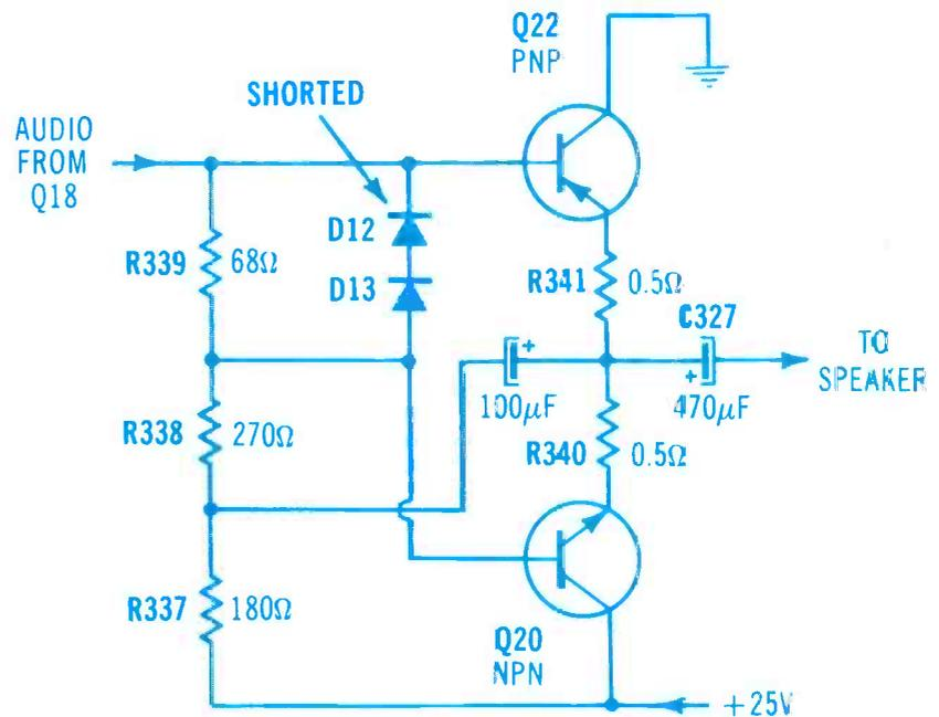
**Figure 5** The bias offset between two complementary power output transistors is very critical if distortion is to be minimized. A shorted D12 bias diode in a Soundesign stereo radio produced a moderate amount of crossover distortion at lower volume levels.
