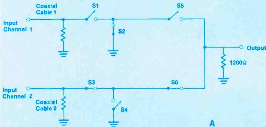
Note: S1 and S2 are a series/shunt switch for Channel 1.
