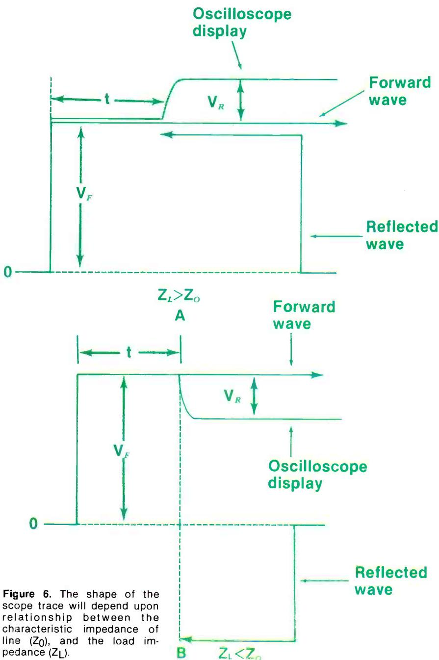
**Figure 6.** The shape of the scope trace will depend upon relationship between the characteristic impedance of line ( $Z_0$ ), and the load impedance ( $Z_L$ ).
