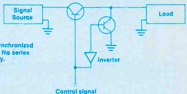
Figure 5. Series/shunt solid-state switch eliminates source and load dependencies inherent with series or shunt switch.
