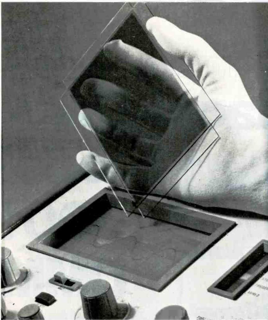
This liquid-crystal, 128-by-256 matrix incorporates the dye-phased change effect to enhance brightness and contrast of a display over a wide variety of ambient light conditions.
