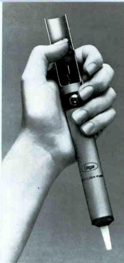
A piston-type desoldering pump can be operated with one hand. The spring-loaded piston is set with the thumb and released by the push of a button, creating a vacuum that draws molten solder into the chamber.
