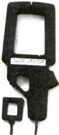
also with any make Snap-Around whose jaws fit the sensor coil with an I.D. of  $\frac{3}{4}$ " x  $\frac{15}{16}$ ". The Multi-Tran extends amperage readings by 10 times, up to 1000A ac, when a maximum of 100A ac is read.
