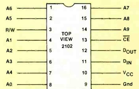
**Figure 1.** Pin-outs for the type-2102 1K-by-1 static MOS RAM. A is an address bit pin, D is a data pin, R/W is a read/write control pin and CE is a chip enable pin. The bar over CE indicates that the active state occurs when the chip enable is 0 (low).
