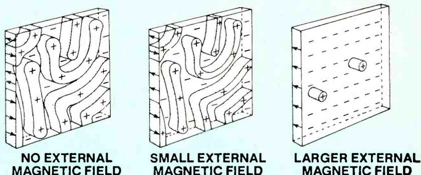
Magnetic domains in thin film under increasing magnetic bias field.
