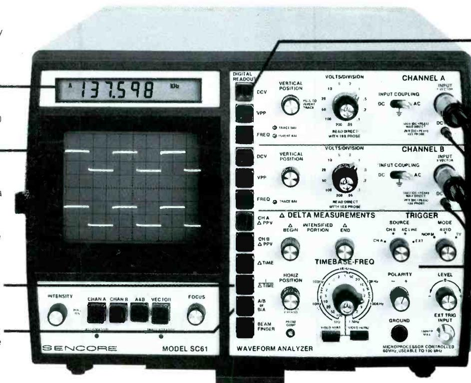
**Autotracking DCV, PPV, Freq:** Measure DCV to .5%; PPV to 2%; freq. to .001%. Just push a button for either Channel A or B.
