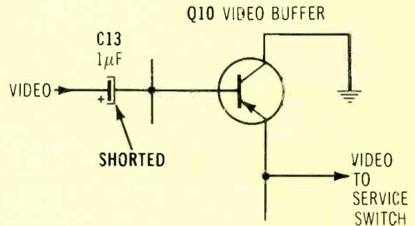
**Symptom** – Excessive brightness with retrace lines
