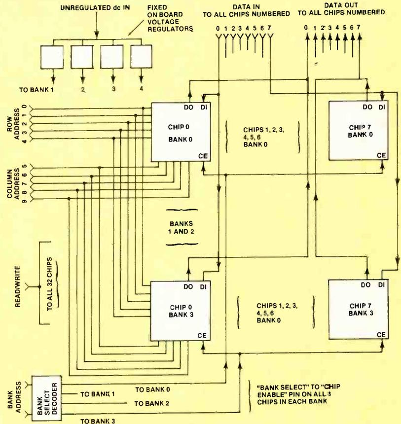
Figure 3. A 4K-by-8 memory organized with 32 1K-by-1 static RAM chips. Chips 1 through 6 in each bank are not shown, and banks 1 and 2 are not shown. *Data in* and *data out* pins on all similarly numbered chips are in parallel. *Chip enable* pins on all eight chips in each bank are in parallel and are used for *bank select* purposes. *Read/write* pins on all 32 chips are in parallel.
