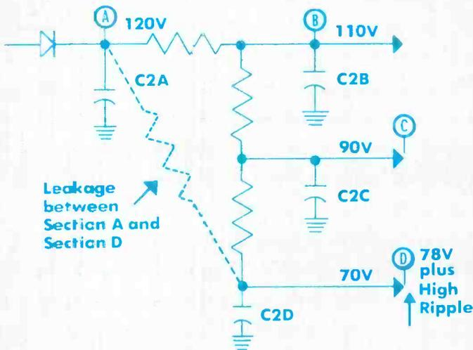
Leakage between sections of a multi-section electrolytic capacitor changes voltages, couples signals and creates odd symptoms in the circuit.
