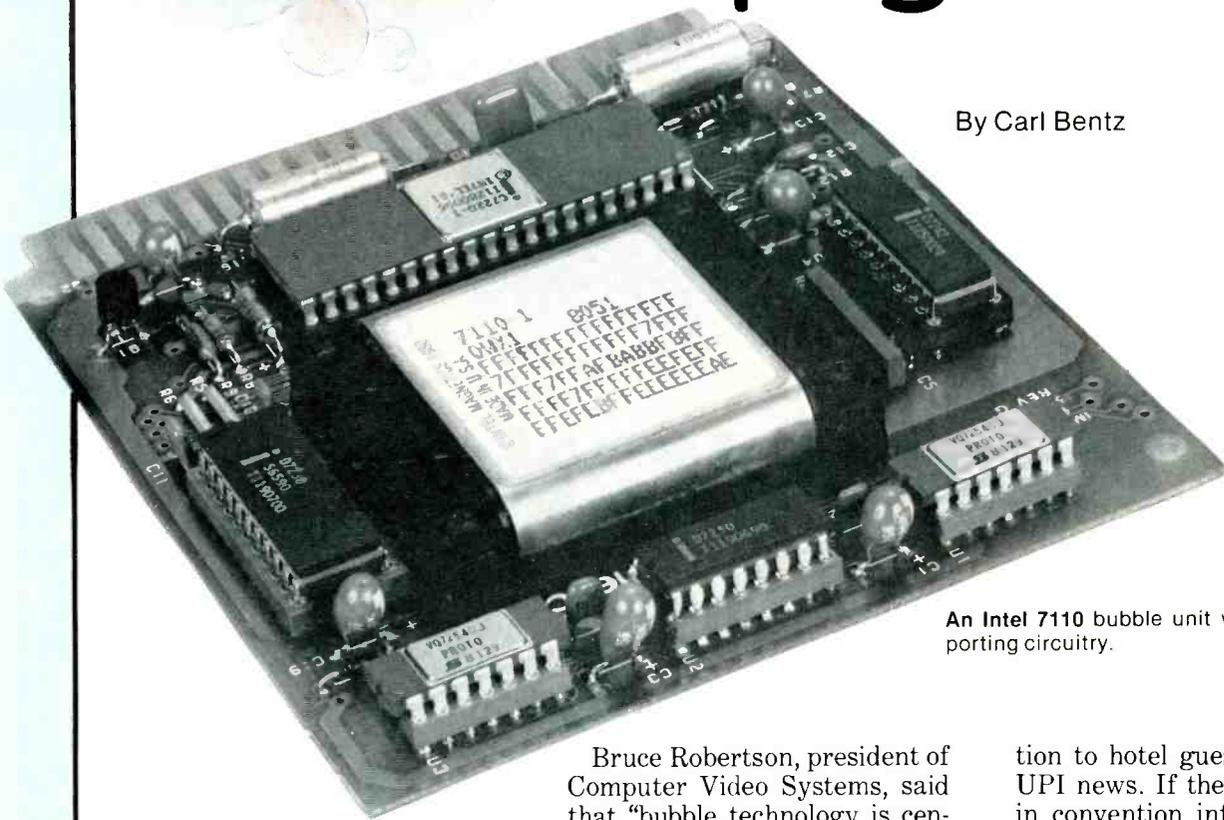
An Intel 7110 bubble unit with the supporting circuitry.
