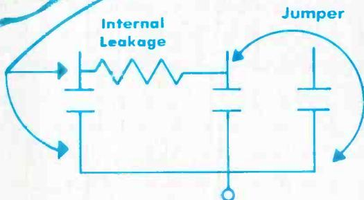
Leakage between sections of a multi-section electrolytic capacitor is indicated by an increase in leakage current when testing one section and a short is connected across another section.
