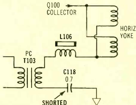
**Symptom** – No sound or raster; receiver in shutdown without high-voltage
