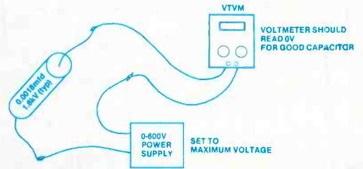
If a capacitor analyzer is not available, you can check a capacitor with a power supply and a VTVM. After an initial surge of the meter, it should drop back to zero.
