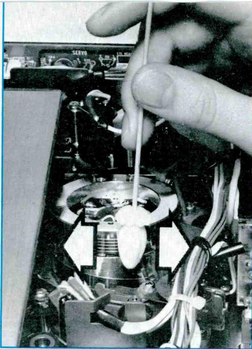
**Figure 11.** Video heads in VHS machines are cleaned by the same side-to-side motion of a cleaning swab soaked in head-cleaner liquid. (Photo courtesy of Nortronics.)
