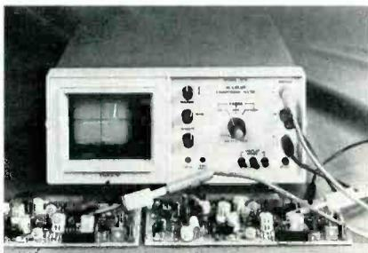
test, and a *compare* mode allows the operator to easily detect the difference between good and bad circuit elements by switching the CRT display at a 1Hz rate.
