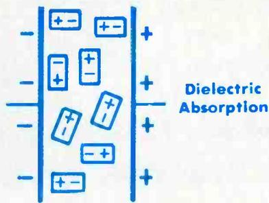
Dielectric absorption is a phenomenon caused when some of the dipoles in the dielectric fail to release their energy when the capacitor is discharged.
