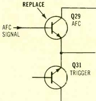
**Symptom** – Incorrect horizontal frequency; cannot be corrected by hold control
