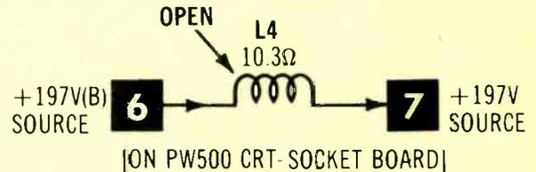
**Symptom** – Excessive brightness with retrace lines, shutdown in a few seconds
