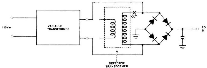
A variable transformer may be used to determine the required specifications of a replacement power transformer when the original unit is defective and no replacement information is available (see text).
