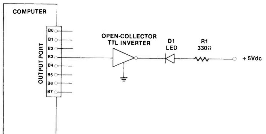
Figure 7. The LED indicator is interfaced to the I/O port through the TTL inverter.
