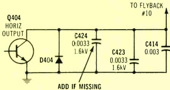
**SYMPTOM** — Narrow picture and excessive 32kV HV
