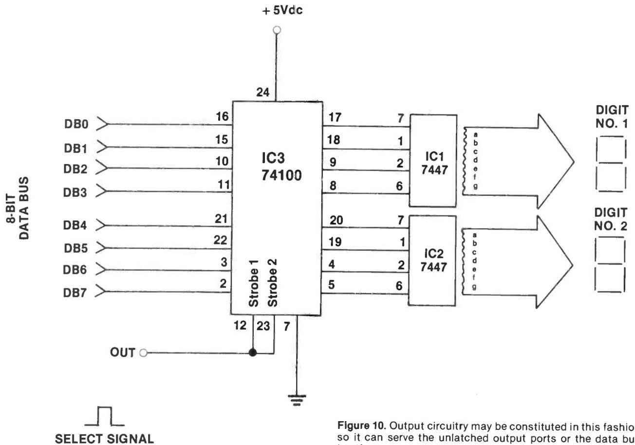
Figure 10. Output circuitry may be constituted in this fashion so it can serve the unlatched output ports or the data bus itself.
