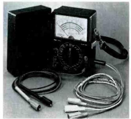
tion tester that includes a transmission line test set, 10-tone generator and a volt-ohmmeter. The model 3 is designed for installation or repair service measurement of power influence, circuit noise, circuit loss or line milliamp checks on telephone company or privately installed cable systems.
