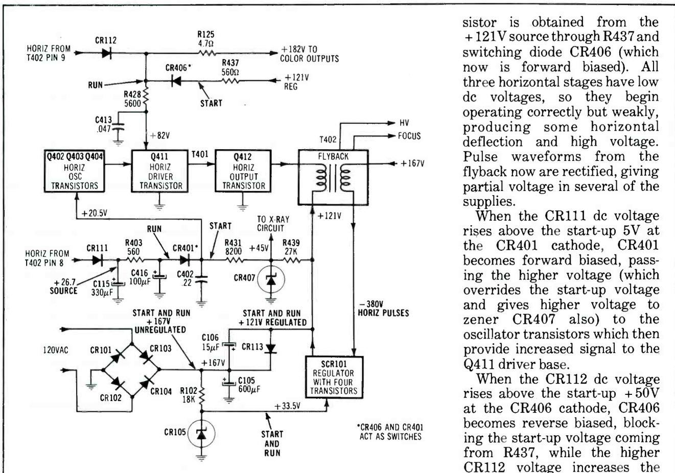
Figure 1. This partial schematic shows several important power supplies.
