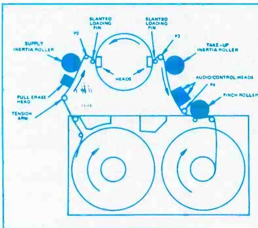
**Figure 8.** This drawing shows the tape path from the cassette, through the machine and back into the cassette.
