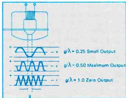
**Figure 2.** When recording-head current is held constant for all frequencies, the amplitude of the playback-head signal depends on flux strength across the head gap. This is in turn dependent on the ratio of head gap to wavelength.
