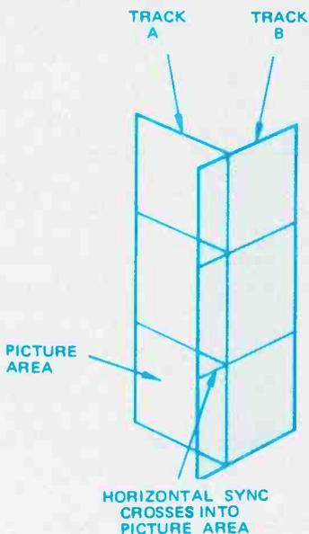
**Figure 13.** The most severe beat produced by track overlap is from the horizontal sync pulses in the luminance signal, because the sync repetition rate does not vary with changes of video waveform and amplitude. These beats are eliminated through interleaving.
