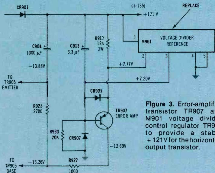
**Figure 3.** Error-amplifier transistor TR907 and M901 voltage divider control regulator TR905 to provide a stable +121V for the horizontal-output transistor.
