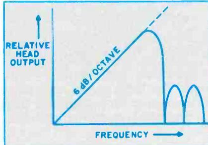
**Figure 3.** Without equalization, this playback response is obtained from constant-current recording. Maximum response occurs at the 2-wavelength point. For frequencies above the peak, the response falls rapidly to a null (zero output) at the 1-wavelength signal frequency.
