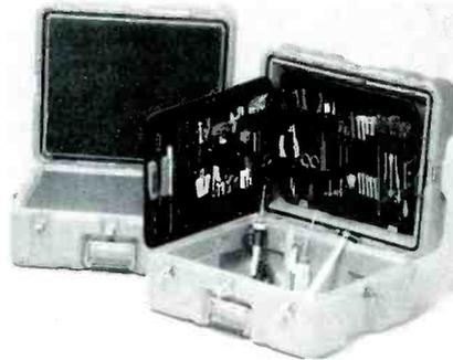
Designed for use in extreme environments, the cases have full parameter neoprene gaskets to seal out dust and water, and recessed stainless steel ¼-inch turn latches that can be secured in transit with 4-inch cable ties. Survivor cases are available with polyurethane foam slabs for protecting instruments, or with two removable tool pallets.
