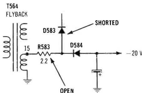
**Symptom** – Only half height, and picture is white with retrace lines
