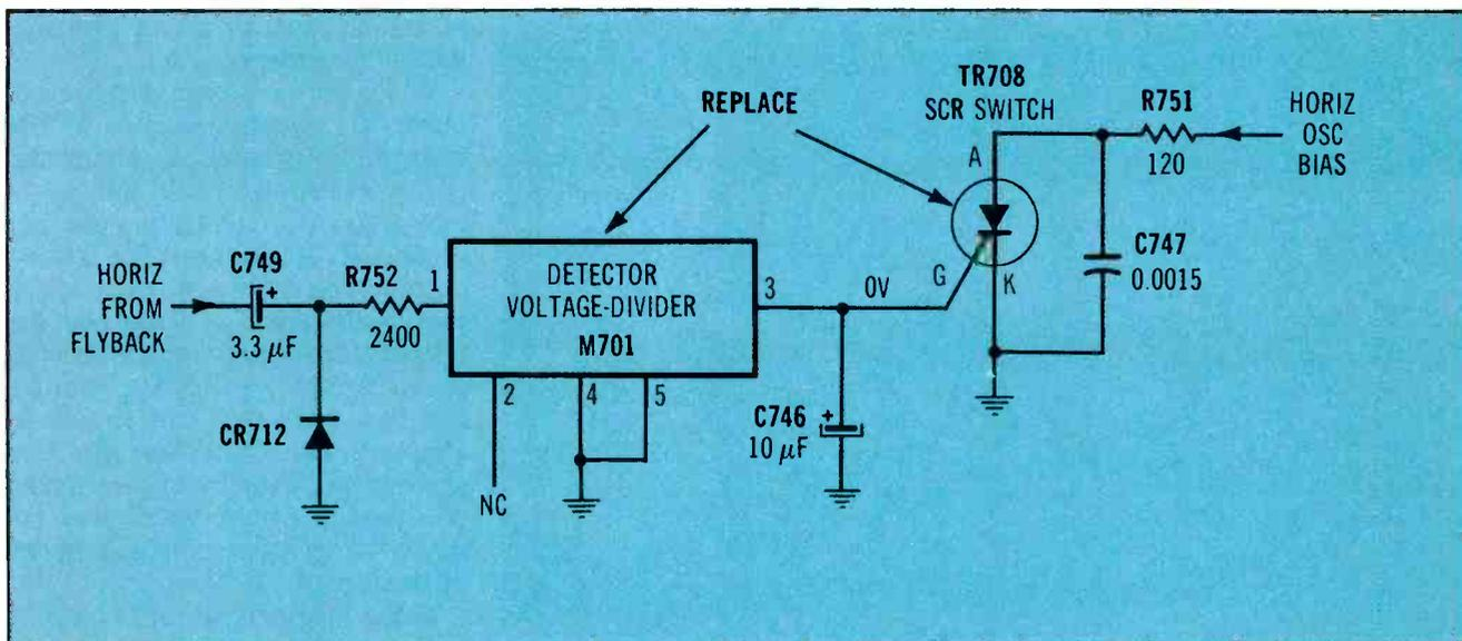
**Figure 8.** Failsafe circuit. Horizontal pulses from the flyback are rectified and applied to M701 detector voltage-divider component. If these pulses become excessive in amplitude, a positive voltage from M701 is applied to the TR708 gate, causing TR708 conduction, which kills the horizontal oscillator.
