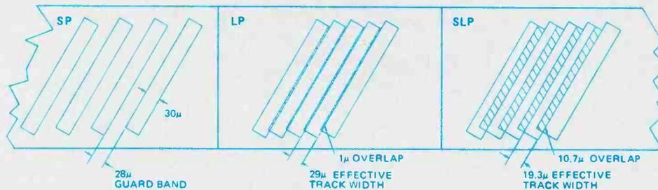
**Figure 12.** With standard play (SP) mode, the video tracks have a wide space between them. In LP mode, there is a slight overlap. A large degree of overlap is produced by the SLP 6-hour mode. Overlapping produces beats, unless corrected.
