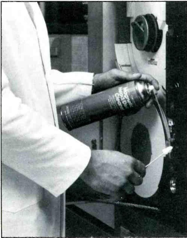
Mixture of Freon TF and isopropyl alcohol under pressure of CO<sub>2</sub> propellant penetrates and flushes away contaminants on magnetic tape or disc heads. The cleaner dries instantly, requiring no wiping and leaving no residue.
