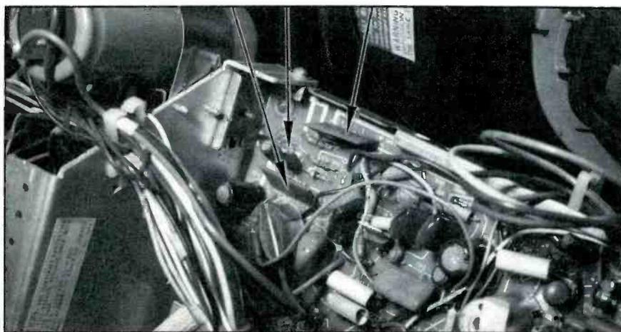
Figure 9. Arrows locate these fail-safe and power-supply components (from the left): M701; TR708 SCR; and M901.
