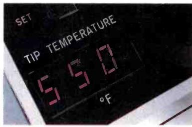
When you need controlled output soldering for sensitive components, you don't need uncontrolled temperature fluctuations at the work station. In the Weller EC Series, the tip temperature is maintained throughout the range of 350°F–850°F to within 10°F. In addition, an electronic system utilizes thyristor power control with zero voltage thyristor drive. This
