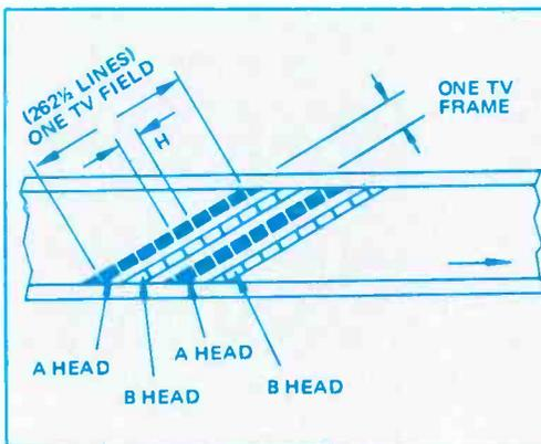
**Figure 6.** Each of the two video heads records a track having 262.5 lines of video. Then each pair of tracks has one complete video frame of 525 lines.
