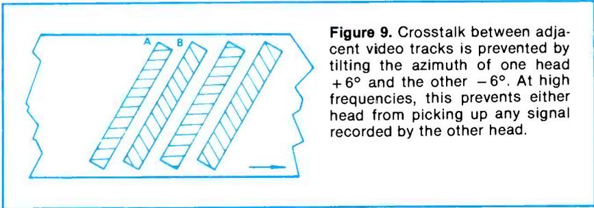
**Figure 9.** Crosstalk between adjacent video tracks is prevented by tilting the azimuth of one head  $+6^\circ$  and the other  $-6^\circ$ . At high frequencies, this prevents either head from picking up any signal recorded by the other head.
