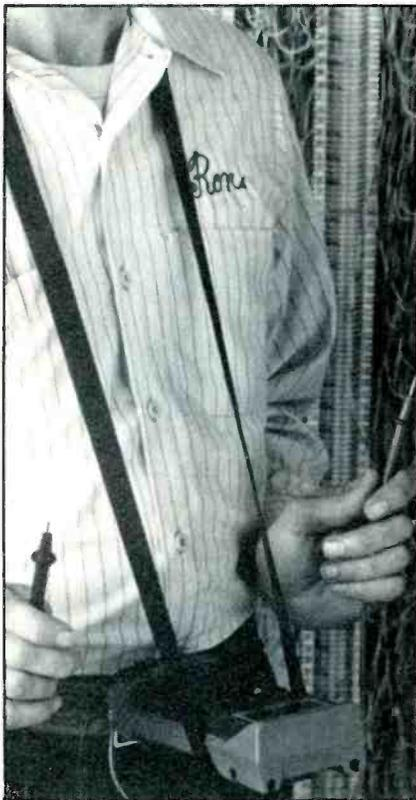
**Figure 6.** A handy accessory is the plastic holster that cradles the model 77 DMM. Grooves and space are provided for storage of the test probes. Two belt loops are provided. One allows the meter to be hung from the belt for transportation. The other loop, with the plastic strap that is pictured, holds the meter out straight where the readouts can be viewed. This no-hands operation is convenient when the test points are difficult to find and to touch with the probes.
