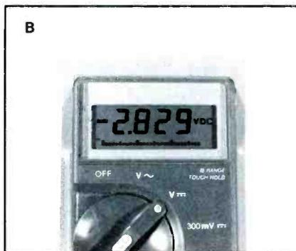
Figure 4. A positive dc voltage (notice the VDC symbol) produces a positive polarity sign on the analog bar graph (A) but no positive symbol before the digital readout. (B) Reversed test probes produce virtually the same digital readout but with negative polarity signs before the digital and analog displays. Automatic upranging occurs slightly above the 3200 count, while downranging occurs at about a 2800 count.
