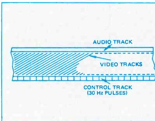
**Figure 7.** VHS machines record one audio track along the top of the tape, a control track for 30Hz pulses along the bottom, and diagonal tracks from the video heads over the center.
