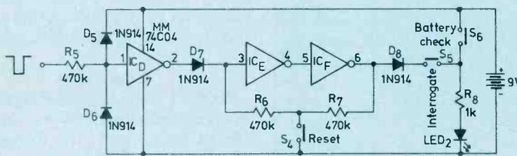
**Figure 2.** A few modifications result in a latch for negative pulses. If both latching circuits are built together from a single MM74C04, the 9V battery and battery check (S3) need not be duplicated.
