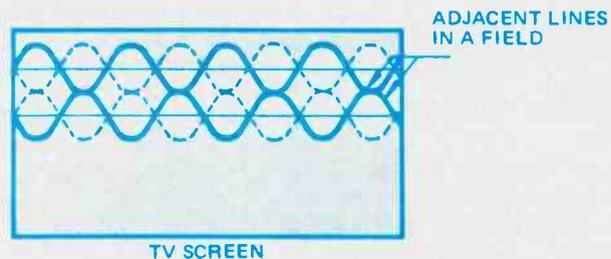
**Figure 14.** Interleaving chroma carriers are shown here. Remember that the top tips of the sine waves produce a brighter raster, and the bottom peaks darken the raster. Therefore, each pair of 3.58MHz sine waves averages to zero change of brightness.
