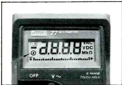
**Figure 2.** During the internal self-test procedure (which model 77 performs immediately after power is applied to the meter), all LCD symbols, digits, decimals and the complete bar graph are made visible. The arrow points to the manual range-advance symbol on the LCD display. The same symbol is used by model 77 to show when Touch Hold is activated.
