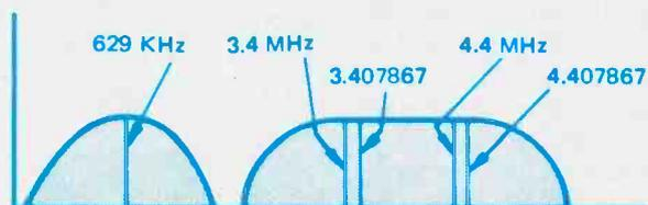
**Figure 15.** These are the VHS frequencies after addition of the 7867Hz frequency offset that removes the sync beats by making the interference an interleaving frequency. See the text for a more complete explanation.
