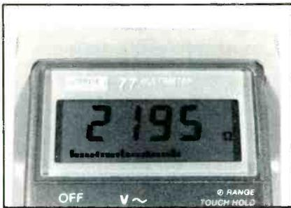
**Figure 5.** A 2200Ω resistor tested 2195Ω on the 3200Ω resistance range. Notice the corresponding analog bar-graph indication, and the ohms symbol at the right.
