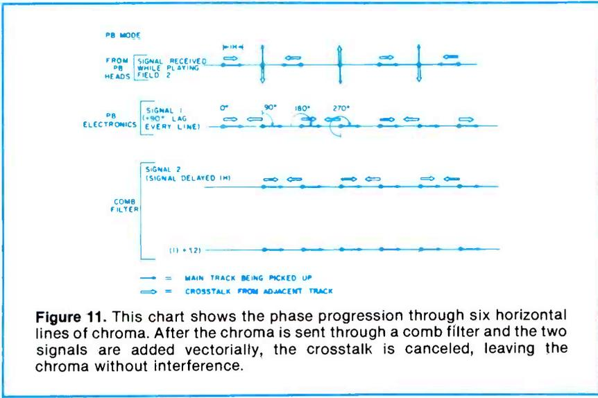
**Figure 11.** This chart shows the phase progression through six horizontal lines of chroma. After the chroma is sent through a comb filter and the two signals are added vectorially, the crosstalk is canceled, leaving the chroma without interference.
