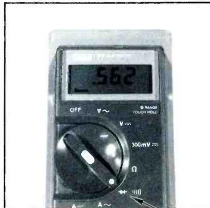
Figure 3. The diode symbol with the audio-sound symbol identifies the combined voltage-drop diode (and transistor junction) test and the continuity indication. Both tests have an audio tone or a tone chirp under certain conditions.
