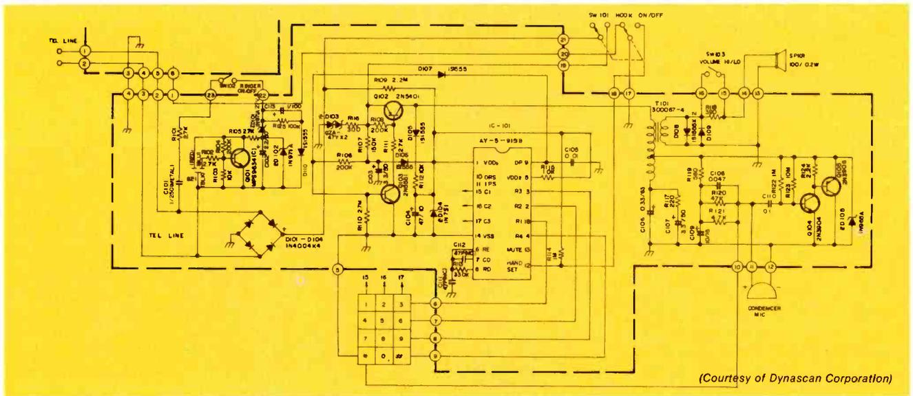
**Figure 3.** The schematic diagram of this phone illustrates its all-electronic nature. The IC in the center generates dialing pulses and stores the last dialed number for redial.
