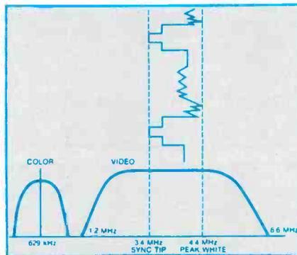
**Figure 4.** Equalization is made easier by moving the 4MHz bandwidth up higher in frequency. VHS machines record the luminance signal as an FM carrier whose frequency changes according to amplitude variations. The color sidebands are separated and recorded at 629kHz.
