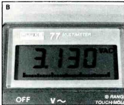
**Figure 1.** Length of the analog bar graph (below the digits) depends on the input signal relative to the range of the digital display. (A) A 3.13Vac signal displayed on the 32Vac range produces a short analog graph of less than 10% of a complete bar graph. A voltage of 16V should produce a 50% bar graph, etc. (B) The same 3.130Vac voltage produces a complete bar graph when the 3.2V range is selected. Notice the Vac symbol that shows the ac-voltage function has been selected.
