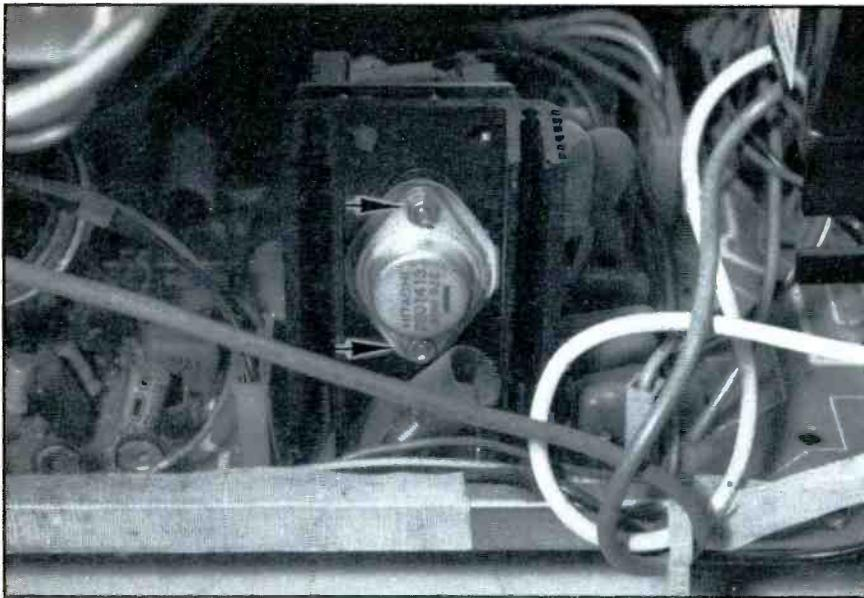
**Figure 7.** Two nuts (located by arrows) must be removed and the base and emitter leads unsoldered from a small circuit board before TR704 horizontal-output transistor can be removed from the chassis.
