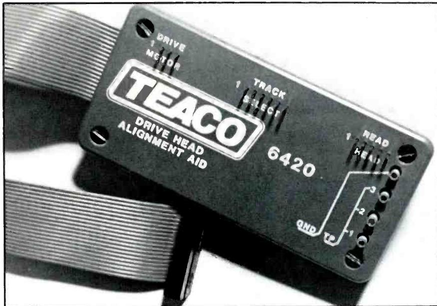
**Figure 4.** TEACO (Terry Electronic Assembly Company) is introducing the 6420 Drive Alignment Aid, which is designed to assist in radial head alignment of the 1451 drives of Commodore 64 and VIC 20 computers. Hookup with either a single channel or dual channel scope.
