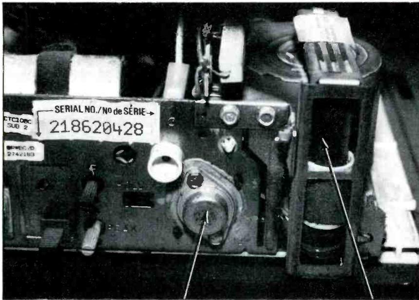
Suspect shorted turns in the flyback transformer when the receiver shuts down quickly and the horizontal-output transistor case feels warm, indicating that it has been carrying excessive current. Often this indicates damage to the transistor as well. Once you have installed a new horizontal-output transistor, use a variable-voltage transformer to operate the receiver at lower ac line voltage while you identify and correct the problems.
