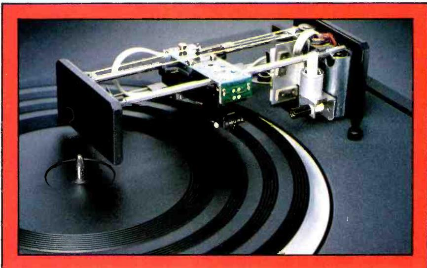
slippery polymer material, glides over the surface of the record, propelled by a pulley-driven cord. The motion is provided by a micro-computer-controlled servomotor.
