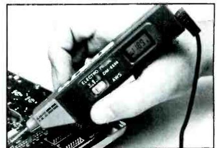
At 6<sup>3</sup>/<sub>8</sub>"x11<sup>1</sup>/<sub>8</sub>"x3<sup>3</sup>/<sub>4</sub>", the DM-6590 is a miniaturized instrument that fits comfortably in the hand and contains a built-in probe tip for one-hand operation. It is designed for reading ac voltage, dc voltage and resistance in tight, hard-to-reach areas such as crowded circuit boards.
