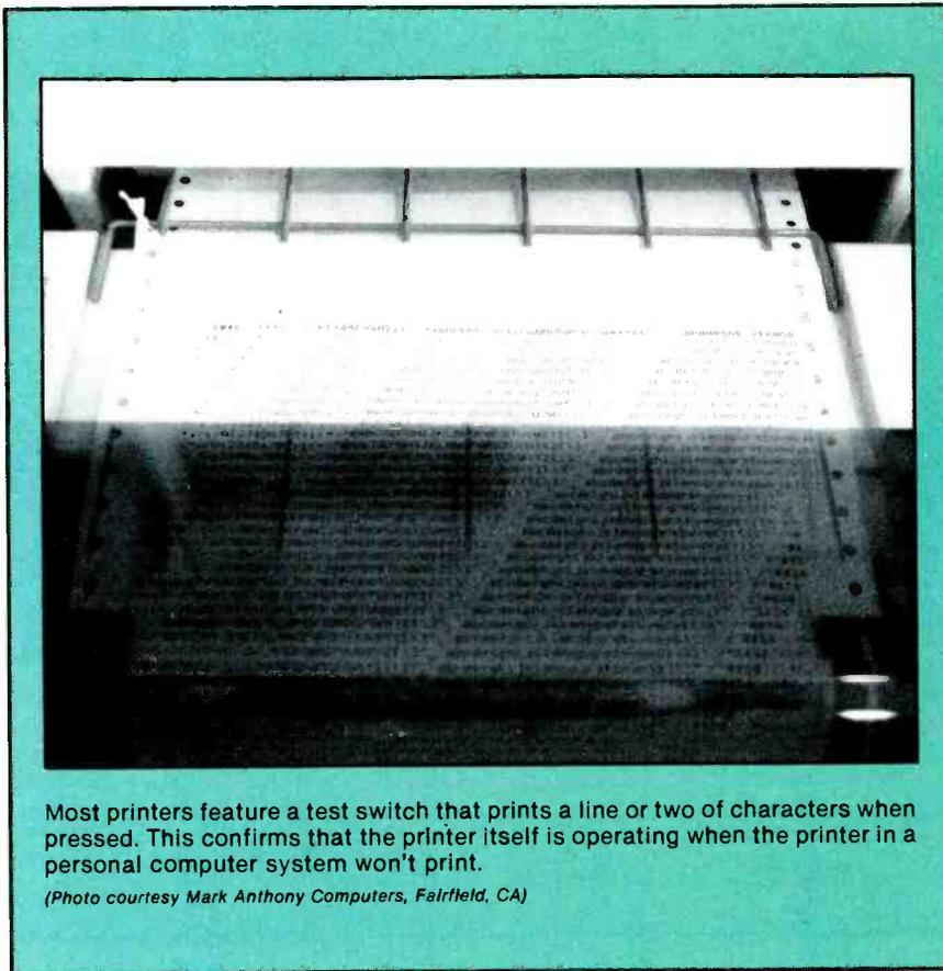
Most printers feature a test switch that prints a line or two of characters when pressed. This confirms that the printer itself is operating when the printer in a personal computer system won't print.
