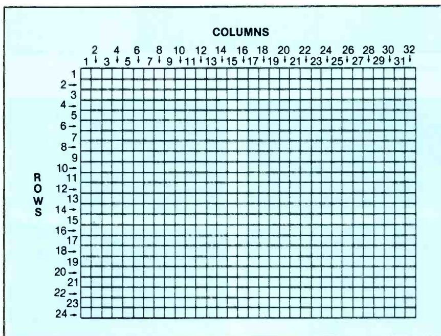
Figure 2. Row and column layout of the TI 99/4A video screen
