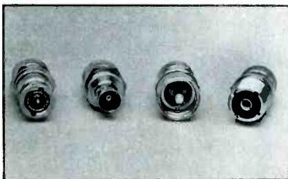
These connectors accommodate popular cable sizes such as RG58, RG59 and RG62 up to RG6U. Solid, foam and air dielectric cables can be used. The center contact has a spring member that accepts the variation in conductor sizes. Maximum jacket size acceptable is about 0.275, depending on the cable braid thickness because the braid is folded back over the jacket before insertion of the cable into the connector.
