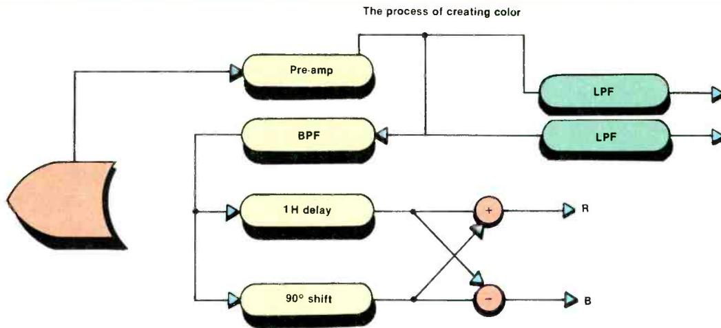
**Figure 3.** The camera electronics performs amplification, filtering, delay and frequency shift to convert the output signal from the scanning process into color, luminance and resolution information components.
