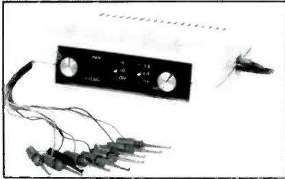
MX-8 features include: a frequency range to 5MHz; 40Vpp input range; analog and digital compatibility, including CMOS and overvoltage protection to 100V. It comes with an ac adapter, and nine E-Z-HOOK probes for quick and simple positive connections.
