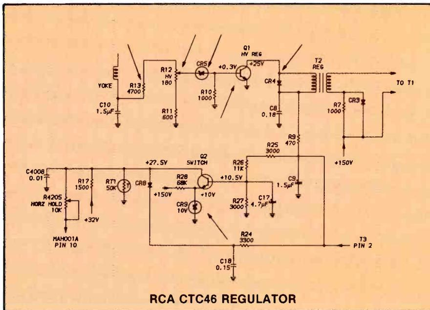
Figure 4. Arrows point to the components most likely to produce excessive high voltage in RCA CTC46A chassis (Photofact 1278-3). Suspect R13, R12, CR5, CR4, Q1 and T2 if the high voltage cannot be adjusted. Or, check Q2 and CR9 if the HV can be adjusted correctly, but the horizontal hold cannot be locked. In this older model, excessive HV or a shutdown-circuit defect changes the horizontal frequency so much that the hold control cannot lock the picture.
