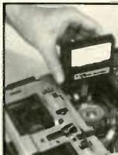
**Video Head Protrusion Gauge:** Universal, fast, safe method of measuring the amount of video head tip wear. Measures in microns and thousandths of an inch. Allows accurate predictions of remaining head life. Head wear provides useful information regarding VCR condition and wear on other components. Stop guessing about head wear. Accessory "S1" stand allows use on any VCR.
