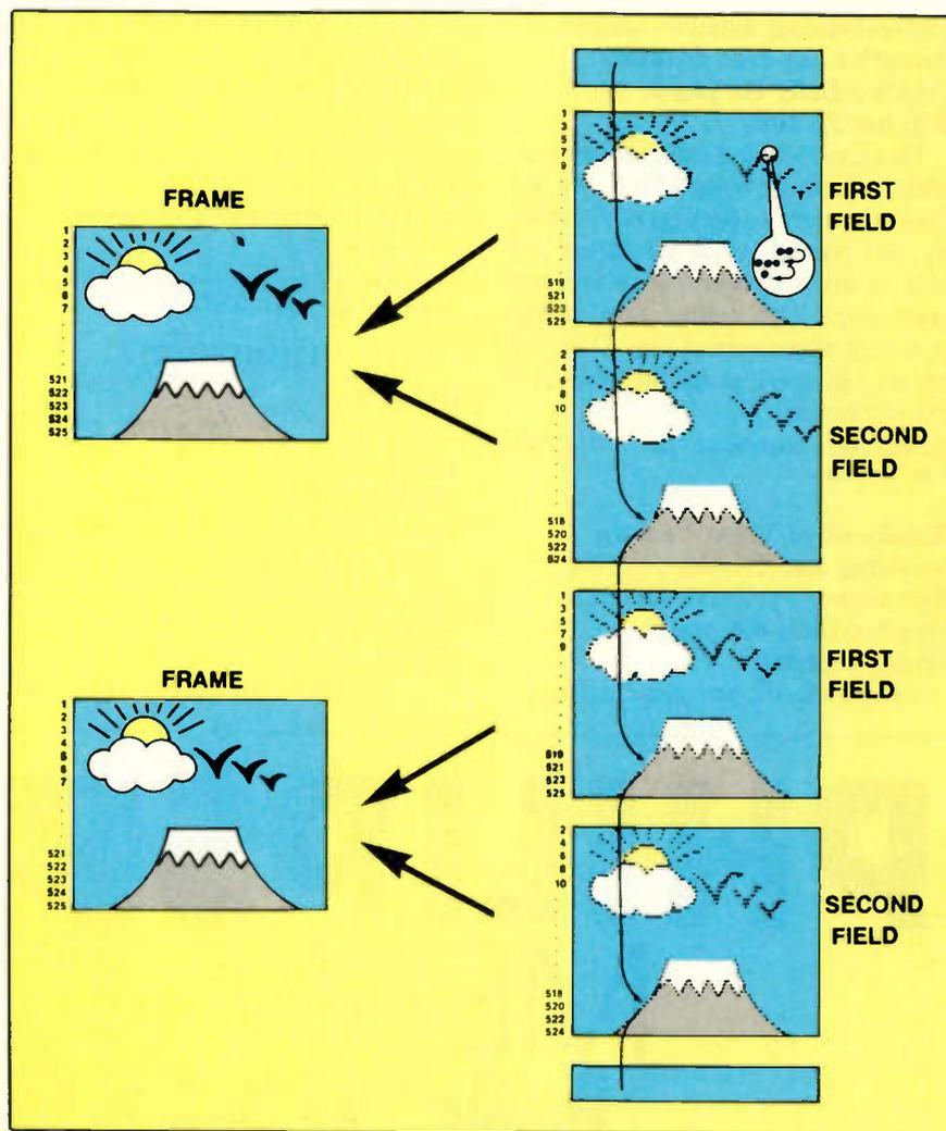
**Figure 1.** In frame double scanning, flicker is eliminated by filling in the gaps between the scanning lines in the two fields that make a frame. The static images (in this case, the mountain) are filled with the appropriate pixels of the previous field stored in frame memory chips. The mobile images (the flying birds in this example) are filled with the same pixels just scanned in the previous scanning line stored in the line memory chip.
