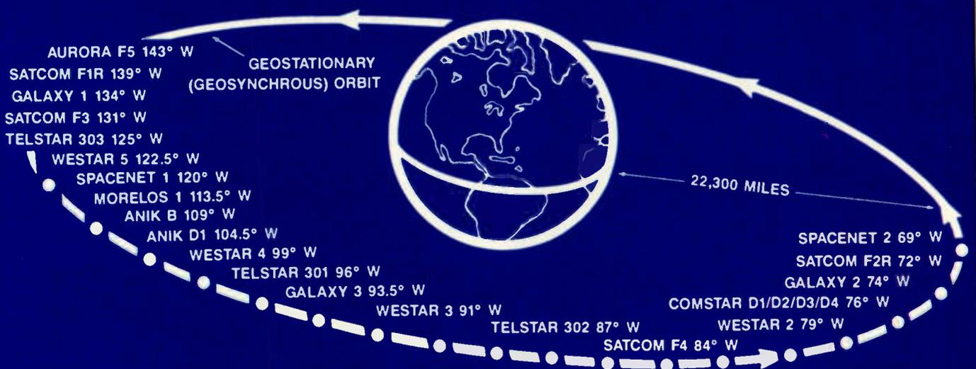
Figure 1. All of the domestic television satellites are located in an orbit directly about the earth's equator between 69° west longitude and 143° west longitude. Because their orbital speed just matches the rotational speed of the earth, each one is, in effect, stationary above a point on the earth.
