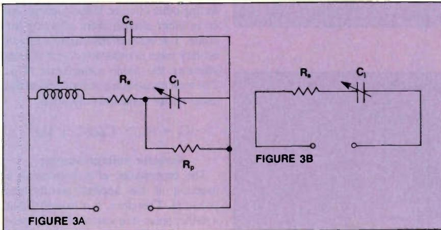
**Figure 3.** The equivalent circuit for a varactor: Figure 3A shows the actual model circuit; Figure 3B shows one that is simplified but, nonetheless, valuable to understanding the varactor's operation. The equivalent circuit in Figure 3B is based on the assumption that certain parameters shown in Figure 3A are negligible.
