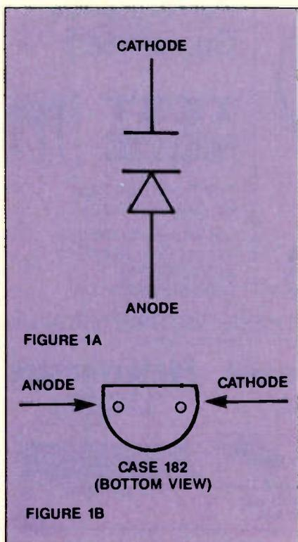
**Figure 1.** Figure 1A shows the usual circuit symbol for varactors. In some cases, the "capacitor" at the top end of the "diode" symbol has an arrow through it to denote variable capacitance. Varactors come in several different standard diode packages, including the 2-terminal "sorta-like-transistor" Type 182 package shown in Figure 1B.
