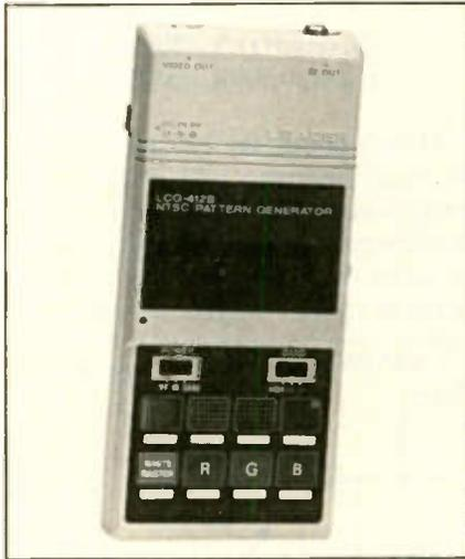
weighs less than 14 ounces, including six AA power cells, and features 75% color bars, dot, crosshatch and full raster signals of 100% white, red, green and blue. The unit features RF output on U.S. broadcast VHF and UHF channels in addition to  $IV_{pp}$  video output into a  $75\Omega$  load.
