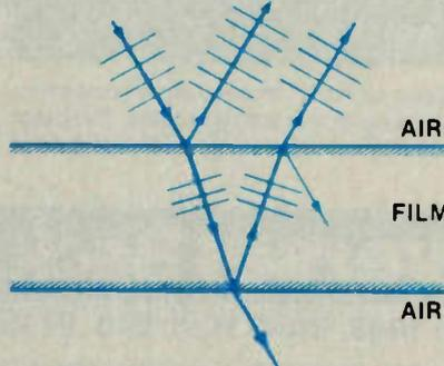
The angle of incidence is equal to the angle of reflection, both measured from the normal, which is a line meeting the reflecting surface at an angle of  $90^\circ$ .
