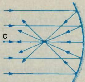
A convex mirror causes light to be reflected divergently toward its source. A virtual image appears behind the mirror.
