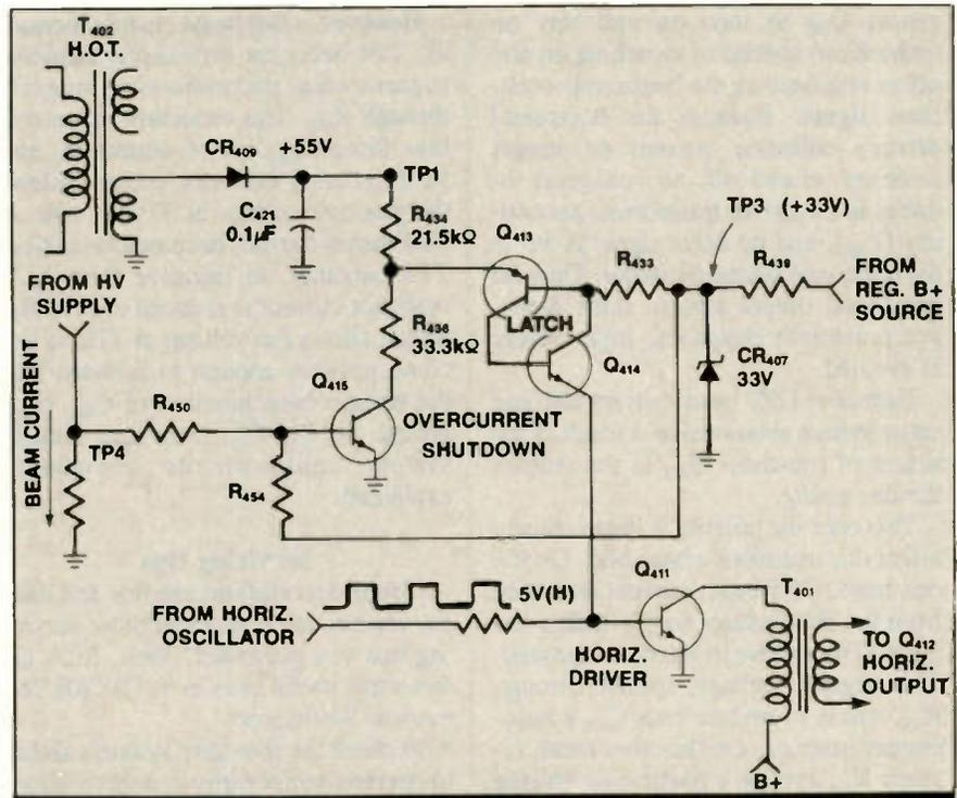
Figure 2. The protection circuitry in this RCA CTC108 chassis schematic disables the horizontal deflection system by cutting off the horizontal drive if either high voltage or beam current increases beyond certain limits. Transistors Q<sub>413</sub> and Q<sub>414</sub> form an x-ray protection latch, and transistor Q<sub>415</sub> senses excessive CRT beam current.
