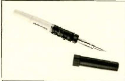
use as either a soldering iron or a hot-air gun. The 4.4-ounce unit can operate for about three hours per butane fill up. Varying the gas flow controls the temperature, which ranges from 650°C to 1,202°C when the unit is used as a hot-air gun, and 250°C to 500°C when it is used as a soldering iron.
