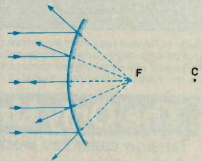
A concave mirror causes light waves to be reflected and converged at a focal point in front of the mirror.
