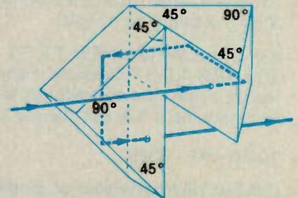
Although rarely used in TV optics, the double Porro prism with  $45^\circ$ - $45^\circ$ - $90^\circ$  angles allows realignment of light for easier viewing in high-quality binoculars.
