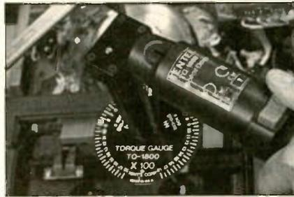
torque driver simulates the 9.5cm/sec U-Matic tape pulling speed. Torque measurements may be made either clockwise or counter-clockwise directly on the supply or take-up spindle.
