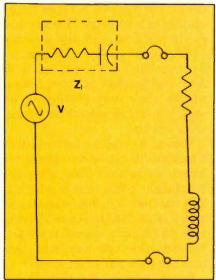
**Figure 3.** In the case of an ac circuit with a capacitive internal impedance, in order to transfer the maximum power to the outside world, make the load resistance equal to the internal resistance and use an inductance to resonate with the internal capacitance so that you have a series resonant circuit.
