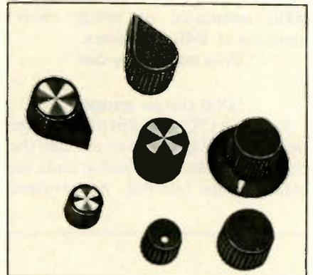
Mil-spec knobs, which are made of polycarbonate, are manufactured in 26 variations of the five most widely used styles and are available in 0.125 and 0.250 diameters. The commercial knobs, made of ABS thermoplastic with spun aluminum inlays, are available in 32 variations of the six most popular styles and come in 0.125 and 0.150 shaft diameters.
