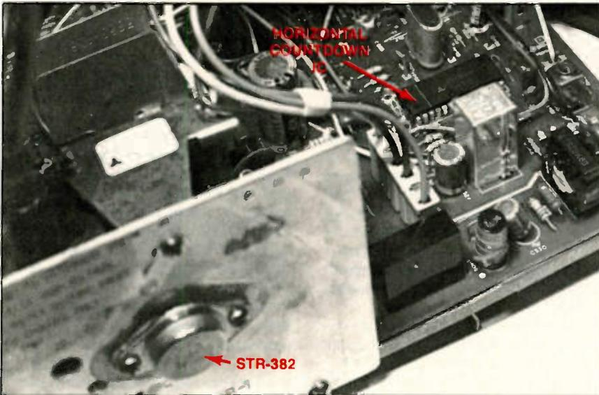
When the low-voltage-regulator output is normal but the horizontal circuits are overloading, scope all waveforms at the horizontal countdown IC and the driver circuits that follow. The basic problem must originate in the horizontal circuit, so keep on testing there.
