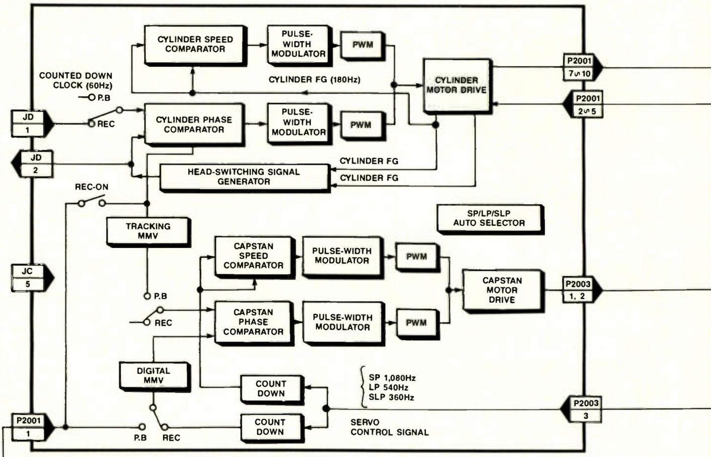
correct. The speed at which the tape is fed past the heads must also be correct, so signals recorded on the tape during record are fed to the capstan along with video-head speed and position information during playback to keep the video heads tracking accurately over the video tracks.
