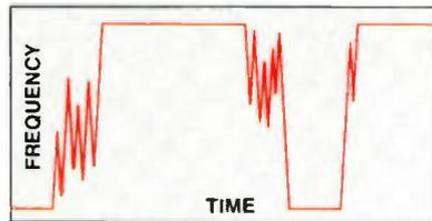
**Intermittent alert.** A key application of audible readout. The HD 153 pinpoints intermittents by emitting a "crackling" sound when they're detected. The response sounds in about 1 msec—far faster than the information appears on any DMM display.
