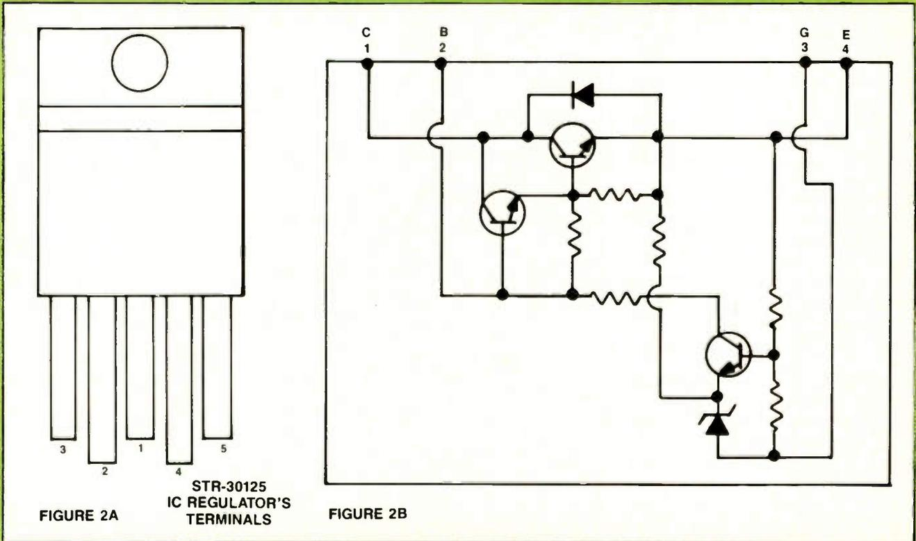
Figure 2. Except for the five terminals instead of the usual three (Figure 2A), STR-30125 regulators resemble TO-220 types often used for vertical-output transistors. An equivalent of the IC's internal circuitry, using transistors, diodes and resistors, is shown in Figure 2B.
