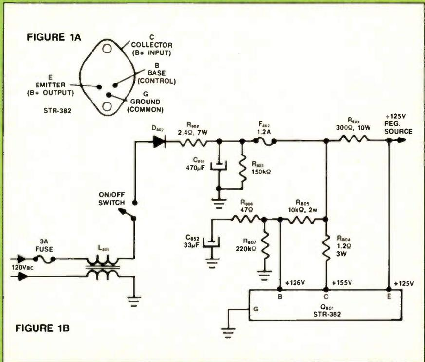
Figure 1. Q<sub>801</sub>, the B+ IC regulator of the Samsung CT-333KA portable, has the physical appearance of a horizontal-output transistor, except it has three terminals, not the usual two (Figure 1A). However, the STR-382 IC probably contains diodes, transistors and resistors in addition to the power transistor. A B+ adjustment control or an external voltage-stabilizing zener diode is not required, according to the Figure 1B schematic.
