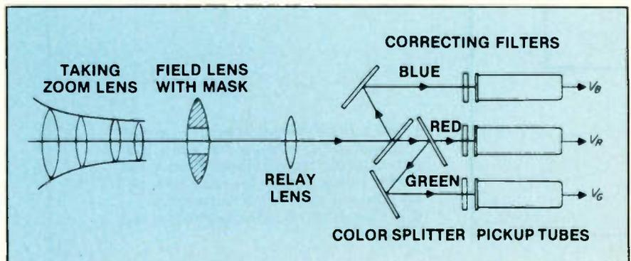
**Figure 1.** Dichroic mirrors may be used to separate a full color image into red, green and blue images for the pickup tubes.
