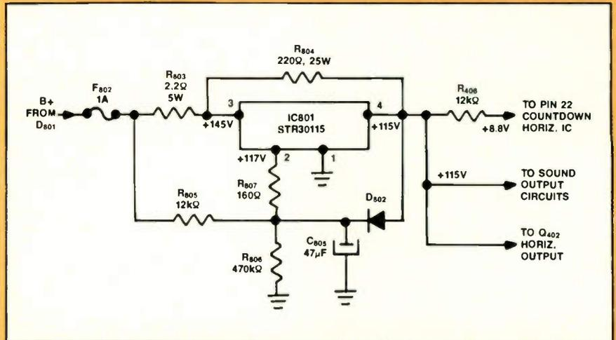
Figure 3. Regulated output voltage of +115V from IC<sub>801</sub> (STR-30115) provides voltage for the sound and horizontal circuits. During start-up, +8.8V for the horizontal countdown IC pin 22 is brought through R<sub>406</sub> from the +115V supply. Troubleshooting circuits that have IC voltage regulators is very similar to troubleshooting others without ICs except that several components are not available for testing, and terminal-to-terminal IC tests show unusual readings.
