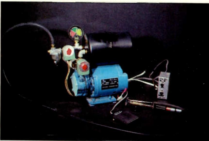
In the first system constructed, the pump is on the bottom. The tank is above, supported by the connecting pipe. This particular tank had two outlets, which were both used, so only one tee was required (visible under the gauge). The control box, on the right, is mounted to a leg of the workbench, while the pump unit sits on the floor under the bench. The footswitch and iron are visible in the foreground.
