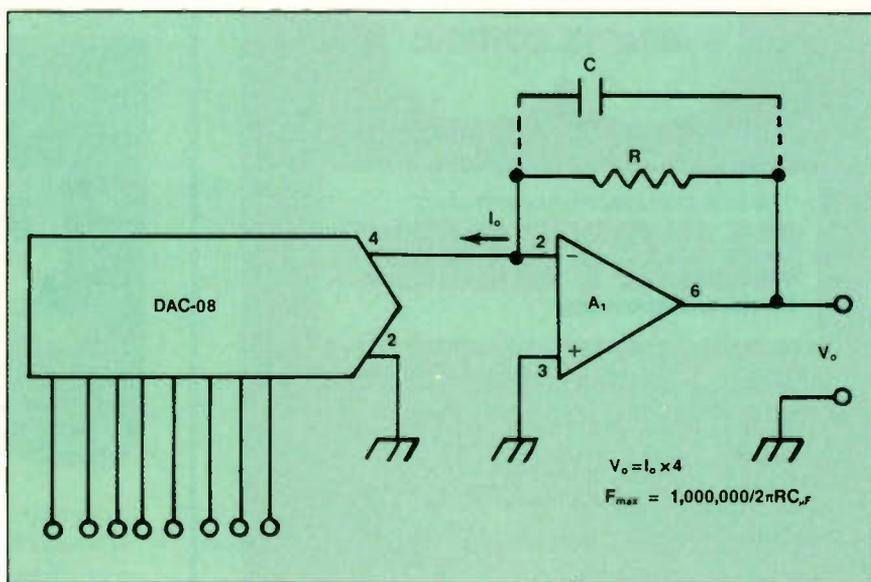
**Figure 1.** A simple method for converting  $I_o$  to an output voltage ( $V_o$ ) with a low output impedance (less than  $100\Omega$ ) is to use an inverting follower operational amplifier. The output voltage is simply the product of the output current and the negative feedback resistor:  $V_o = R \times I_o$ .
