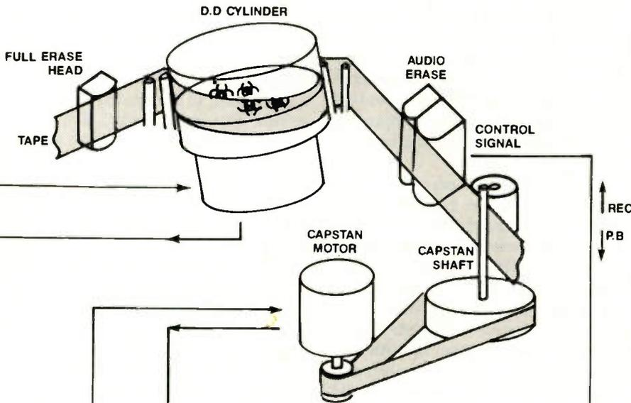
Figure 1. Noise that travels through the playback picture may be caused by a dirty, mis-adjusted or disconnected control head. In this particular case, absence of a linear audio signal isolated the problem to audio/control. (Block diagram courtesy Thomson Consumer Electronics.)
