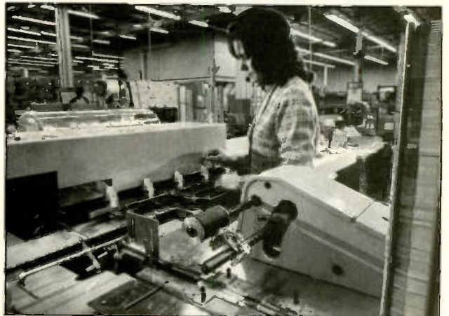
In this operation, ECG replacement semiconductors are packaged in boxes by equipment that imprints type numbers and basing diagrams on the individual cartons. The machine indexes 40 times per minute and can accommodate all semiconductor carton sizes.
