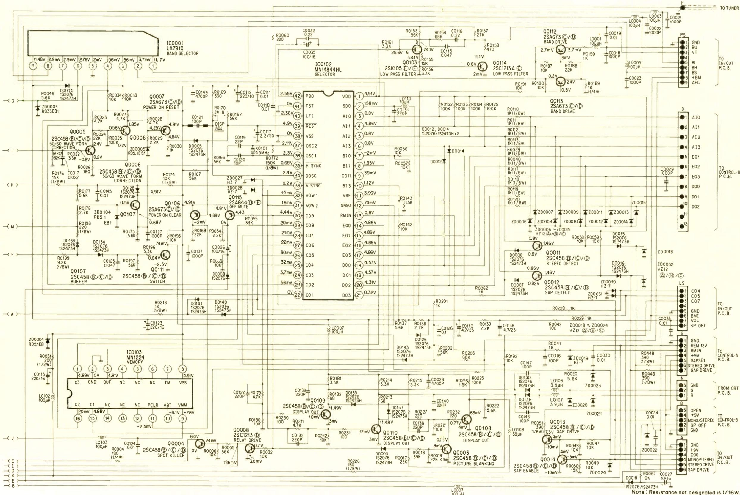
Product safety should be considered when component replacement is made in any area of a receiver. The shaded areas of the schematic diagram designate sites where safety is of special significance. It is recommended that only exact cataloged parts be used for replacement of these components.
