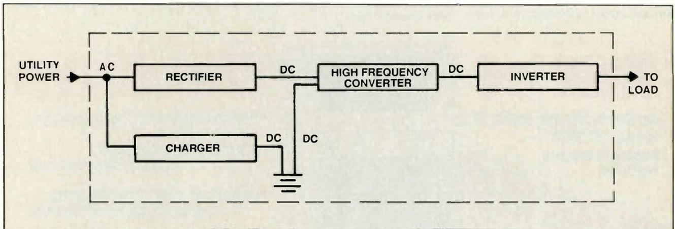
**Figure 6.** Newer generation UPS systems provide on-line topology with a sine-wave output generated by a high-frequency, PWM inverter. A low-impedance filter replaces the output transformer. These units can be smaller, lighter and nearly the same price as off-line and hybrid systems.
