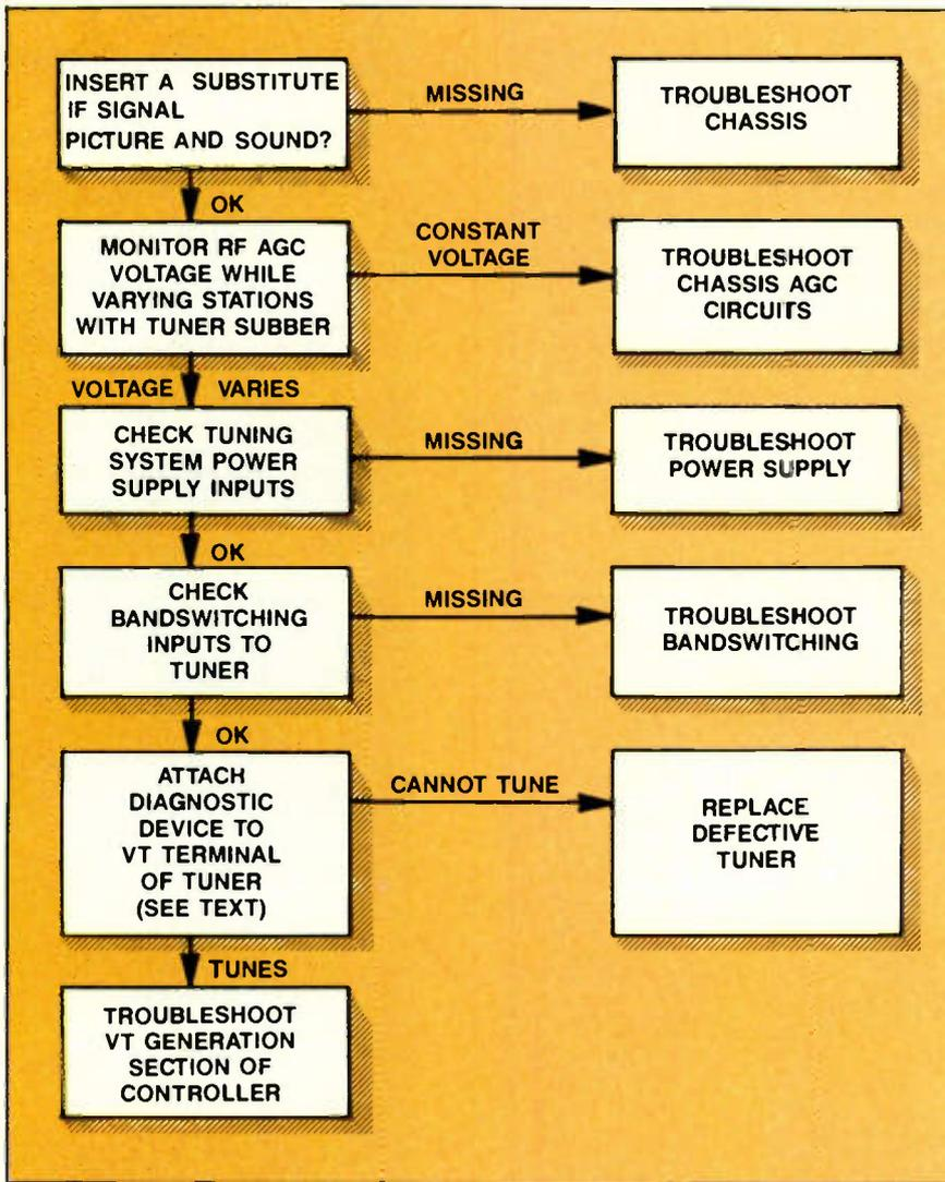
**Figure 2.** When troubleshooting voltage-synthesis tuning systems, first try reprogramming. If this is unproductive, follow the general steps outlined in this general flowchart to verify that the problem is indeed in the tuning system.
