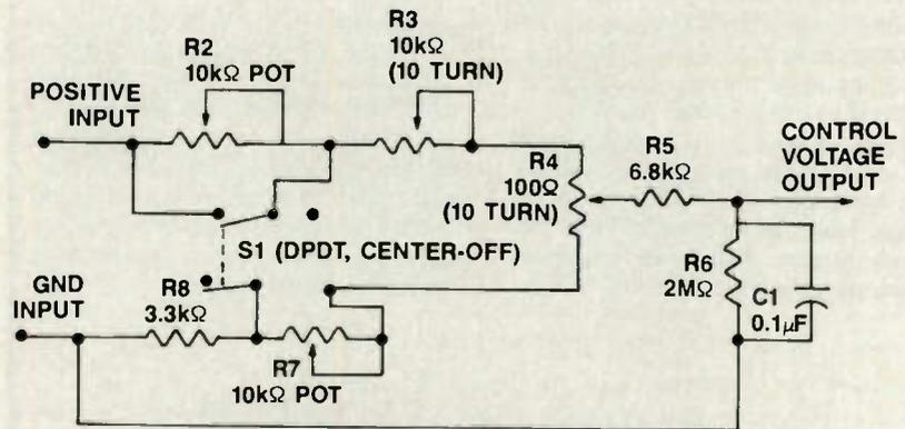
NOTE: S1 IS SHOWN IN THE HIGH POSITION. IN RUN POSITION, BOTH SECTIONS OF THE SWITCH ARE OPEN (CENTER-OFF).
