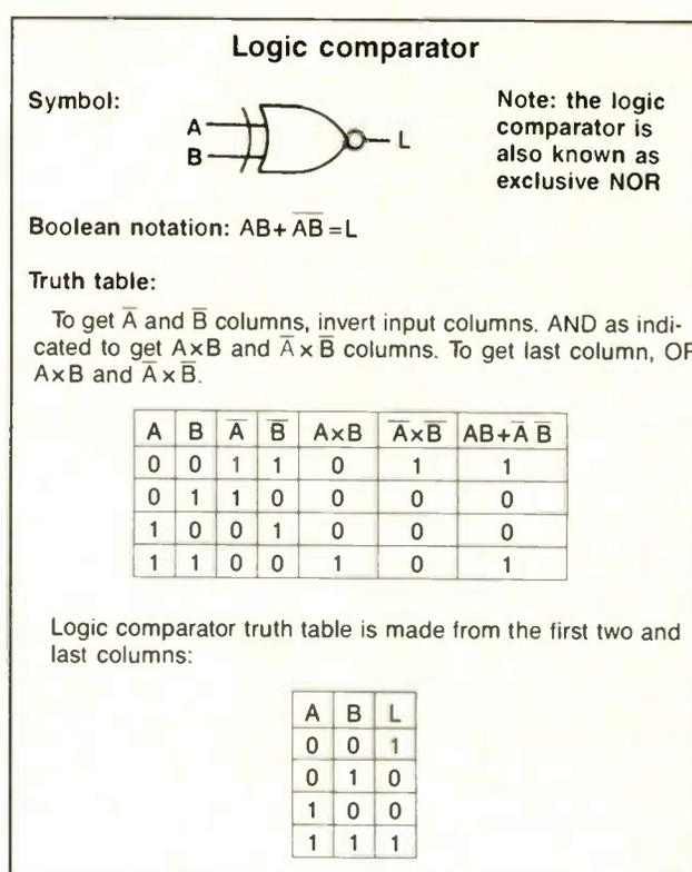
**Figure 4.** There is a logic 1 output from the logic comparator whenever the inputs are identical. For a 2-input comparator, both inputs must be either logic zeros or logic ones to get a logic 1 output. This relationship can be written as  $AB+\overline{A}\overline{B}=L$ .
