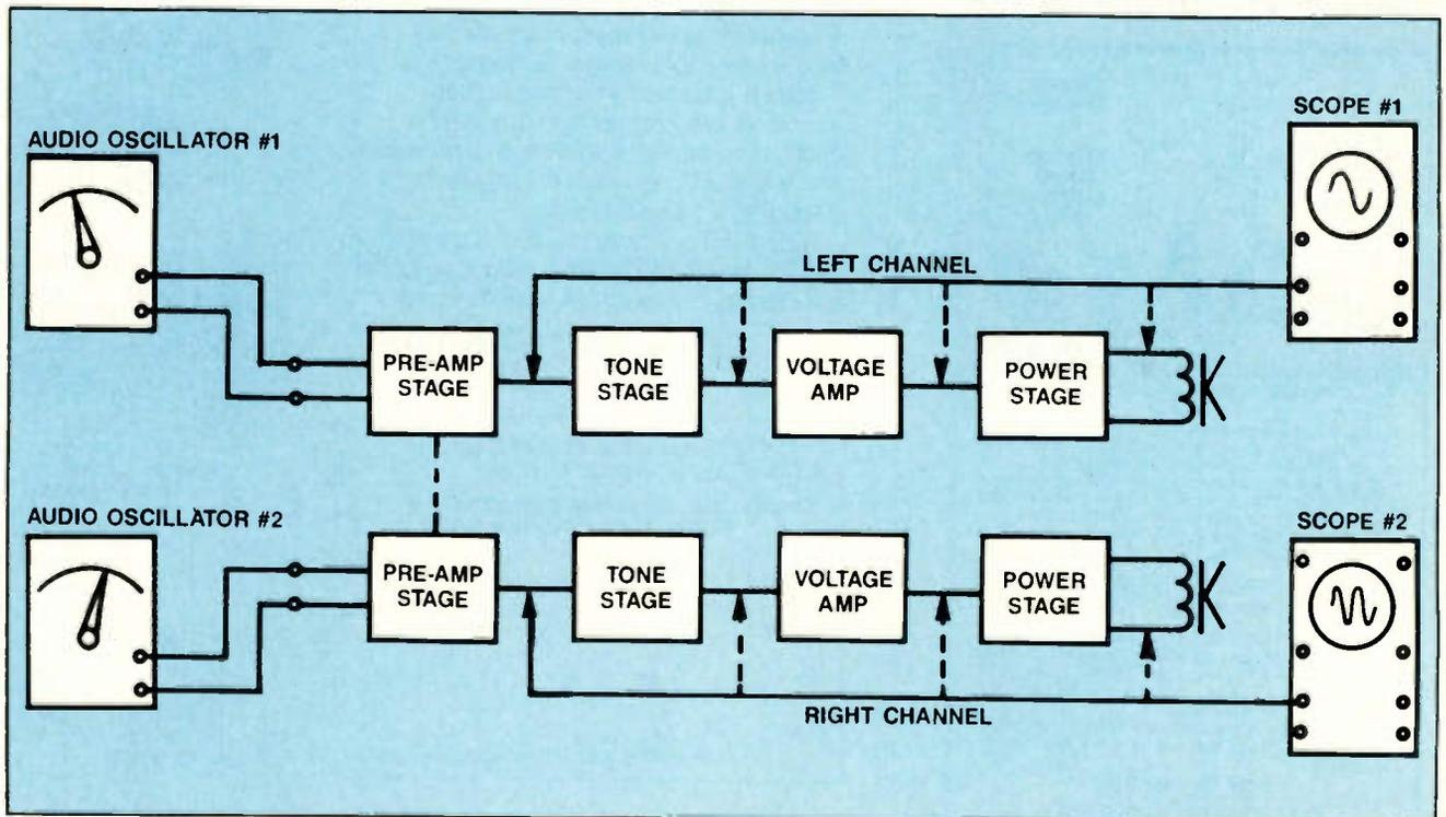
Figure 1. One way to trace stereo separation problems in amplifiers or pre-amps is by means of two audio oscillators, each set to a different frequency, each feeding one channel of the amplifier. Then, using a dual-trace oscilloscope, the technician can check for stereo isolation stage by stage.
