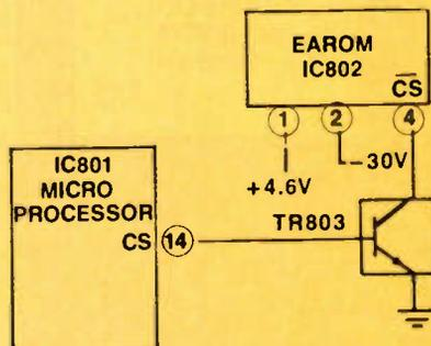
Figure C. This schematic drawing of the timer board that controls the tuner functions shows IC801, the control microprocessor, and IC802, an EAROM.
