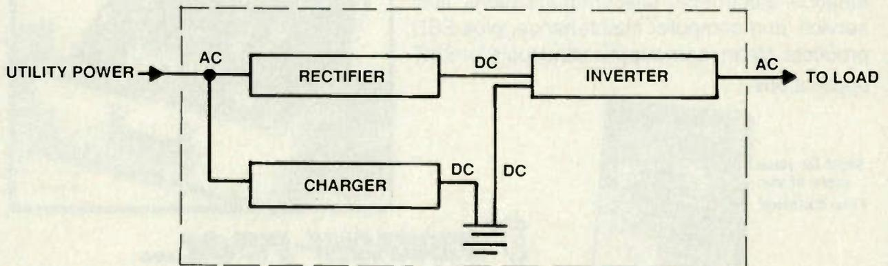
**Figure 3.** The on-line UPS offers no switching, 100% line condition and regulation, sustained brownout protection and sine-wave output. However, it is usually more expensive, larger and heavier. The unit's inverter powers 100% of the load at all times.
