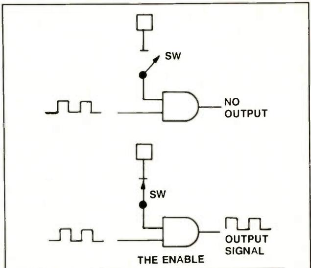
**Figure 6.** In Figure 5, if you put a switch in series with the lead to logic 1, the circuit becomes an ENABLE. When the switch is open, no signal passes through ( $A \text{ AND } 0 = 0$ ). With the switch closed, the output signal is the same as the input signal ( $A \text{ AND } 1 = A$ ).
