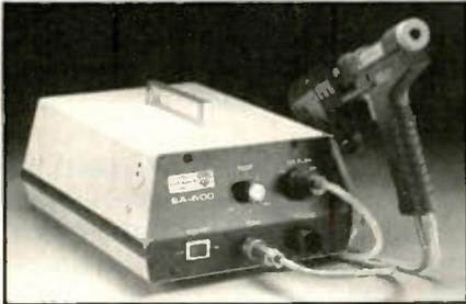
power source. The unit comes with felt and steelwool filters, anti-seize compound, a desoldering gun with tip, a sponge, and cleaning tools for the desol-
