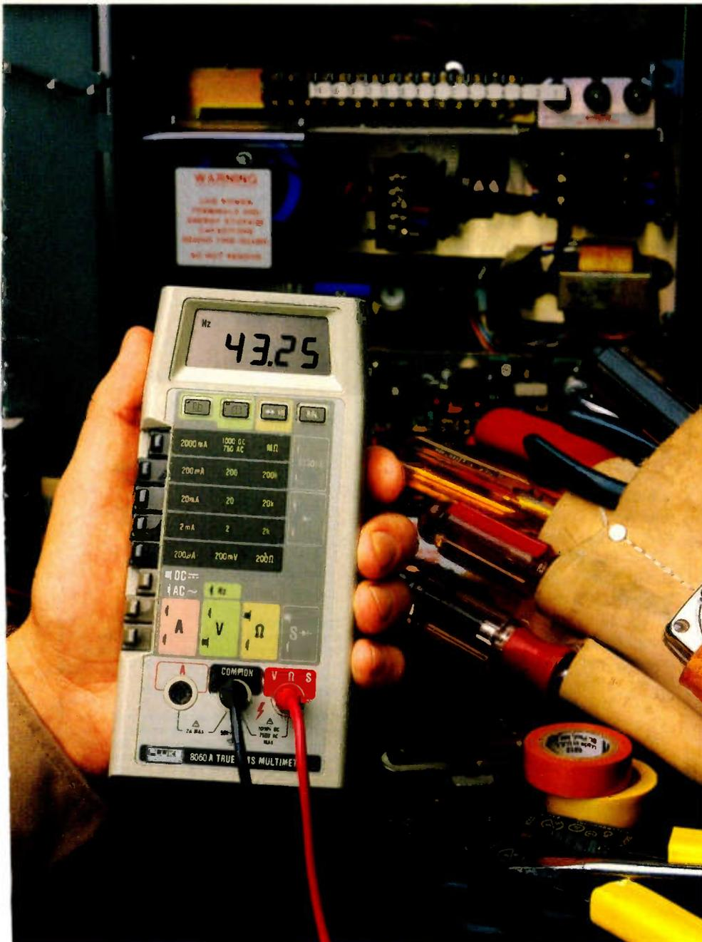
**The Fluke 8060A 4½-digit handheld multimeter.**
