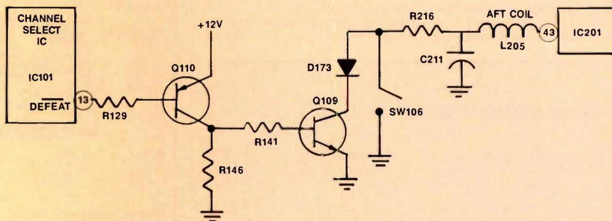
**Figure E.** When the user changes channels, pin 13 of IC101 goes low and turns on Q110 and Q109, which pulls pin 43 of IC201 low and defeats the AFT circuitry within IC201. Once the tuning system has stabilized, pin 13 of IC101 goes high and normal AFT control resumes.
