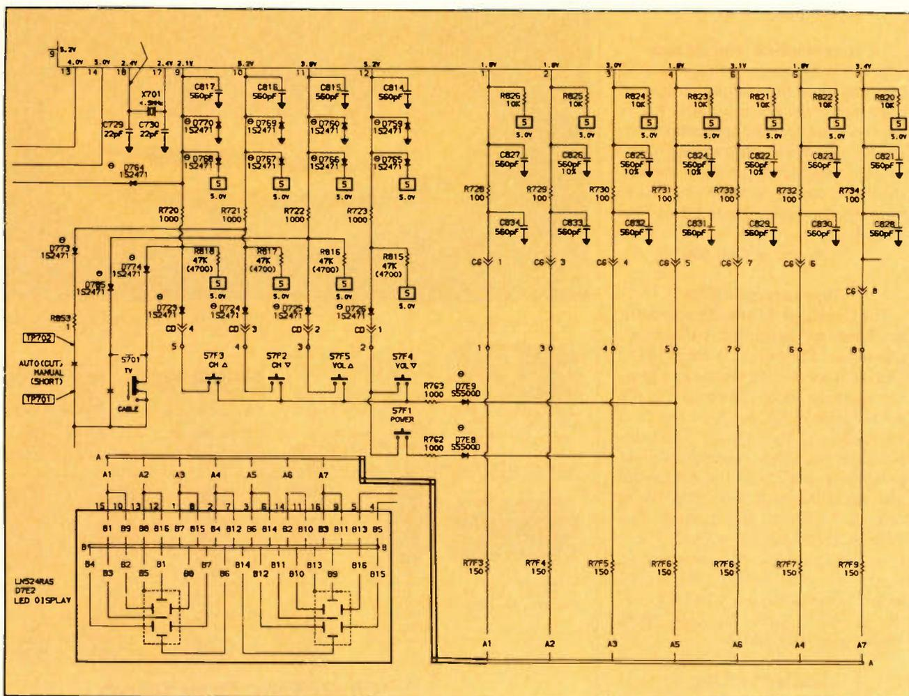
Figure 1. Although paralleling resistors R815, R816, R817 and R818 with other resistors to reduce the resistance treated the uncontrollable volume symptoms in this TV, a new channel LED display treated the underlying problem.
