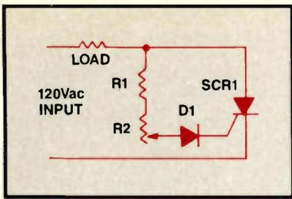
**Figure 4.** A variable-resistance circuit controls the firing angle from approximately  $0^\circ$  to  $90^\circ$ . If R2 is adjusted for maximum resistance, gate current may never be sufficient to turn on the SCR; thus the load is turned off. As R2's resistance is decreased, gate current eventually reaches sufficient amplitude to trigger the SCR.
