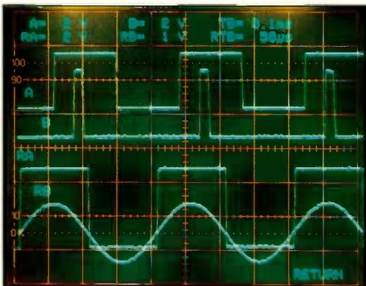
Modern DSOs not only display the waveform of a signal, but the microcomputer circuitry also calculates and displays such parameters as frequency, period, amplitude and more.
