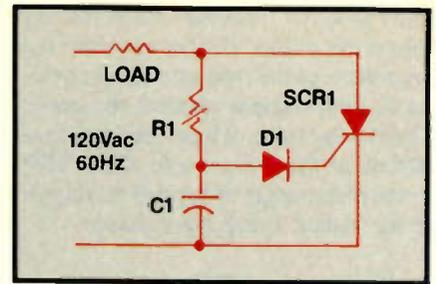
**Figure 9.** Sharper control of SCR triggering is achieved with a Shockley diode. D1 remains in the blocking state until the C1 voltage is high enough to reach  $V_{bo}$ . The capacitor's charging rate is determined by the R1-C1 time constant. When  $V_{bo}$  is reached, the diode switches on, allowing a rush of current that fires the SCR, energizing the load.
