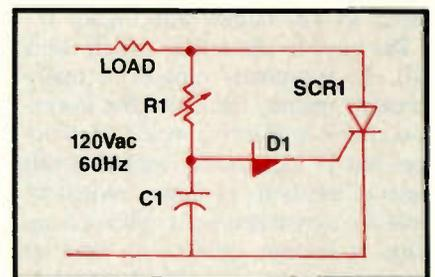
**Figure 6.** With the addition of an R-C phase shift circuit, up to  $90^\circ$  of phase delay is gained. C1 charges through R1, delaying the triggering of the SCR. An increase in the resistance of R1 increases the firing angle up to  $180^\circ$ , at which point the thyristor remains off and no current flows through the load. Reducing the resistance of R1 allows C1 to charge more rapidly, triggering the SCR earlier and increasing the SCR's conduction angle and power in the load.
