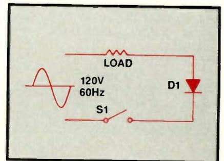
Figure 1. In this static-switch (line-gated), half-wave rectifier, when S1 is open, as in Figure 1a, no gate current can flow. The SCR remains in the off state and no current flows through the load. When S1 is closed and line A is positive (Figure 1b), gate current flows, firing the SCR and effectively closing the cathode-to-anode circuit of the thyristor for virtually the full 180° of the input voltage's positive alternation.
