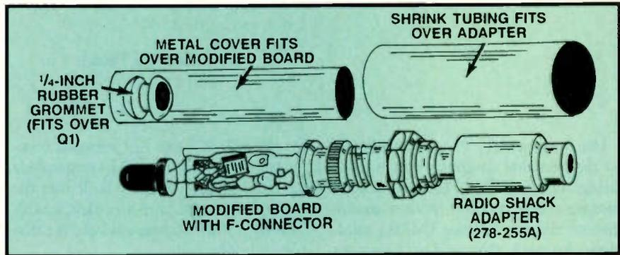
Figure 2. To provide proper shielding, enclose the probe in a suitable metal housing, such as a discarded 300Ω to 75Ω antenna matching transformer. The transformer's circuit board can be stripped of its components, shortened and used as a construction base for the IR probe. With an adapter, the microphone cable can be easily connected to the transformer's F connector.
