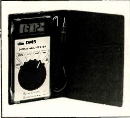
overrange indicators. The meter autoranges over five dc voltage ranges from 200mV to 500V, four ac voltage ranges from 2V to 500V, or six resistance ranges from 200Ω to 20MΩ.
