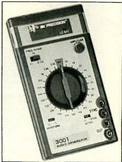
model 3001 is a RC-type oscillator that features selectable sine- or square-wave outputs with a 23-position rotary switch and a x1/x100 slide switch to select from 46 frequencies. A separate sync output provides a fixed-level signal at the same frequency and phase as the main output.
