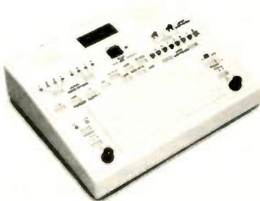
**Analog model:** 2 DC/2 AC power supplies, 200 Hz to 200 kHz function generator. **Digital model:** 3 DC power supplies, 8 LED logic indicators, built-in logic probe and pulser. Both have 1380 solderless tie points. No support circuits required. At 900 Philips ECG distributor locations or call 1-800-526-9354.
