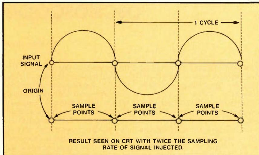
**Figure 2.** To assure that the waveform representation is correct, a digital storage oscilloscope must be capable of sampling at rates greater than twice the highest frequency that you will encounter. Sampling at less than twice the frequency of the signal can result in a waveform that does not accurately represent the waveform. In this worse case, a sine wave can look like a straight line. This problem is known as *aliasing*.
