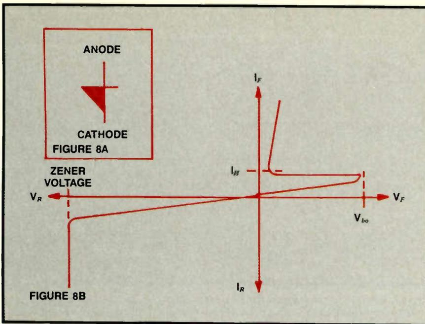
**Figure 8.** The Shockley diode is a unidirectional PNP 2-terminal thyristor. When the applied voltage makes the anode positive in relation to the cathode, the diode remains essentially an open switch — even though forward-biased — until  $V_{bo}$  is reached. Then the anode-to-cathode voltage suddenly drops as current begins flowing through the device; it thus enters the forward conduction region.
