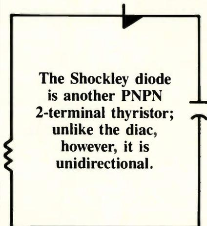
cally somewhere between 20V and 35V in different diacs. When breakover occurs, the voltage across the device drops sharply as the current through it increases; hence its negative resistance.
