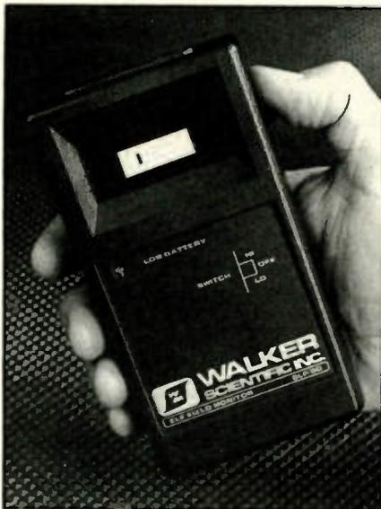
generated from any ac 60Hz device. A 10-segment LED display illuminates to indicate the level of radiation present. The monitor features two measurement ranges: low range, from 1 to 512 milligauss; and high range, up to 51.2 gauss.
