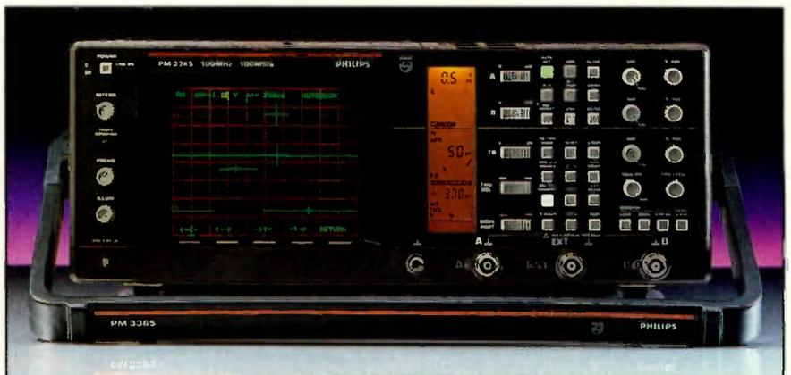
DSOs and analog oscilloscopes both display electronic signals, but the DSO also stores signals, performs calculations to determine and display waveform parameters, and transmits data to a computer to be saved on disk.
