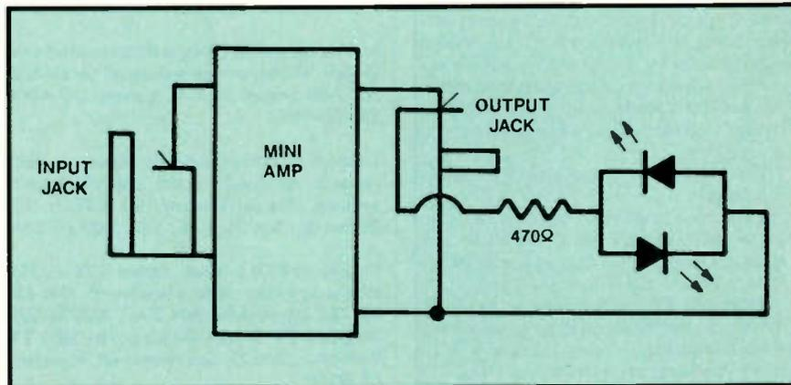
Figure 3. When using the mini-amp to test LEDs, you might find it hard to hear the sound made by a dc-driven LED as the probe is moved past the LED. This modification replaces the speaker with LEDs to give a visual, not an audible, indication.
