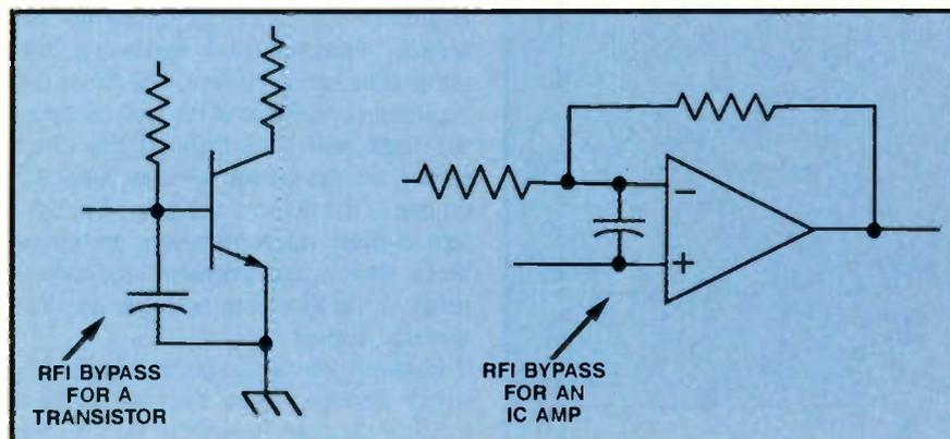
Figure 1. Filter capacitors can be used as an RFI bypass for transistors and IC amps. A 5pF to 100pF capacitor from the inverting to non-inverting inputs can be used with ICs. For transistors, the capacitor should be connected between the base and emitter as close to the transistor as possible.
