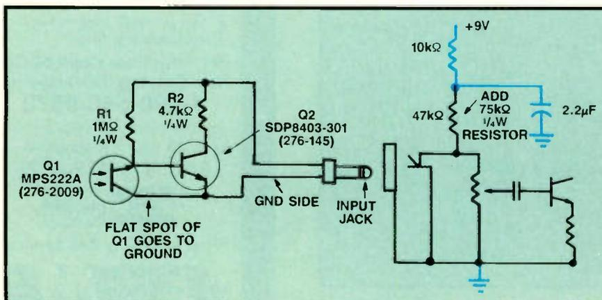
Figure 1. To build a remote control transmitter, construct a simple pickup probe and add one additional internal resistor to the modified mini-amp. To eliminate motorboating, modify the circuit as shown by the colored lines.
