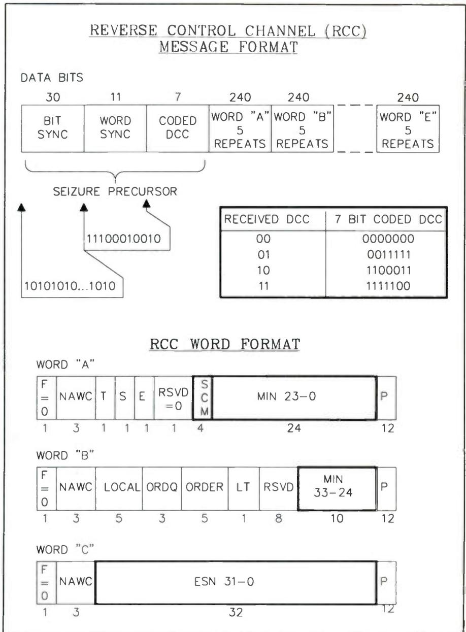
Figure 2. Reverse control channel data format.
