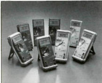
They are extremely useful for testing large electrolytics thus eliminating the need for a dedicated capacitance tester. The models 79 and 29 have Smoothing, a Fluke exclusive feature which displays the running average of eight readings, providing stable readings even with unstable signals. They also have a proprietary Lo-ohms function which provides 0.01 ohm resolution with high noise rejection to sense very small resistance changes.
