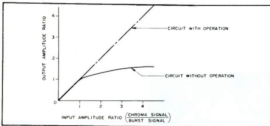
Figure 4. Characteristics of Color Saturation Control.
