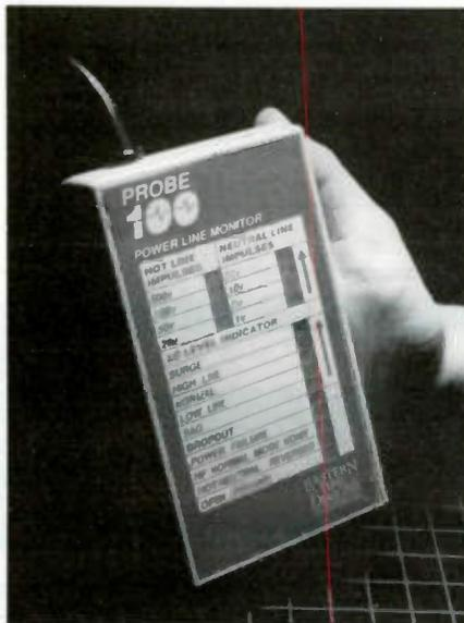
plugged in overnight and it will record and store the disturbance events through LED lights which stay latched or lit until reset by the operator. First, check to see if you have a wiring problem of the Hot/ Neutral wires reversed or open ground. Then leave the unit plugged in for 24 to 72 hours, check the LEDs's periodically and at the end of the test. Refer to the manual for an explanation of the disturbances that occur.
