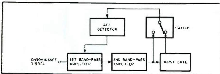
Figure 3. Block diagram of Color Saturation Control.
