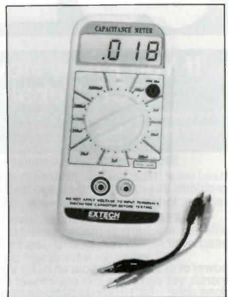
has a resolution of 0.1pF to 10uF. Excitation voltage is 2.8 volts peak maximum. The meter measures 7.3 x 3.4 x 1.5" and weighs only 10 oz. This fast response meter comes complete with
