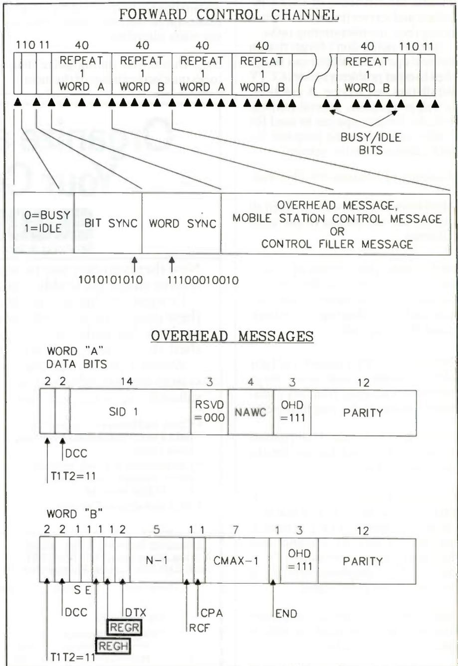
Figure 1. Control (paging) channel digital data stream.
