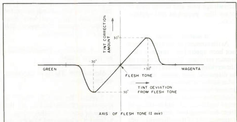
Figure 2. Tint control characteristic.
