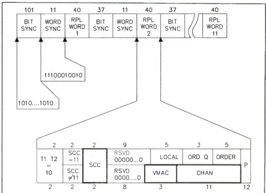
Figure 6. Mobile station control message data format.
