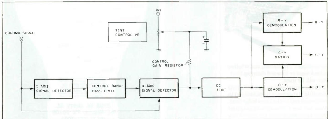
Figure 1. Block diagram of Automatic flesh tone Control Circuit.
