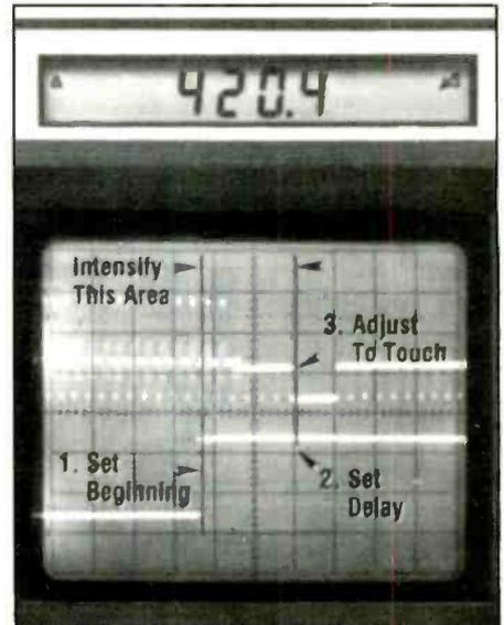
Figure 7. Use the delta time function, if your oscilloscope has this feature, to preset the time needed between signal, and then adjust the circuits until the signals touch the intensified area of the waveform.
