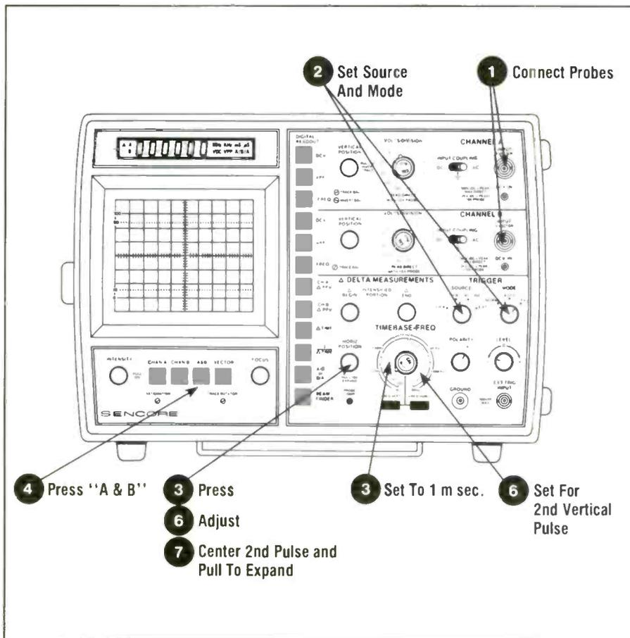
es on the channel A trace - one at the left edge and the second one near the right edge of the screen. (Channel B should show a square wave transition near the second sync pulse.)
