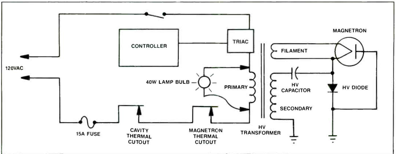
**Figure 3.** A 40W pigtail socket light bulb, or ac meter connected to the primary winding of the power transformer indicates if primary circuits are normal.
