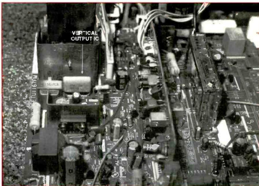
Figure 2. The defective vertical deflection IC (X0238CE) in a Sharp 19SB60R model was replaced with a TCE SK7653 universal replacement.
