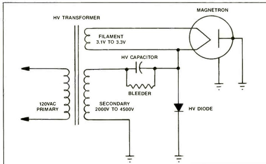
Figure 2. The basic high-voltage doubler circuit with transformer, high-voltage capacitor and diode.
