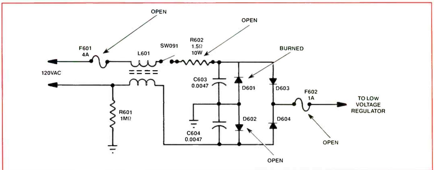
Figure 7. When this Curtis Mathes CM81 console was subjected to a higher than normal line voltage, several components in the low voltage circuit were damaged. In addition, several sections of the PC wiring were burned.
