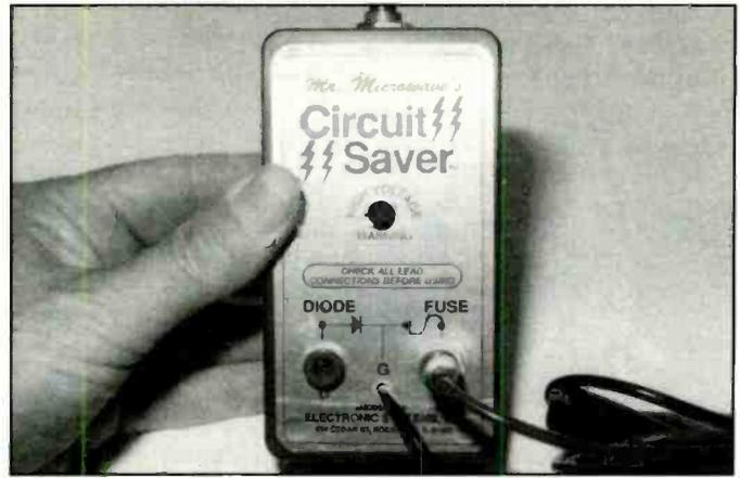
**Figure 9.** When the microwave oven keeps blowing the fuse, clip the Circuit Saver across the fuse holder and just reset the circuit breaker, instead of replacing those expensive chemical fuses each time.
