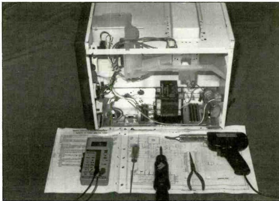
Figure 1. Do not touch anything: hands, tools, or test leads to the oven while operating.
