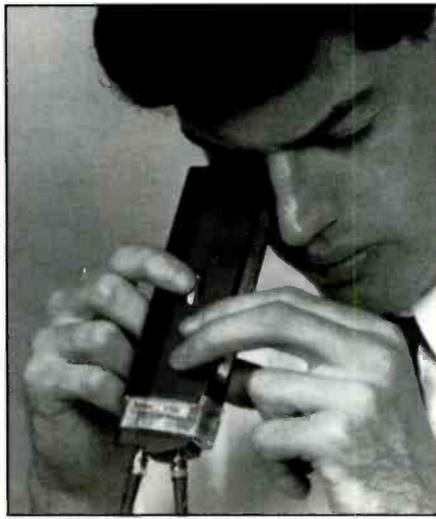
viewing, emphasizes polish irregularities, providing the best test to how well the connector has been polished. One can even confirm "PC" convex polishing in this mode. The device even offers zoom capability, with a 60X to 100X range. It is compatible with many common fiber optic connectors.
