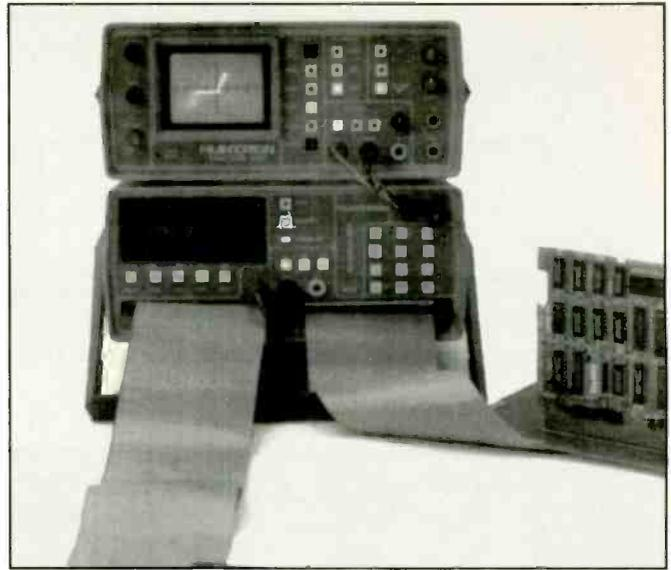
This device has dual inputs so it routes signals from a known good part and the suspected bad part to a signature analyzer. All you do is attach a clip to the IC being tested and use the switcher's 40 push buttons to display the signature at each of up to 40 pins. You can even customize the cable with special edge connectors or interface devices.
