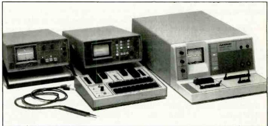
**Figure 58.** The instrument on the far right provides the capability to handle 64-, 40-, and 20-pin IDC connector sockets. It has a 40-pin ZIF (zero insertion force) socket built in, and an IEEE-488 interface.
