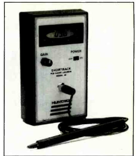
Figure 54. The Shorttrack allows the user to probe a PC board to determine where current falls off, and therefore where there is a short circuit.
