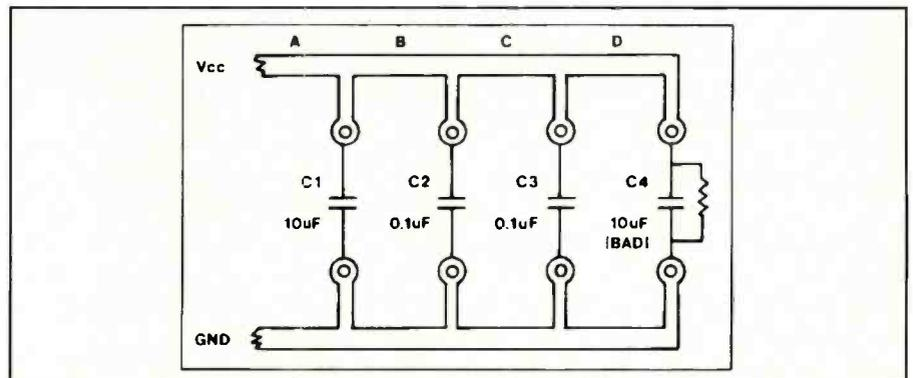
Figure 55. The shorted capacitor of these four paralleled capacitors will draw the most current, more than the other three non-short-circuited capacitors, thus allowing the user of the short circuit tracker to find the bad capacitor.
