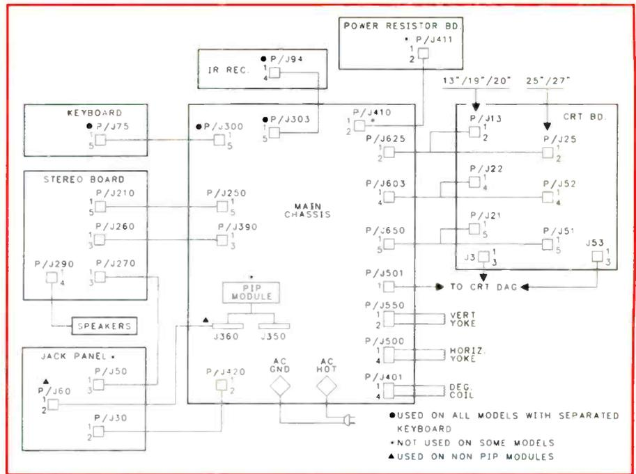
**Figure 2.** This simplified wiring diagram shows how the various portions of the S1/S4 sets are connected together.
