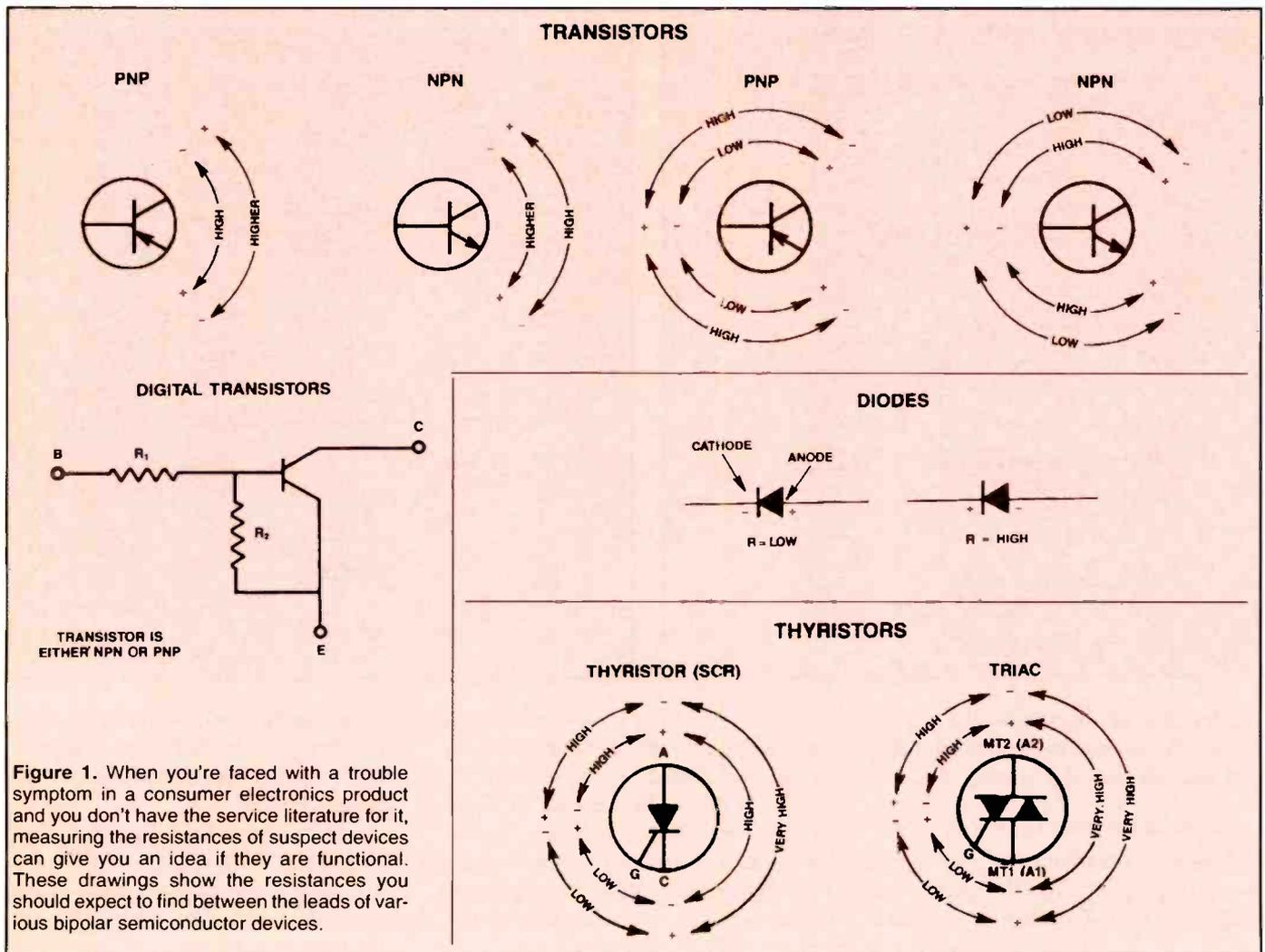
Figure 1. When you're faced with a trouble symptom in a consumer electronics product and you don't have the service literature for it, measuring the resistances of suspect devices can give you an idea if they are functional. These drawings show the resistances you should expect to find between the leads of various bipolar semiconductor devices.
