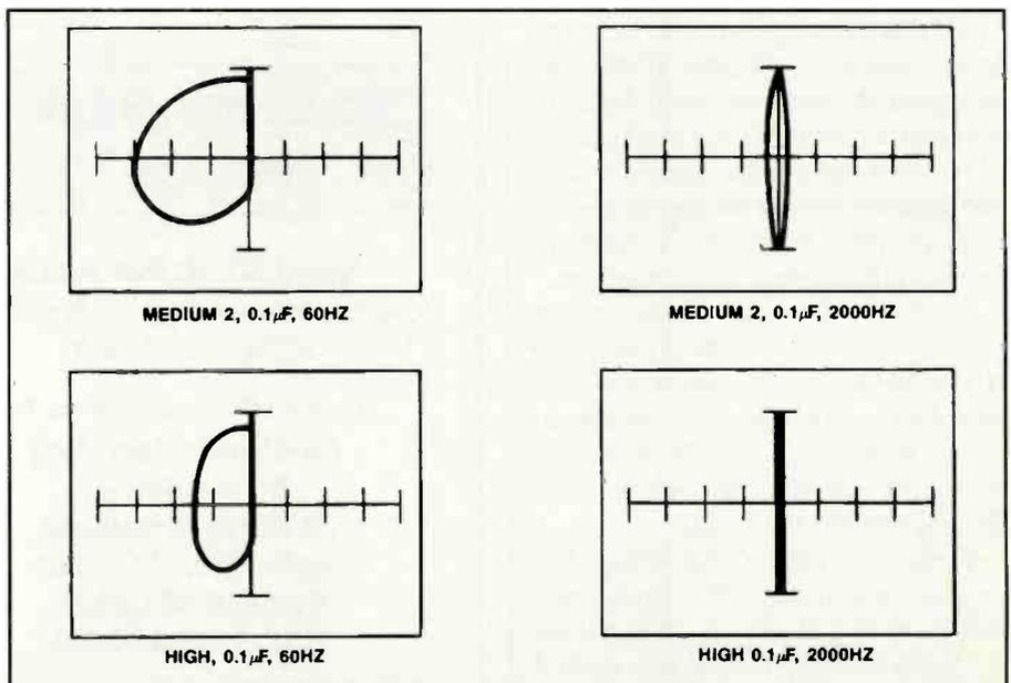
Figure 49. A 50k $\Omega$  resistor in parallel with a 0.1 $\mu$ F capacitor yields this signature.
