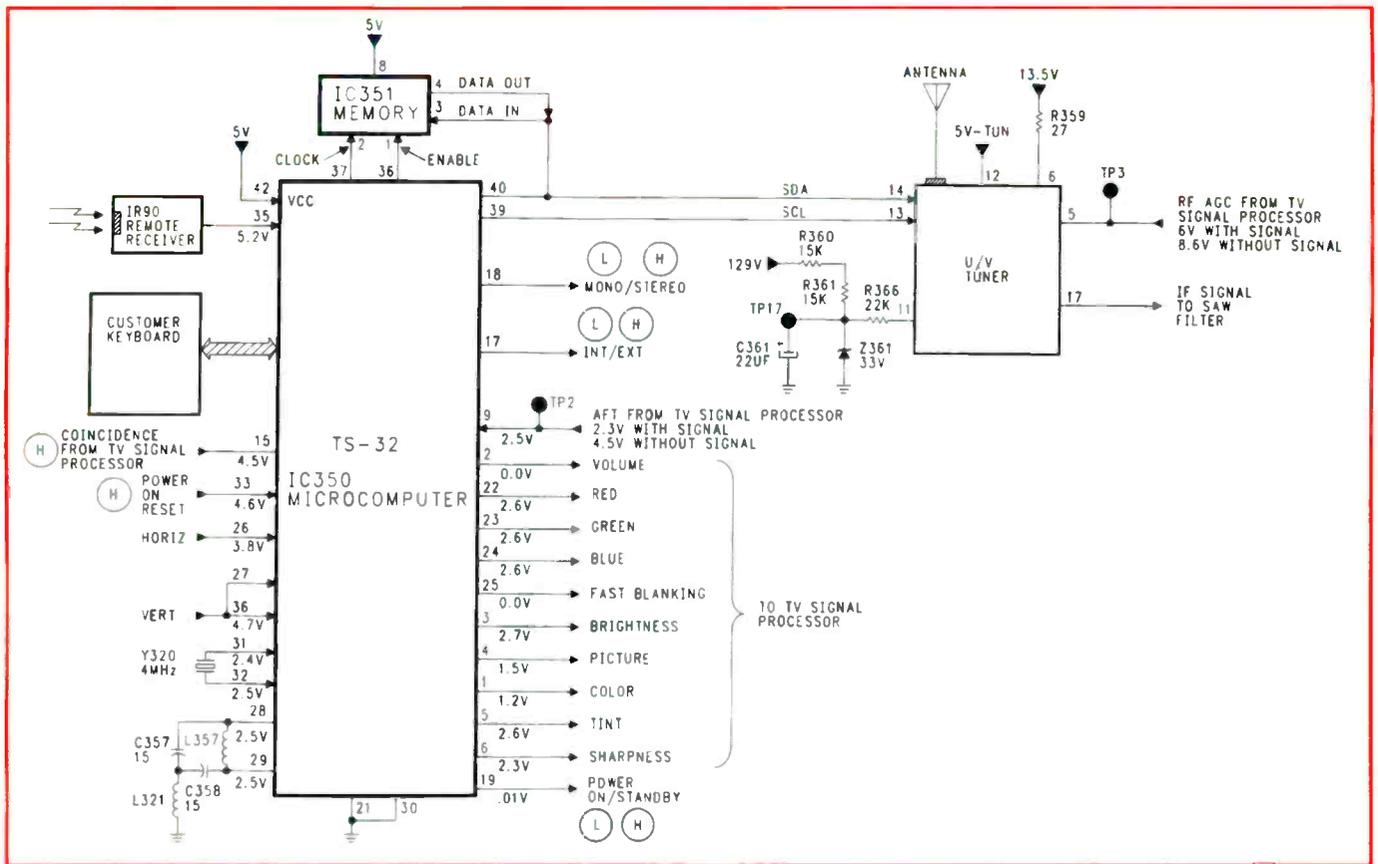
**Figure 5.** The tuning system in this TV set, as in many modern products, contains a microcomputer, with its attendant memory, to provide a wealth of functions electronically.
