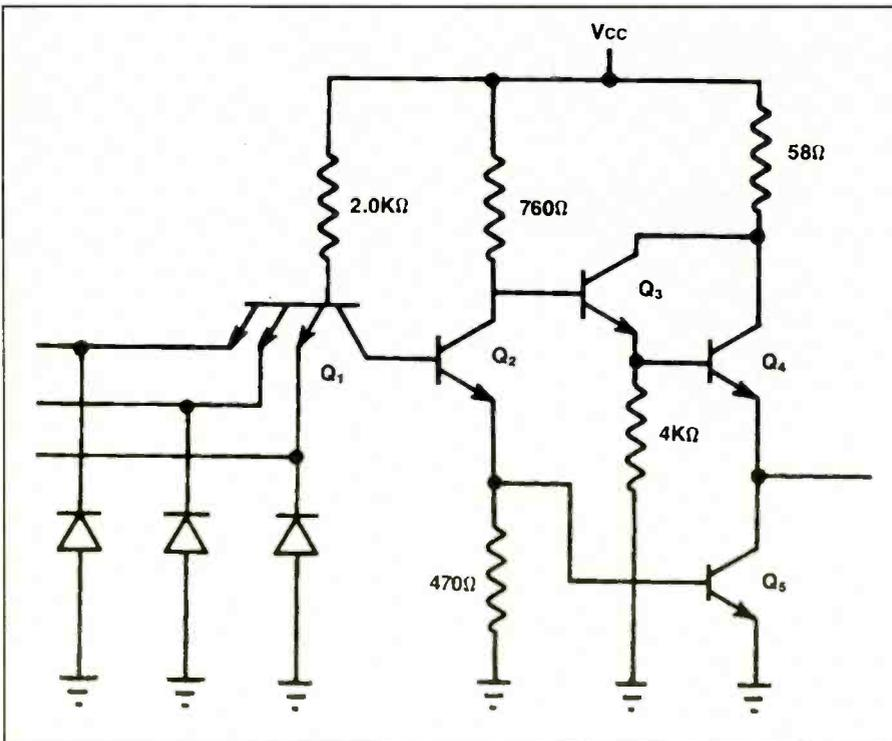
Figure 51. A typical TTL (transistor-transistor logic) gate. These gates are similar in that they have an input gate, phase shifter, (Q2) with emitter and collector load resistors, a pull-up mechanism (Q3/Q4) and a pull-down transistor (Q5).
