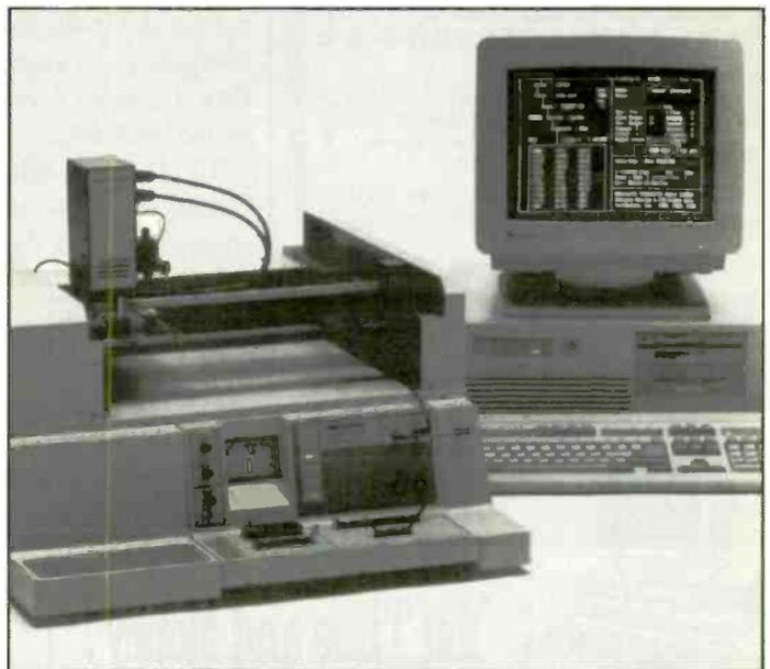
Figure 62. The probe allows automation of board testing.
