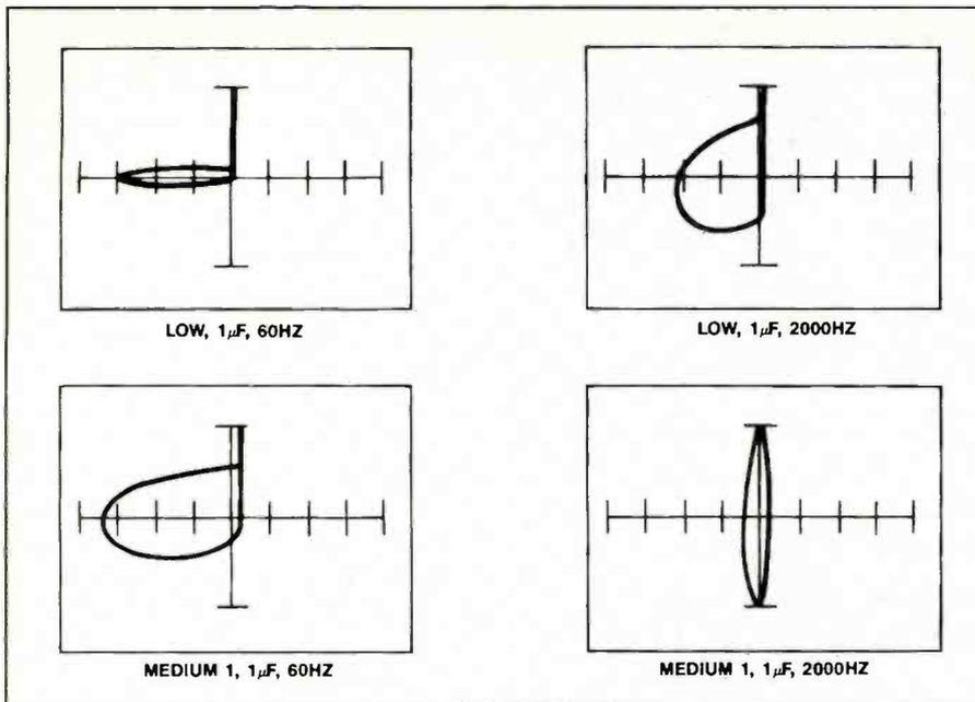
Figure 50. The signature of a 1kΩ resistor in parallel with a 1μF capacitor.
