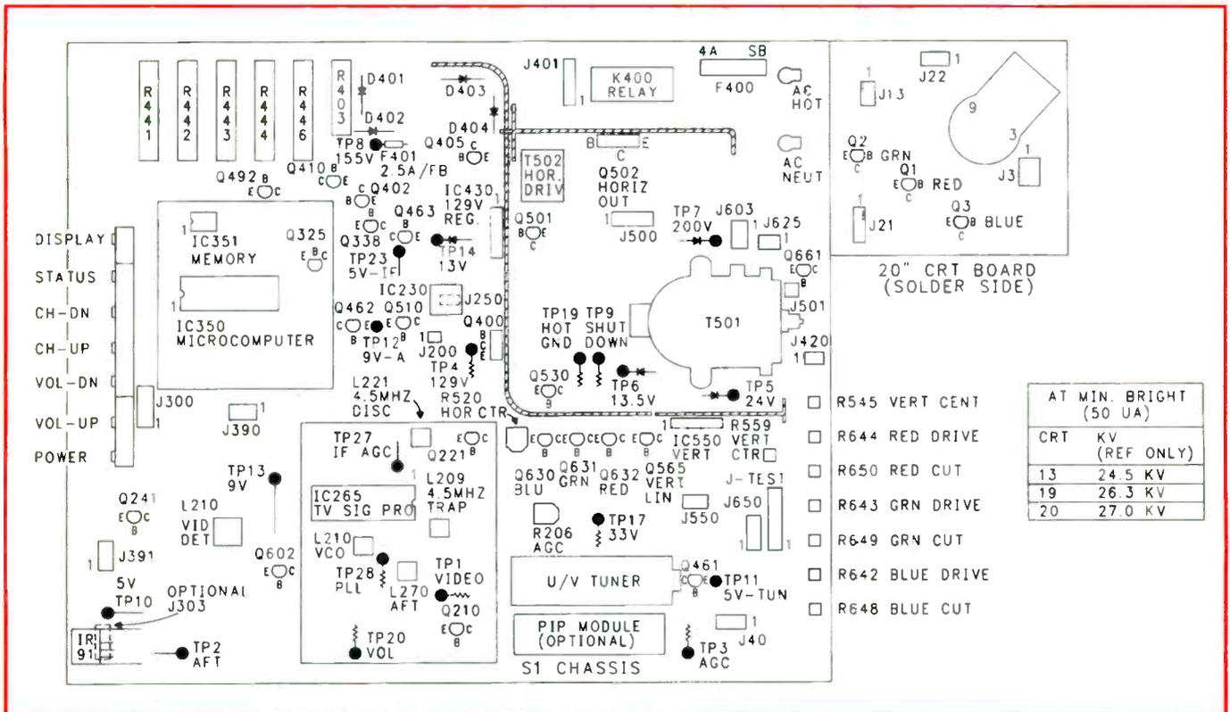
**Figure 3.** This layout shows where the various components are located on the S1/S4 chassis.
