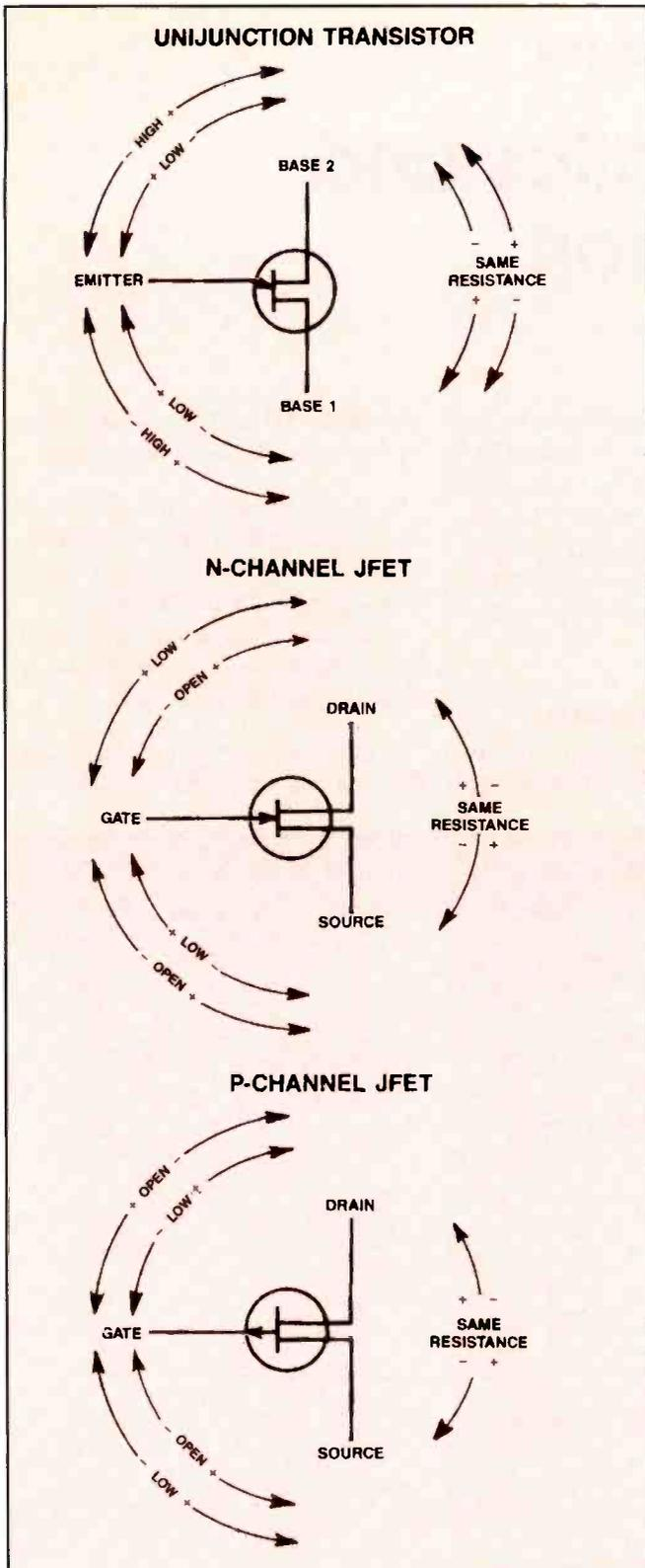
**Figure 2.** You can get an idea if a unijunction transistor or JFET is operational by measuring resistances between elements. These drawings show the resistances that you will measure if the unit is functioning properly.
