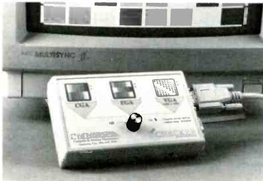
Checker I (photo)- Color patterns for CGA, EGA, & VGA monitors. Battery or AC operation.....\$229.95
