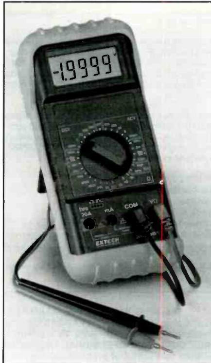
200mV to 750V, dc current and ac current in five ranges from 200µA to 20A, and resistance in seven ranges from 20Ω to 20MΩ. Basic dc accuracy of 0.05%. Also includes audible continuity, diode, and transistor test. The large LCD readout reads up to 19,999 counts for resolution to 10µV, 0.1µA and 0.01Ω. Also indicates function, polarity, low battery and overload. Fuse protected. Comes complete with test leads, rubber protective holster, and 9V battery.
