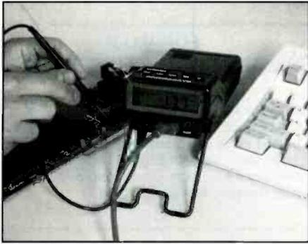
ature measurement capabilities include twelve °C/°F ranges from -200C to +1372C (-328F to +2500F) with 0.1C resolution to +1000C.
