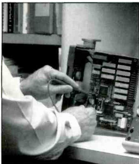
The tasks performed by a technician in servicing a consumer electronics product usually follow a logical procedure. The technician begins by performing a thorough visual check to see if there are any obvious signs of the cause of the problem: things like burned resistors, charred circuit boards, loose connectors, cracked circuit board traces, broken switches, etc.
