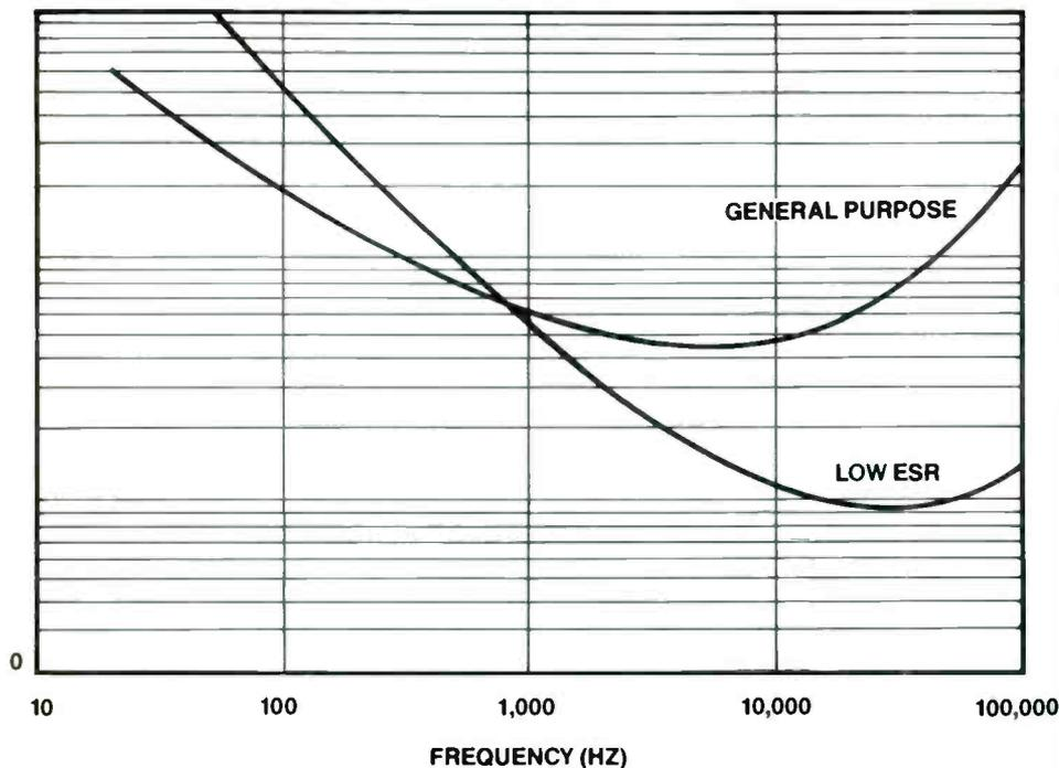
**Figure 2.** ESR is frequency dependent. If you viewed the frequency versus ESR graph chart of a low-ESR electrolytic you would find the ESR is biased so that the ESR is lower at high frequencies than it is at low frequencies.
