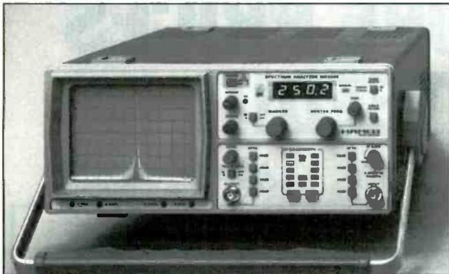
Both models are equipped with a 4-digit LED readout and can selectively display either Center or Marker Frequency. If Marker Frequency is selected, a dot is added on the screen to facilitate frequency determination.
