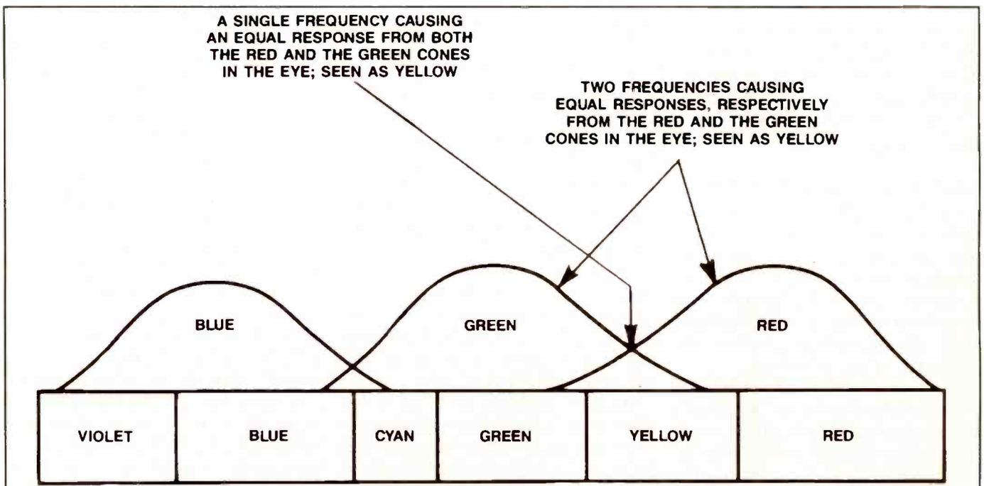
**Figure 1.** This is a drawing showing hypothetical response curves of the red, green and blue cones of the eye, and how two frequencies causing equal responses, respectively, from the red and the green cones might be seen as the same color as one frequency causing an equal response from both groups of cones.
