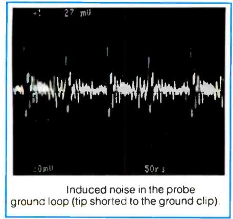
Figure 3. Induced noise in the ground loop with the probe tip shorted to the ground clip.
