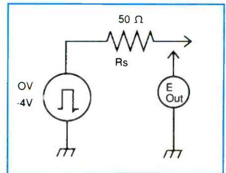
Figure 4. The principle of operation of a bias offset probe.
