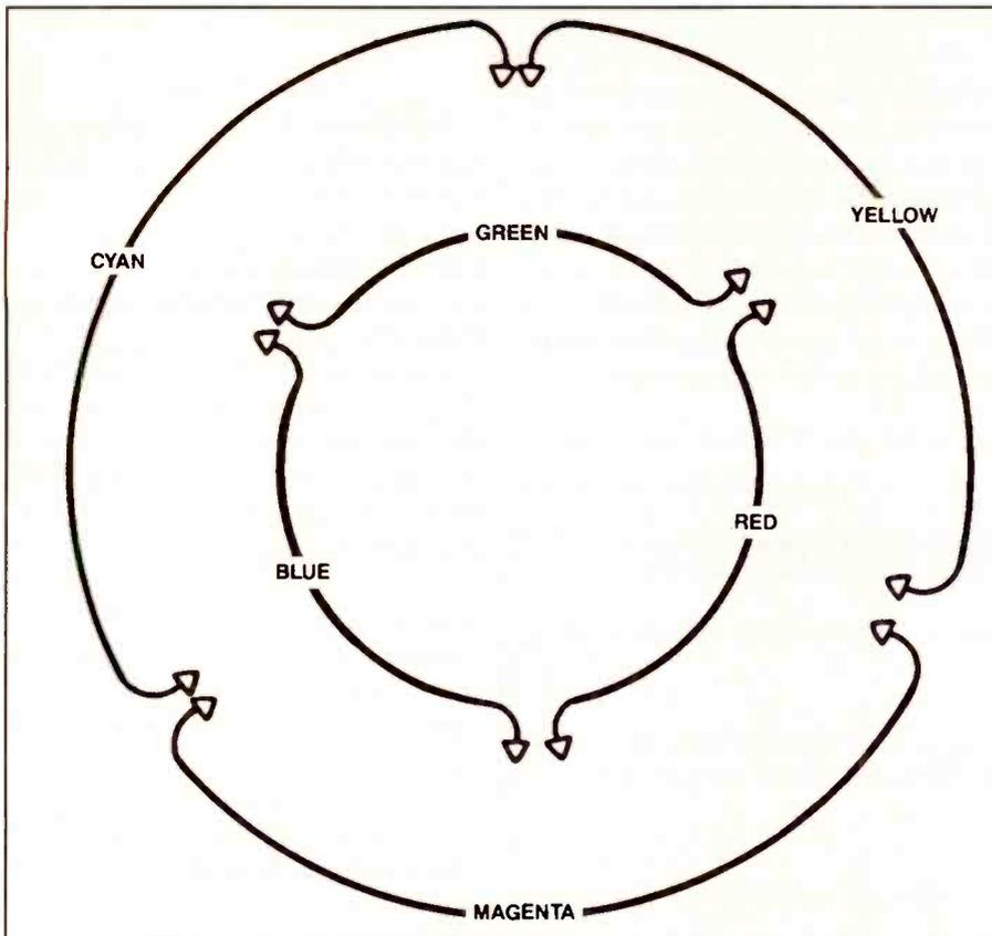
Figure 3. Any two primary additive colors adjacent to each other on the inside circle add to produce the color between them on the outside circle. Any two primary subtractive colors adjacent to each other on the outside circle subtract to produce the colors between them on the inside circle.
