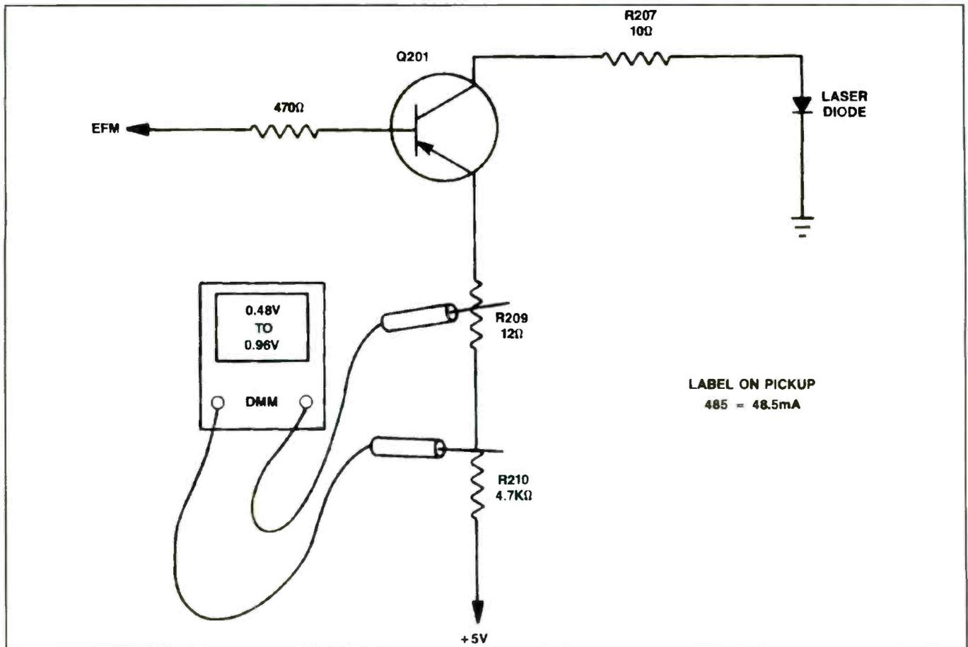
Figure 3. Voltage measurements across the emitter resistor can be converted to current, indicating if the laser diode is functioning.
