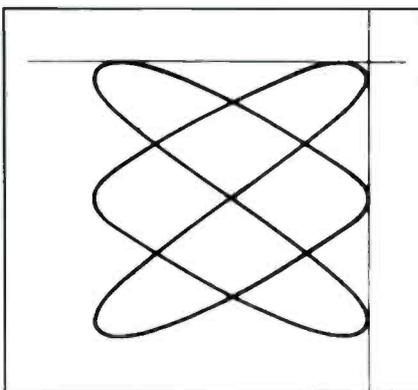
**Figure 3.** To solve TYEK question number 6, draw horizontal and vertical lines against the curve as shown here. The number of times the curve touches the vertical line divided by the number of times it touches the horizontal line is equal to the horizontal frequency divided by the vertical frequency. In this case  $3:2 = 450:f_V$ . Therefore,  $f_V = (450 \times 2)/3 = 300\text{Hz}$ .
