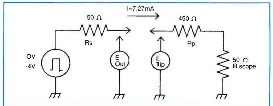
Figure 5. A bias offset probe connected to a 50Ω source.
