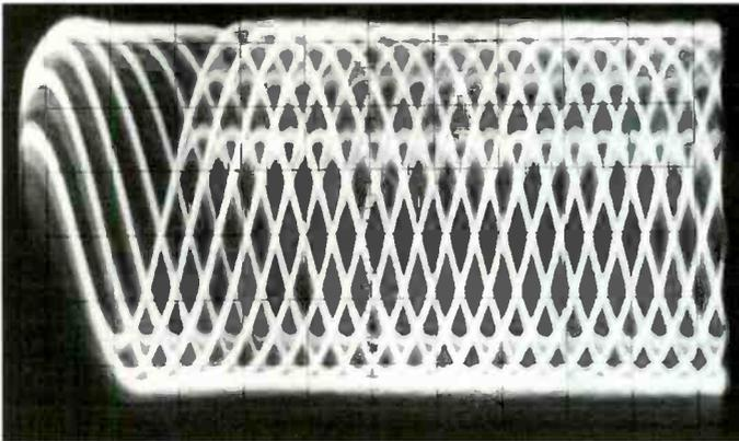
**Figure 3.** A good EFM waveform voltage should have a clear-cut diamond shape with very little jitter.
