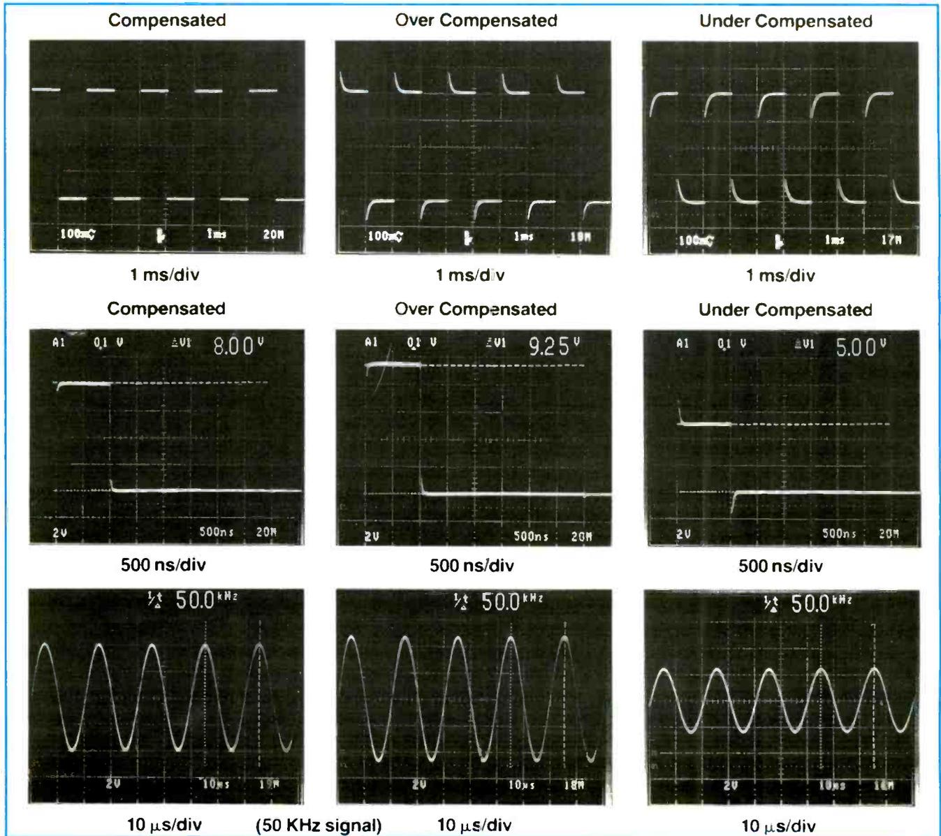
Figure 1. Compensating the probe.
