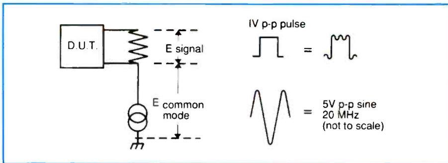
Figure 11. A simplified block diagram of a device under test.
