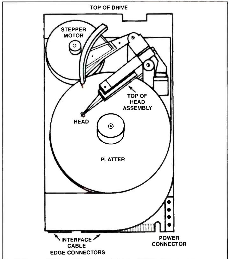
**Figure 1.** This is what a typical hard disk drive looks like with its cover removed. The drive assembly includes heads, cylinders, and platters. Each platter in the hard disk drive has two sides. In operation, read/write heads move across the platters while data is stored in tracks and sectors on the platters.
