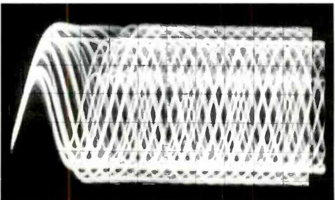
**Figure 6.** The jittery or bouncing EFM waveform may indicate improper focus error adjustment.
