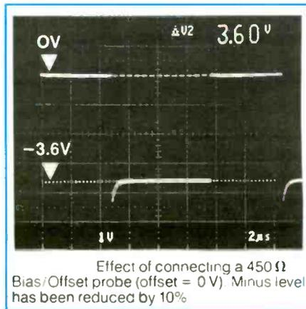
Figure 7. The same pulse as that in Figure 6, acquired with a 450Ω probe added.
