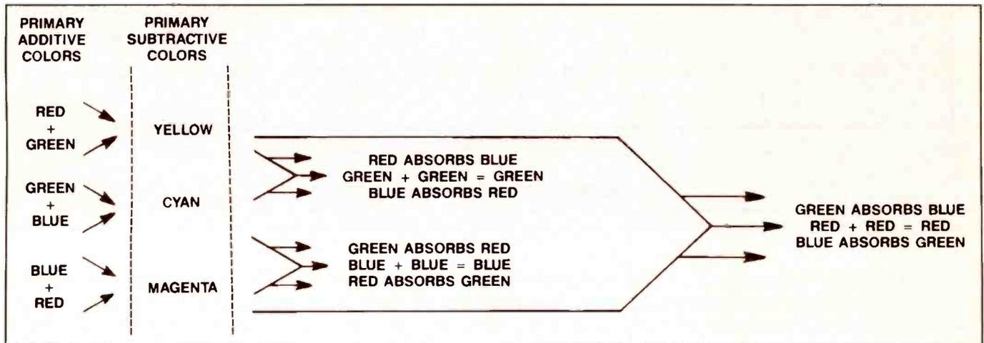
**Figure 4.** Starting at the left of the figure, light sources are added to produce secondary additive colors. The colors obtained, shown between dotted lines, are the primary subtractive colors. These primary subtractive colors combine with each other to reflect the colors after the equal signs.
