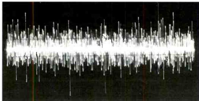
**Figure 12.** The sled motor movement may be seen as varying lines of a scope waveform taken at the slide motor terminals.
