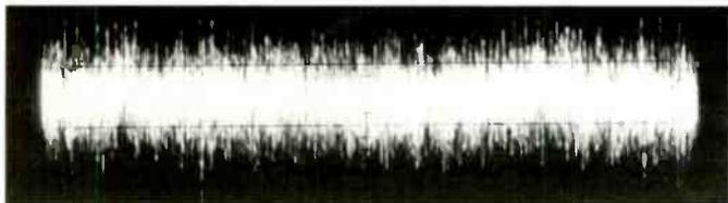
**Figure 9.** The tracking error (TE) signal can be signal traced with the scope from tracking IC to tracking driver and tracking coil.
