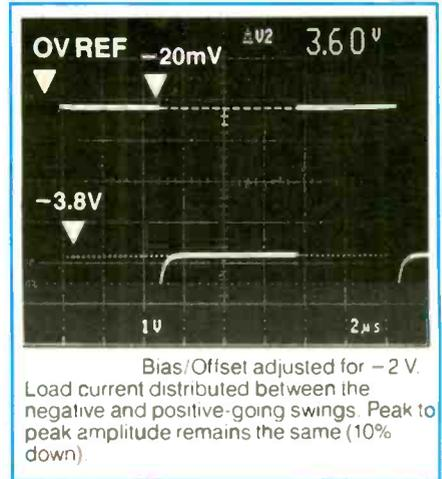
Figure 9. Adjusting bias to equally distribute current.
