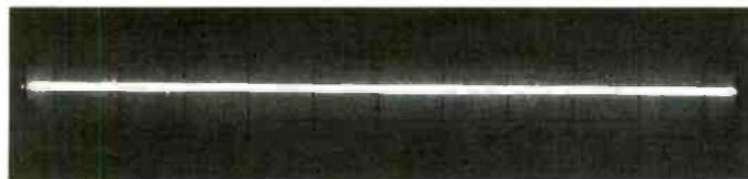
**Figure 11.** No motor movement may show a white line waveform without any motor lines.
