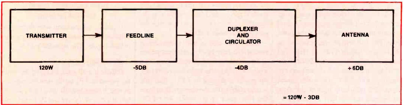
**Figure 2.** A system consists of a transmitter that has a power output of 120W, a feedline with 5dB loss, a duplexer and circulator with 4dB loss and an antenna with 6dB gain. What will be the effective radiated power of this system.
