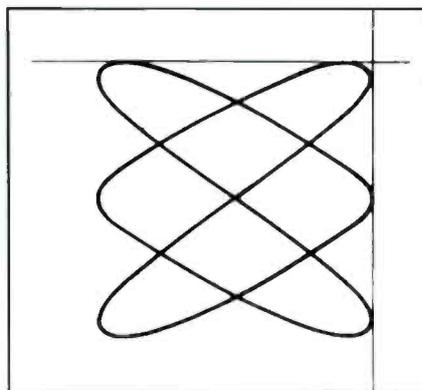
**Figure 3.** To solve TYEK question number 6, draw horizontal and vertical lines against the curve as shown here. The number of times the curve touches the vertical line divided by the number of times it touches the horizontal line is equal to the horizontal frequency divided by the vertical frequency. In this case  $3:2 = 450:f_V$ . Therefore,  $f_V = (450 \times 2)/3 = 300\text{Hz}$ .
