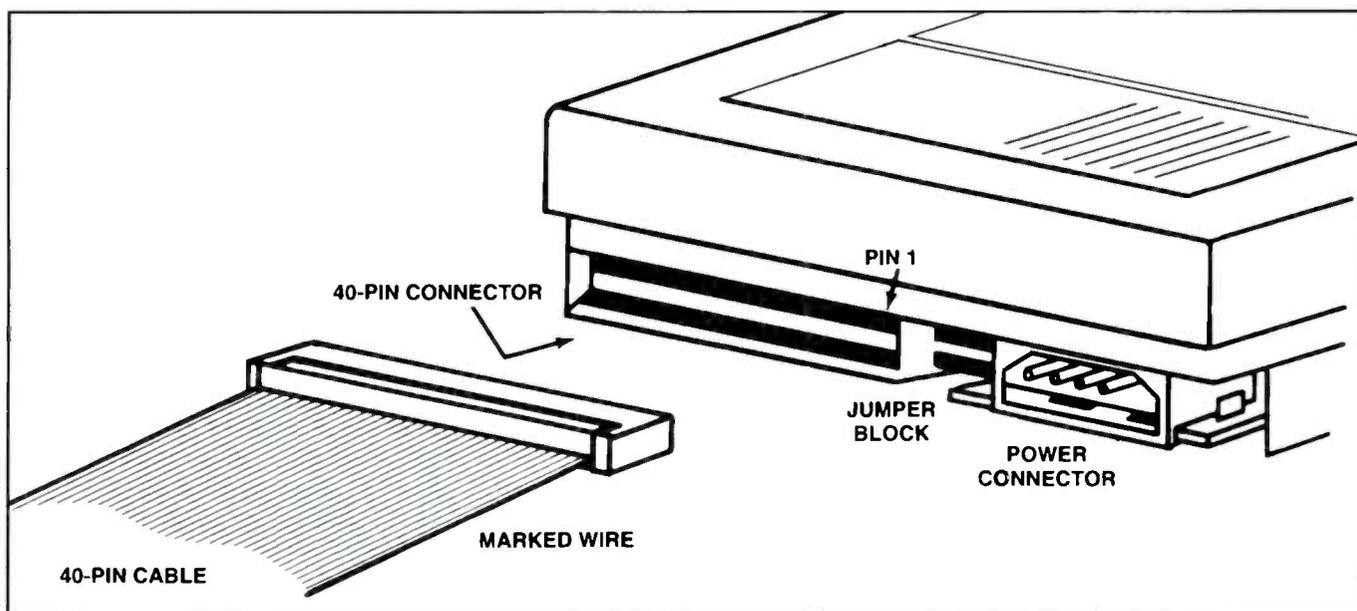
**Figure 3.** The IBM-compatible IDE interface cable connection.
