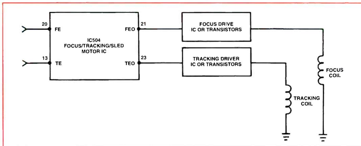
**Figure 8.** The focus error output (FEO) and tracking error output (TEO) signals are fed from the focus/tracking/sled IC.
