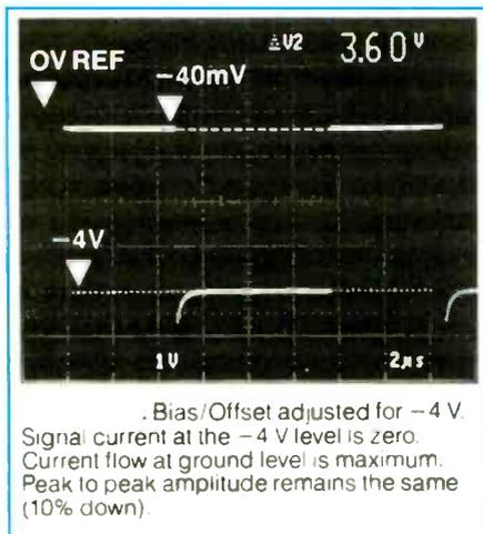
Figure 8. Adjusting bias to offset loading effects.
