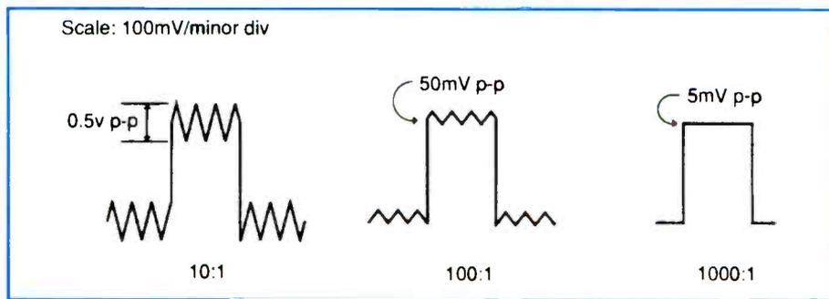
Figure 12. "Cleaning up" a signal by increasing the CMRR.
