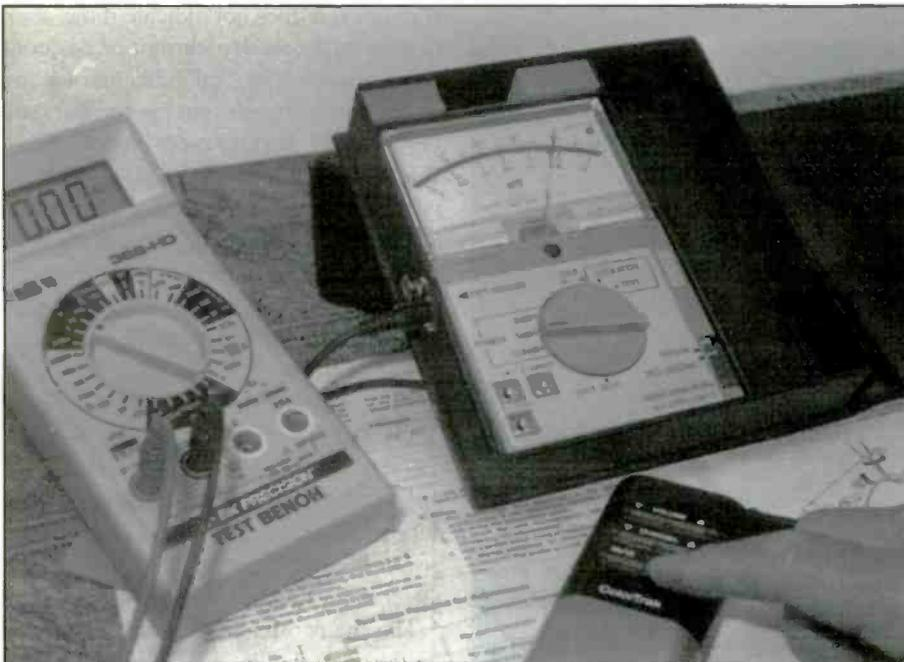
**Figure 8.** Check the suspected remote control with the infrared laser meter using the higher power ranges.
