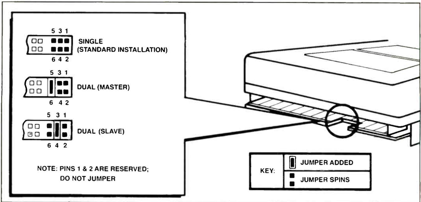
**Figure 4.** IDE hard disk drives do not have terminating resistor packs. However, a set of jumpers on the underside of the drive can be used to configure the drive as a master or slave. On a Western Digital Caviar drive, those jumpers are placed as shown here.
