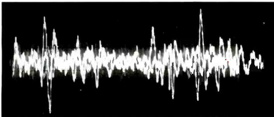
**Figure 7.** Connecting the oscilloscope across the focus coil winding indicates if signal is present at the coil assembly.
