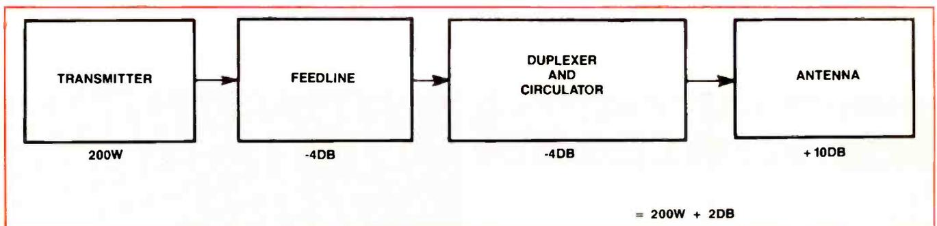
**Figure 1.** A system consists of a transmitter that has a power output of 200W, a feedline with 4dB loss, a duplexer and circulator with 4dB loss, and an antenna with 10dB gain. What will be the effective radiated power of this system?
