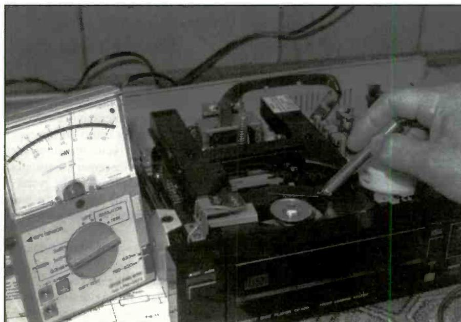
**Figure 6.** In most CD players, the infrared protecting interlock system must be defeated before the laser diode comes on.
