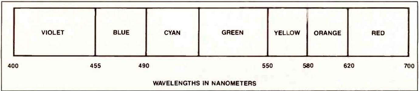
Figure 2. A rough sketch of the placement of colors in the spectrum of visible light, with wavelengths given in nanometers, or billionths of a meter.
