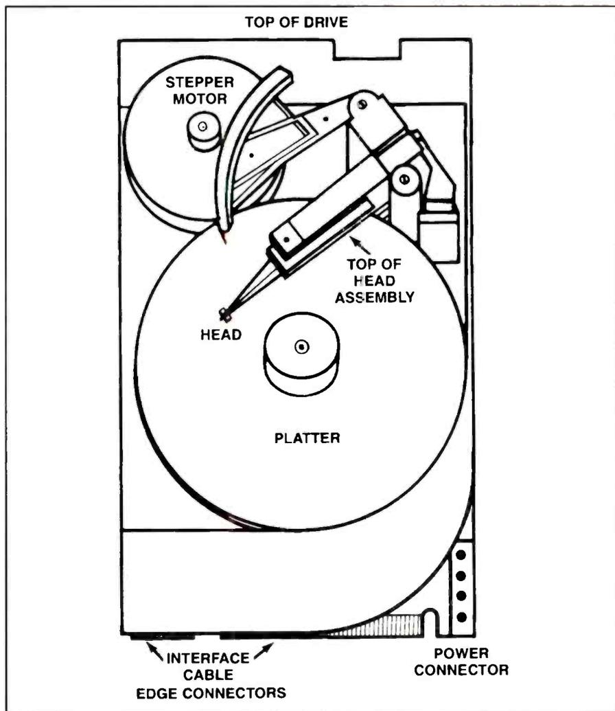
**Figure 1.** This is what a typical hard disk drive looks like with its cover removed. The drive assembly includes heads, cylinders, and platters. Each platter in the hard disk drive has two sides. In operation, read/write heads move across the platters while data is stored in tracks and sectors on the platters.
