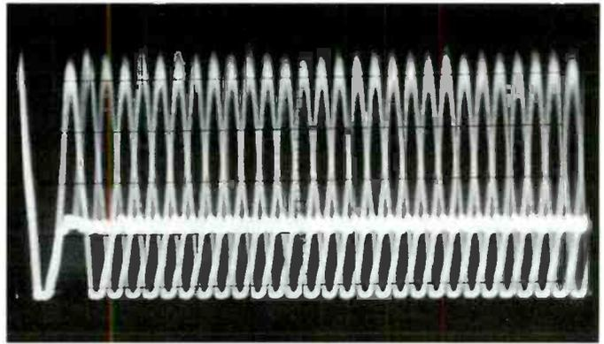
**Figure 4.** The PLL-VCO waveform voltage can be measured and adjusted from ground (bottom) to white or dark line. Some manufacturers use a frequency counter to adjust for the correct frequency.
