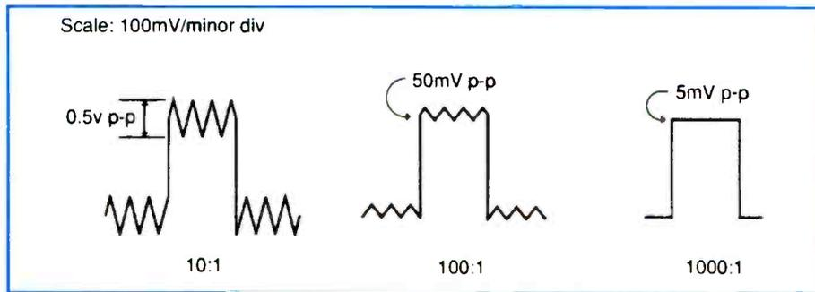
Figure 12. "Cleaning up" a signal by increasing the CMRR.
