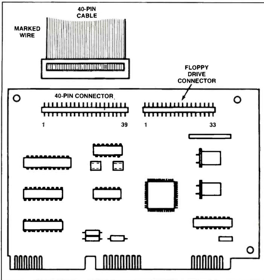
**Figure 2.** The IDE interface card has no "intelligent" electronics and works simply as an adapter. In IBM-compatible microcomputers, a 40-pin interface cable connects the drive to its interface while IBM computers use either a 40-pin or 72-pin cable.
