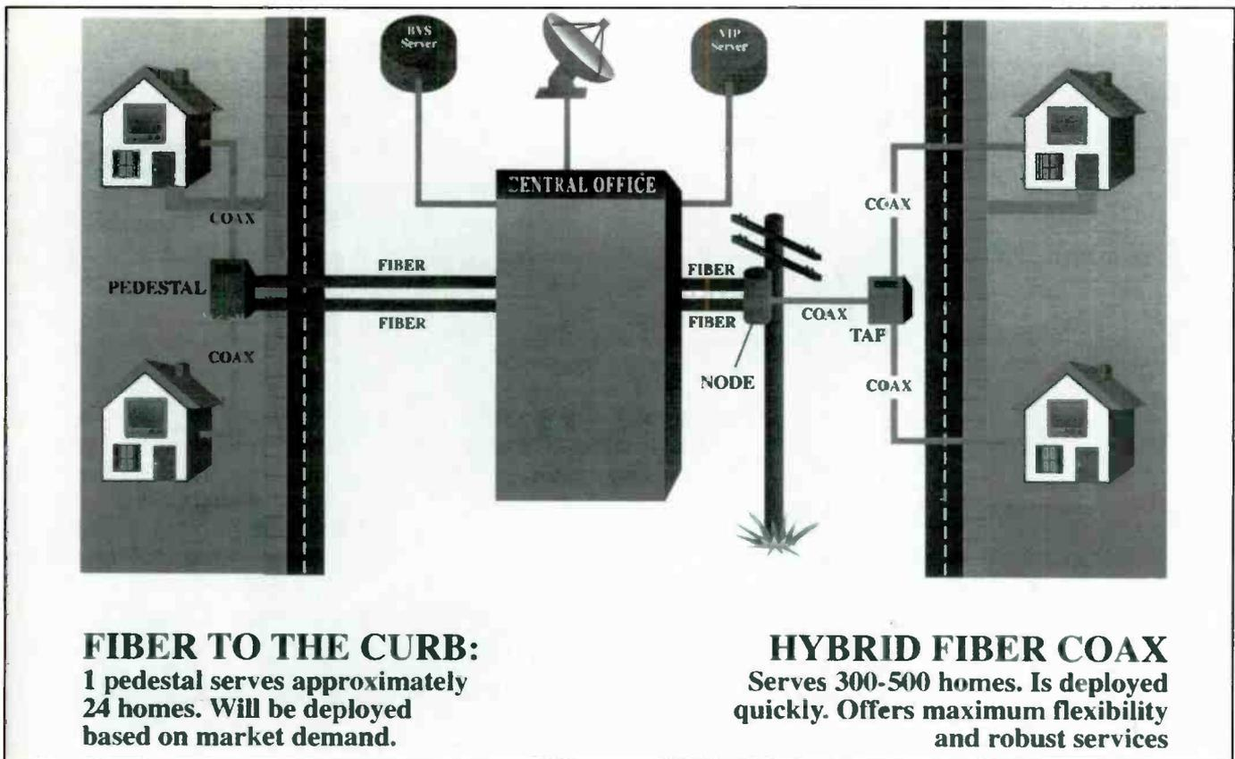
**Figure 2.** In a switched digital fiber-to-the-curb system, video programming and information are provided in a digitally compressed format (MPEG) by the video information providers and transported digitally by fiber optic equipment to the central office.
