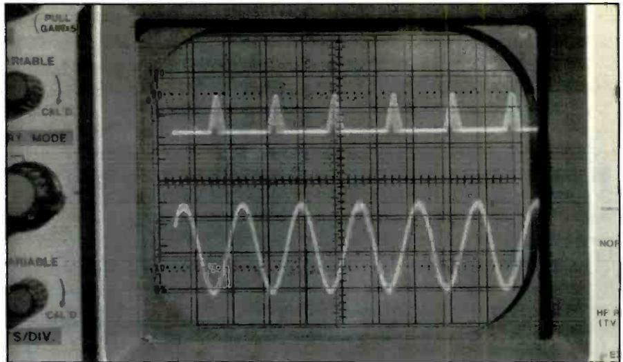
**Figure 6.** This oscilloscope photo shows the FG signal at pin 2 of IC203 (sinewave at bottom), a quad op amp. Pin 2 was the inverting input of the amp labeled "C.FG AMP". The spike at the top of the screen is the output of the op amp. The positive spike, present only when the motor was running well above its normal speed, occurred during the interval of the negative peak.
