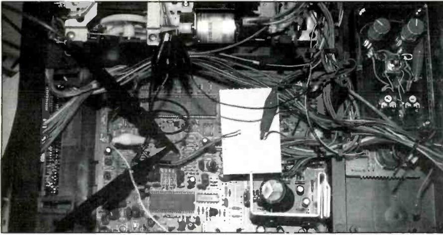
**Figure 4.** I opened the capstan motor control line and connected the device's positive lead to the motor side of the line and the negative lead to the VCR's ground.
