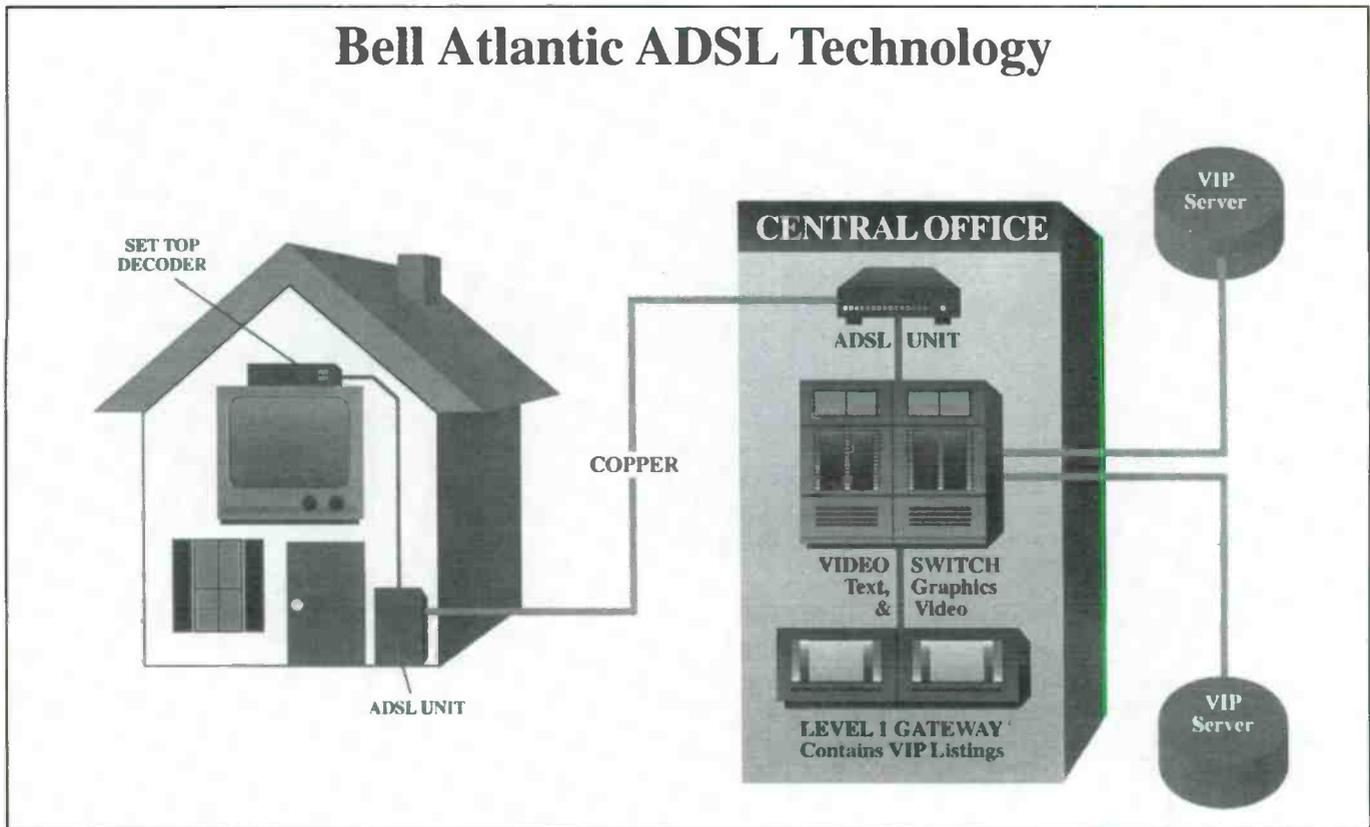
Figure 3. ADSL, in its present state of development, permits the multiplexing and transmission of a one-way, 1.544 Mbps digital signal along with the POTS (Plain Old Telephone Service) or basic rate ISDN (Integrated Switched Digital Network) signal, and a two-way signaling channel on an integrated basis over a single non-loaded copper pair.
