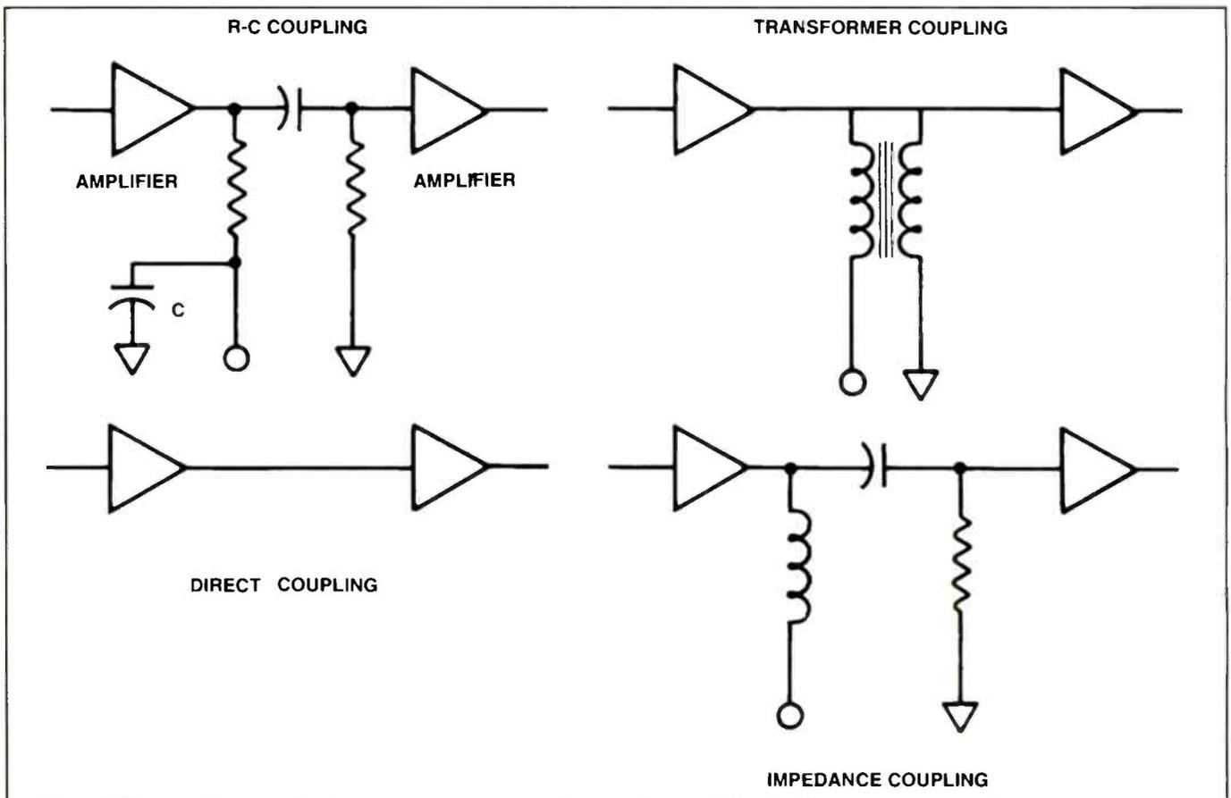
Figure 1. There are only four basic methods of coupling energy from one amplifier to another. R-C coupling, direct coupling, transformer coupling and impedance coupling.
