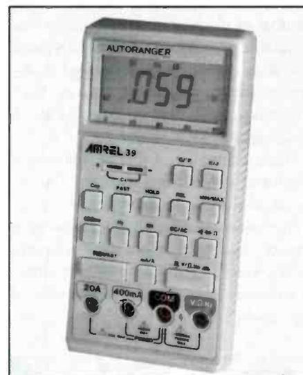
graph. Measurement ranges are 4nF to 4μF for capacitance measurement, 100Hz to 600KHz for frequency measurement, 400mV to 1000Vdc, 400mV to 650 Vac, and 400mΩ to 40MΩ for resistance measurement. They also offer relative mode, data-hold, min./max., memory/read function and true RMS (Model 37).
