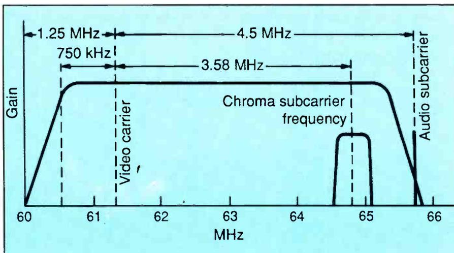
Figure 3. The frequency spectrum of a typical rf channel.
