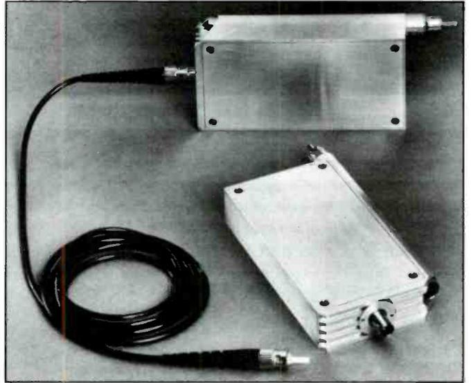
ment (Figure 3), permits the multiplexing and transmission of a one-way, 1.544 Mbps digital signal along with the POTS (Plain Old Telephone Service) or basic rate ISDN (Integrated Switched Digital Network) signal, and a two-way signaling channel on an integrated basis over a single non-loaded copper pair.
