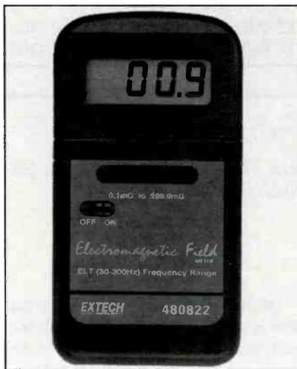
ELF frequency bandwidth of 30Hz to 300Hz. The unit is accurate to 4% at 50Hz to 60Hz with a sampling rate of 2.5 conversions per second to ensure reliable readings. Offering a 3½ digit 1.5 inch LCD readout with overrange indication, the EMF/ELF Meter monitors electromagnetic radiation levels from video terminals, fans, wiring, power lines, and numerous other sources.
