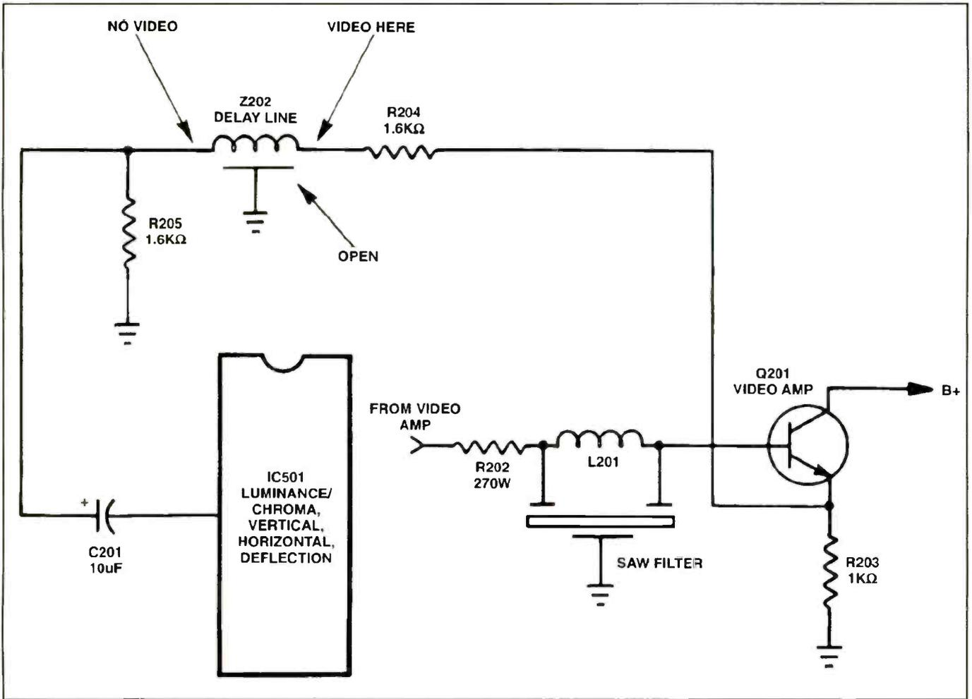
Figure 7. A Goldstar CMT-9428 portable set had no video. The cause of the problem was signal traced to an open delay line (Z202).
