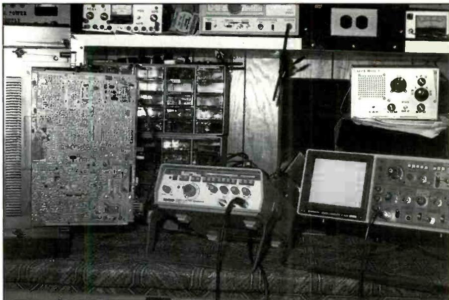
**Figure 1.** Video circuit problems can be diagnosed by signal tracing using a color dot-bar generator or a sine wave generator, with an oscilloscope as indicator.
