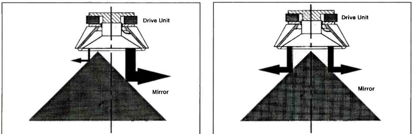
Figure 11. In this system, the sound is aimed at specially designed acoustic mirrors, which produces a stereo listening area greater than the area produced by conventional speakers.
