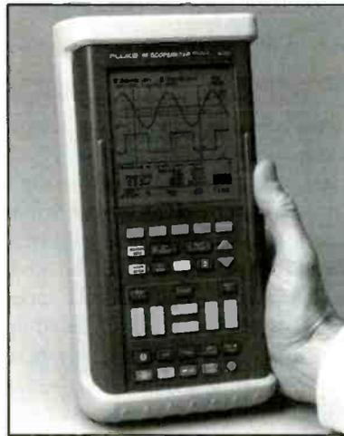
The menu offers direct access to 30 common measurement functions. The user selects the requested measurement from the menu, and the test tool configures itself to make the measurement.
