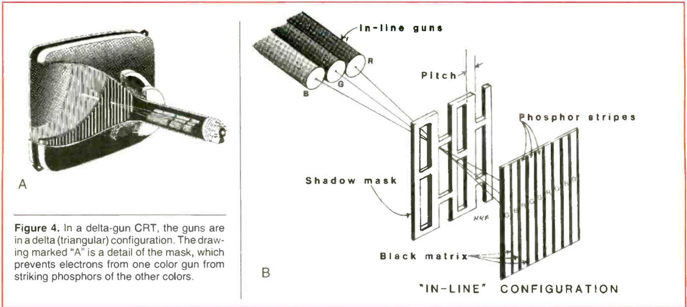
**Figure 4.** In a delta-gun CRT, the guns are in a delta (triangular) configuration. The drawing marked "A" is a detail of the mask, which prevents electrons from one color gun from striking phosphors of the other colors.
