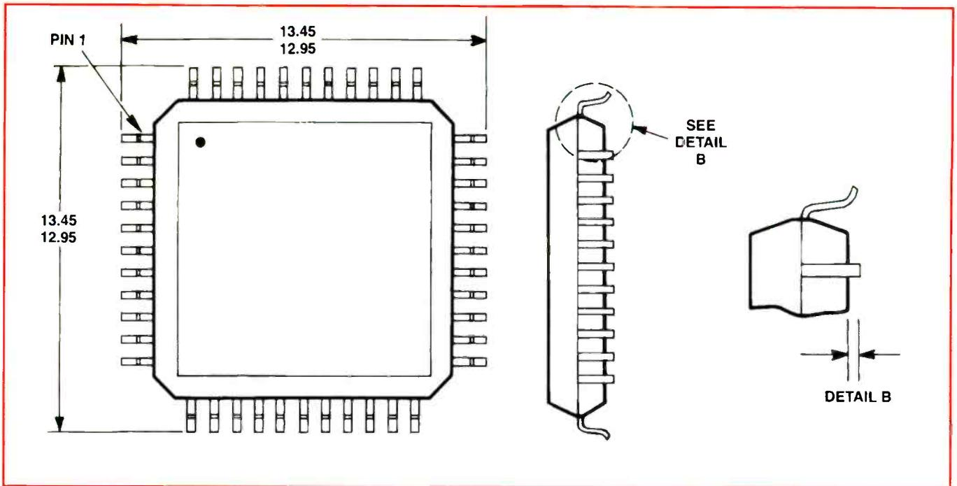
**Figure 7.** A plastic quad flatpack (PQFP) is a JEDEC approved package for devices that have 44 to 256 I/O's. 100 (20 x 30), 120 (30 x 30) and 160 (40 x 40) pins. The package has gull wing leads on all four sides and is characterized by bumpers on the corners. The body is slightly thicker than the QFP.
