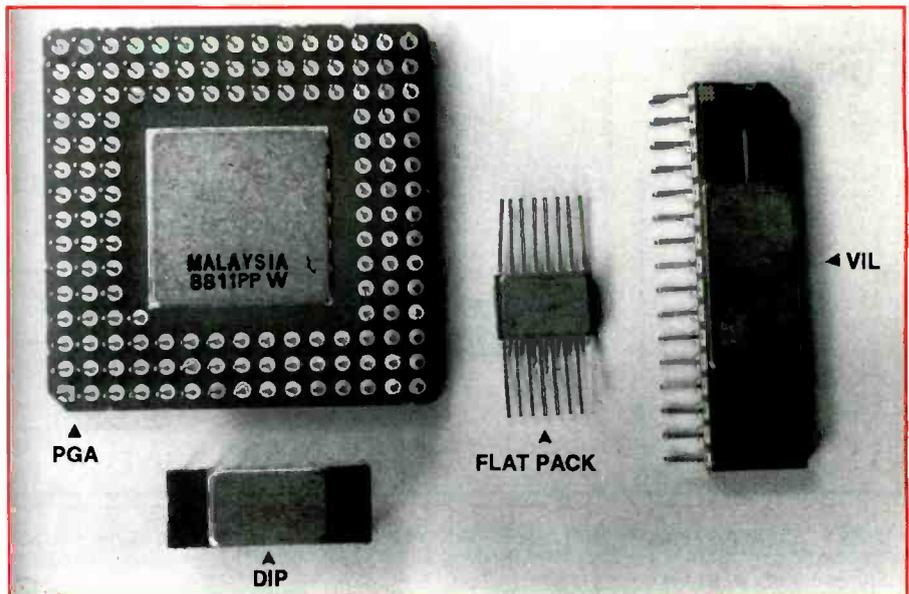
Figure 1. Advances in IC technology, and the needs of today's electronics circuitry, have led to the design and fabrication of IC packages such as the ones shown here.
