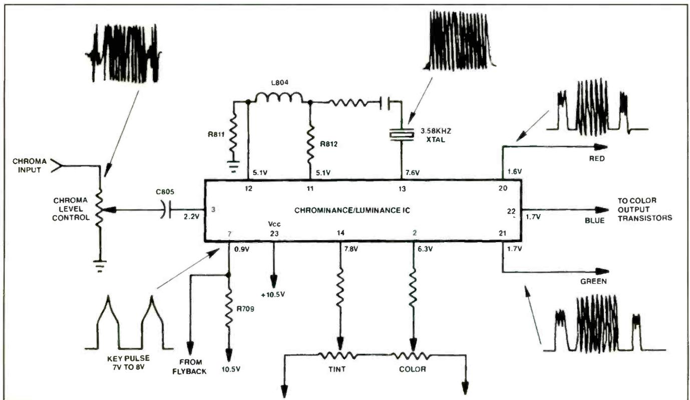
Figure 2. These are typical waveforms and voltages on the chrominance/luminance IC.
