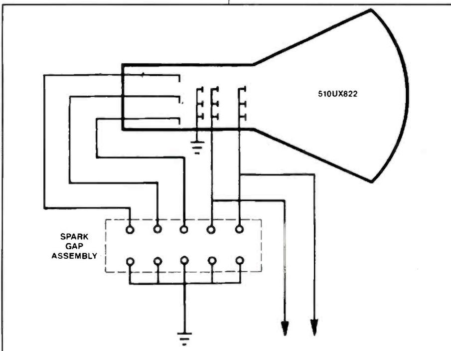
**Figure 11.** A bright blue raster followed by chassis shutdown was caused by dust in the spark gap assembly of a Samsung K25 chassis.
