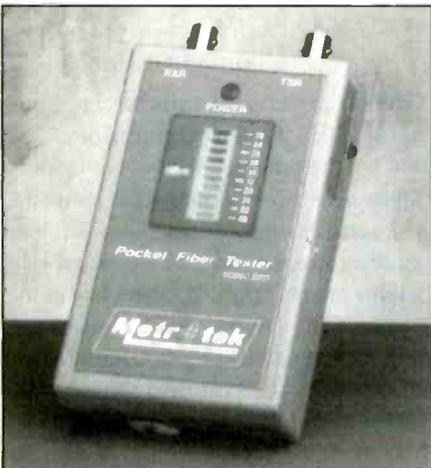
cator measures absolute optical power in 2dBm steps. The tester is available with ST or SMA connectors. Since it contains both a source and a receiver, the unit can be used to test a jumper or a spool of cable. A pair of testers can be used to test long fiber runs between equipment bays or between buildings.
