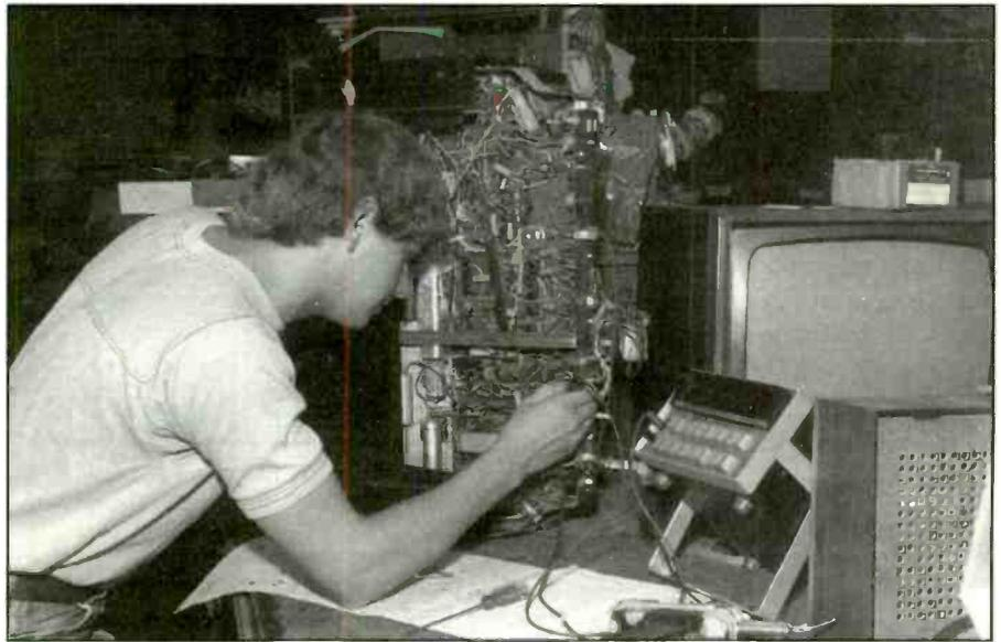
Figure 1. Voltage measurements in the color circuits can help to determine the cause of color problems.
