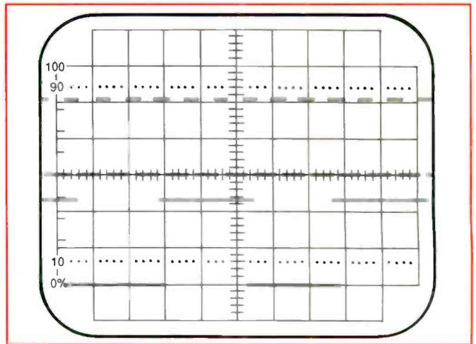
**Figure 3.** The top waveform is the separated PG pulse output at pin 1 of IC2003. The lower waveform is the separated and stretched PG pulse at pin 14 of IC2003 used for headswitching and phase compar-
