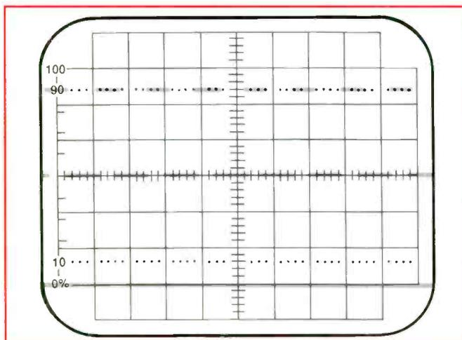
**Figure 4.** The upper waveform is the speed PWM output (pin 13). The duty cycle of this waveform varied during acceleration bursts. The lower waveform is the phase PWM output at pin 12. This waveform showed 5V between acceleration bursts.
