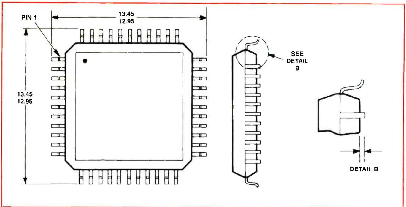
**Figure 7.** A plastic quad flatpack (PQFP) is a JEDEC approved package for devices that have 44 to 256 I/O's. 100 (20 x 30), 120 (30 x 30) and 160 (40 x 40) pins. The package has gull wing leads on all four sides and is characterized by bumpers on the corners. The body is slightly thicker than the QFP.
