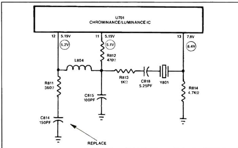
Figure 9. Intermittent color in the RCA CTC120 chassis was caused by an intermittent bypass capacitor, C814.
