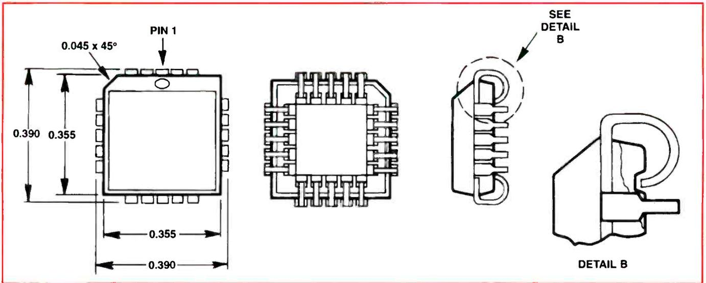
**Figure 4.** The J-lead plastic chip carrier (PLCC) has leads that exit the body then turn under the component in a curve that resembles the letter J. The leads and the solder joints are relatively strong, but because the solder pads are under the package, removal of these ICs during service can be a problem.
