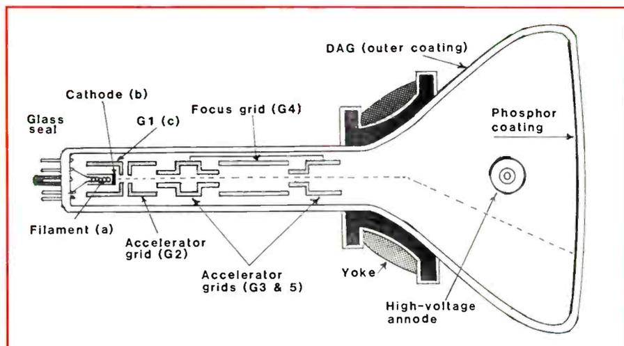
Figure 2. The more commonly used magnetic deflection tubes require a "yoke" mounted on the neck of the tube to deflect the electron beam.
