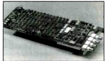
The generators also provide 0.01% frequency accuracy, five selectable output filters, gain and offset controls, and nine built-in waveforms. The output waveforms are accessible via BNC connectors as is the sync out signal. An input BNC connector is provided for signals triggering the generator or for use with an external reference clock. Both generators are capable of 10MHz sine waves and pulses with 20ns widths and 12ns risetimes.
