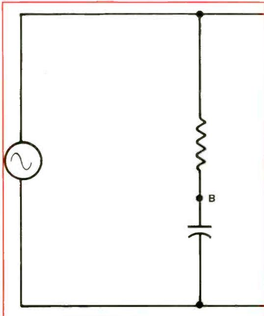
**Figure 3.** Does the voltage at point B in this circuit lead or lag the applied sinewave voltage?
