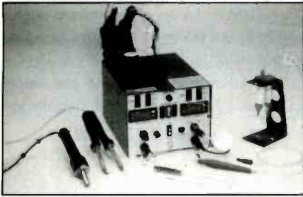
desoldering, reflow soldering, heat tweezing, vacuum handling, conventional soldering, and solder paste dispensing.
