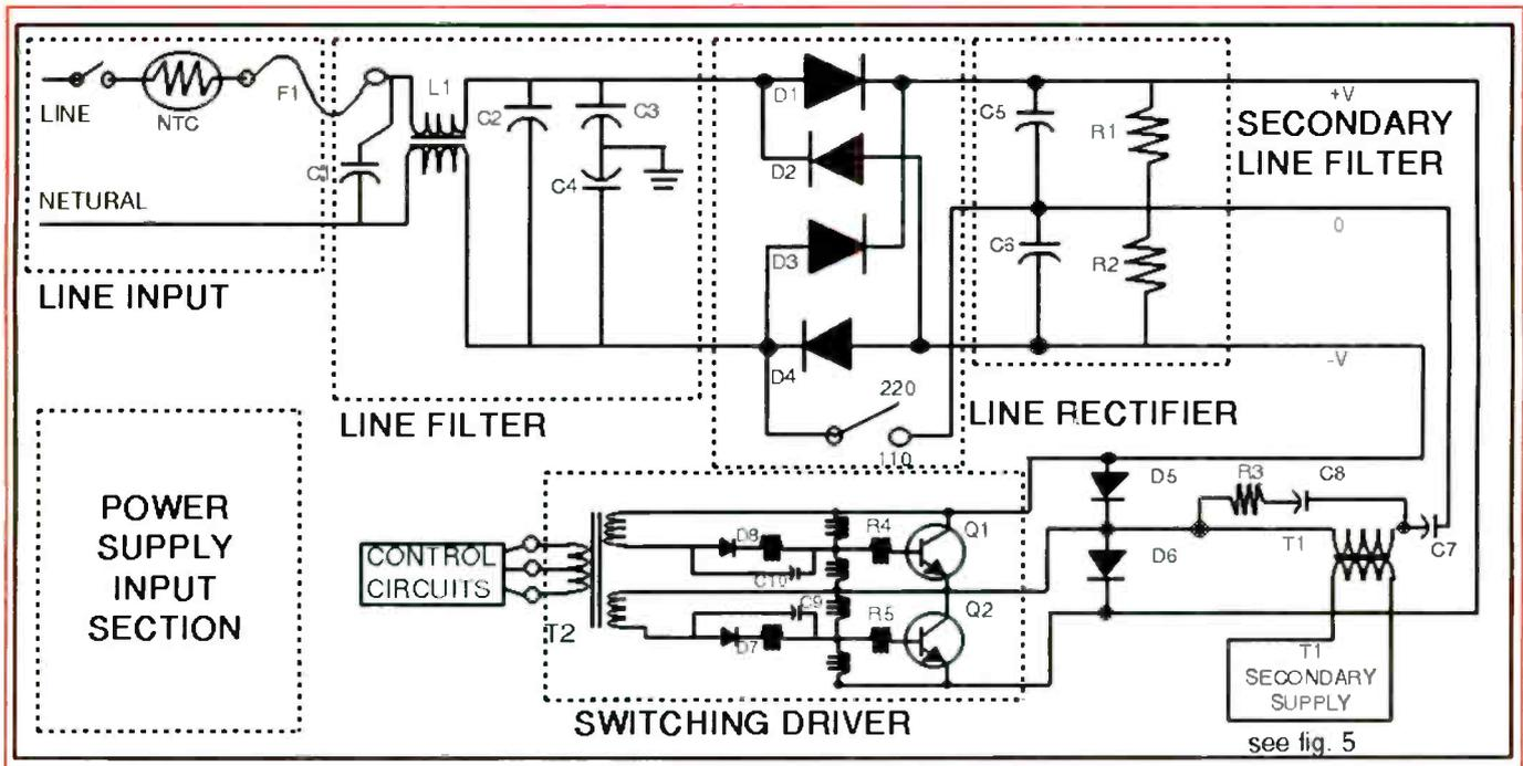
**Figure 4.** A typical computer power supply input section. In the line input section you will notice the off/on switch, fuse, and the NTC (negative temperature coefficient) thermistor. This thermistor has a high resistance when cold, and as it heats up its resistance decreases. This limits the surge of current when the supply is switched on.
