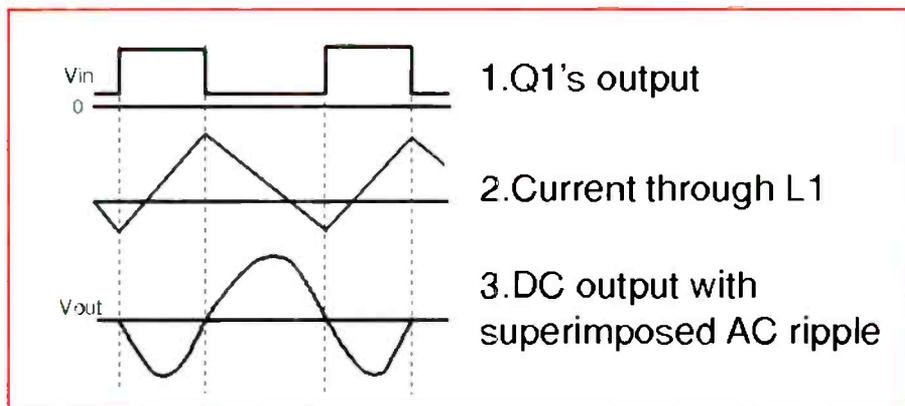
**Figure 2.** The self-oscillating regulator of Figure 1 will produce an output signal that looks like this.
