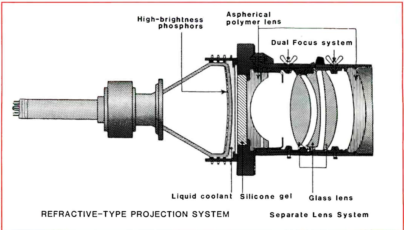
Figure 7. Another type of separate-tube projection CRT is the refractive system.
