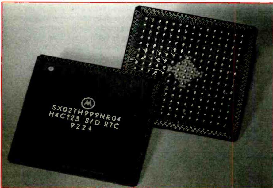
**Figure 8.** This IC package, the OMPAC ball grid array, comes with solder balls attached to the connectors. It is placed on the PC board and the solder reflowed. Fortunately, these ICs, which would be all but impossible for a consumer electronics service center to handle, are not used in consumer products. (Photo courtesy Motorola)
