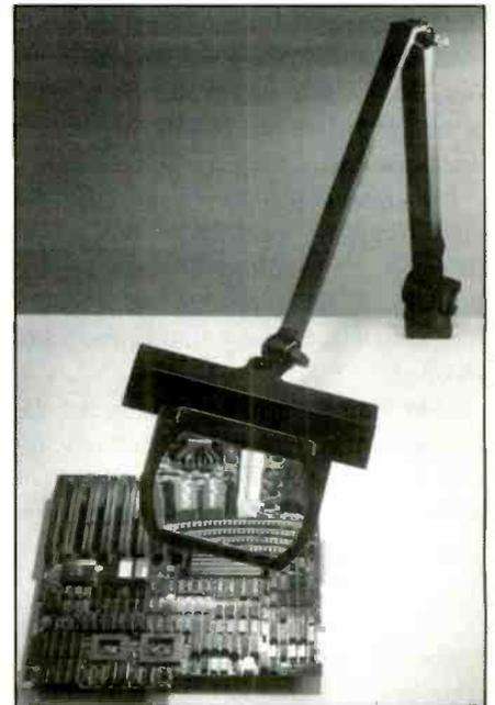
All plastic luminaire parts are manufactured with static dissipative materials. The optical quality glass magnifier has a multi-layer conductive coating, and all metal parts are coated with a static dissipative varnish. The lamp diffuser also has a tin oxide conductive coating.
