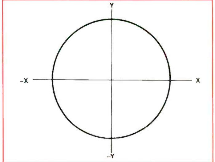
**Figure 2.** This Lissajous pattern is obtained with two sinewaves of equal frequency and equal amplitude. What is their phase relationship?
