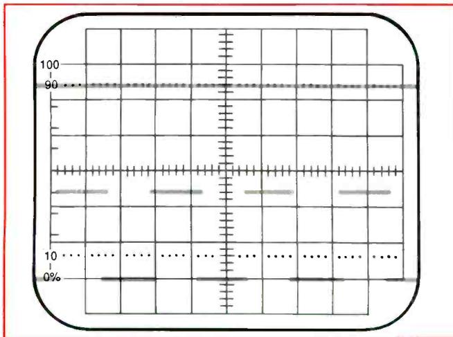
**Figure 6.** The upper waveform shows the speed PWM output (pin 13) at 100% duty cycle with the motor speed raised above normal. The lower waveform is the phase PWM output (pin 12). This signal defaults to a 50-50 duty cycle when the motor speed is raised above normal.
