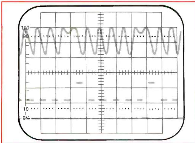
**Figure 2.** The top waveform here is the output of the Hall device, observed at pin 9 of IC2603. The lower waveform is the output of the PG/FG processor at pin 15 of IC2603.
