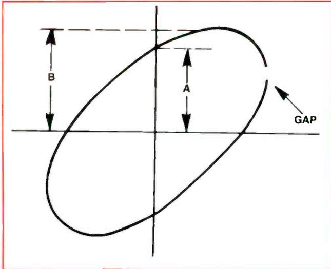
**Figure 1.** If  $A=5$  and  $B=6$ , what is the phase angle between the sinewaves that produced this pattern?
