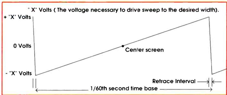
**Figure 3.** The waveform that provides horizontal sweep in a CRT is called a "sawtooth waveform" because of its appearance. It must move the electron beam in the tube horizontally at a constant rate of speed in order to faithfully reproduce the signal applied to the vertical plates.
