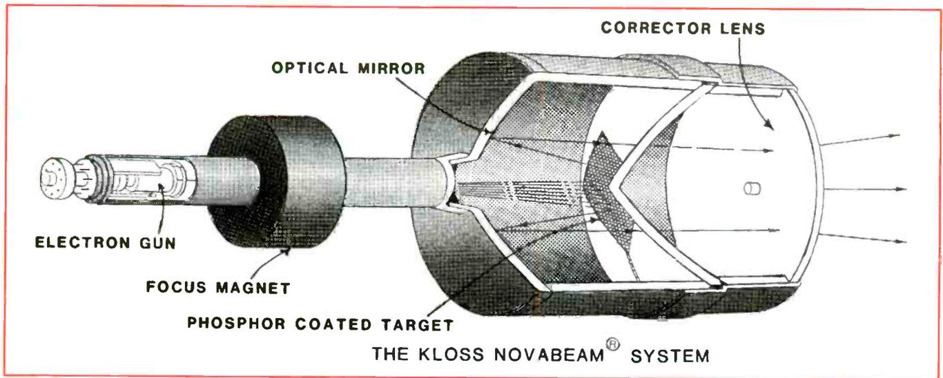
Figure 6. Some projection systems use three separate CRTs: a red tube, a green tube and a blue tube. When the pictures from these three tubes are superimposed into a single picture, a color picture is produced. This is a Novabeam tube, based on the Schmidt optical system, developed by Henry Kloss.
