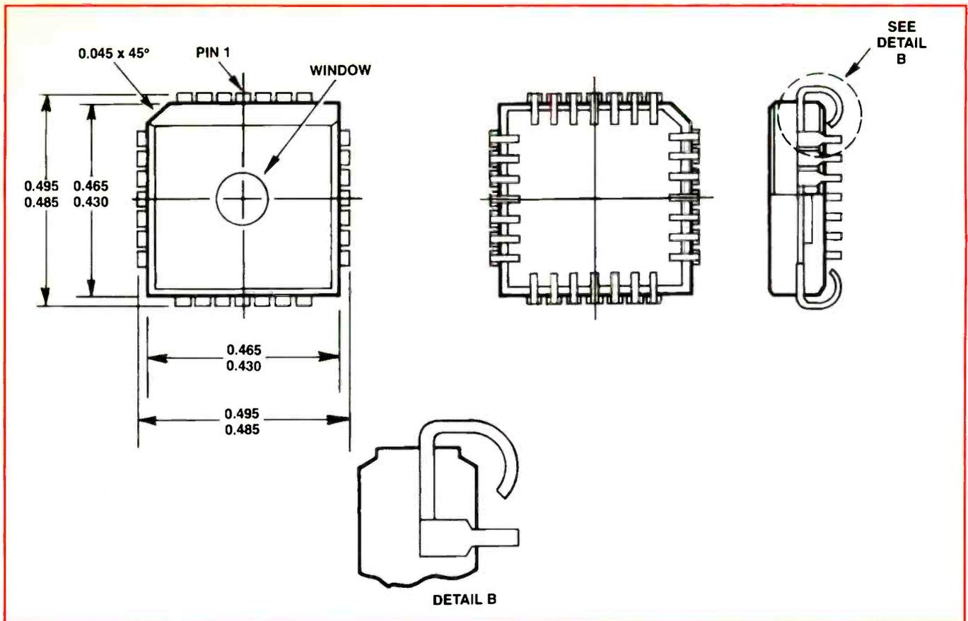
**Figure 5.** The J-lead ceramic chip carrier (JLCC) is similar to the PLCC shown in Figure 4, except that instead of plastic, the body is made of ceramic material. Ceramic ICs are found in military applications where the package must be hermetically sealed.
