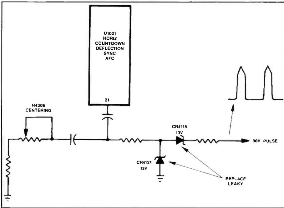
**Figure 10.** Weak horizontal sync and loss of color in an RCA CTC169 were caused by leaky zener diodes CR4121 and CR4115.
