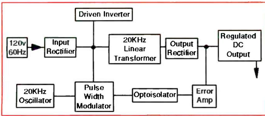
**Figure 3.** This block diagram of a typical computer power supply bears a family resemblance to circuit in Figure 1.
