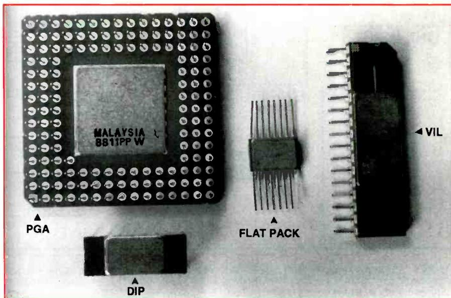
Figure 1. Advances in IC technology, and the needs of today's electronics circuitry, have led to the design and fabrication of IC packages such as the ones shown here.
