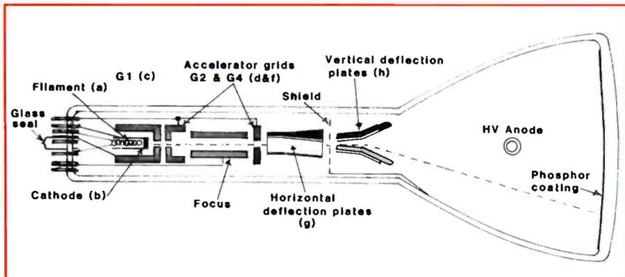
Figure 1. The deflection plates in electrostatic deflection tubes are built inside the tube.
