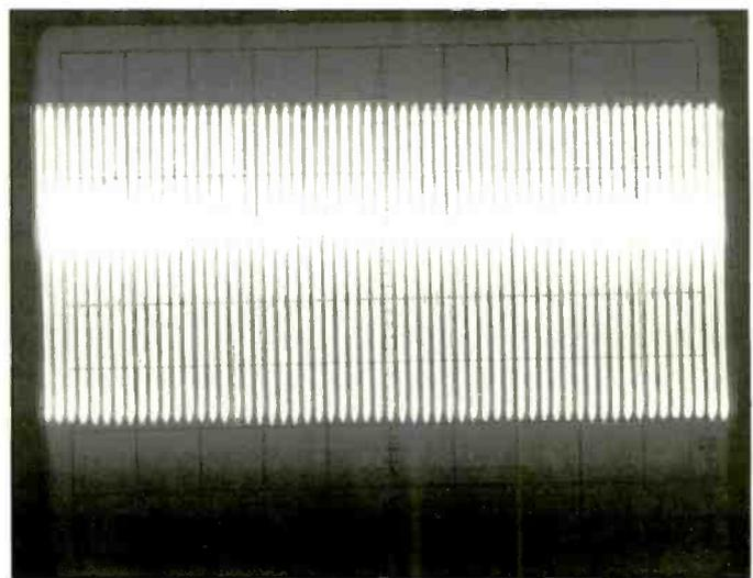
**Figure 5.** The waveform of a normal 3.58MHz crystal tied to one of the chroma IC terminals.
