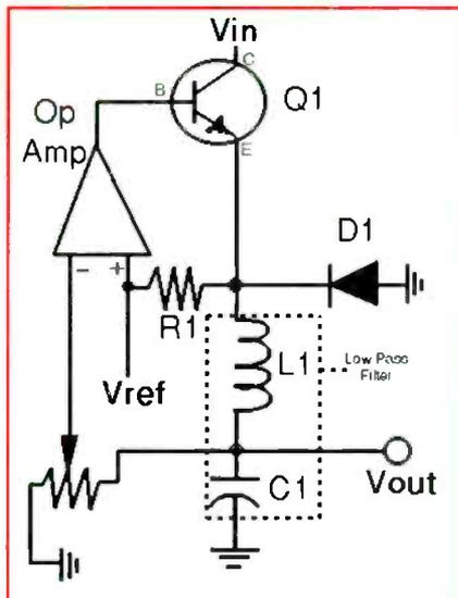
**Figure 1.** This switching circuit is known as a self-oscillating regulator. The transistor Q1 used in this circuit is commonly known as a pass transistor. L1 and C1 form a low pass filter. When Q1 is off, the current stored in L1 and C1 during Q1's last on state, becomes the source of load current. The diode D1 gives the inductor current a return path, and it is often known as a freewheeling diode.
