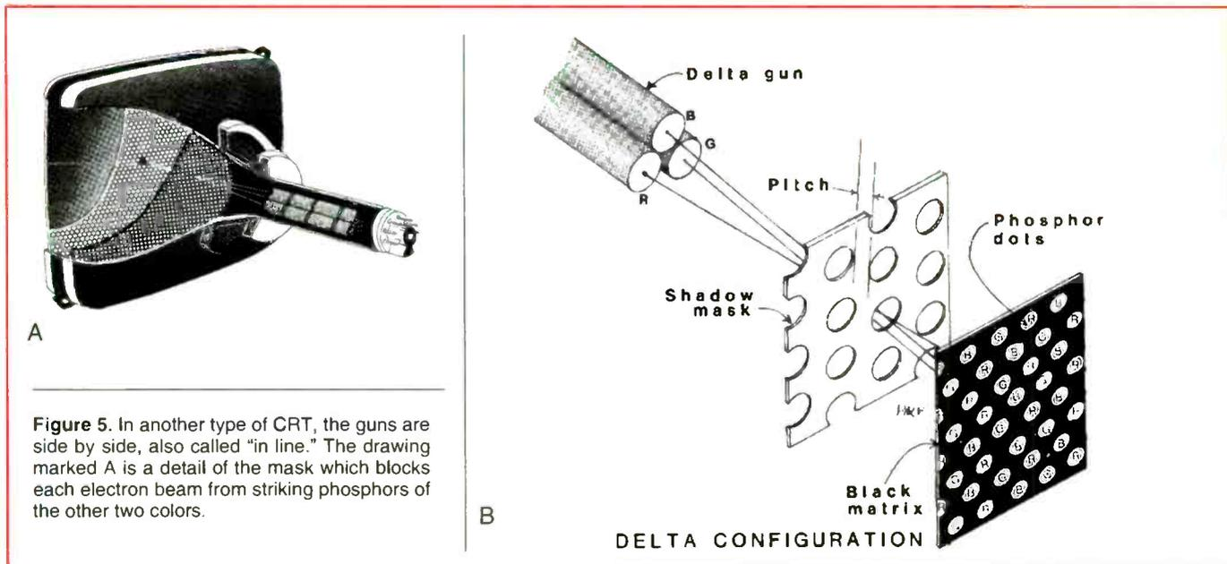
**Figure 5.** In another type of CRT, the guns are side by side, also called "in line." The drawing marked A is a detail of the mask which blocks each electron beam from striking phosphors of the other two colors.
