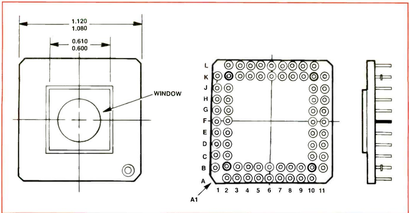
**Figure 6.** A pin grid array (PGA) is a square package with pins covering the entire bottom surface of the package.
