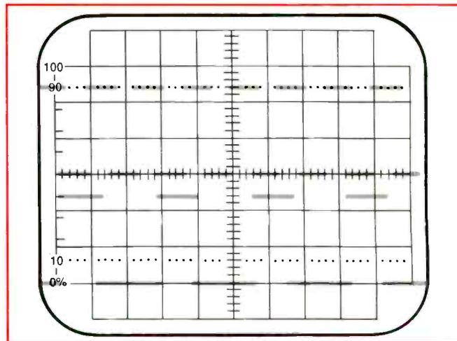
**Figure 7.** These waveforms show the speed PWM (top) and the phase PWM (bottom) outputs after the problem was corrected.
