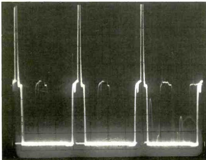
**Figure 4.** If the keyed-burst waveform is missing from the color IC, there will be no color at the output of the chroma IC.
