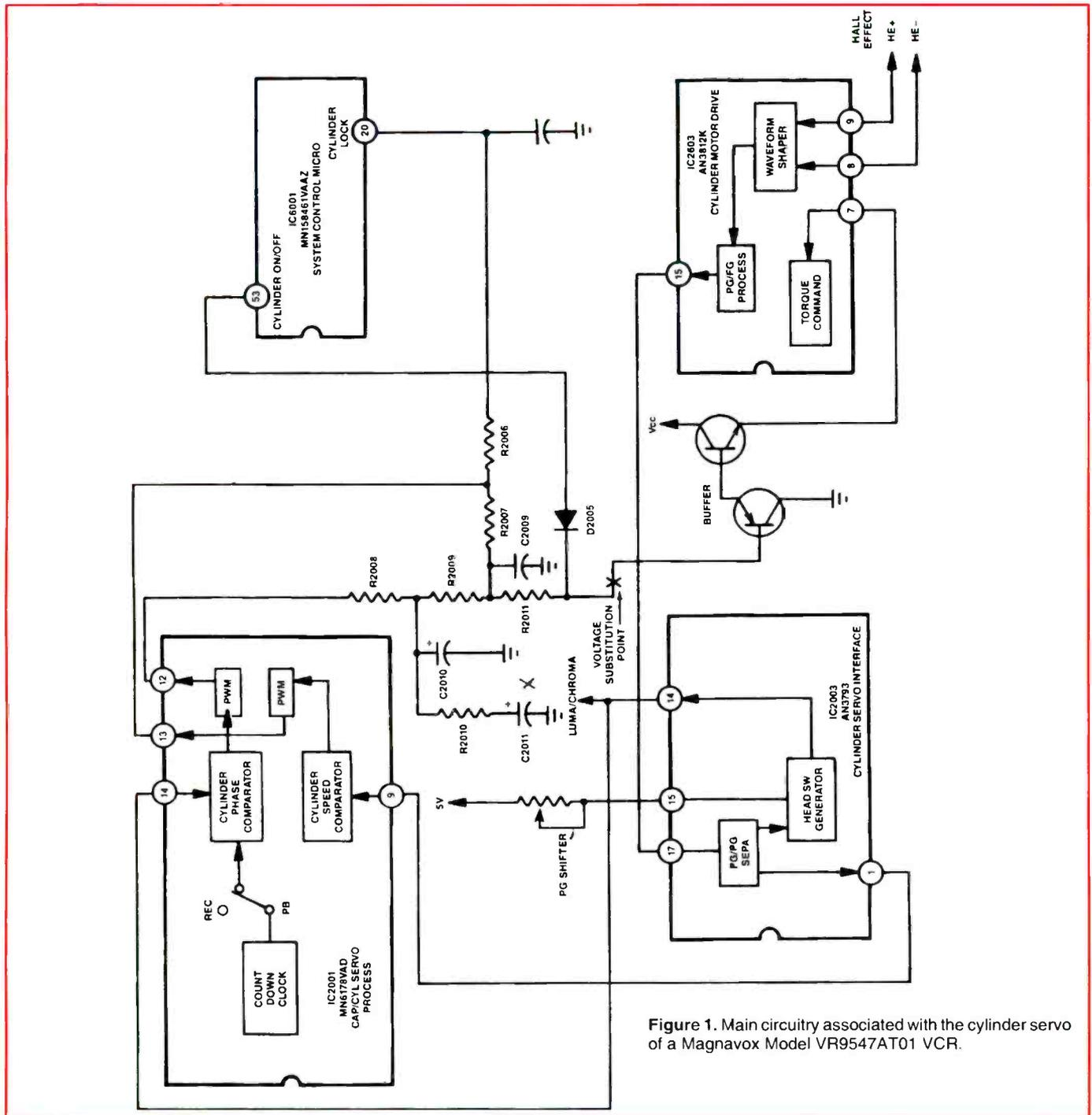
Figure 1. Main circuitry associated with the cylinder servo of a Magnavox Model VR9547AT01 VCR.
