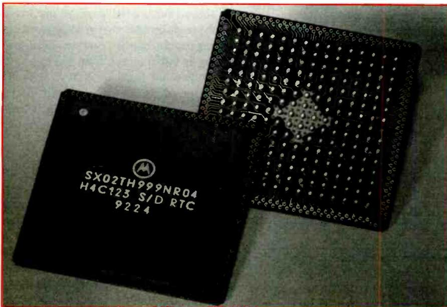
**Figure 8.** This IC package, the OMPAC ball grid array, comes with solder balls attached to the connectors. It is placed on the PC board and the solder reflowed. Fortunately, these ICs, which would be all but impossible for a consumer electronics service center to handle, are not used in consumer products. (Photo courtesy Motorola)
