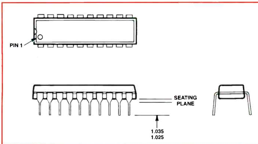
**Figure 3.** The 20-pin plastic dual-in-line package (PDIP) was one of the early, and still popular, types of IC package.
