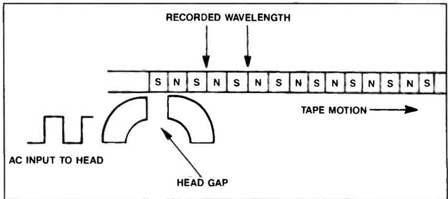
**Figure 4.** The actual size of the small magnetized areas of the recorded tape is called the "recorded wavelength." The recorded wavelength is determined by the tape speed and signal frequency.
