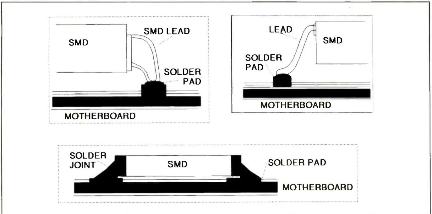
Figure 2. Three types of Surface Mounted Devices.
