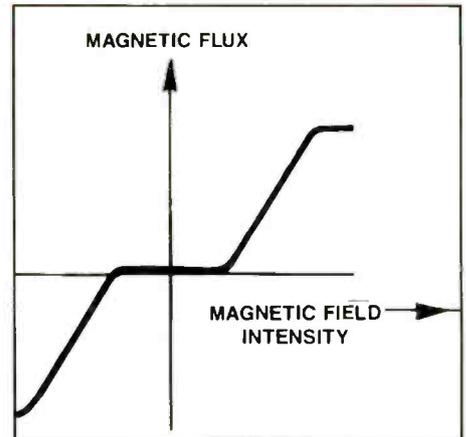
Figure 1. The biggest problem caused by the nonlinear characteristic of the tape's ferromagnetic material occurs at the lower end of the characteristic curve, shown here, where alignment of the magnetic domains does not start to occur until some definite, non-zero amount of magnetizing field is applied.
