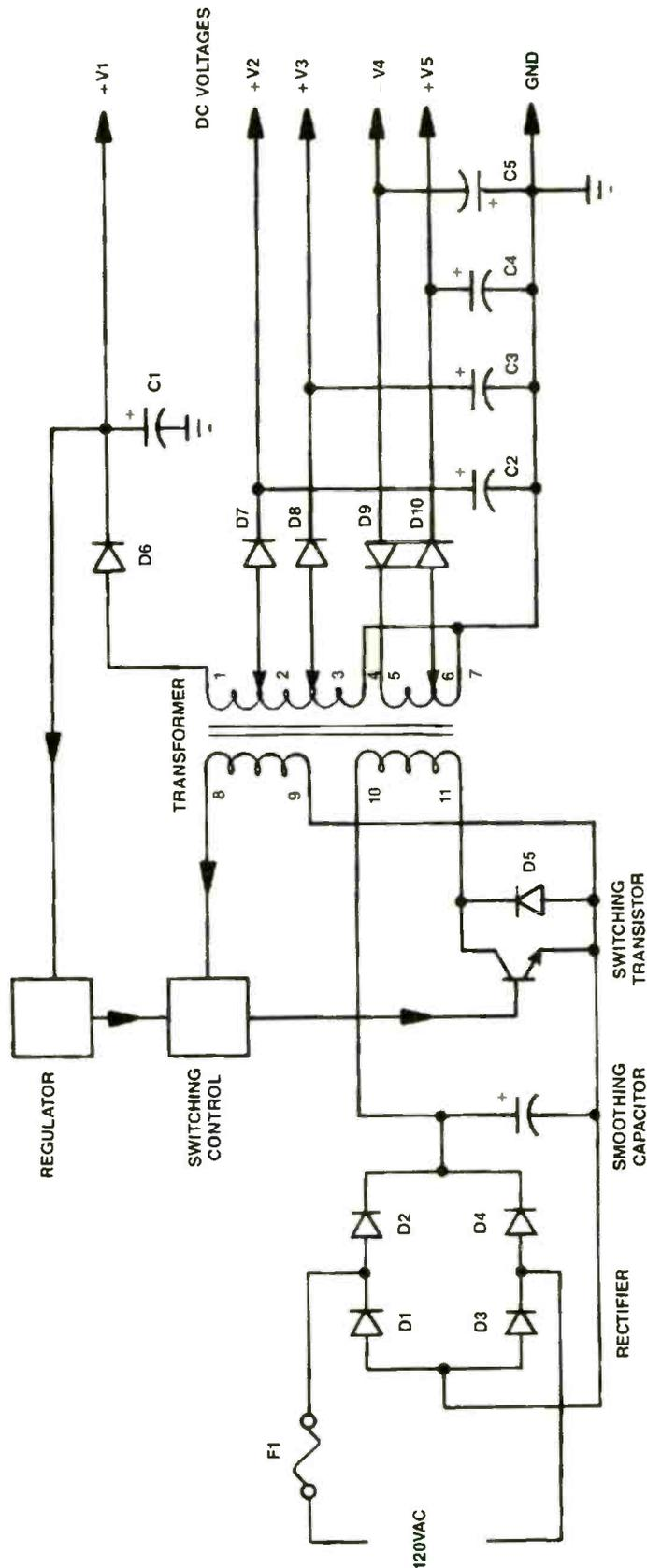
**Figure 3.** Conditions in a switch-mode power supply (SMPS) are different from those in a linear power supply. In this SMPS circuit the diodes are the first components exposed to the surge. The switching control and the switching transistor are also in danger, but very often the smoothing circuit with the high capacitance protects these components.
