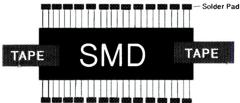
**Figure 4.** Be careful not to let solder short to another pad. Use very fine wire solder and a fine tip iron. In many SMDs the leads are .25 inches apart or less.
