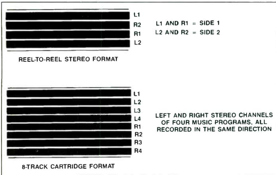
Figure 6. The track formats for R-R and the now obsolete 8-track recorders.
