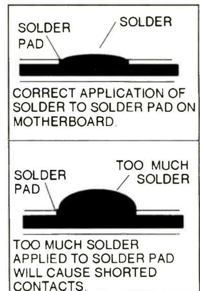
Figure 3. It does not require much solder on the pad to hold the SMD properly.
