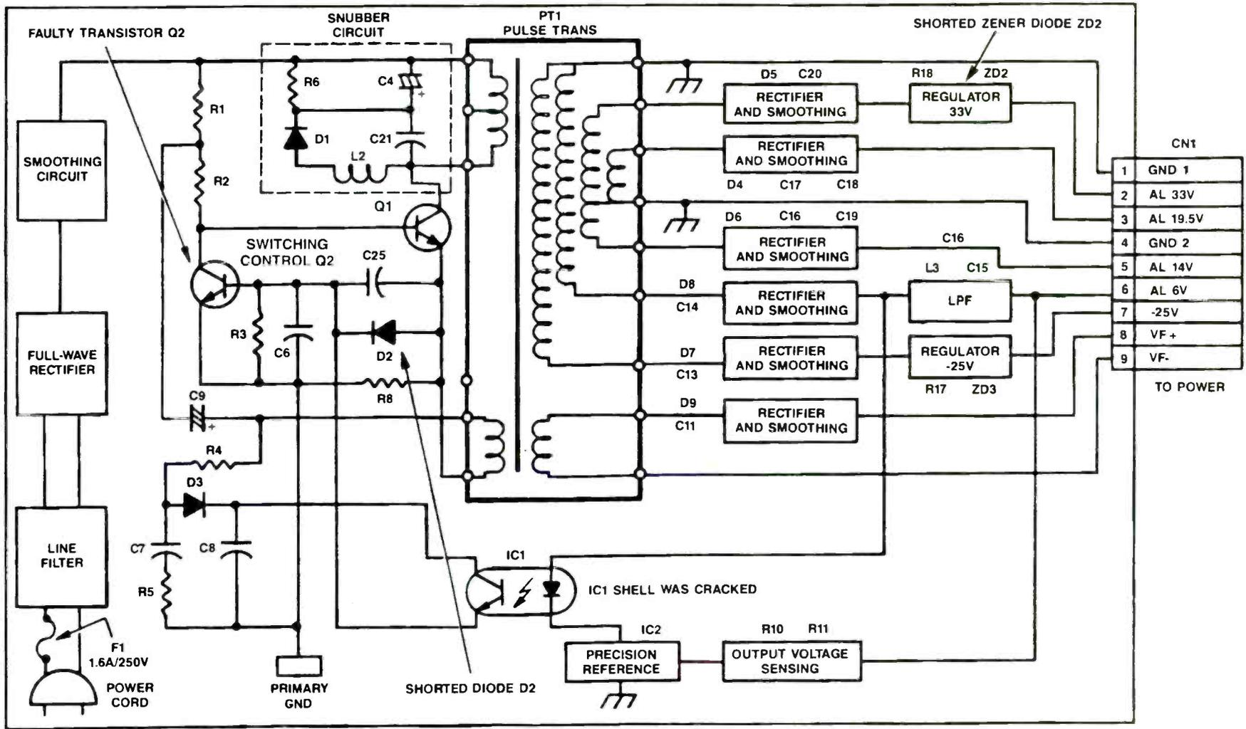
Figure 4. Power supply of the Toshiba VCR model M-228. IC1, which was cracked, is an optocoupler that regulates the switching control and provides isolation between the secondary side and the primary 120Vac part of the SMPS.
