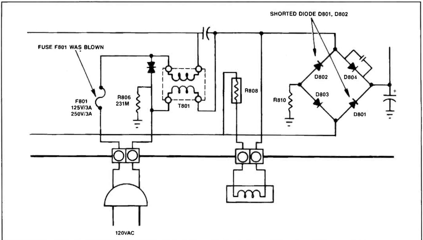
Figure 5. Part of the power supply of the Toshiba TV, CF1311J
