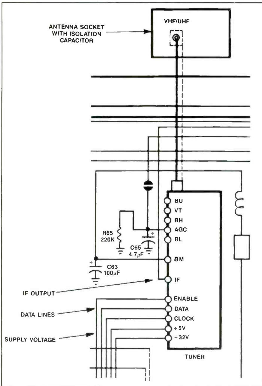
Figure 6. The tuner of the Toshiba TV, CF1311J
