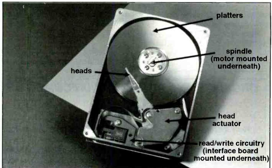
Figure 2. Here is a current hard drive assembly showing the five critical elements.
