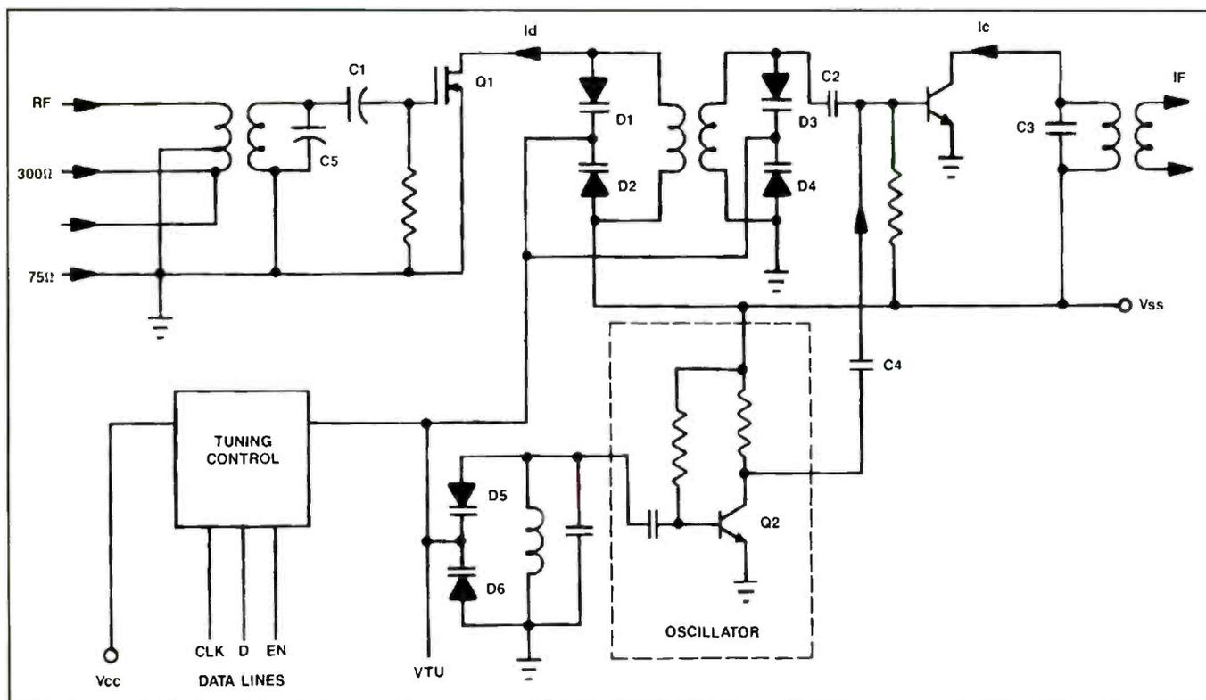
Figure 1. Shows a typical tuner schematic. If a lightning surge gets into the antenna input, the first component to be destroyed is usually transistor Q1, which is a MOSFET in this example.
