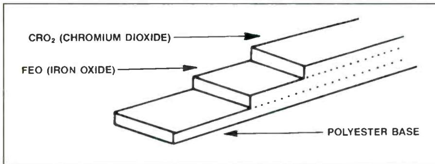
Figure 7. Audio tape is constructed something like this.
