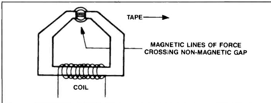
Figure 3. The head places the varying alignment of the magnetic domains on the tape.
