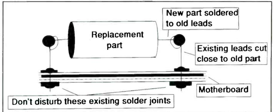
Figure 1. Leave the existing leads in the motherboard by cutting close to the old part. Then, bend the old leads and solder the new part in without disturbing the motherboard.
