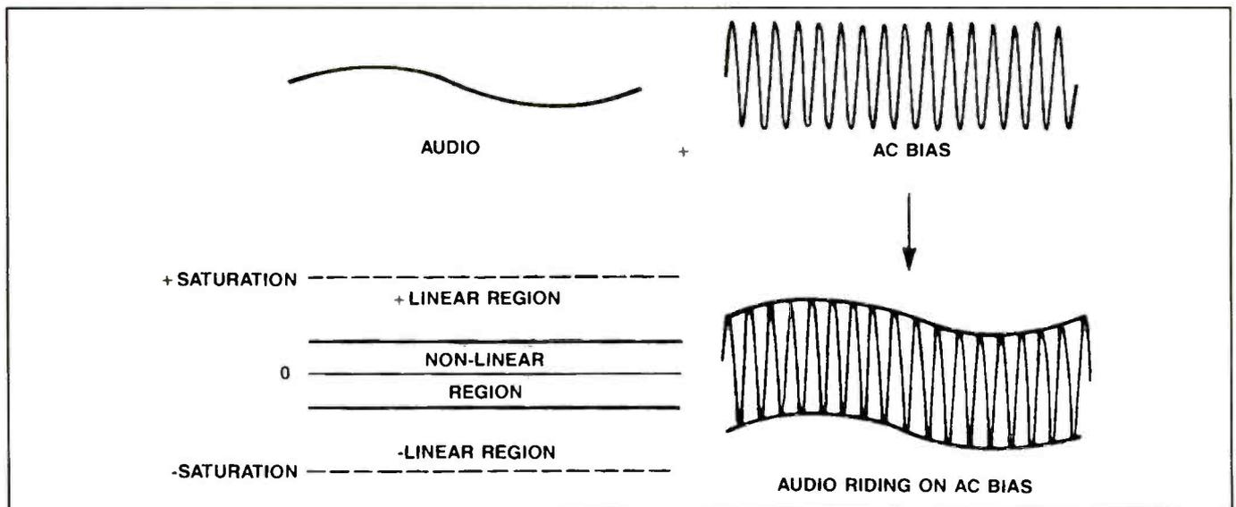
Figure 2. To place the audio signal in the linear region, an ultrasonic bias, in the range of 60KHz to 100KHz, is used.
