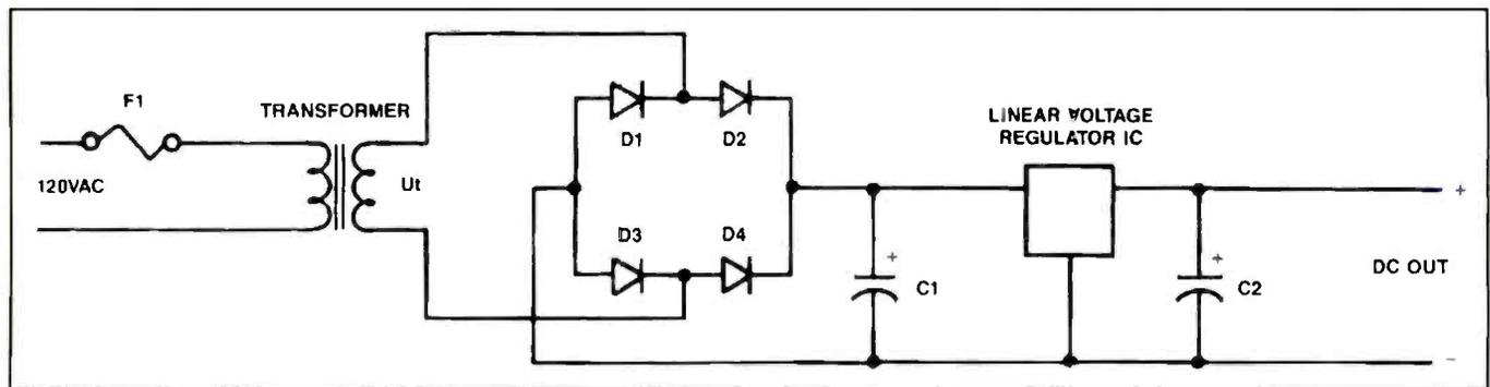
**Figure 2.** In the linear power supply shown here, the power transformer and the diodes are directly exposed to any type of surge on the ac line. These are the components most often destroyed in a lightning storm.
