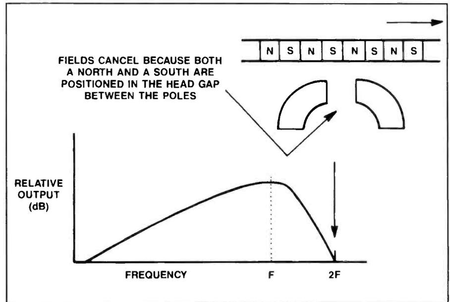
**Figure 5.** This illustration shows the change in relative output of the head as the frequency changes. The recorded wavelength is equal to the writing speed divided by the signal frequency.
