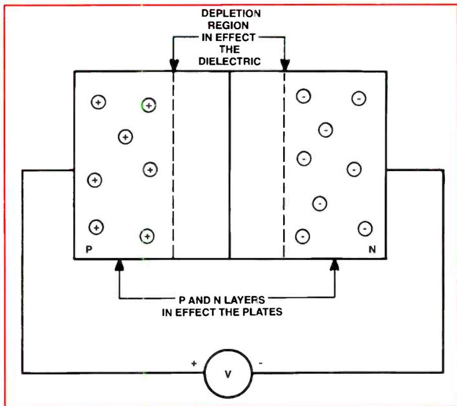
**Figure 3a:** When the reverse bias is increased, the depletion region is widened, effectively increasing the distance between the "plates" hence decreasing the capacitance.
