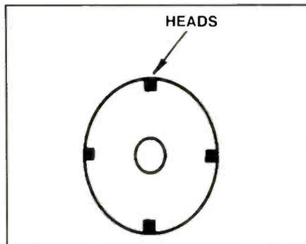
**Figure 1.** The video heads are arranged in this fashion on the quad scanner cylinder. Tape motion is perpendicular to the plane of the cylinder.
