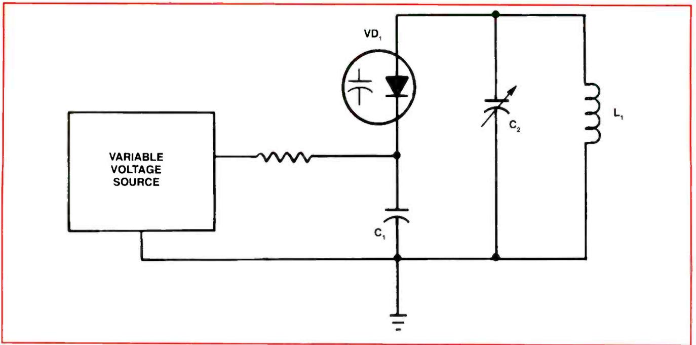
**Figure 3b:** C1 acts as a short to the frequency of interest while isolating the tune voltage from ground. This places the capacitance of VD1 in parallel with C2 and L1. By varying the voltage on VD1, the resonant frequency of the tuned circuit can be changed.
