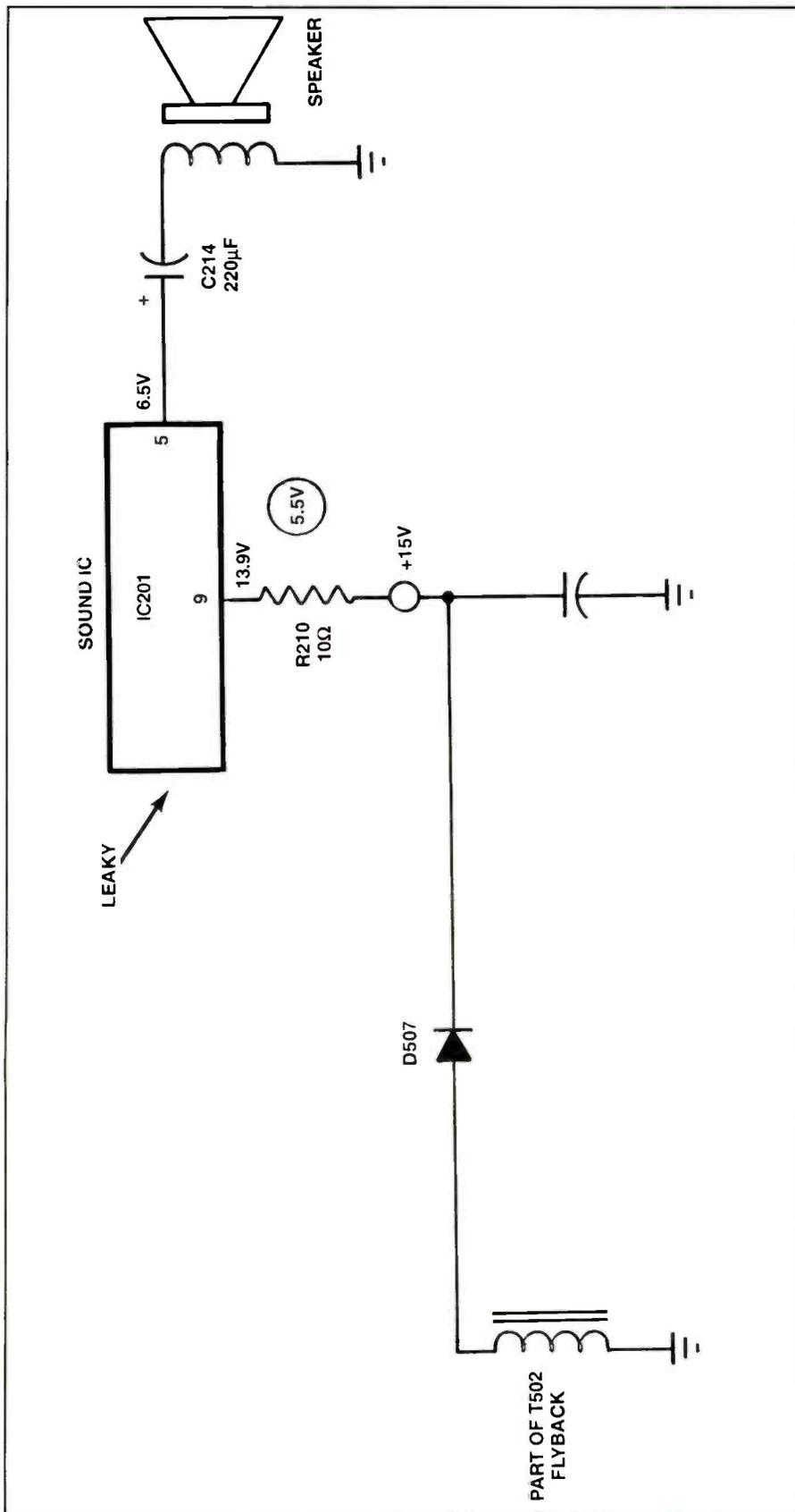
**Figure 6.** When one end of R210 was disconnected from the circuit in this set, the secondary voltage source returned to normal. The problem was found to be a leaky sound output IC, IC201.
