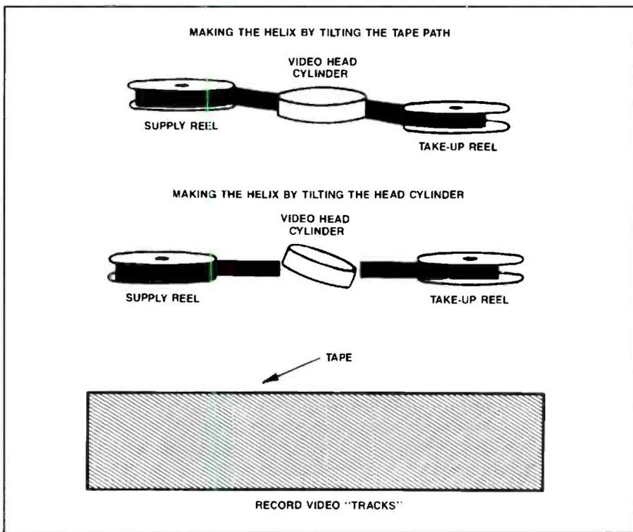
**Figure 4.** One of two methods can be used to create the helical scan pattern of the video signal on the video tape: tilt the tape path or tilt the head cylinder. Modern VCRs tilt the head cylinder because this method can use a smaller, less expensive, cassette. A general idea of the physical arrangement of the video tracks on the tape is shown at the bottom of the figure.
