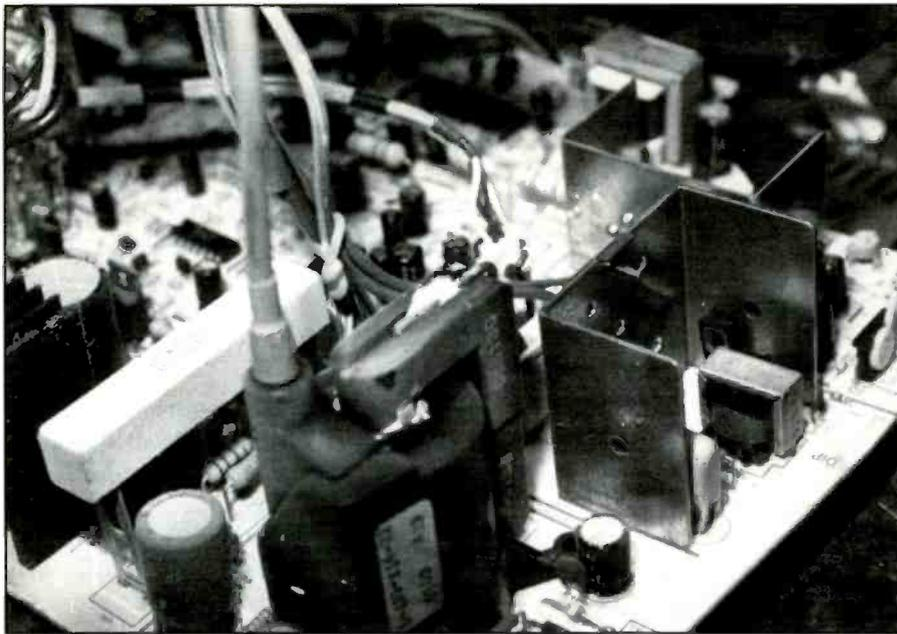
**Figure 7.** Chassis shut-down may occur when one of the circuits supplied by the secondary of the flyback transformer becomes leaky and loads down the supply.
