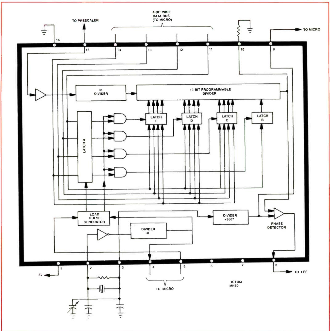
**Figure 7:** One of the more complex blocks in the voltage synthesizer system is the PLL. In this case the internal block diagram of the PLL was shown on the schematic and proved very helpful in troubleshooting.
