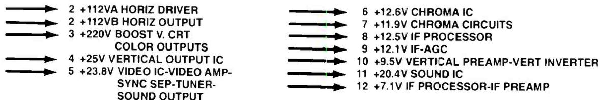
**Figure 3.** The voltage sources shown here numbered, are powered by the flyback secondary. These sources provide power to most of the circuits in this set.
