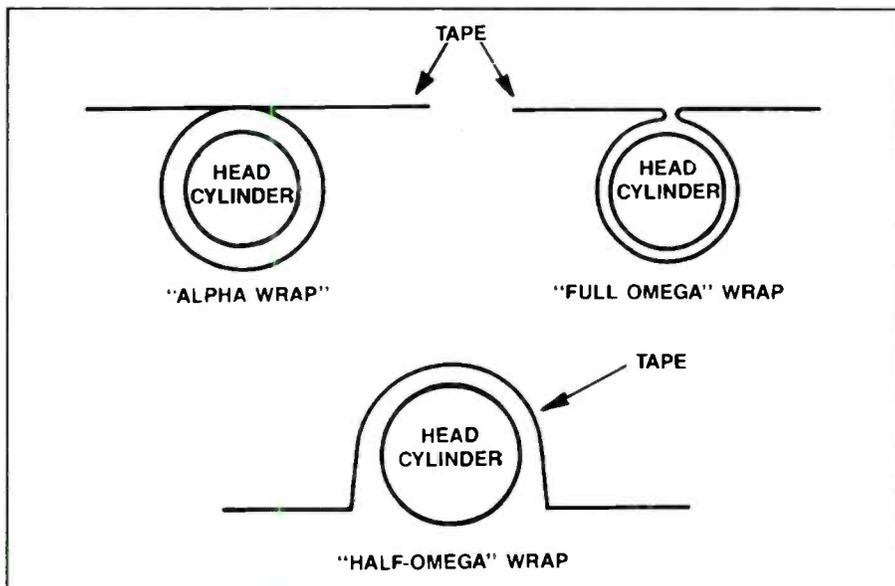
**Figure 3.** The scanner in VCRs that employ "alpha" wrap and the full "omega" wrap, each so called because the arrangement of the tape resembles the respective Greek letter, uses only a single video head. All modern VCRs use the "half-omega" wrap scheme, which requires two video heads spaced 180 degrees apart on the scanner.
