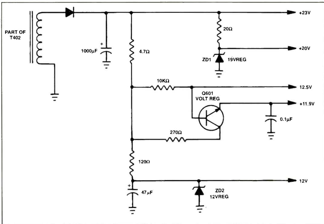
Figure 10. Check for leaky or open voltage regulator transistors and zener diodes in the defective scan-derived voltage sources.
