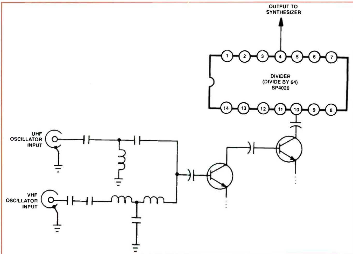
**Figure 8:** The prescaler circuit divides the frequency of the UHF or VHF oscillator by 64 before application to the PLL. This lower frequency, while still related to the original frequency, will simplify the task of the PLL.
