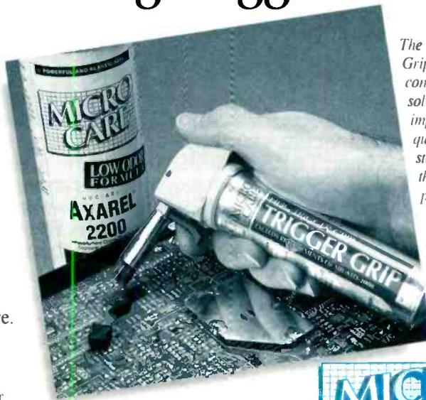
*The Trigger Grip system controls solvent use, improving quality while standardizing the cleaning process.*
