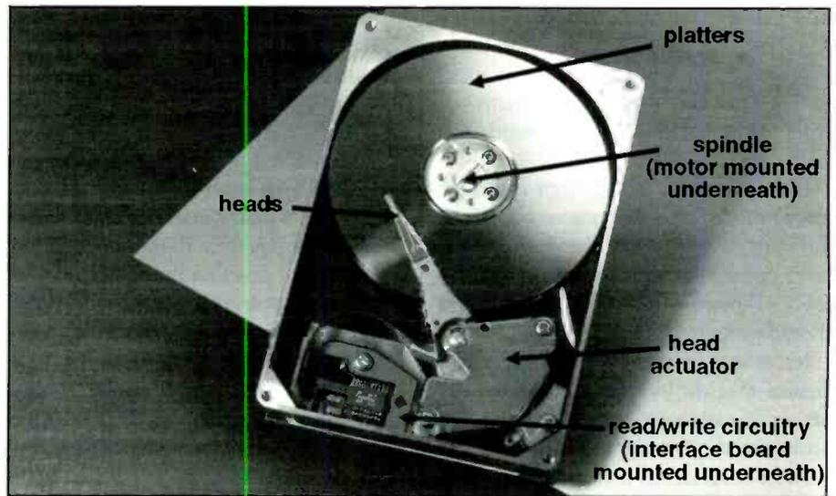
**Figure 2.** In last month’s issue we mentioned the five critical elements of a current hard drive assembly that are shown here.
