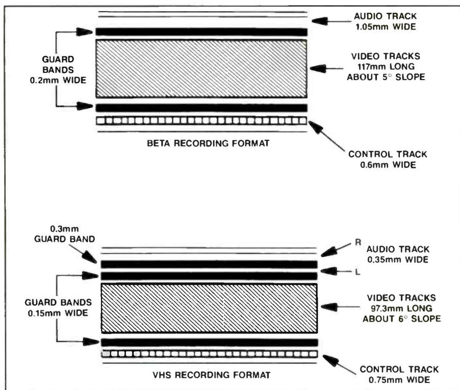
**Figure 5.** The recording scheme for VHS is similar to that of Beta, but the threading and hence the cassettes are different. Even if you put a VHS tape in a Beta cassette, or vice versa, however, it would not play.
