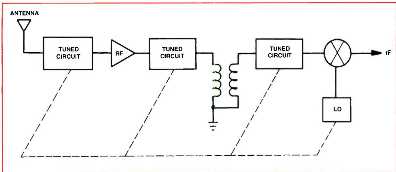
**Figure 2:** In the VHF tuner four circuits are tuned simultaneously. These circuits can be tuned mechanically by changing component values, or electronically by using varactor diodes in conjunction with a variable voltage source.
