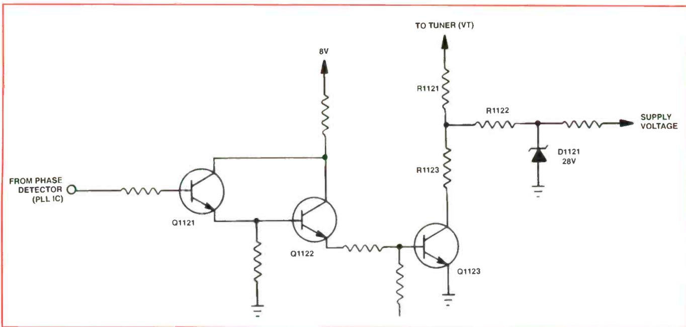
**Figure 9:** The low pass filter amplifies, filters and inverts the tune voltage from the PLL before application to the tuner. The output of the LPF is a good place to open the loop.
