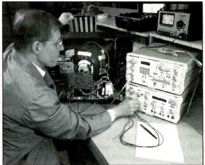
**Figure 2.** Injecting a video signal can help narrow the problem to a single defective functional block.
