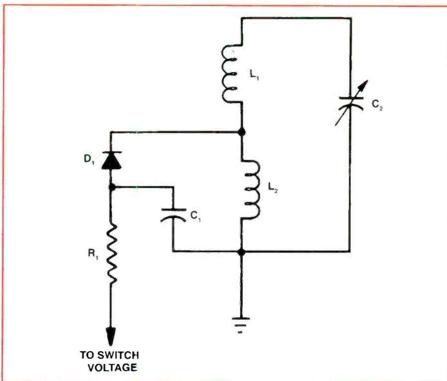
Figure 6: C1 acts as a short at the frequency of interest while isolating the switching voltage from ground. When D1 is forward biased, the lower side of L1 is pulled to ground bypassing L2. This lowers the inductance of the tuned circuit raising the resonant frequency.
