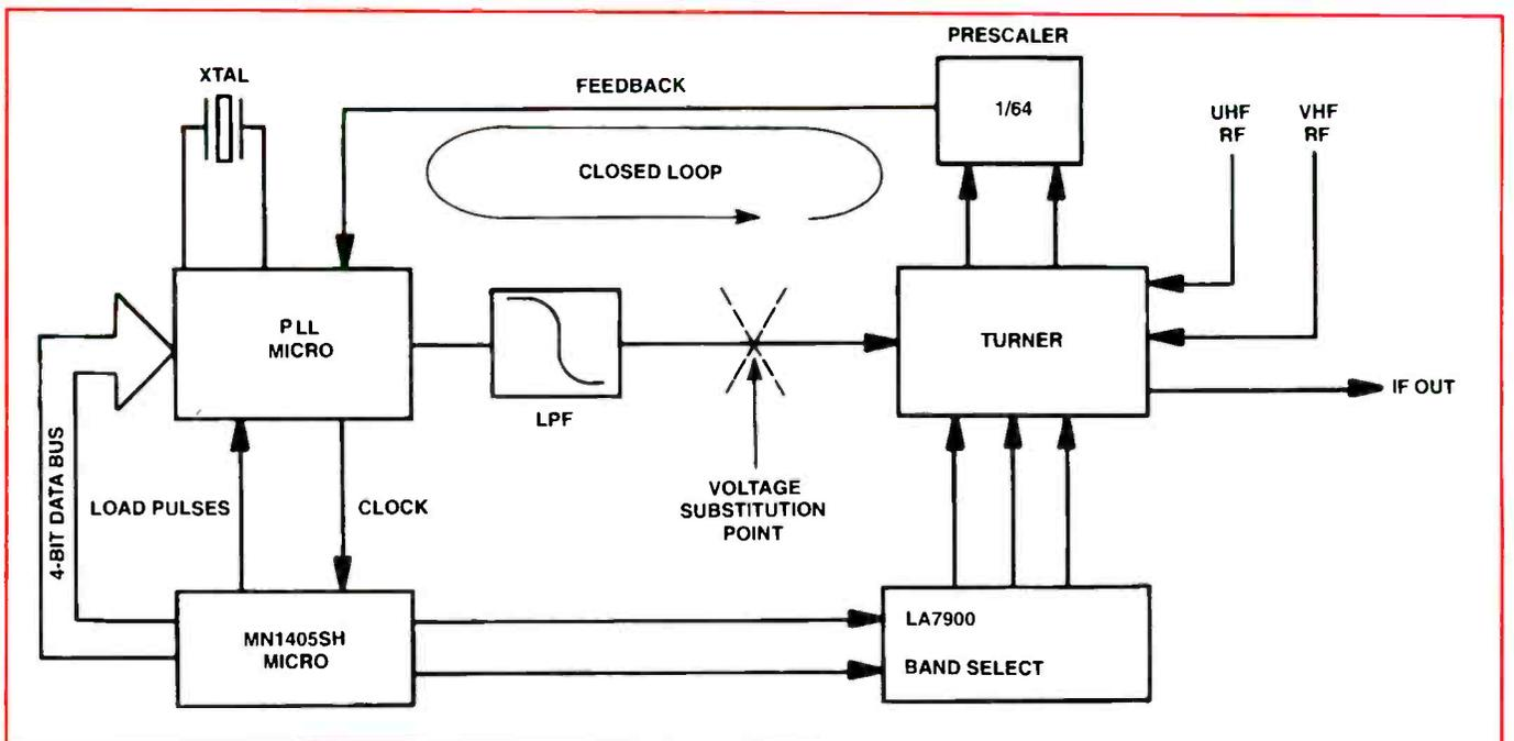
**Figure 4:** In the Sanyo Model 91C94N, all components related to voltage synthesis are located outside of the tuner.
