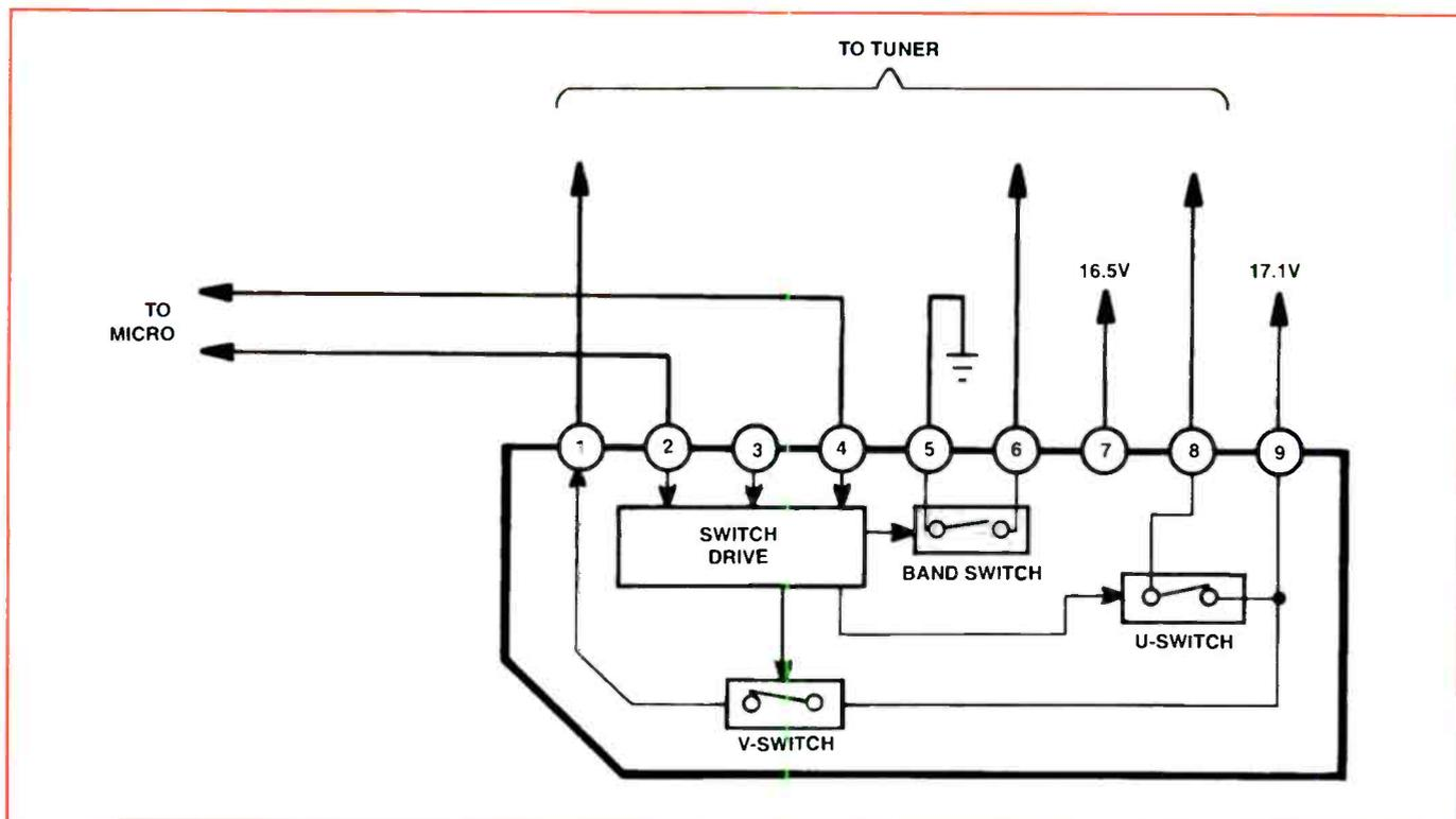
Figure 5: The band selector switch activates or deactivates sections of the tuner in response to signals from the control micro.
