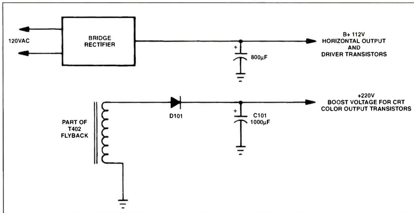
Figure 2. The boost voltage (+220V) in this circuit was taken from a secondary winding of the horizontal output transformer T402.
