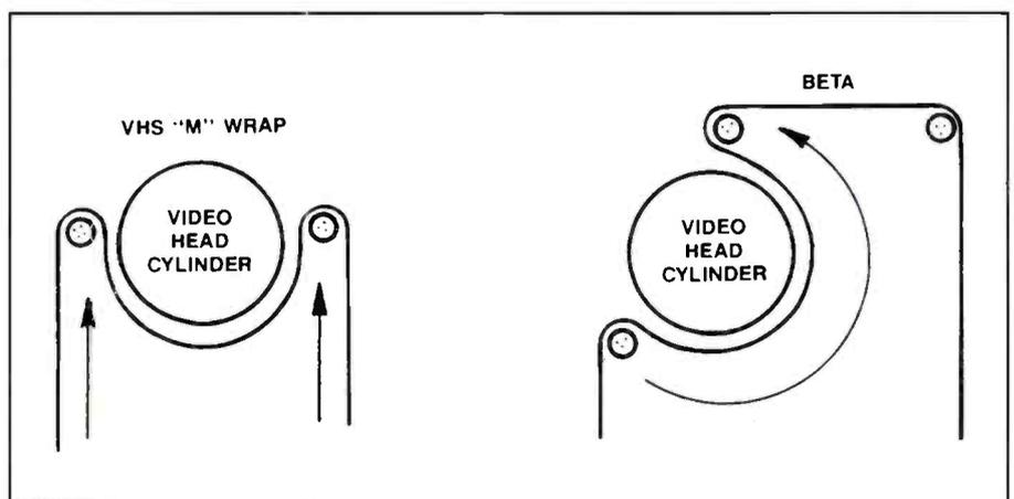
Figure 7. The tape wrap schemes are different in the VHS and in the Beta VCRs.
