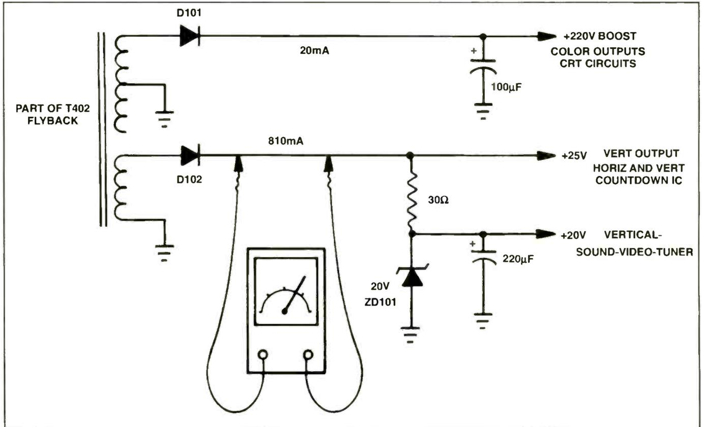
**Figure 8.** You can check to see if a circuit is causing an overload by disconnecting the positive terminal of the silicon diode that's used as a rectifier for that source and inserting a current meter in series with the output voltage source.
