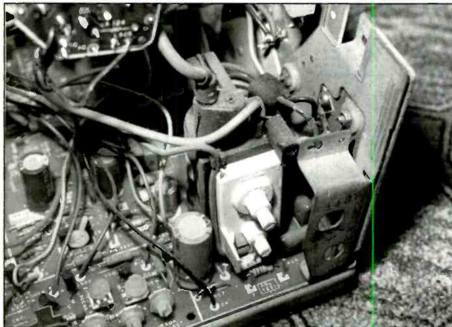
**Figure 4.** Older flybacks provided high voltage, screen and focus voltages from their secondary windings.
