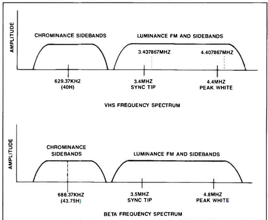
Figure 6. The VHS frequency spectrum is somewhat different from the frequency spectrum for Beta.
