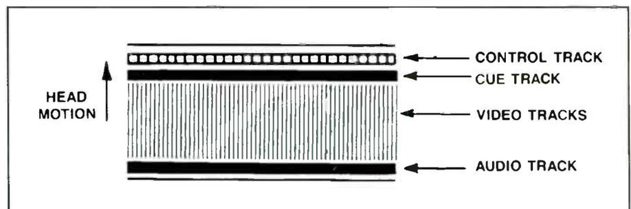
**Figure 2.** The information is recorded in this scheme in the quad videotape format.
