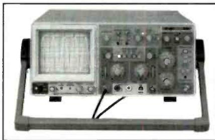
Digital readouts display the volts per division (either channel), seconds per division, and other important operating mode information such as ADD, UN-CALibrated, Probe Attenuation, MAG-nification, Delay Mode, Delay Time, Component Test, and XY Mode. Cursors can measure voltage differences, time differences, and frequency.
