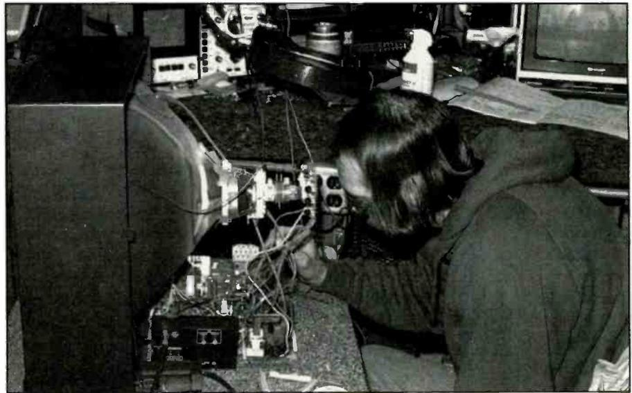
Figure 1. A technician probes a section of a printed circuit board to help locate the intermittent component
