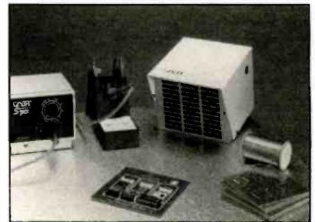
remove solder fumes and other airborne contaminants from the working environment. A powerful fan pulls the fume from the worker's breathing zone. The fumes then pass through an activated carbon filter mat to absorb the noxious gases and odors. This unit is compact in size (8" x 6" x 6") and is useful for situations where benchtop space is at a premium.
