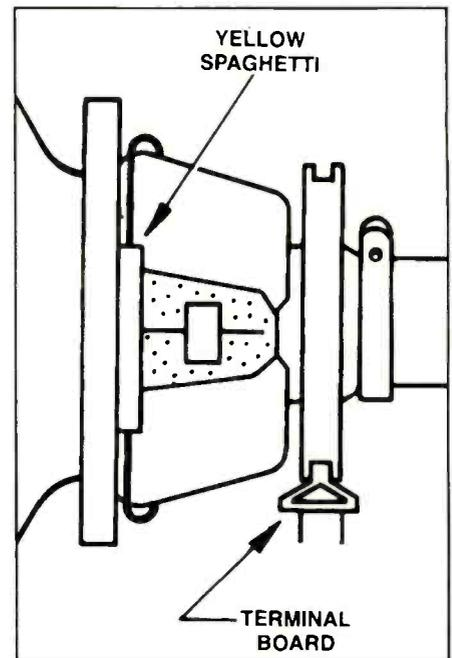
Figure 1. The vertical windings of this picture tube yoke are spliced together inside the yellow section of spaghetti.
