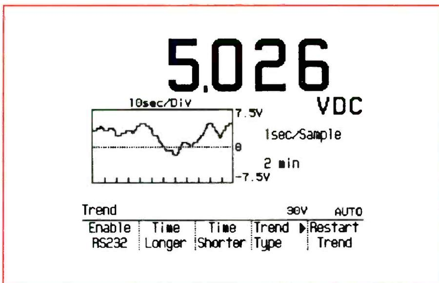
Figure 7. Graphing capabilities enable a GMM to present a documented view of collected data.
