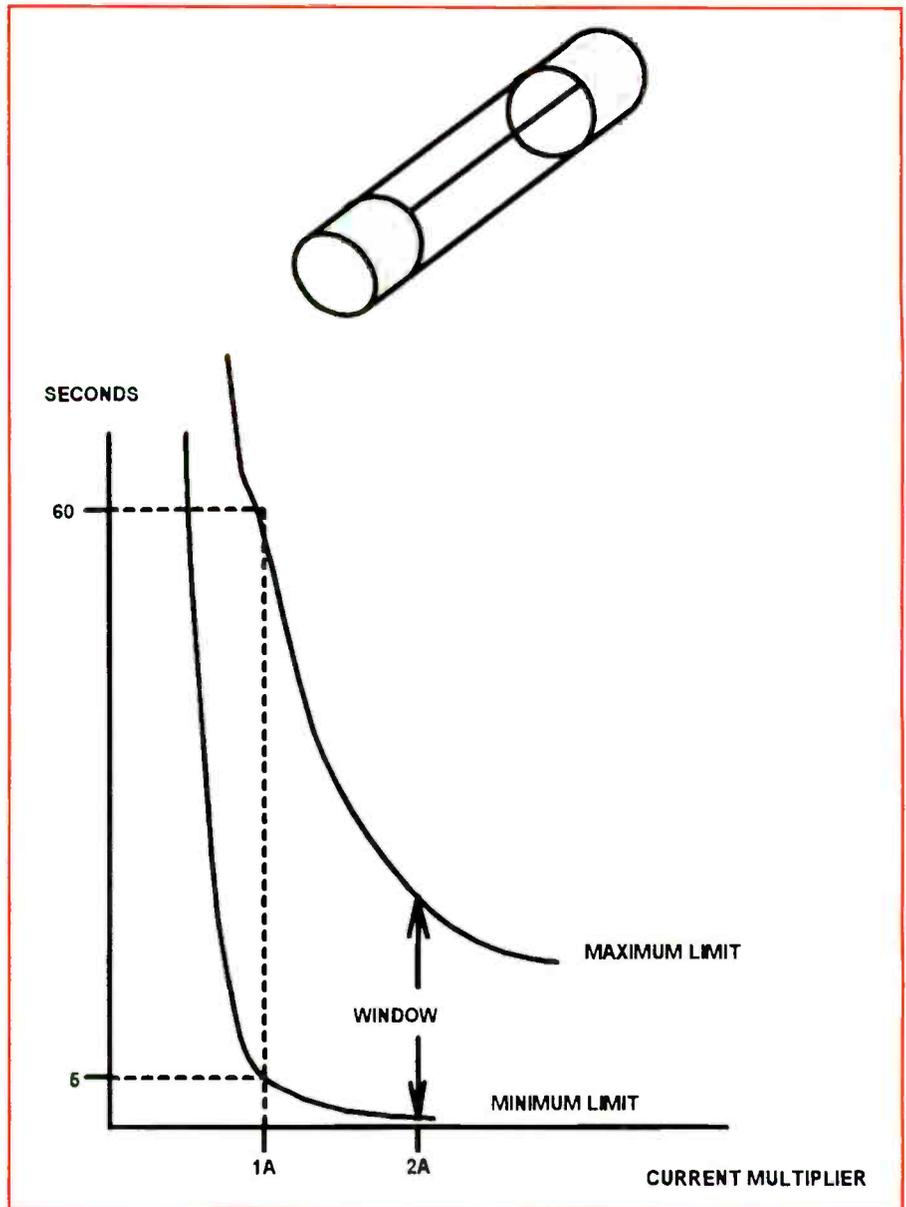
**Figure 3.** A typical 1A cartridge fuse is shown in A. A particular 1A fuse will accept 0.7A almost indefinitely, but at 1A will blow within 5 to 60 seconds. B is a curve of time-to-blow vs current. A "window" (tolerance) is allowed by the standards to compensate for the variability of the manufacturing process and other variables.
