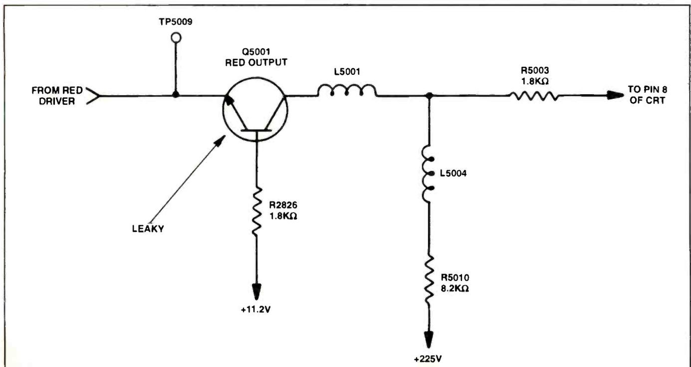
Figure 11. A leaky Q5001, red output transistor, eliminated the color red from the picture.
