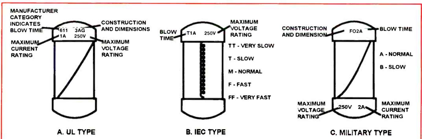
Figure 2. You may encounter different types of fuses, depending upon the type of equipment you work on. These are some of the fuse types you may run across.
