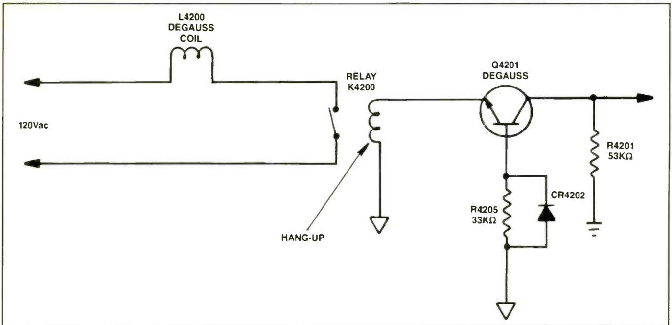
**Figure 13.** A defective or hung-up relay in the TV chassis may cause the TV set to fail to turn off, or it may keep the degaussing coil on all the time.
