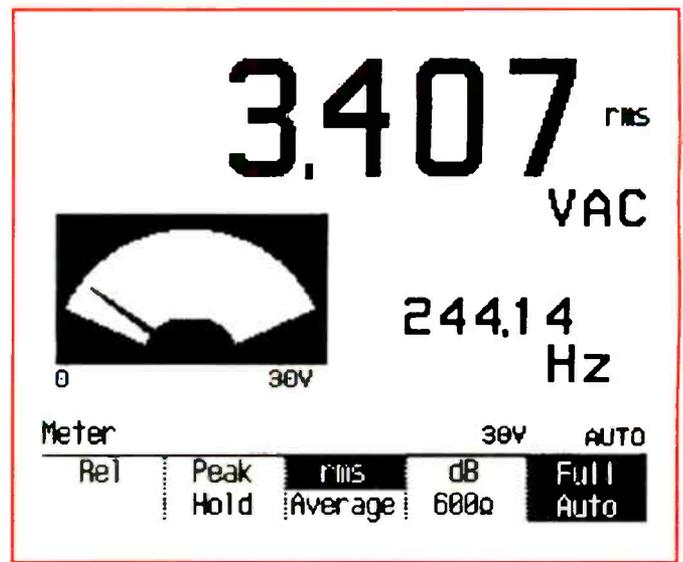
Figure 4. A numeric reading and a needle-like display combine the features of digital and analog multimeters.
