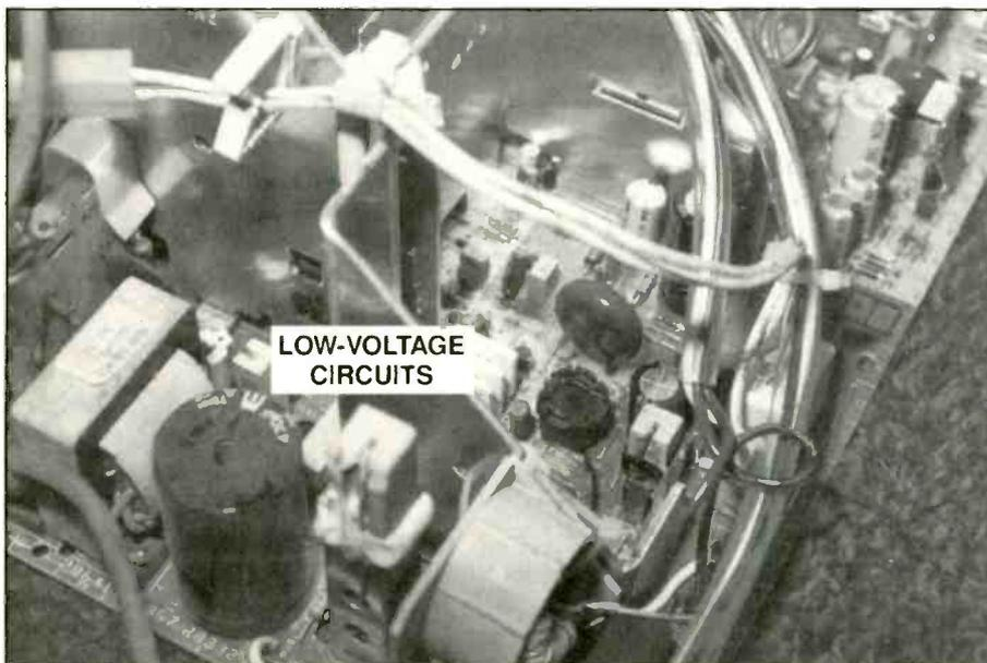
Figure 4. The low voltage circuits in an RCA CTC140 chassis are located as shown here.
