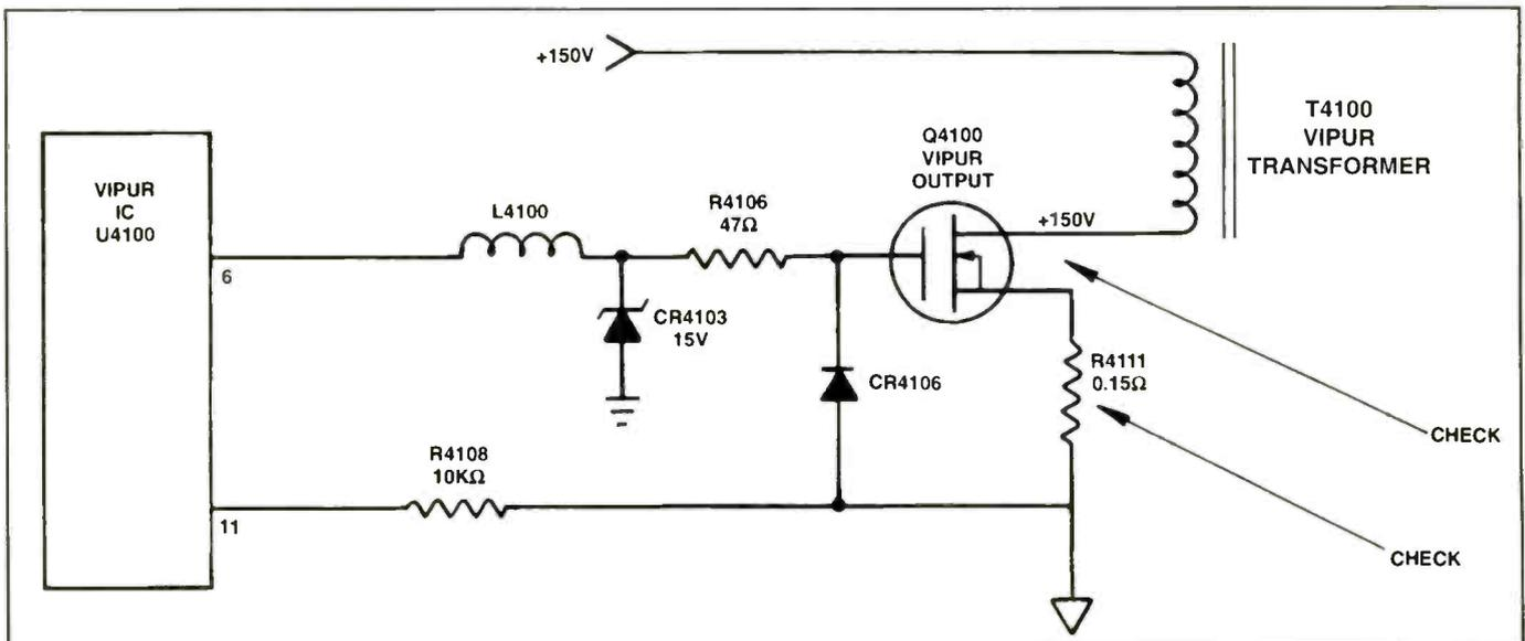
Figure 2. When replacing the VIPUR output transistor, Q4100, in an RCA CTC140, always check R4111.
