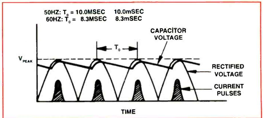
Figure 3. The filtered output of the bridge rectifier looks like this.
