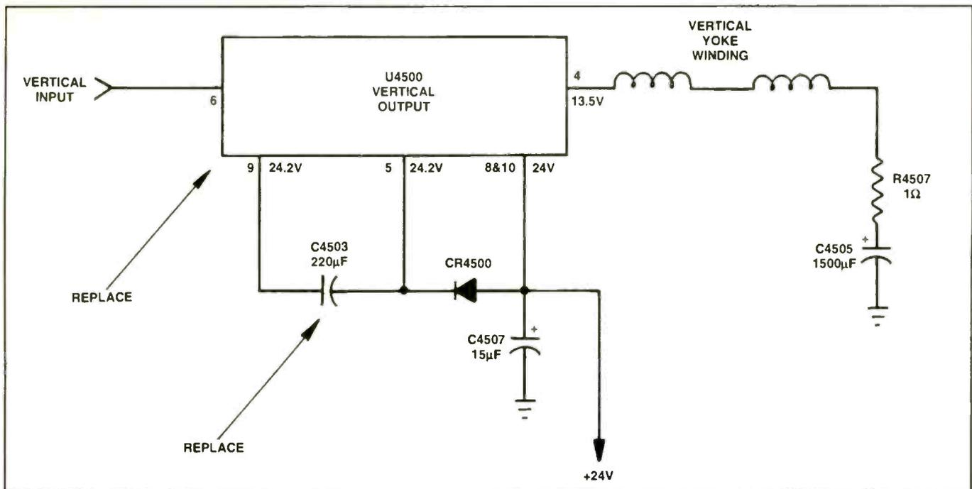
Figure 7. Intermittent vertical sweep was solved by replacing C4503 and U4500.
