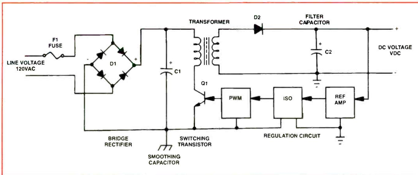
**Figure 5.** For many consumer electronic applications the flyback regulator, such as this one, is used. A diode bridge is used to rectify the 120Vac/60Hz line voltage. There is no need to use a line voltage transformer before rectification.
