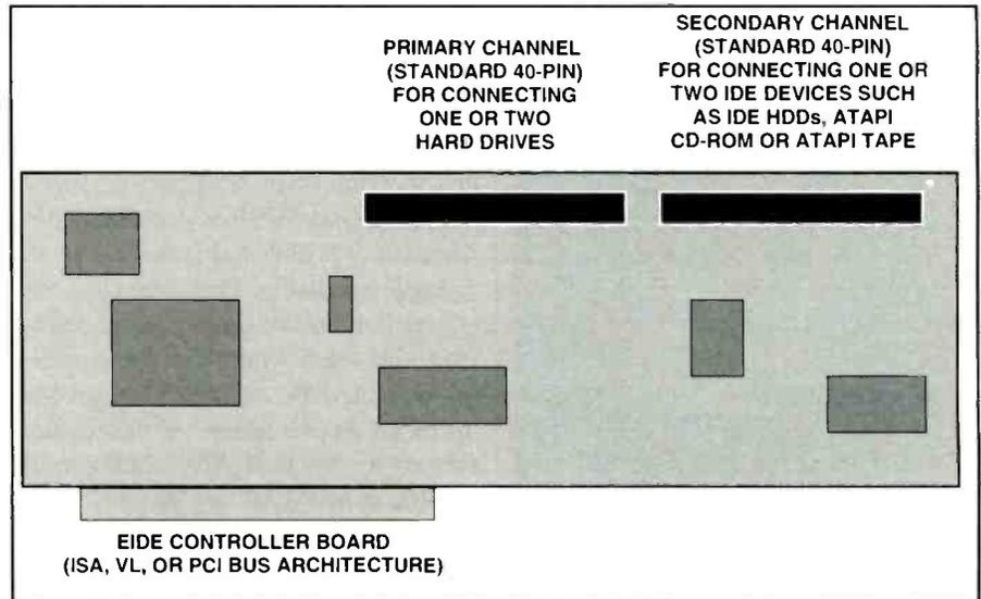
Figure 1 - IDE allows two drives (master and slave) to reside on the same port (1F0h) and Interrupt (IRQ 14), but it does not support any other devices. EIDE seeks to overcome this limitation by adding a second "channel" to the EIDE controller.
