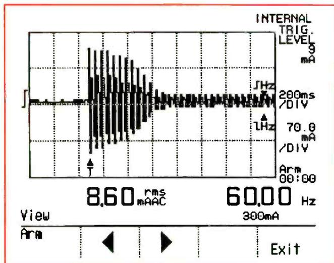
Figure 1. A comprehensive graphic view of a current waveform from an induction motor.
