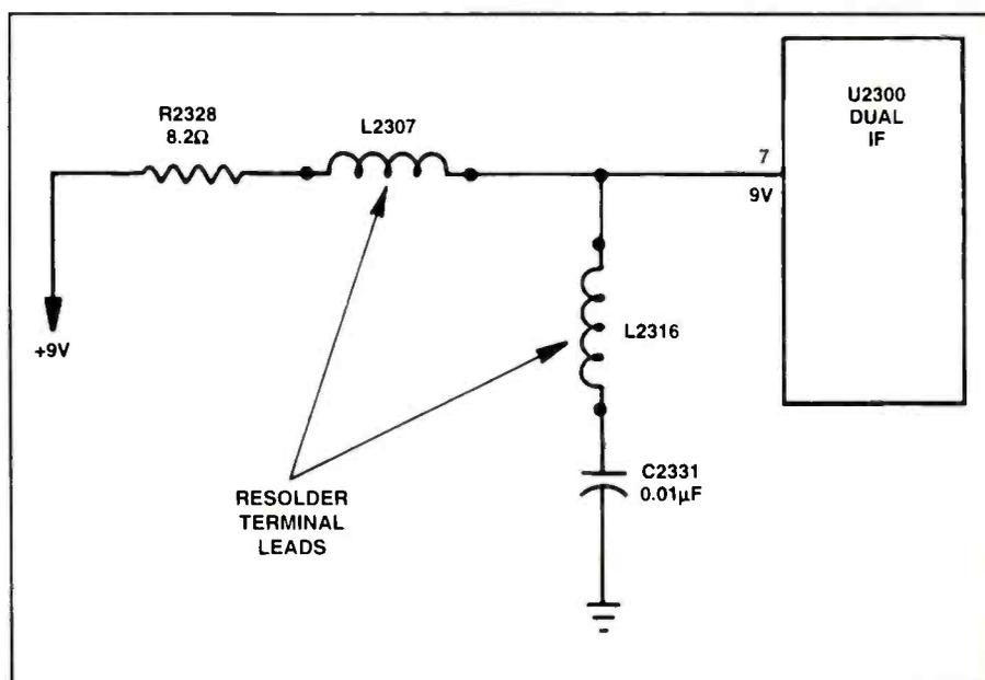
Figure 9. Poor soldered connections on L2307 caused an intermittent flashing picture.
