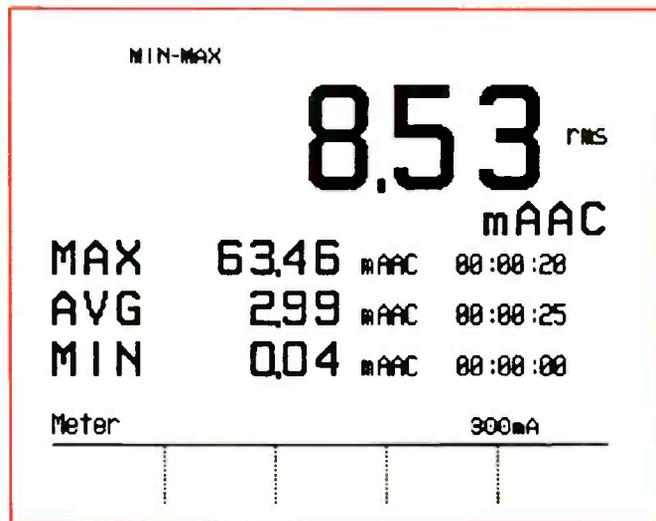
Figure 2. Minimum and maximum rms current readings from the motor.
