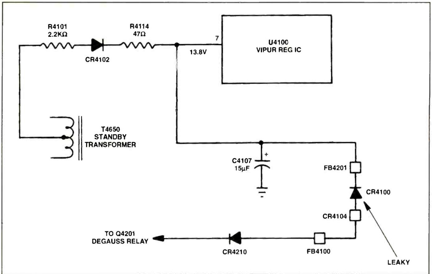
Figure 3. A leaky CR4104 produced low voltage at pin 7 of U4100, which in turn caused a dead chassis.
