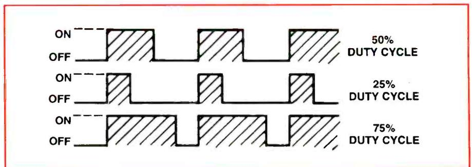
Figure 4. In pulse-width modulation, during the on cycles the pulse train energy is stored in a magnetic field. During the off cycles this energy is used to provide output power.
