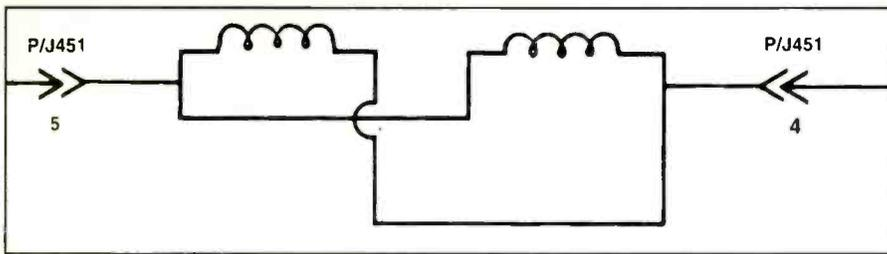
Figure 2A. The vertical windings were incorrectly shown in parallel in this diagram.
