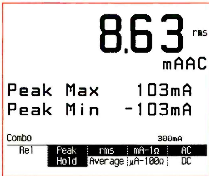
Figure 3. Peak current readings, both minimum and maximum, from the motor.
