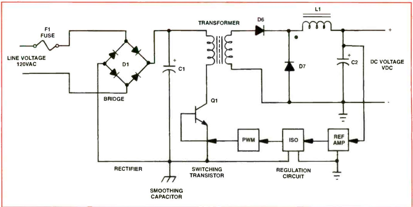
**Figure 6.** This is a forward switched mode power supply. Although the circuit looks almost like the flyback converter, there are fundamental differences in the operation. This circuit does not store a significant amount of energy in the transformer but in the output inductor.
