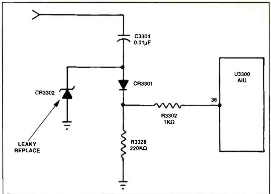
Figure 12. The remote control would not operate after several hours of operation in an RCA CTC140 chassis.
