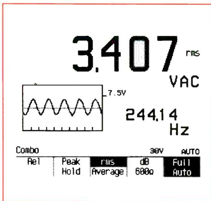
**Figure 6.** Numeric and graphical views combine the features of a multimeter and scope.
