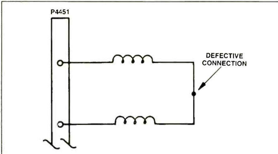
Figure 2b. The windings are in series, as shown in the PROFAX schematic.
