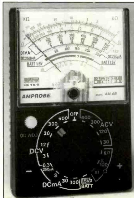
supersede the AM-6A, while providing additional functions and extended range capabilities such as: 1.5V battery test scale, dB scale; for telecommunication applications, higher input impedance (4KΩ/Volt), fuse and diode protected for misapplication up to 250V, 5μA to 300mA dc current measurement capability, 10mV to 600Vdc voltage measurement capability, dual resistance scale up to 1MΩ, and a larger mirrored display.
