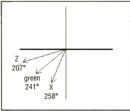
**Figure 7.** This diagram shows the phase angles of the X and Z signals relative to that of the green signal.
