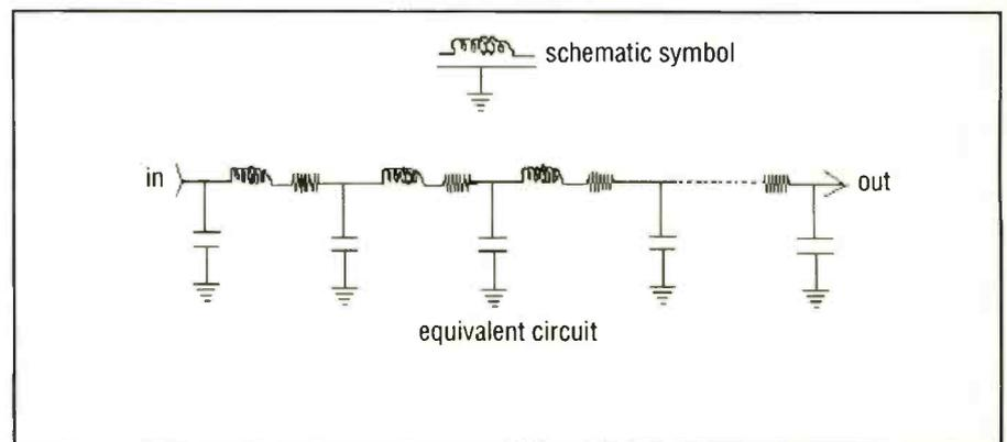
Figure 15. The video delay line is in the luminance signal path to match the delay in the color circuits. The delay is about 0.8 $\mu$ sec. It is a coil wound over an insulating tube and foil strip. The effect is like having a capacitor in parallel to ground.
