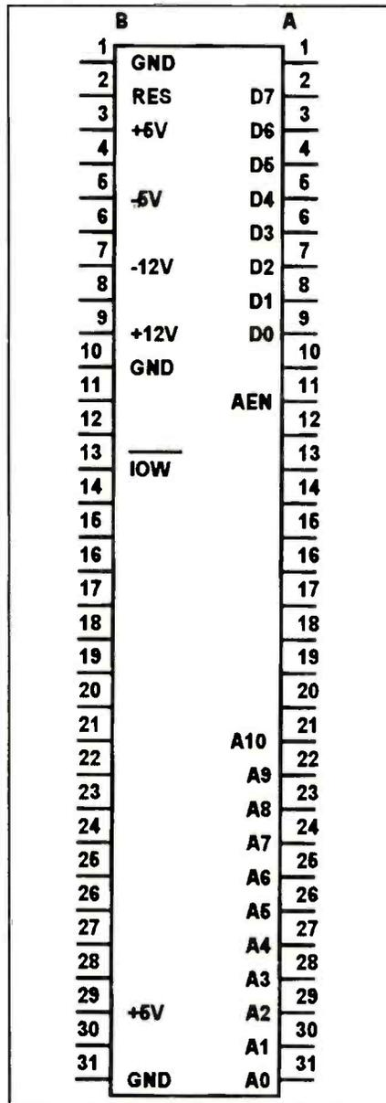
Figure 1. The expansion slot into which the POST code reader card plugs has these pin designations. Looking at the cards from the component side, the pins that plug into the motherboard are A1 to A31 starting from the rear and counting to the front of the computer. Looking at the other side, the solder side, the pins are designated B1 to B31 starting from the rear to front. The A side is used for mostly address and data pins. The other side is used for power and control pins.
