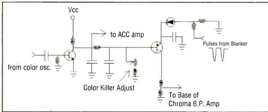
**Figure 11.** The color killer, shown here, senses the presence of the color burst, either out of the burst amp or the color oscillator. If the burst signal is not present, the circuit causes the set to produce only a monochrome picture.
