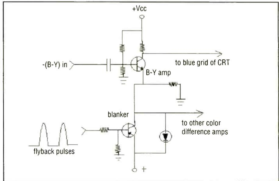
**Figure 9.** A blanker stage, such as this one provides blanking of horizontal retrace.
