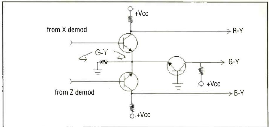
**Figure 8.** With the vectors positioned as shown in Figure 7, equal amounts of the X and Z signals produce the G-Y signal. This is a simplified diagram of the circuit that produces the G-Y signal from the X and Z signals.
