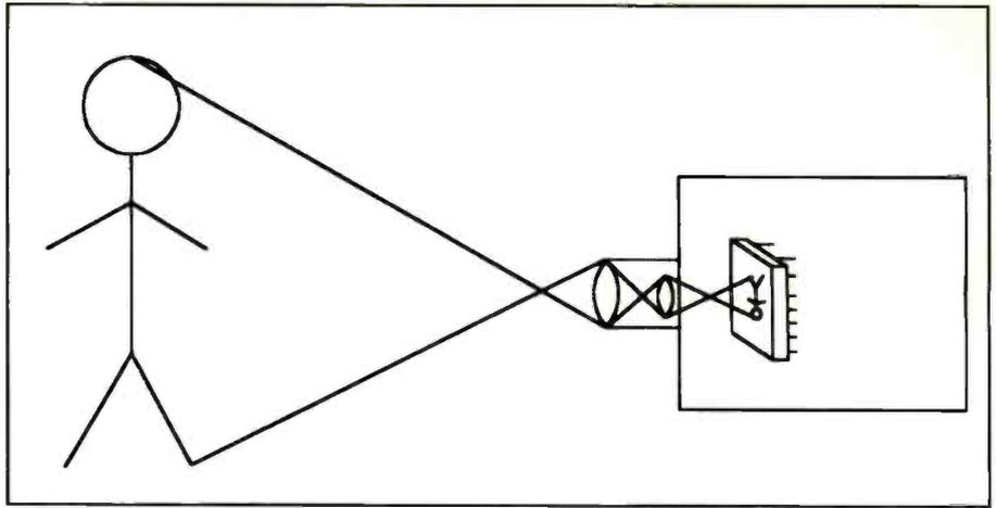
Figure 2. The lens focuses a small amount of light from the scene onto the CCD pick-up.
