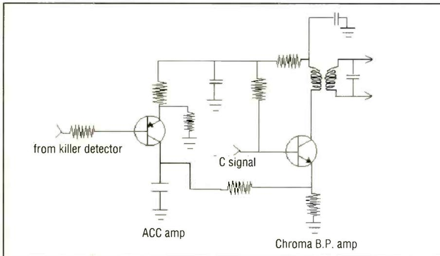
**Figure 12.** This circuit connects to the point in the circuit of Figure 11 marked "to ACC amp". It is an automatic gain control for the color signal.
