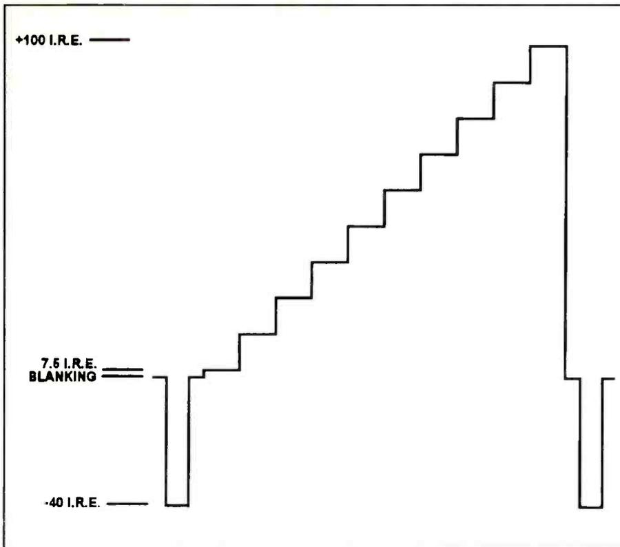
Figure 6. The IRE measurement scale is often used by camera and test equipment manufacturers to specify video and sync levels above and below the blanking reference level.
