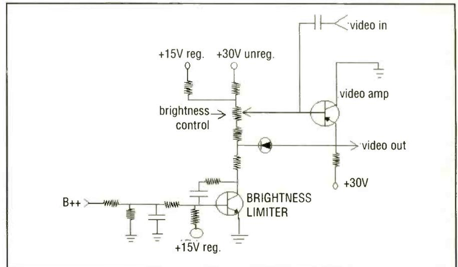
Figure 14. The automatic brightness level (ABL) circuit generally does two things: it maintains the correct brightness in spite of changes in ac line voltage, and maintains the correct levels in spite of changes in CRT anode current.
