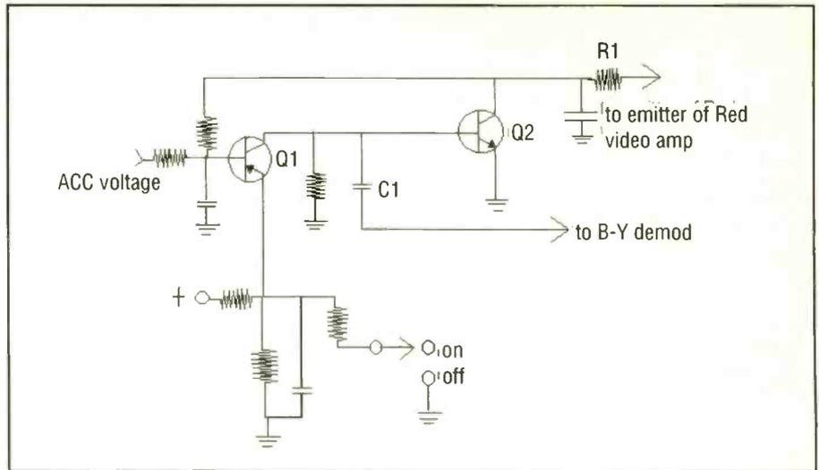
Figure 13. The automatic tint control (ATC) provides for correct picture tint.
