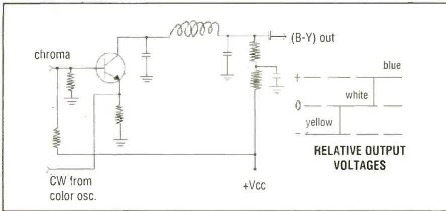
**Figure 4.** A color demodulator is a differential or additive type amplifier with the color signal at one input and the 3.58Mhz oscillator CW at the other. As the phase between the two vary, the output amplitude will vary. This is an example of a B-Y demodulator.
