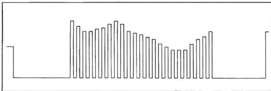
**Figure 4.** Since there are spaces between the CCD photodiodes, and the charges are digitally sampled, the CCD output signal is "choppy."
