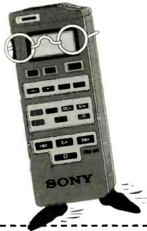
A must have for all 8mm servicers! In this video we show you less commonly used features of a very common servicing tool...the RM-95. These tips and tricks will help to speed troubleshooting and repair of your 8mm products. The tape covers the RM-95's emergency codes, forced power mode, emergency inhibit mode, individual motor operation mode, and concludes with the demonstration of a useful RM-95 modification that everyone should know about!
