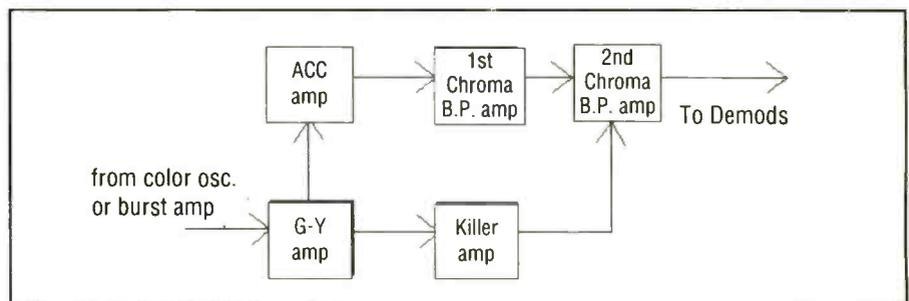
**Figure 10.** The color killer and acc circuits are related as shown here.
