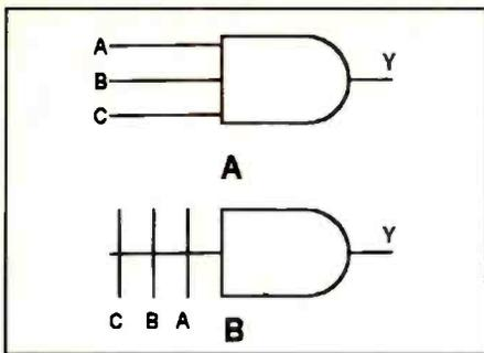
**Figure 5.** The AND logic gate in a is a standard AND logic gate. Note the difference between it and the PAL AND logic of b. In the case of the PAL AND logic gate, only one input is shown for each AND gate no matter how many inputs the AND gate may have.
