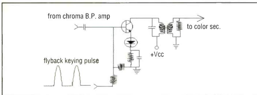
**Figure 3.** The burst amp removes and amplifies the color burst used to lock in the color oscillator. To enable it to amplify only the color burst, it is keyed on only during the blanking interval when the burst occurs.
