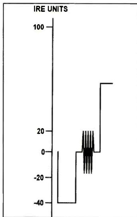
**Figure 8.** The chroma burst signal is an 8-to-10 cycle sample, just following horizontal sync, of the 3.58MHz reference signal the camera used to create the 3.58MHz chroma signals.
