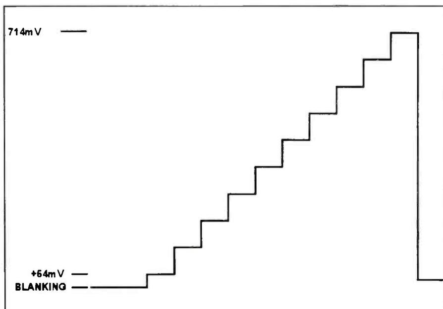
**Figure 5.** During active video time, the signal level ranges between 54mV (black) and 714mV (white).
