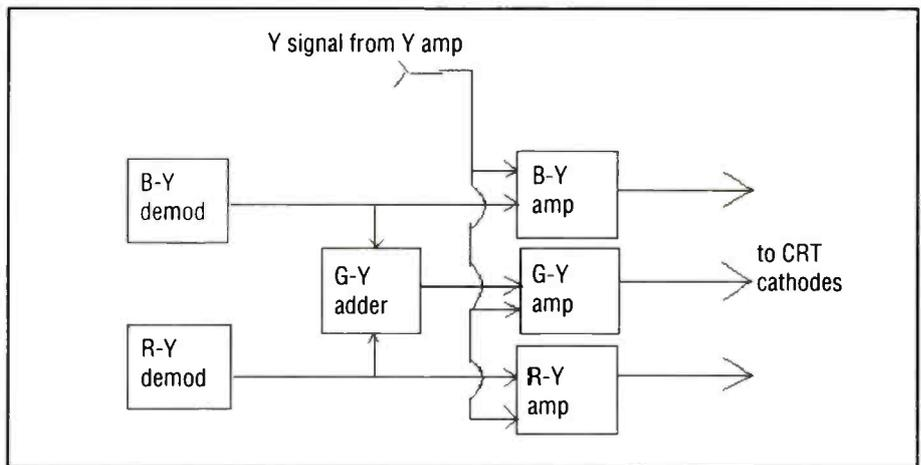
Figure 6. This illustrates a method of obtaining the G-Y signal, as well as a method of mixing the luminance (Y) component back in to the color difference signals.
