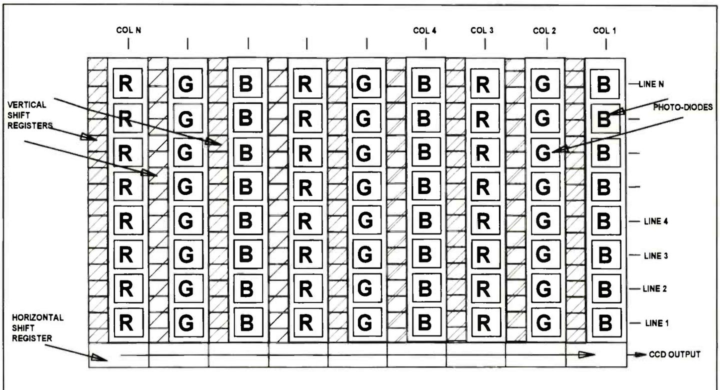
Figure 3. The vertical shift registers collect charges from the photodiodes and feed them to the common horizontal shift register to be delivered to the CCD output.
