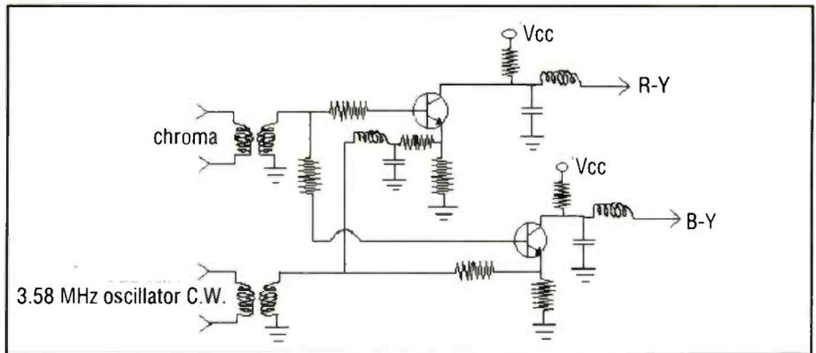
Figure 5. This is the schematic diagram of transistorized R-Y and B-Y demodulators.
