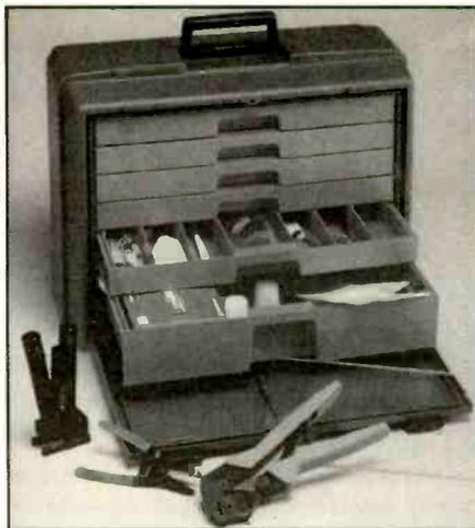
complete kit of tools to put connectors on fiber, but don't require the portability and durability of a fiber optic field service kit. The benchtop kit features a six-drawer Flambeau case with everything needed to terminate AMP's Light Crimp fiber connectors, except the connectors, polishing pucks, and epoxy.
