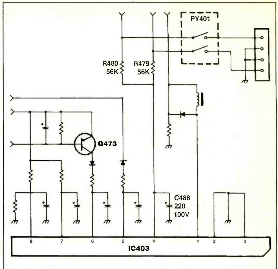
**Figure 4.** The Fisher RS-280 has an advanced protection circuit built in (IC403). If there is something wrong in the power amps the receiver shuts down through relay PY401.
