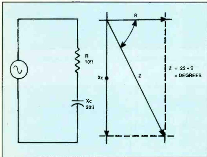
**Figure 4.** To determine the impedance of this circuit graphically, draw phasors that represent the resistance and the capacitive reactance of the components at right angles, draw the resultant impedance, and measure the length of the resultant.
