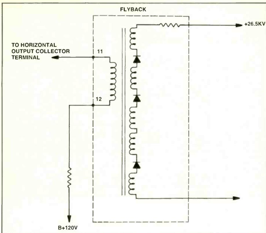
Figure 3. The secondary or high voltage winding of the horizontal output transformer will not show continuity on the highest range of meter.
