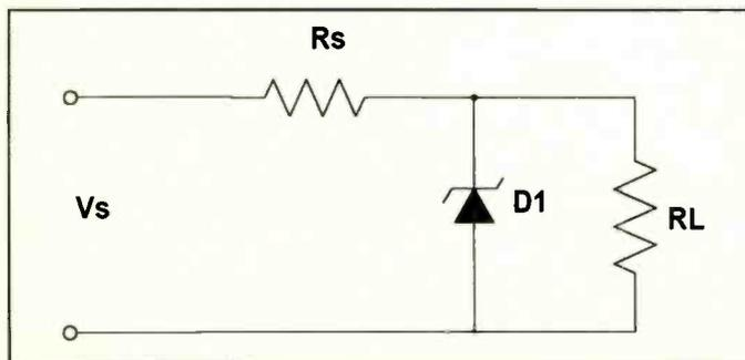
Figure 2. By connecting a Zener diode as shown here, the output voltage of the power supply can be kept relatively constant.
