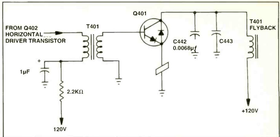
**Figure 4.** The normal horizontal output transistor with an integral damper diode will show a low resistance on the diode-transistor test using the digital multimeter and infinite resistance with reversed test leads.
