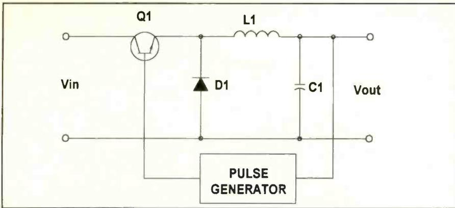
**Figure 4.** A switching power supply senses the output voltage, using it to vary the the duty cycle of a pulse generator that determines the on time of the transistor that provides energy to the output, thus keeping the output voltage relatively constant.
