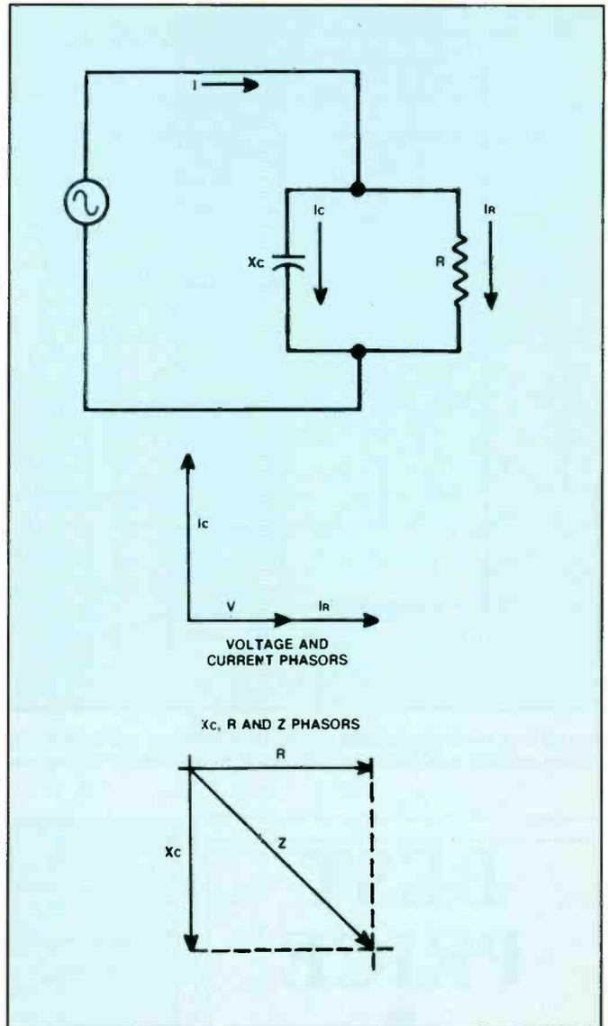
**Figure 5.** In a parallel circuit, the procedure for finding the total circuit impedance is the same as it is for the series circuit.
