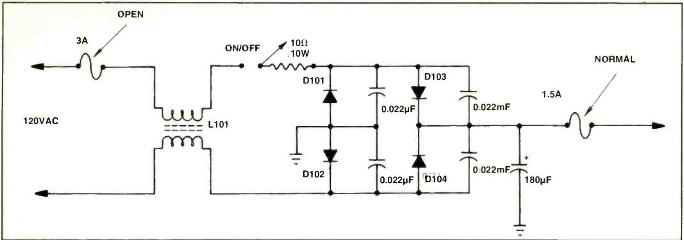
Figure 5. No leakage was found across the silicon diodes and filter capacitor in the low voltage power supply.
