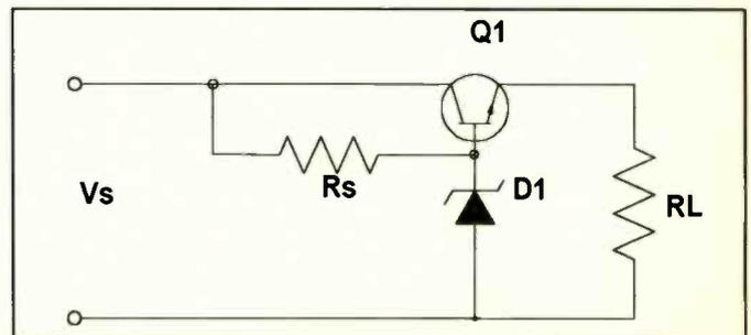
Figure 3. A transistor in the circuit, called a pass transistor because the current passes through it, improves the operation of the basic regulated linear power supply.
