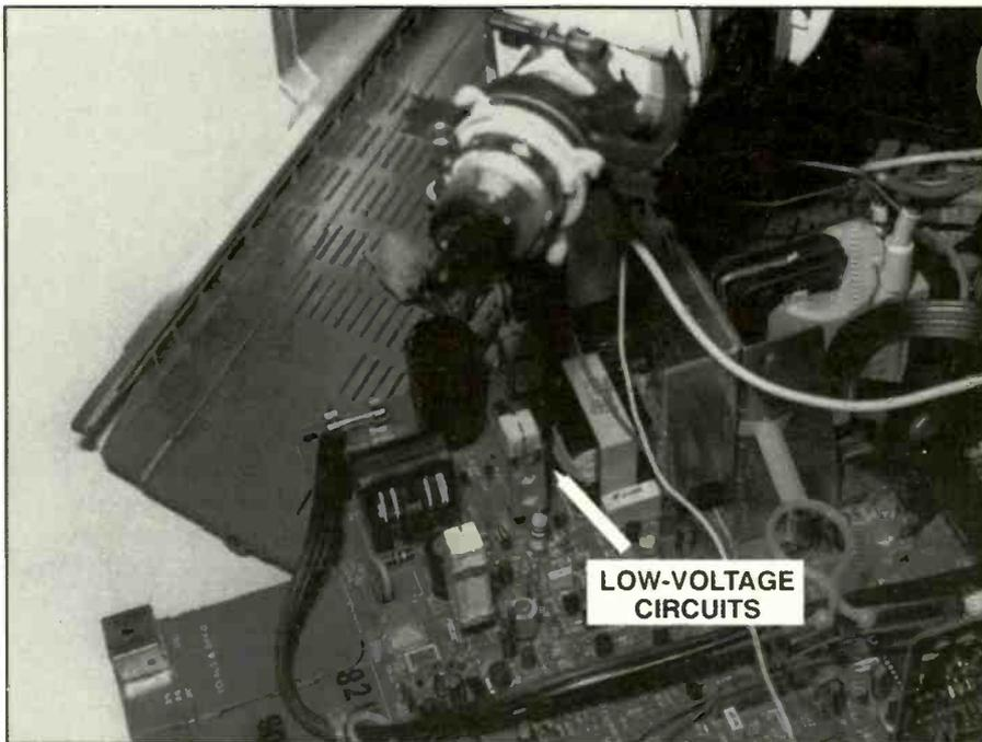
Figure 1. Shorted power line components in the low voltage power supply can cause a fire.
