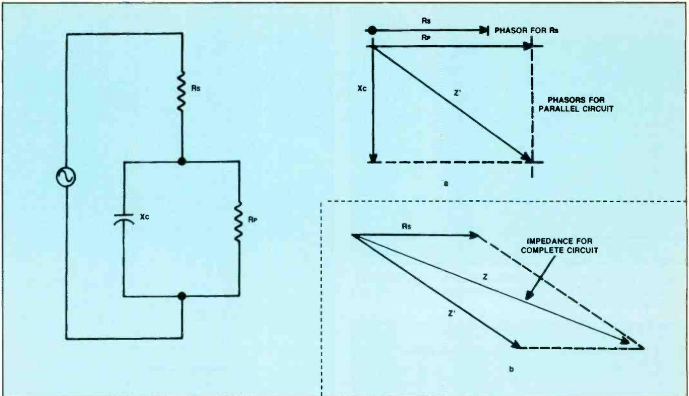
**Figure 6.** In this series-parallel circuit, the impedance can be found by first determining the impedance of the parallel circuit segment graphically, then graphically combining that calculated impedance with the resistance in series with it.
