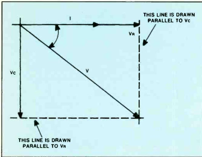
**Figure 3.** This is a different way of representing the circuit of Figure 2. Because current is the same throughout a series circuit, I is used as a reference in this phasor diagram.
