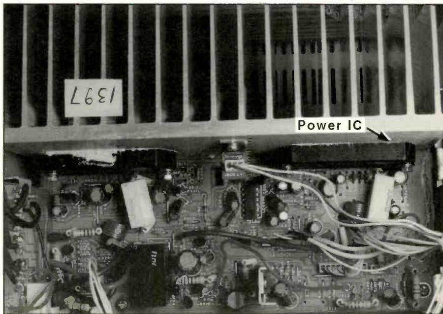
Figure 1. The power amplifier in the Sherwood S-2770RCP receiver is based on the STK4040 IC.
