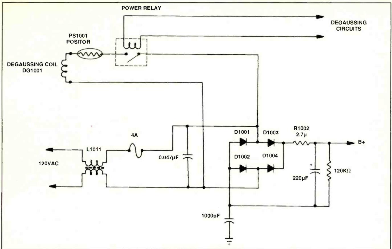
Figure 7. A power relay controlled by transistors or microprocessor closes the degaussing coil circuits to degauss the set.
