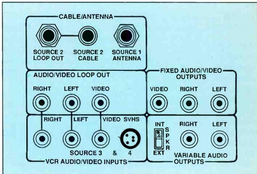
Figure 1. This jack pack has two pairs of jacks that provide audio output. The pair labeled "fixed audio," has line level audio suitable for input to an external stereo amplifier.
