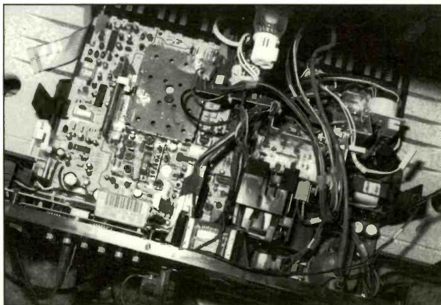
Figure 2. I checked the top of the chassis for burned spots, signs of arcing and burned components and other fire damage.
