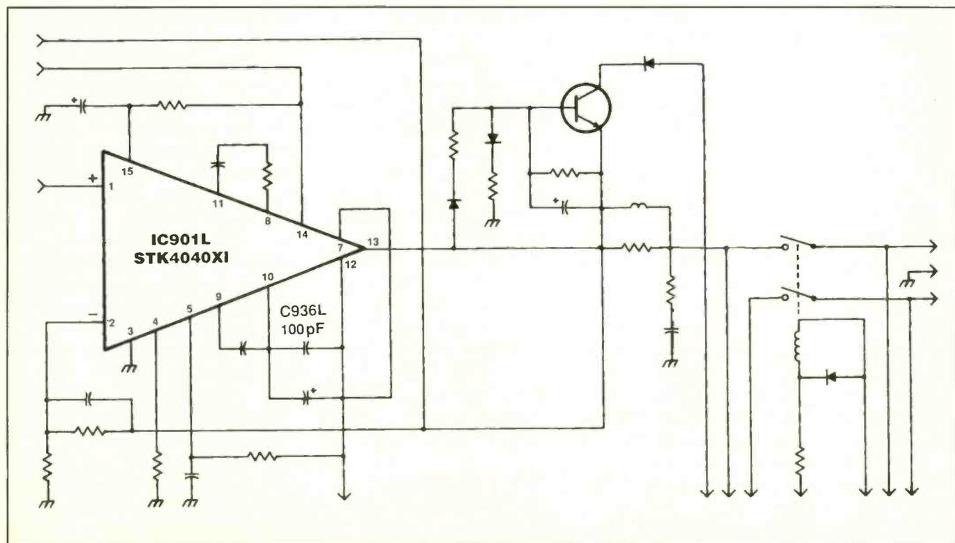
Figure 2. This is the portion of the Sherwood S-2770RCP receiver that is of interest for this service procedure. I started troubleshooting at the output (pin 13) of the STK4040.
