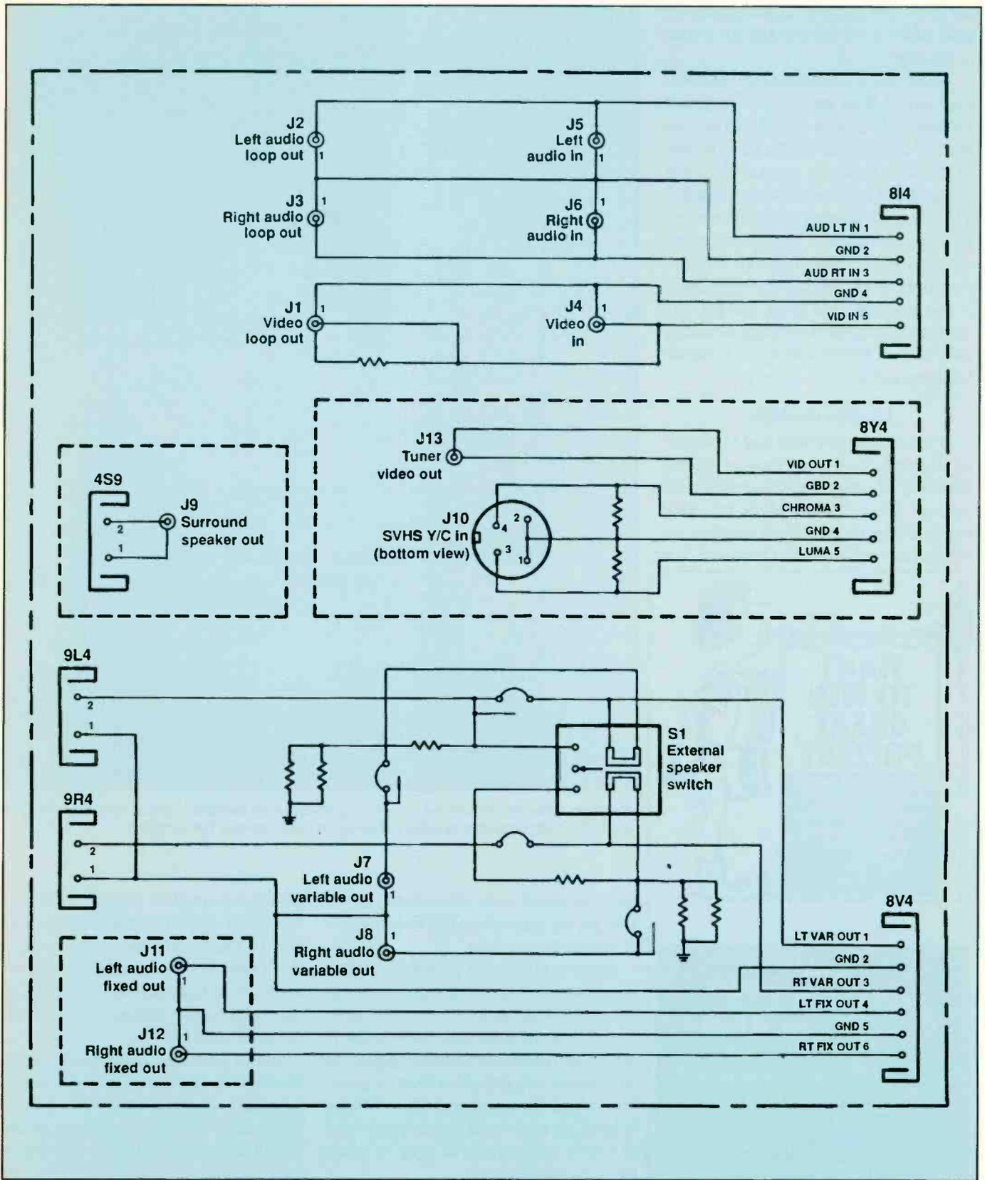
Figure 2. By connecting the speakers to the "Variable Audio" jacks, I can control the speakers volume at my chair using the TV remote control.
