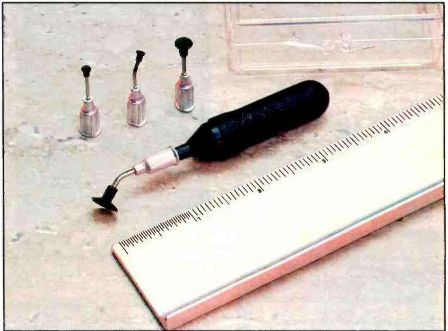
Photo 1. Tiny parts, such as surface mount components, may require special handling devices, such as this vacuum-operated handling tool. (Photo courtesy Virtual Industries)
