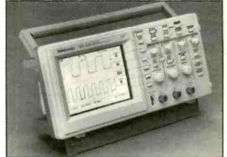
The new scopes rely on digital real-time (DRT) oversampling technology to provide high waveform quality, update rate, and stability. Both models sample at 1 GS/s, at least 10 times their bandwidth. This advanced high-speed technology enables users to capture signal details invisible on analog scopes.
