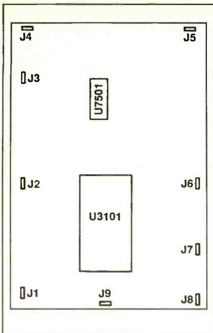
**Figure 3.** Loose connections between the tuner, microprocessor shields and the printed circuit board in the RCA CTC175/177 may cause no startup, snowy picture, loss of vertical deflection, no audio, and phantom front panel control operation, to name the most common problems. If you encounter any of these symptoms, remove the old solder, carefully inspect the circuit board for cracks, and resolder.
