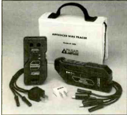
The transmitter can be directly connected to deenergized lines to search for opens or shorts or directly connected to energized lines to identify breakers and circuit paths. The receiver contains two user selected detectors for "Open" or "Current" tracing for a transmitter to re-
