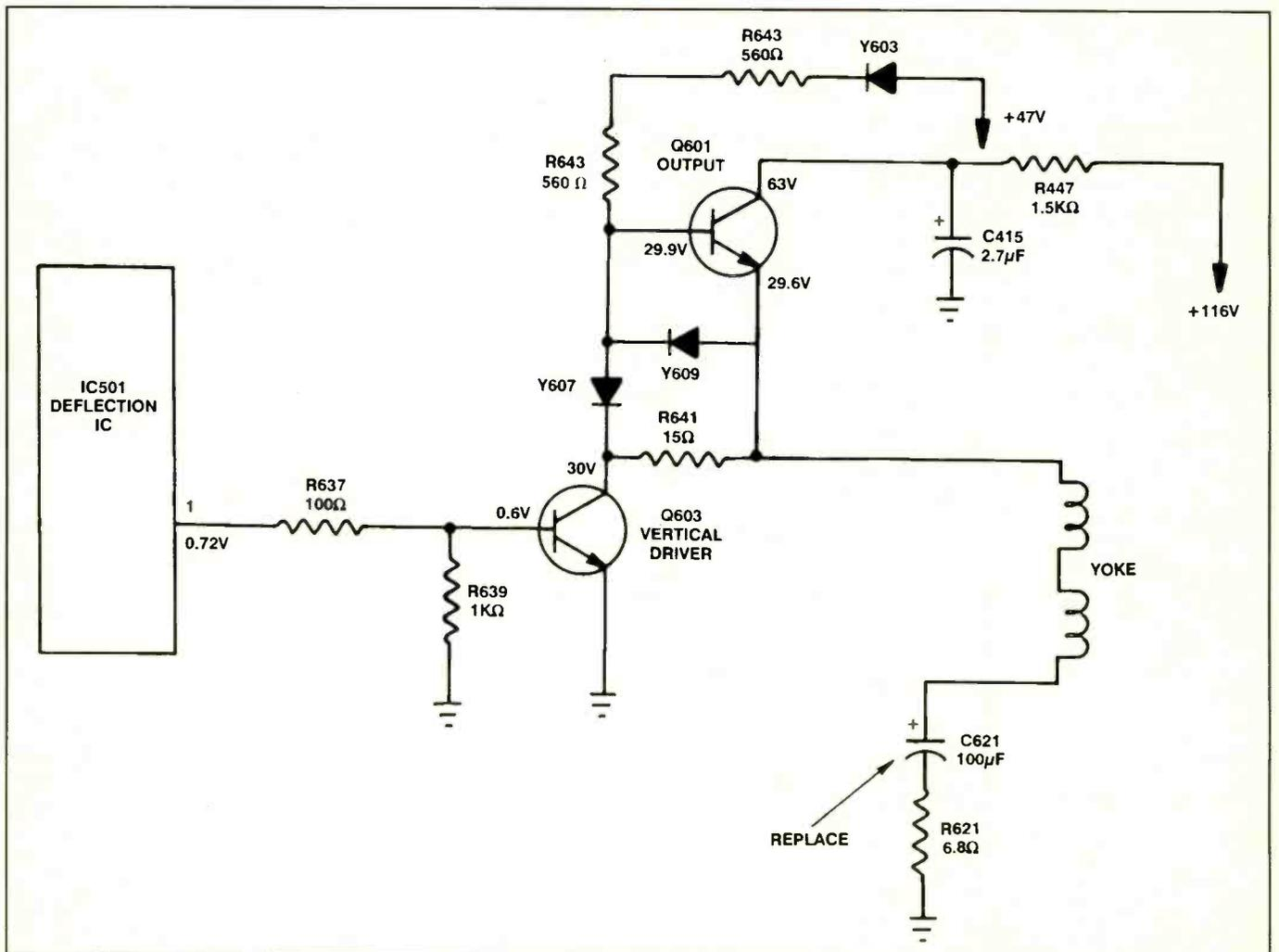
**Figure 10.** There was only one-half-inch of a folded over picture in the center of a GE 19PC-F chassis. The cause of this symptom was traced to a defective capacitor, C421.
