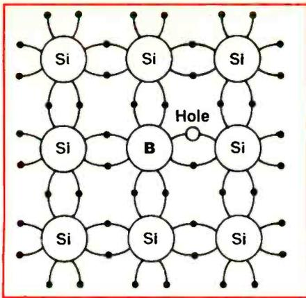
Figure 4. The addition of acceptor impurities renders a p-type crystal with an excess of holes, which improve conduction characteristics.
