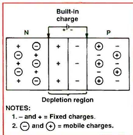
Figure 5. The joining of p-type and n-type crystals forms a p-n junction or diode.
