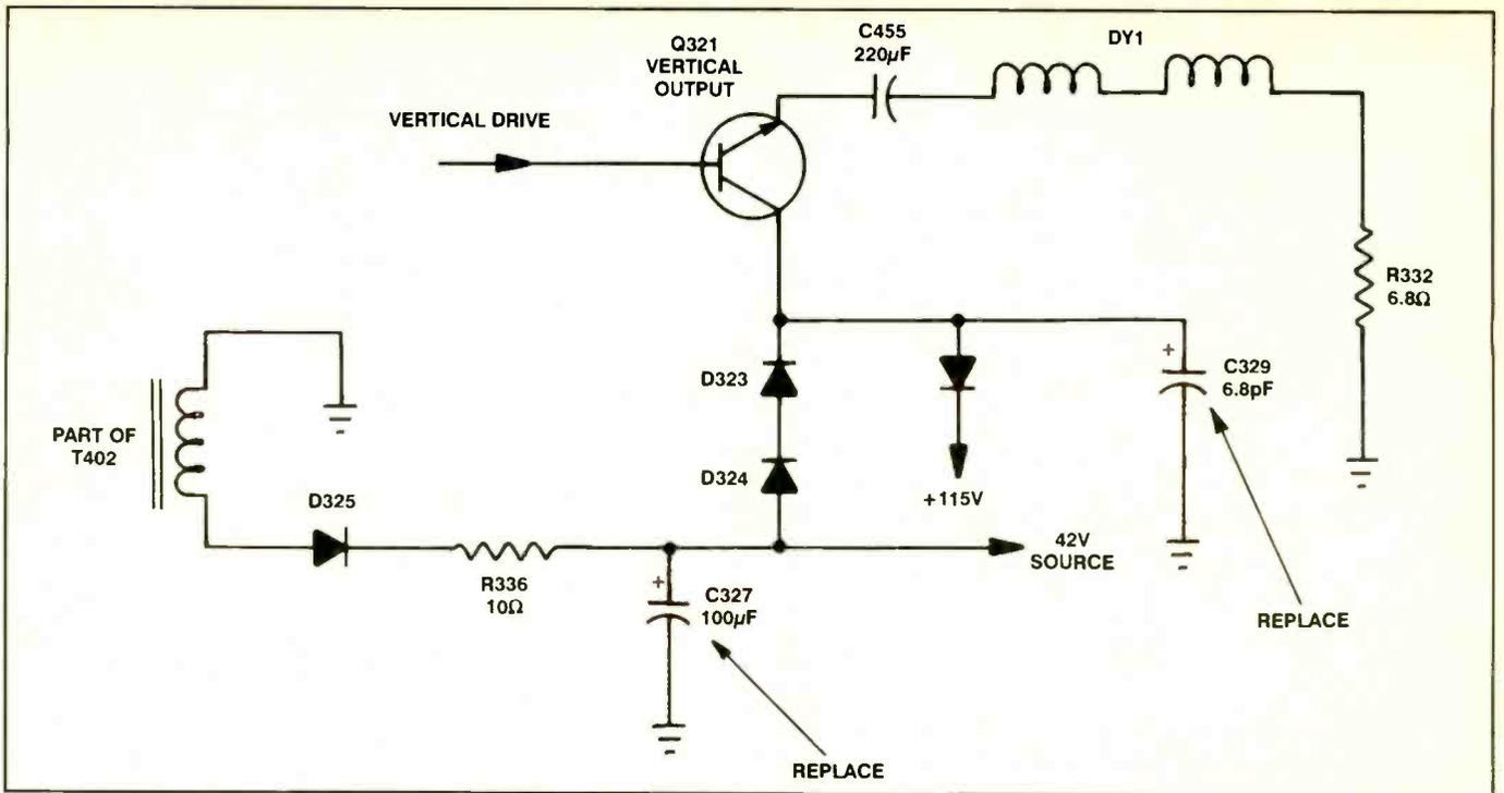
**Figure 9.** A black area at the top and bottom of the screen was caused by a defective C327 in the low voltage supply of a Goldstar CMR-4160 television set.
