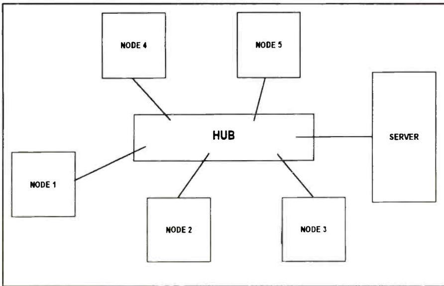
**Figure 4.** A network based on the star topology passes all data to each device through a centrally-located device called a hub. A star network offers easy installation and management. The drawback of a star network stems from the potential of data arriving at the hub simultaneously.
