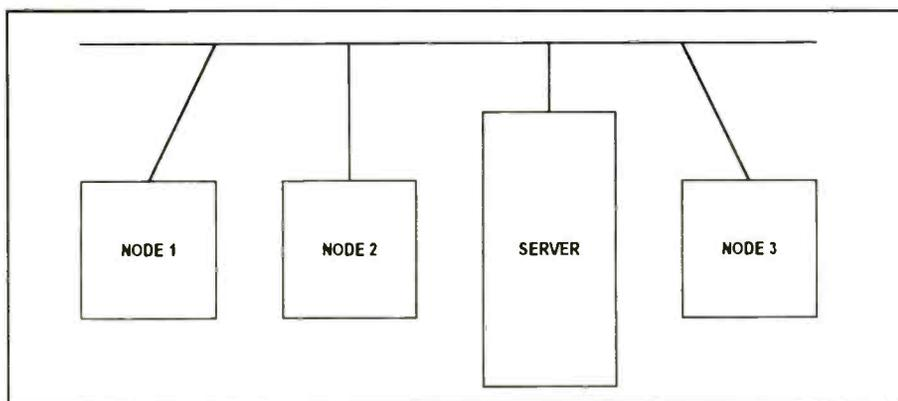
Figure 2. A bus network provides an inexpensive, easily installed, network option.
