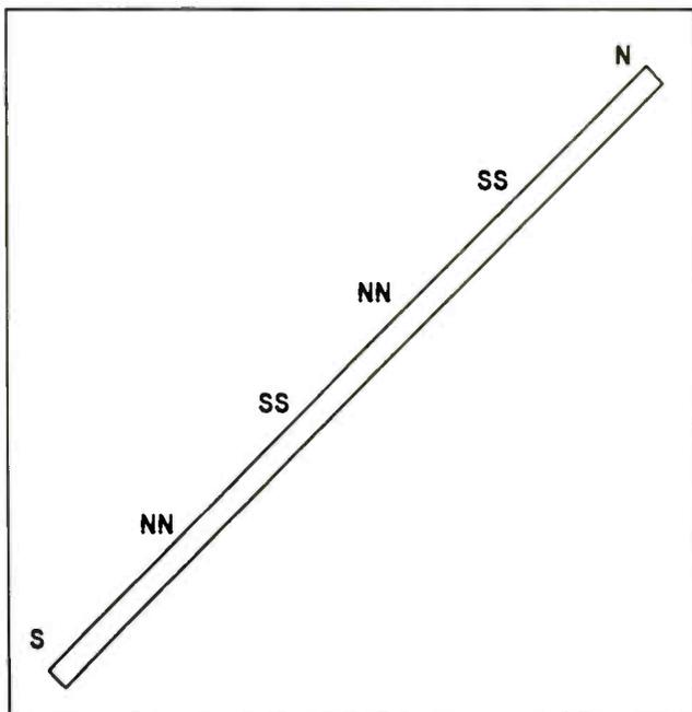
← **Figure 2.** If you try to create the equivalent of a unit north pole by magnetizing a long iron rod, you will wind up creating a number of what are so-called consequent poles along the length of the rod.
