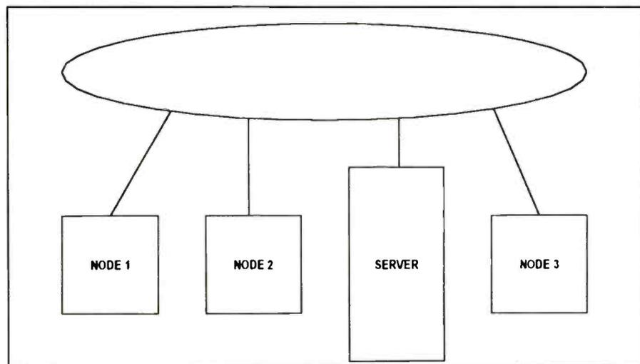
Figure 3. In a ring network, one device connects directly to two other devices, thus offering reliability in that the failure of one device usually does not affect the performance of other devices. However, the ring network is the most difficult to install and the most expensive of the three network topologies.
