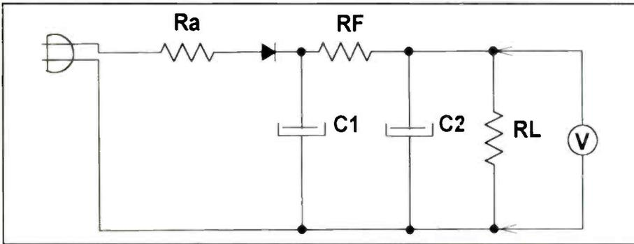
**Figure 1.** What is resistor Ra in this circuit called? And what will the meter indicate if capacitor C2 becomes open-circuited?
