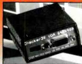
Looking for a SMALL battery operated monitor test pattern generator that will fit in your pocket? The Checker Jr. is it. It displays a very useful 64 color pattern. You can evaluate size, focus, linearity, color tracking, and balance. It operates in the 640 x 480 mode (31.5KHz x 60Hz.), and is very easy to use. Use it anywhere.
