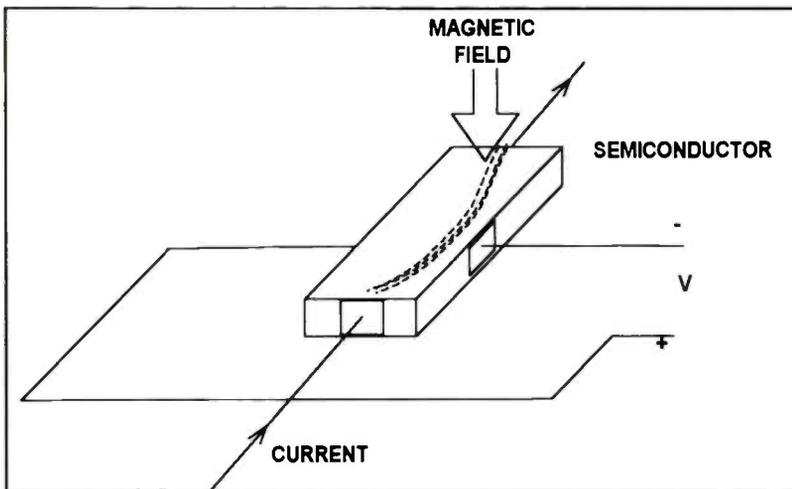
**Figure 4.** To measure the strength of a magnetic field you can use a Hall device. The magnetic field cuts through a small semiconductor slab. In a Hall device, electrons crowd to one side of that slab and create a voltage. The magnitude of the voltage is proportional to the strength of the magnetic field.
