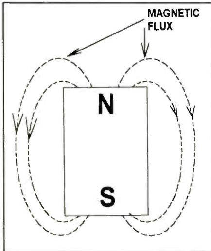
**Figure 1.** The flux lines surrounding this magnet show the direction in which a unit north pole (an imaginary construct) would move under the influence of the magnetic field.
