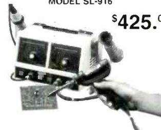
Top of the line repair system will handle desoldering Temperature controlled soldering from 300°F to 790°F (150°C to 420°C), desoldering temperature range 410°F to 900°F (210°C to 480°C).
