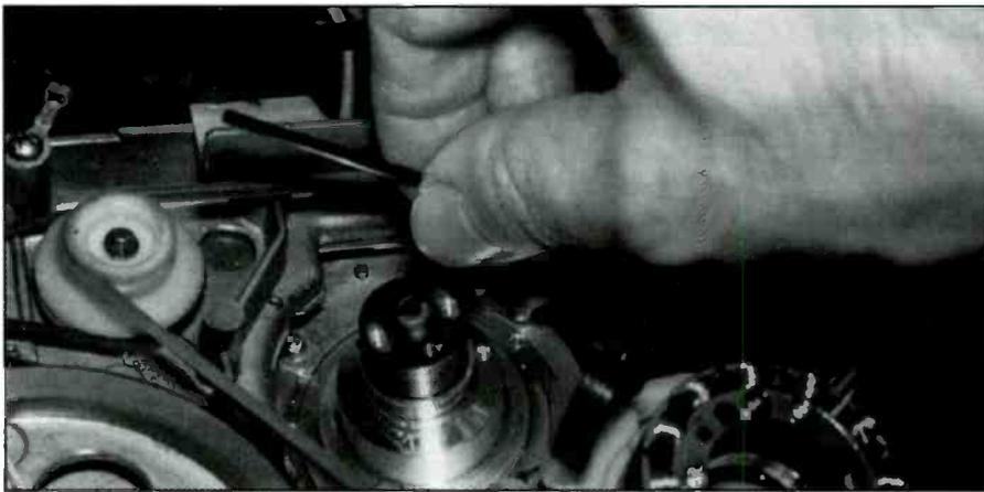
Figure 7. Loosening the shaft collar at the bottom of a VCR cylinder motor.
