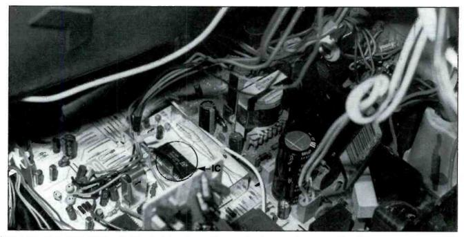
Figure 2. The stereo microcontroller, multiplex decoder, and multiplex demodulator in one of these sets might be included in a single largeIC.
