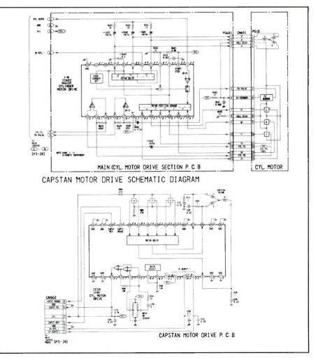
**Figure 9.** Called a mode motor in some camcorder designs, the capstan motor establishes the tape movement in the play, record, rewind, fast forward, and search modes. Typically, the motor will drive mechanical assemblies through either gear or belt-driven mechanisms. The circuits that provide the drive signals for the capstan motor are found in this circuit, and the capstan motor drive section of the main circuit board.
