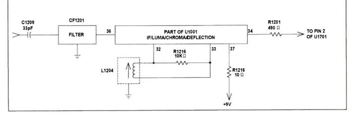
Figure 5. CF1201, L1204, and U1001 can all be causes of hum and buzzing noises in the RCA CTC166, and CTC167 chassis.
