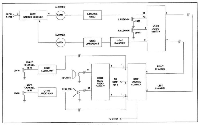
Figure 1. A block diagram of the stereo circuits in the RCA CTC166 television chassis.
