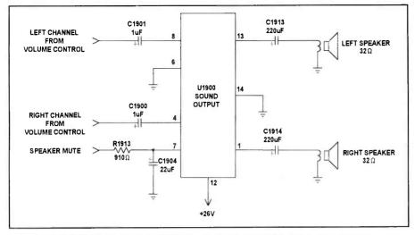
Figure 4. The dual sound output IC (U1900) can cause many different audio problems.
