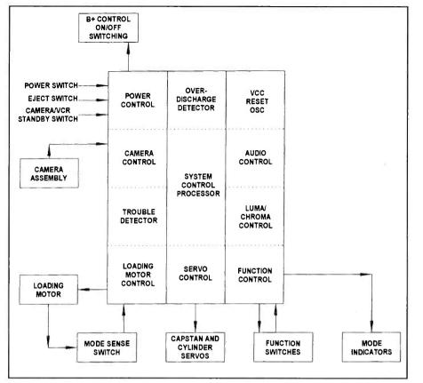
**Figure 7.** As shown in this block diagram, different parts of the control processor maintain the functions of the VCR and camera assemblies. With the VCR portion of the control system, the loading motor control area drives the motor and circuitry that engages levers and gears that control the mechanical operation of the video cassette recorder.
