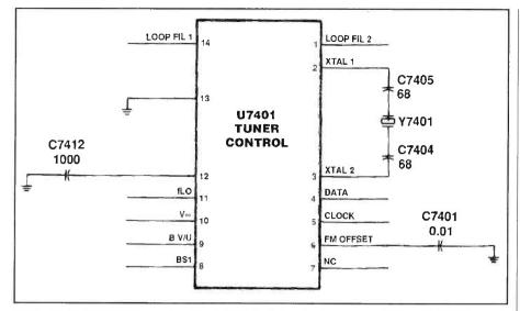
Figure 2. Crystal Y7401 develops the reference signal for the tuner controller IC, IC7401. Look for a 4MHz signal at about  $1V_{PP}$ . A defective crystal will cause one of two problems: a completely dead tuner or one that drifts off frequency.
