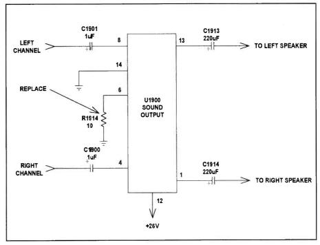
Figure 9. After replacing integrated circuit U1900 to cure extreme audio distortion, check R1914 to see if it is open or burned or otherwide damaged.
