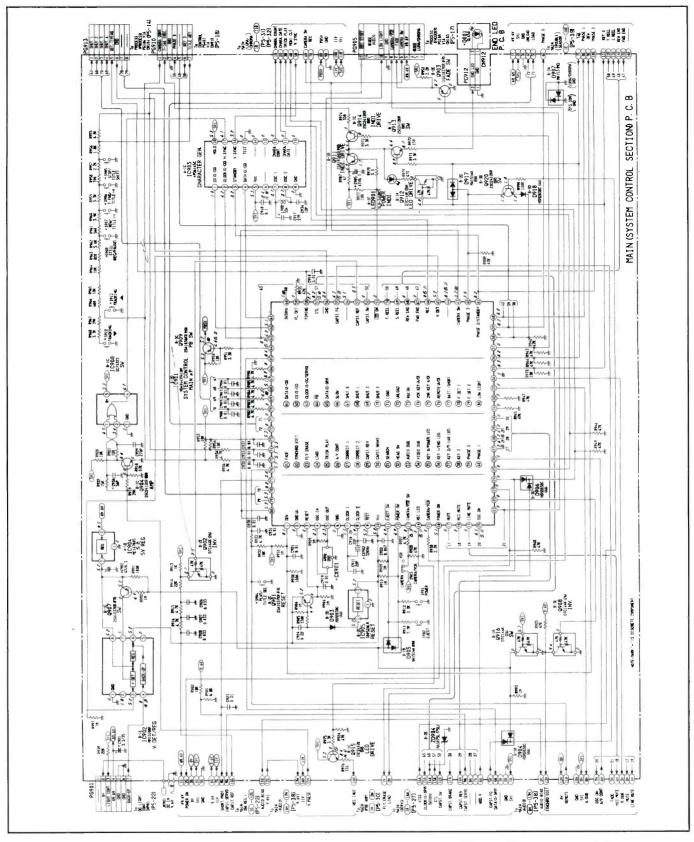
Figure 6. This is the system control section of the main printed circuit board. Integrated circuit IC901, an 80-pin system-control microprocessor, controls the camera assembly; the VCR operation; the power supply; and the power distribution circuitry of the camcorder.
