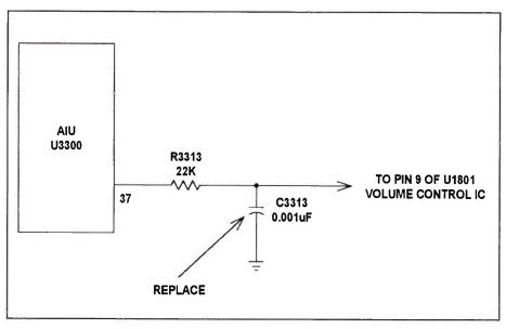
Figure 7. In the RCA CTC157, if the symptom is noisy sound, replace C3313.
