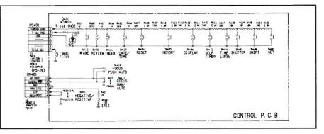
**Figure 8.** The system control processor and the function switches are shown in this schematic diagram. The VCR portion of many camcorders uses a keyboard input matrix system that applies through pins 11, 15, 29, 47, and 48 of the system control microprocessor.
