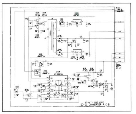
**Figure 1.** A camcorder, which is portable, is different from a VCR in that it needs a dc-to-dc converter to convert the battery voltage into the various voltages required by the circuitry.
