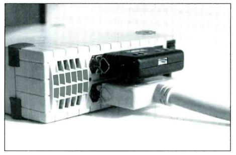
**Figure 3.** When you encounter a problem on a SCSI bus, always first inspect, and then test the cables, since they are the easiest part of the Bus to test. Check the cables for cracks and breaks, especially around the strain relief.
