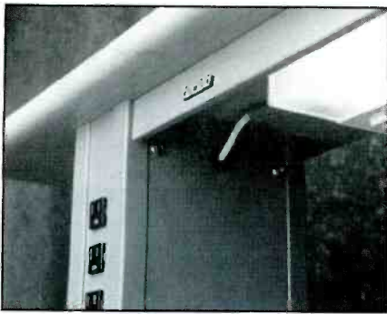
Figure 2. Manufactured workbenches can provide lighting options that help get the light on the work where it is needed. (Photo courtesy Teclab).
