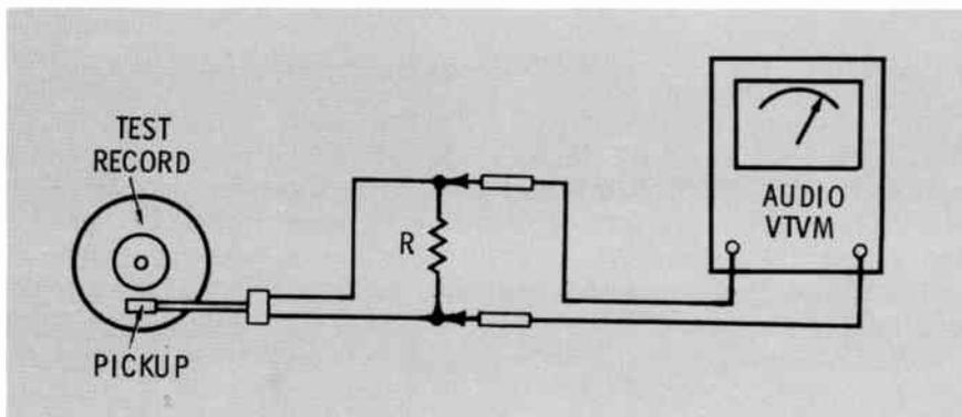
Fig. 2 Test setup for checking cartridge output voltage.
