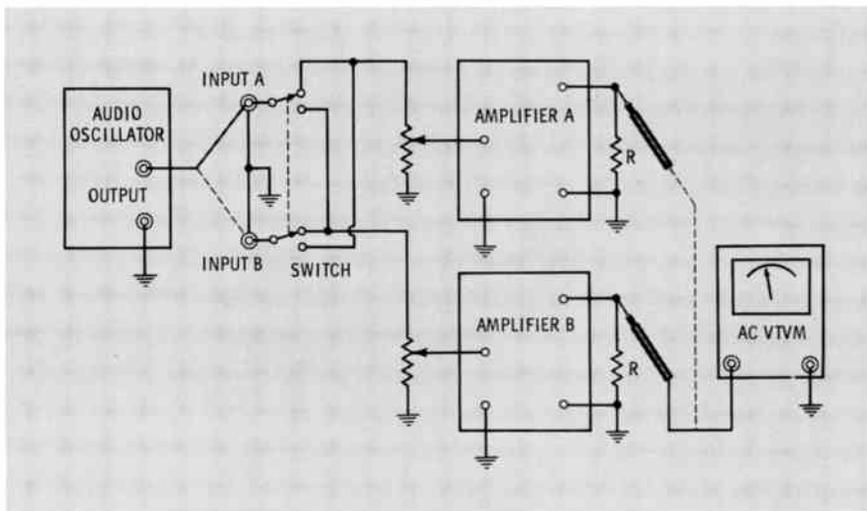
Fig. 9 Checking crosstalk between stereo amplifiers.
