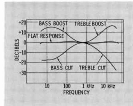
Fig. 9. Response curves for bass and treble tone controls.
