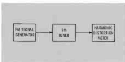
Fig. 10 Test setup for measuring the harmonic distortion of an FM tuner.
