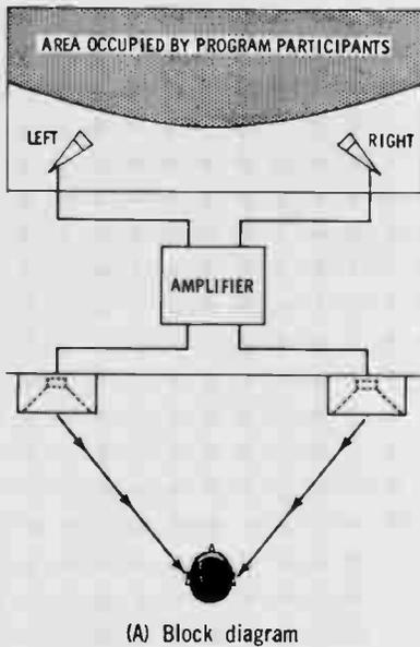
Fig. 2 Basic concept and characteristics of FM stereo system.
