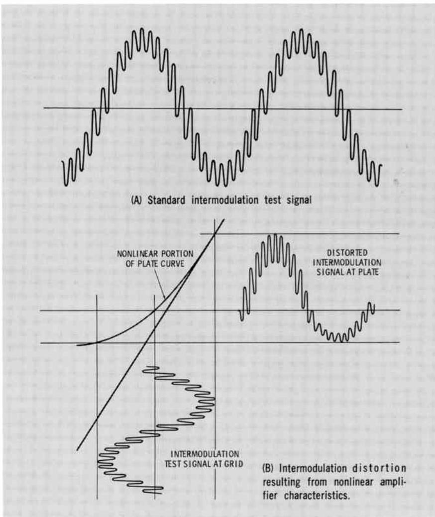
Fig. 15 Test signal and results of intermodulation distortion test.
