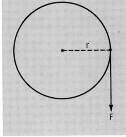
Fig. 12 Illustration of twisting force called torque.
