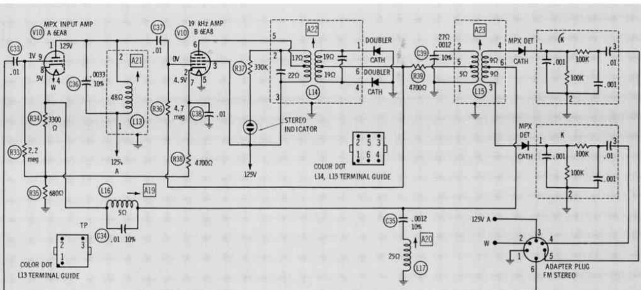
Fig. 7. Envelope-detection multiplex circuit.
