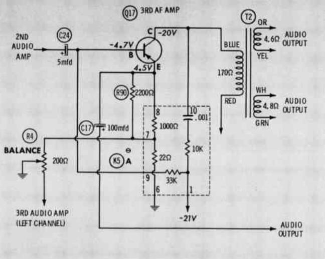
Fig. 14 Leaky coupling capacitor, C24, caused distortion in right channel.
