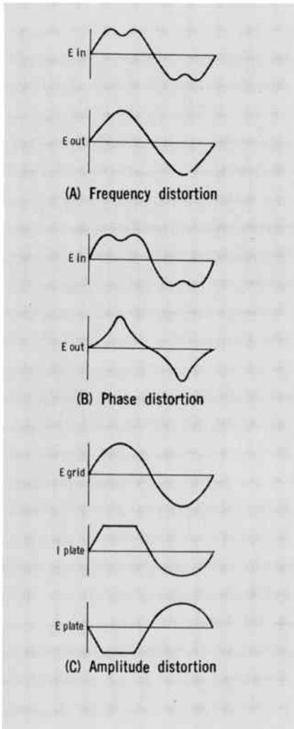
Fig. 11 Three basic types of amplifier distortion.
