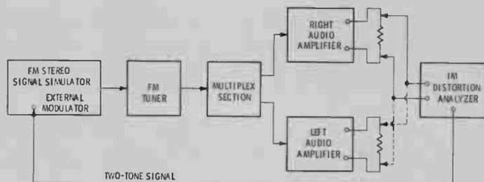
Fig. 11 Test setup for measuring the intermodulation distortion in an FM multiplex stereo system.
