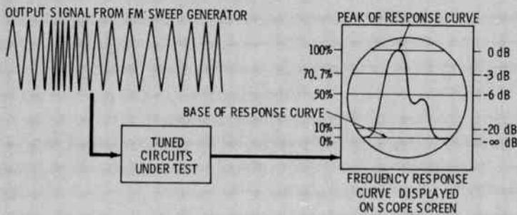
Fig. 10. Basic principle of sweep alignment.
