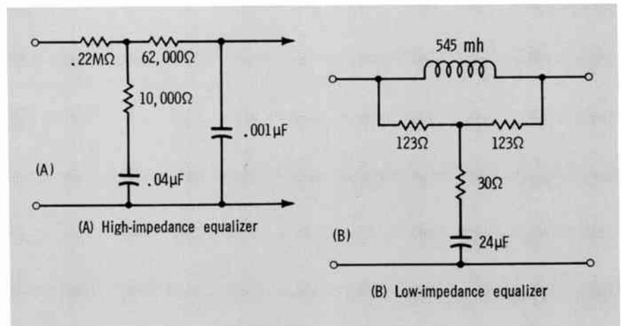
Fig. 5 Equalizer circuits can be used to improve frequency response.
