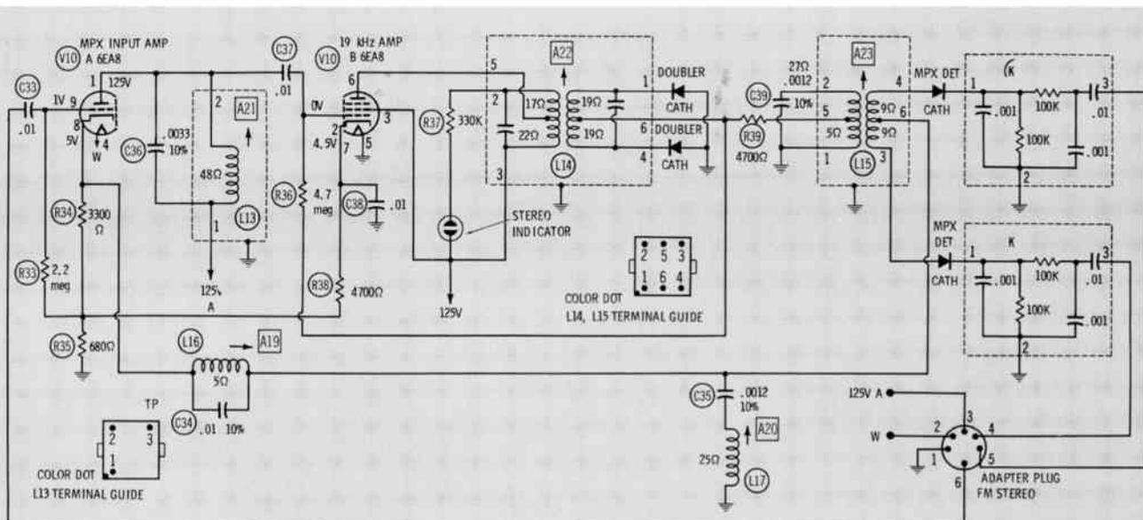
Fig. 7. Envelope-detection multiplex circuit.
