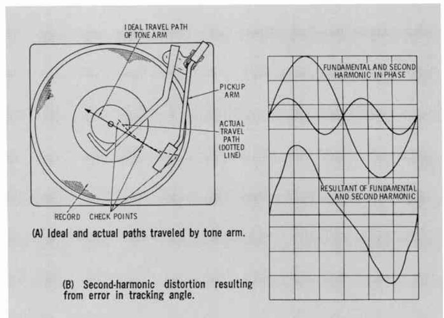
Fig 6 Illustrations showing tracking characteristics and harmonic distortion resulting from improper tracking.
