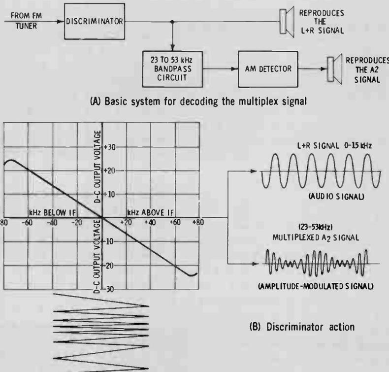
Fig. 6 Method for reproducing the multiplexed signal.
