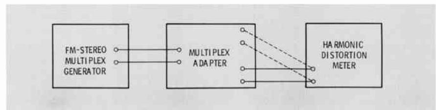
Fig. 7 Harmonic-distortion test setup for a multiplex adapter.
