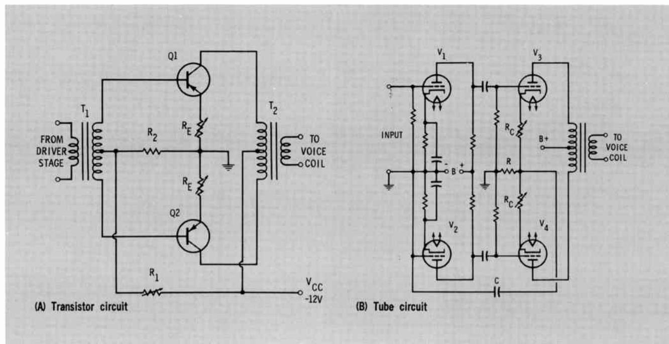
Fig. 1 Basic transistor—and tube-type push-pull circuits.
