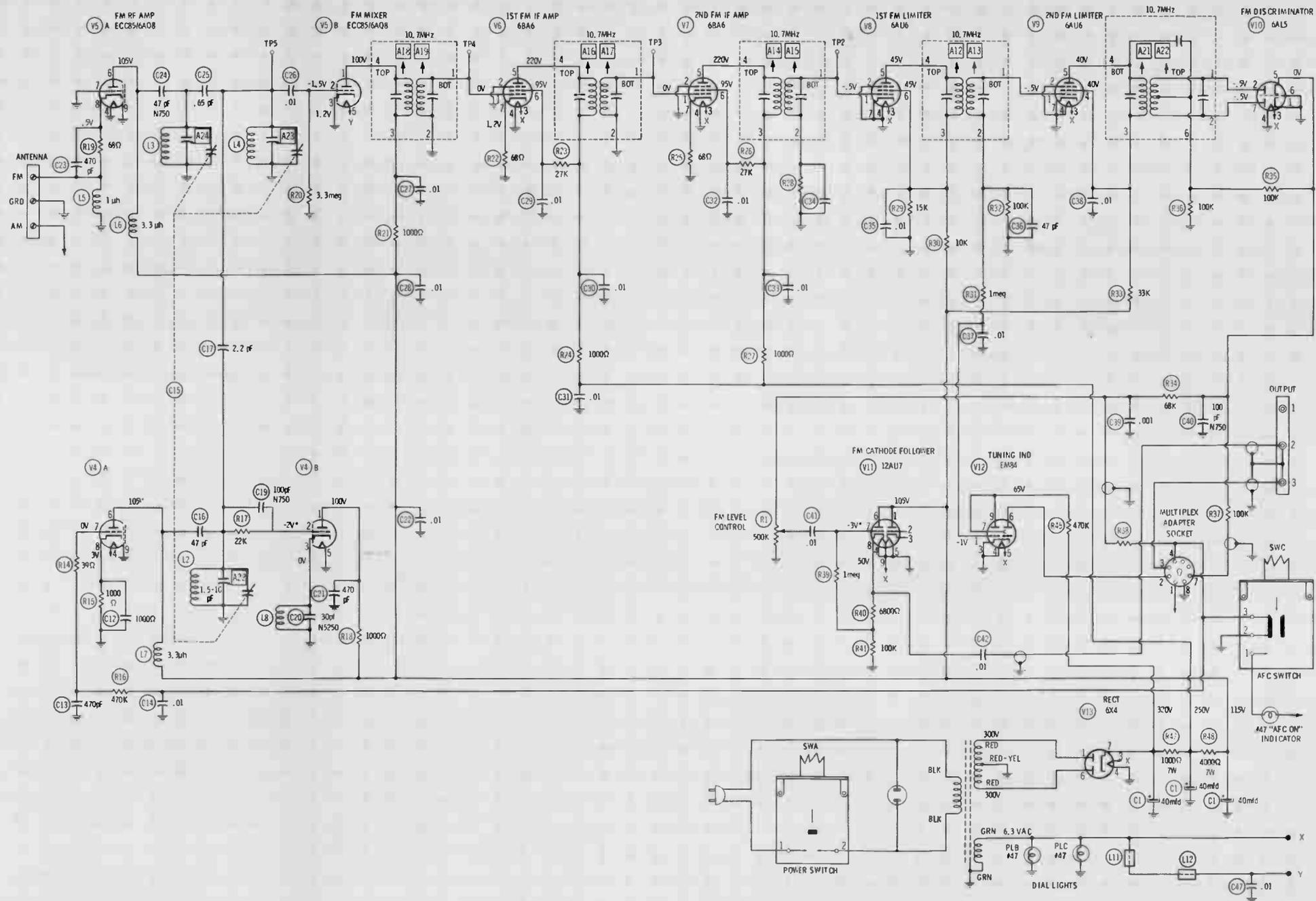
Fig. 2. Complete schematic diagram of a typical tube-type FM tuner.
