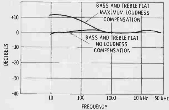
Fig. 4 Typical frequency response of a preamplifier, with tone controls set for flat response and the volume control at maximum.
