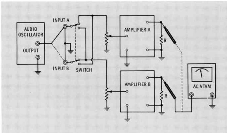
Fig. 9 Checking crosstalk between stereo amplifiers.
