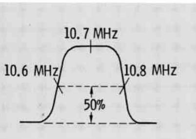
Fig. 4. IF amplifier frequency response.
