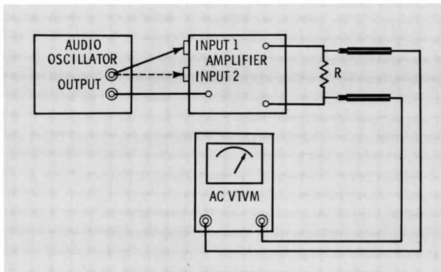
Fig. 10 Test setup for checking crosstalk between inputs of an amplifier.
