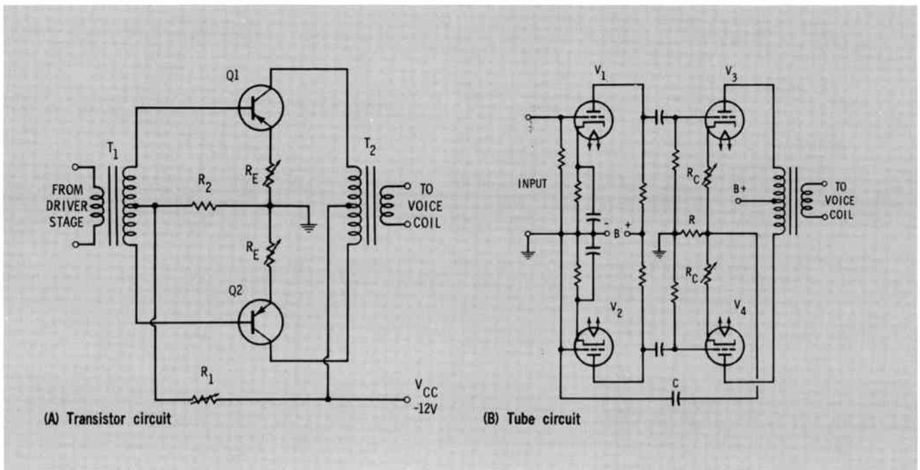
Fig. 1 Basic transistor—and tube-type push-pull circuits.
