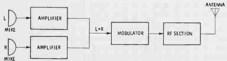
Fig. 3 L and R signals are mixed to produce monaural signal.
