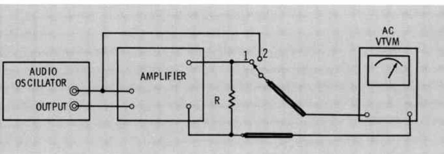
Fig. 13. Equipment setup for testing frequency response of audio amplifier.
