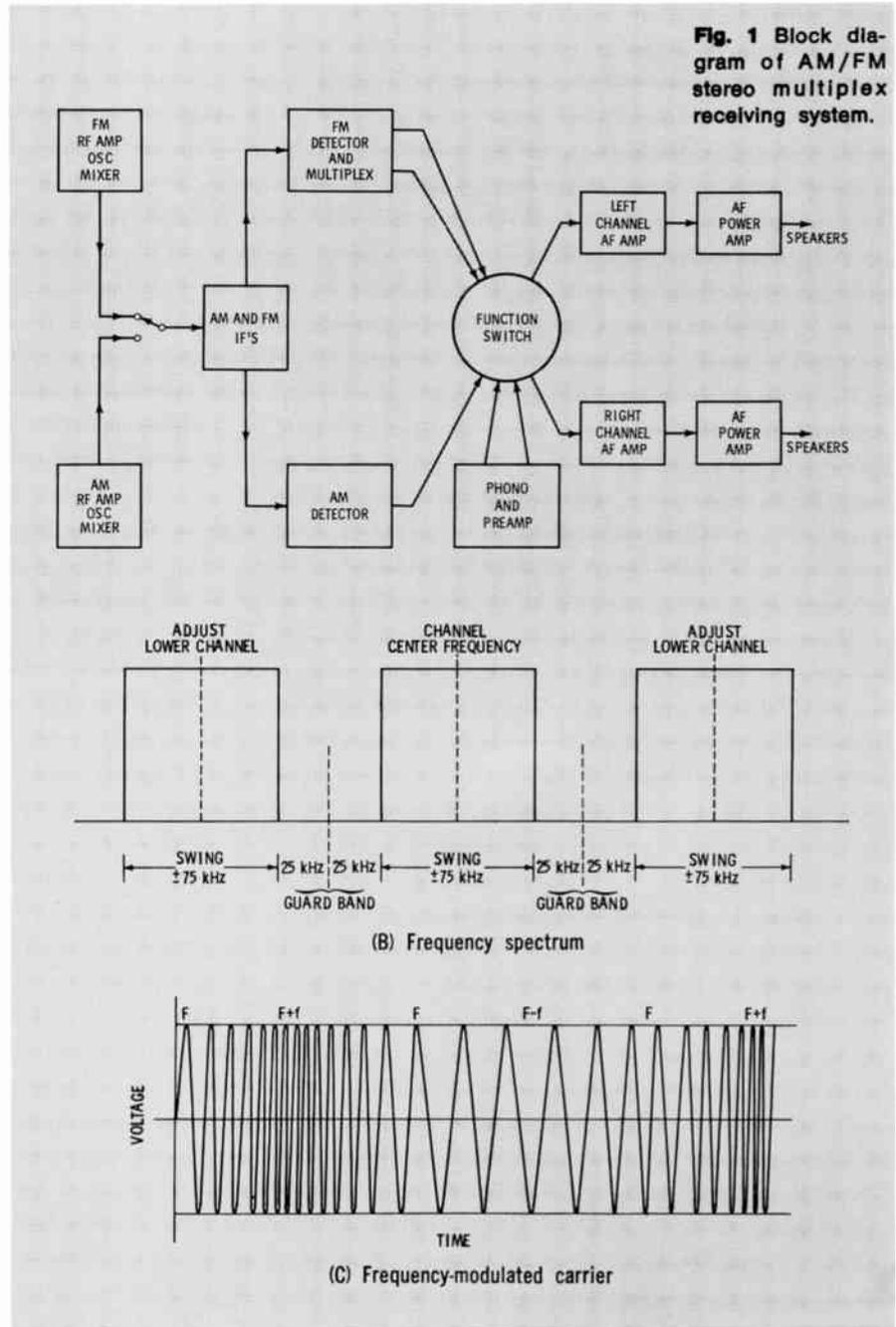
the L and R signals at the receiver. Note also that the system specified by the FCC is a compatible system. In other words, to a conventional FM receiver (monophonic receiver) the multiplex signal "looks like" an ordinary FM signal. But to a stereo-multiplex receiver, the multiplex signal "looks like" separate L and R signals.
