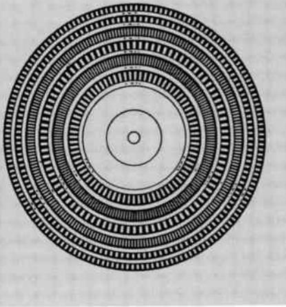
Fig. 11 Stroboscopic disc for measuring turntable speed.
