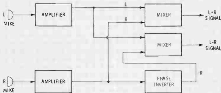
Fig. 7 Developing the L+R and L-R signals.
