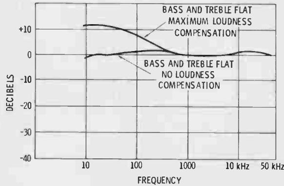
Fig. 4 Typical frequency response of a preamplifier, with tone controls set for flat response and the volume control at maximum.
