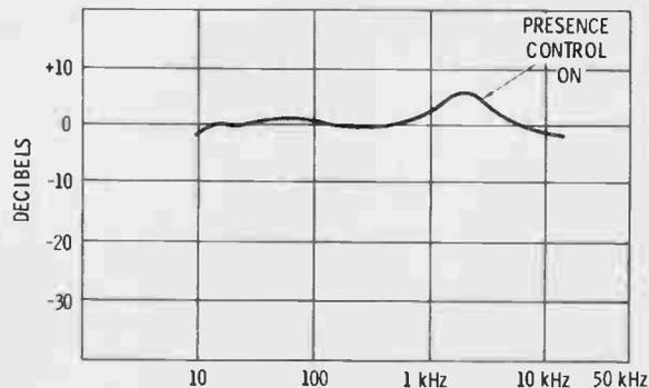
Fig. 5 Preamplifier response obtained with presence control on.
