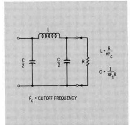
Fig. 15 A single-section, low-pass Pi filter used in rumble test.
