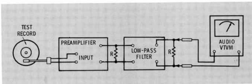
Fig. 14 Test setup for measuring rumble.
