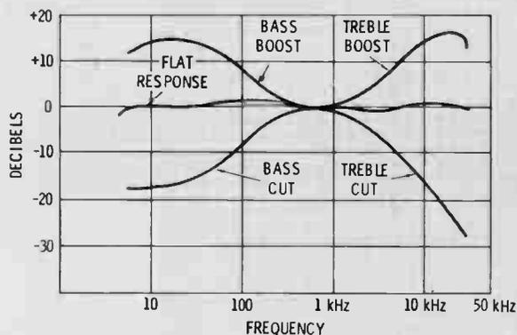
(B) Flat response, with added curves showing the effect of bass and treble controls
