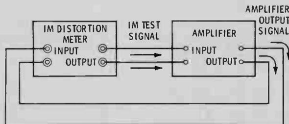
**Fig. 18** Test setup for measurement of intermodulation distortion.
