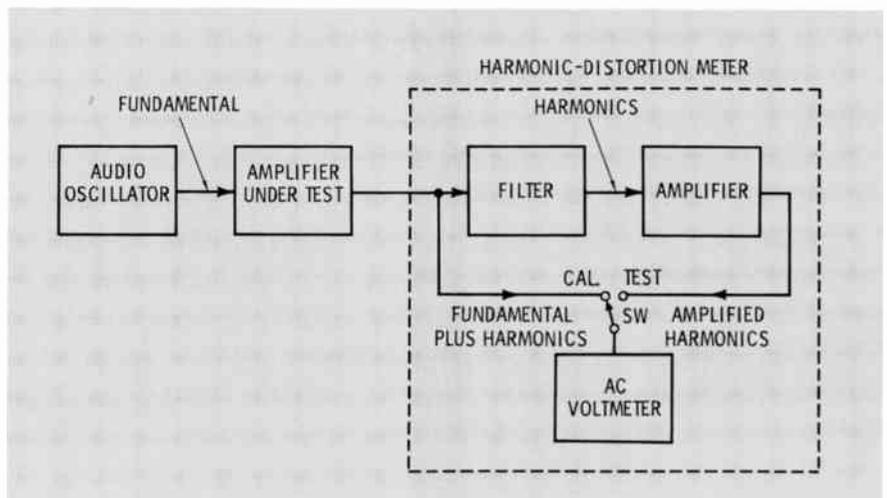
Fig. 14 Test setup for measuring harmonic distortion.
