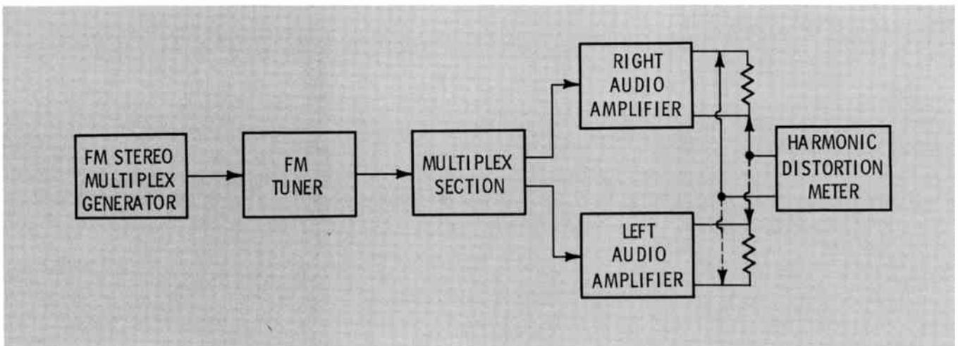
Fig. 1 Test setup for performing harmonic distortion measurement.
