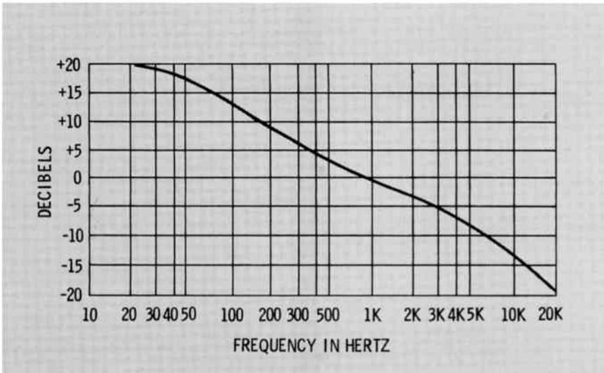
Fig. 7 Record Industry Association of America (RIAA) equalization curve for play-back of records.
