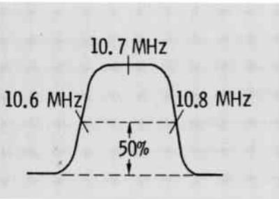
Fig. 4. IF amplifier frequency response.
