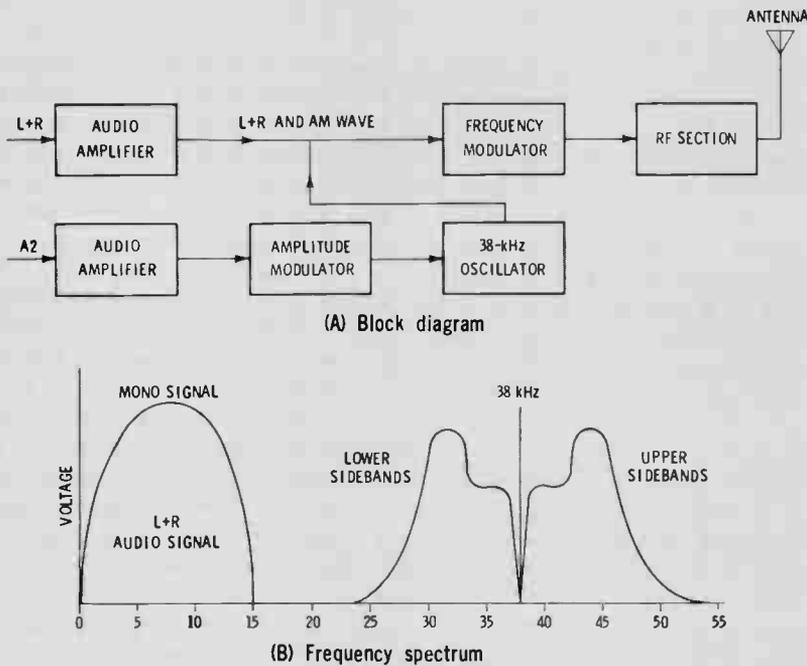
Fig. 5 Amplitude-modulated 38-KHz subcarrier combined with L and R signals.
