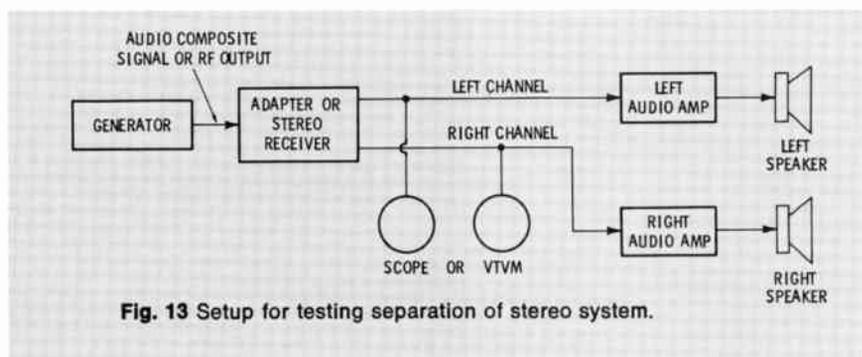
Fig. 13 Setup for testing separation of stereo system.
