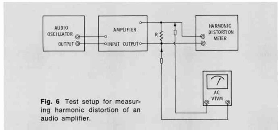
Fig. 6 Test setup for measuring harmonic distortion of an audio amplifier.
