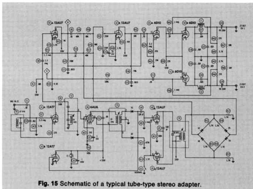
Fig. 15 Schematic of a typical tube-type stereo adapter.
