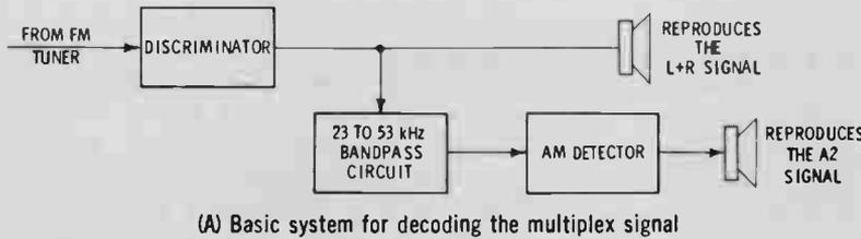
(A) Basic system for decoding the multiplex signal
