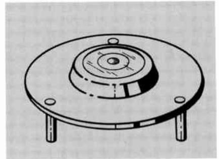
Fig. 13 Device for leveling a turntable.
