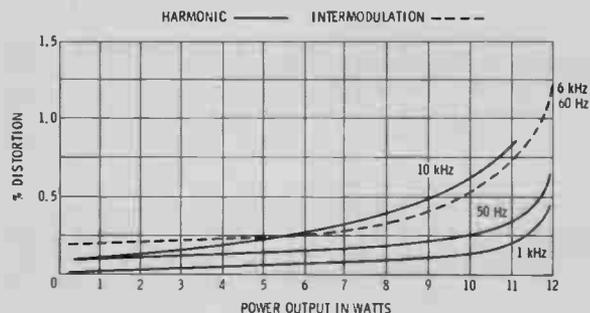
**Fig. 19** Harmonic and intermodulation distortion percentages for a typical high-fidelity amplifier.
