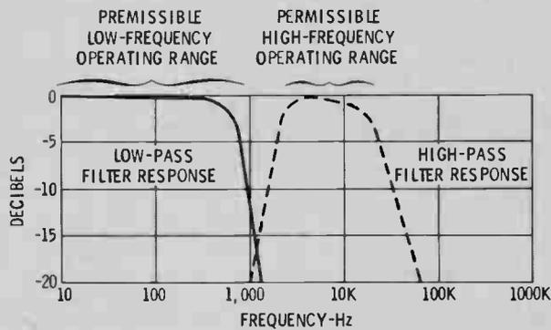
**Fig. 17** Characteristics of the filters in a typical intermodulation distortion analyzer.
