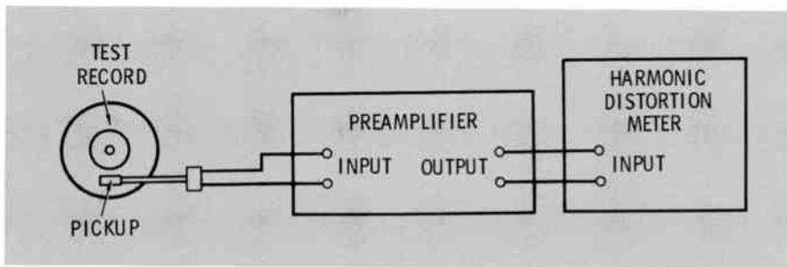
Fig. 7 Test setup for measuring harmonic distortion.
