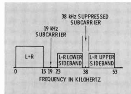
Fig. 8. Frequency spectrum processed by multiplex adapter.
