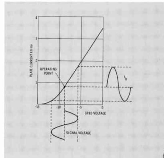
Fig. 13 Compression of the negative half cycle.
