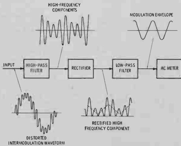
**Fig. 16** Basic configuration of an intermodulation distortion analyzer.
