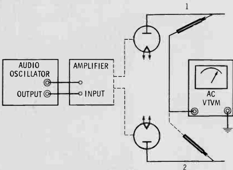
Fig. 2. Test setup for checking AC balance.
