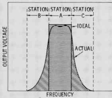
Fig. 3. Frequency-response curve.
