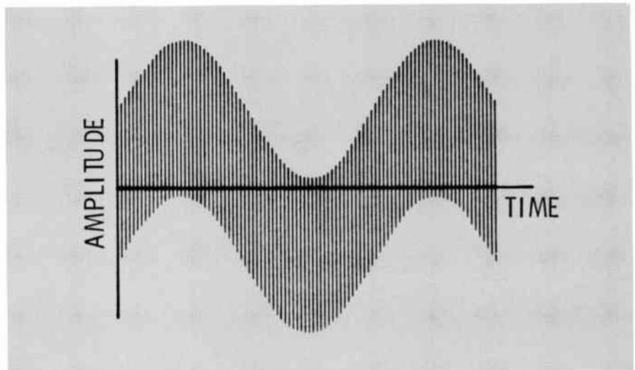
Fig. 4 Hum voltage superimposed on low-frequency waveform.
