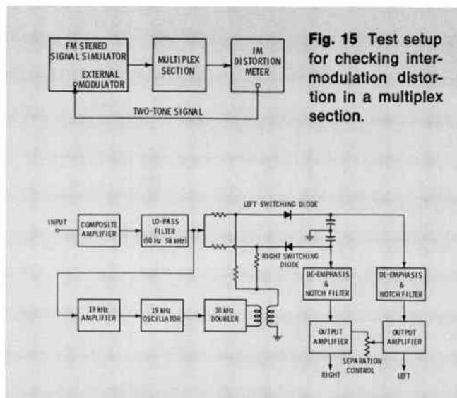
Fig. 15 Test setup for checking intermodulation distortion in a multiplex section.
