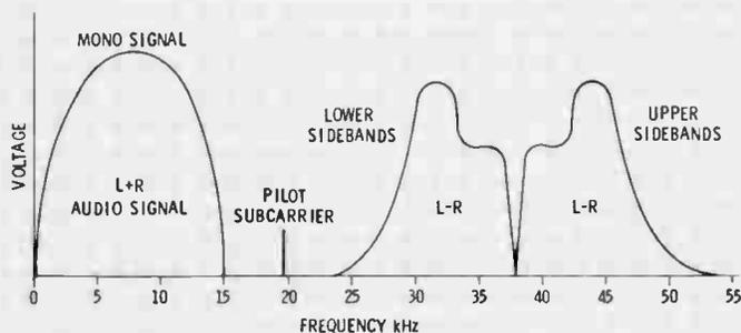
Fig. 10 Composite stereo signal showing 19-KHz pilot subcarrier in empty portion of spectrum.
