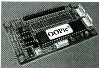
*The OOPic supports 31 I/O lines, and runs on 6-12-volt DC power. Connectors are provided for the I/O lines, programming cable, memory sockets, and Philips I<sup>2</sup>C network.*
