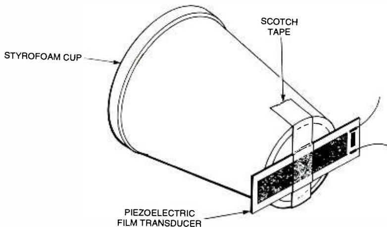
Fig. 2. In this experiment, a 0.63- × 2.9- × 0.008-inch laminated piezoelectric film transducer is converted into a microphone by scotch taping it to the bottom of a Styrofoam cup.
