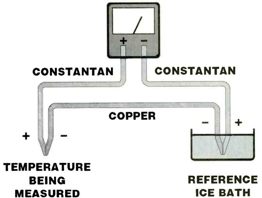
Fig. 1. Thermocouple temperature measurement makes use of the Seebeck Effect to create millivolt-sized signals proportional to temperature differences. The traditional "cold junction" shown here is usually replaced with a small and precise voltage reference.
