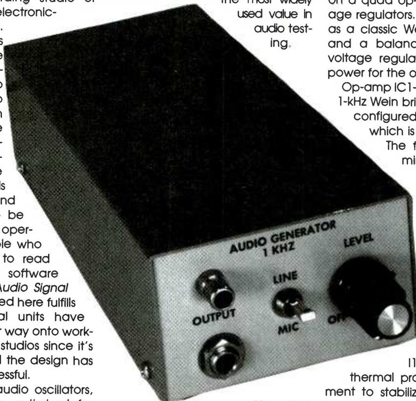
You'll also be pleased to know that this circuit handily outperforms most service-grade audio generators. For example, the prototype produced a rock-stable 992 Hz, 2.5-volt sinewave output. Total harmonic
