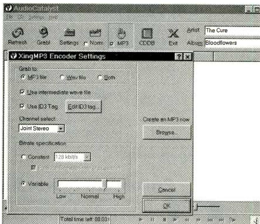
For fast ripping of music from CDs, AudioCatalyst is tough to beat. Be sure to use its VBR features for best quality. The setting shown here, between Normal and High, is an average rate of 160 Kbps.
