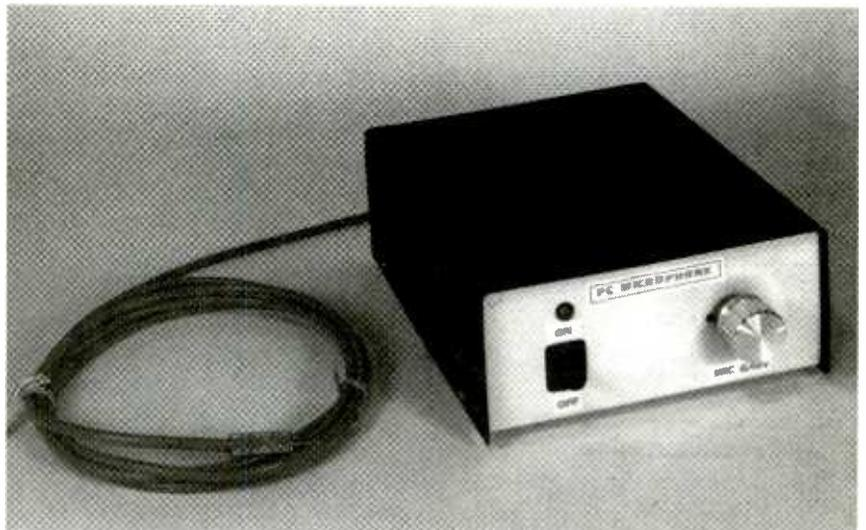
are less common than dynamic microphones but available. Whatever the microphone type (except carbon microphones, which are essentially obsolete anyway), if it's not an electrostatic one, you'll need the PC Microphone Swapper. It is designed to connect a non-electrostatic microphone to your computer's sound-card.
