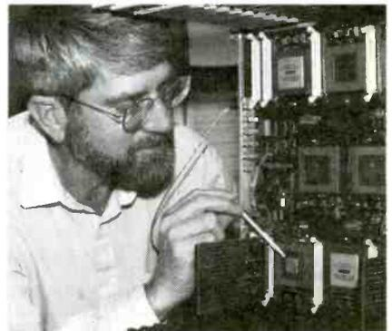
Lyndon Pierson points to the unclassified encryptor chip—the world's fastest encryption device—that his Sandia research team designed.
