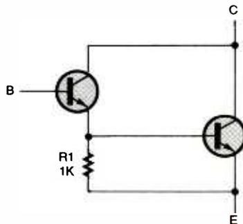
Fig. 2. A Darlington transistor behaves electrically like a two-transistor gain stage. The amplified collector current from the first transistor feeds the base input of the second transistor. The overall gain of the circuit is the gains of the two transistors multiplied together. For that reason, Darlington transistors have phenomenally high gain ratings.
