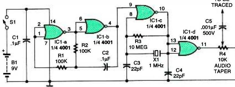
Fig. 1. A simple carrier-wave transmitter injects an RF signal into a wire; an AM radio can pick up the signal as a low-pitched "growl."
