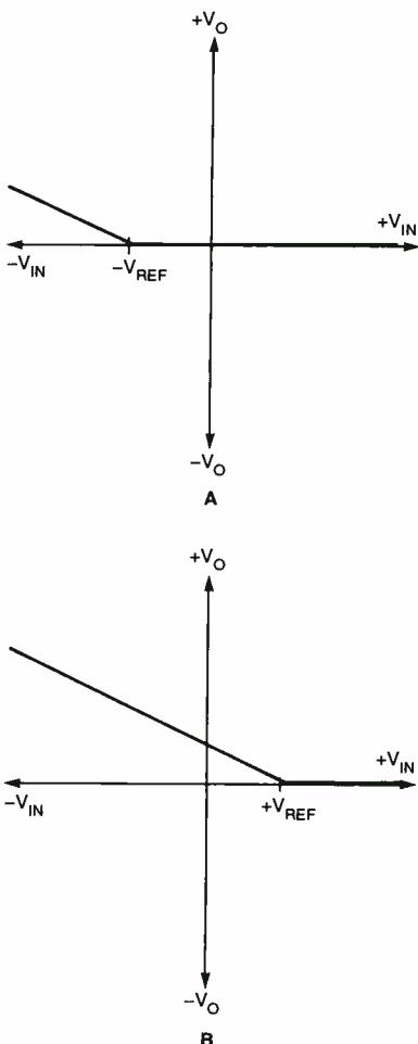
Fig. 10. The transfer characteristics for the circuit in Fig. 9 are shown here. In A,  $V_{REF}$  is negative, while  $V_{REF}$  is positive in B. In both cases, the transfer curve is offset by the reference signal.
