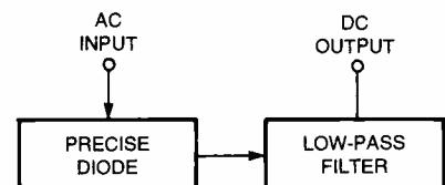
Fig. 5. Shown here is the block diagram of a circuit that's designed to create a DC level that is proportional to the average voltage (or rms value) of the output waveform by time-averaging the pulsating DC.
