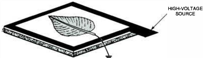
*Fig. 5. Ground the subject—in this case a leaf—using a wire and an alligator clip. Position the camera directly over the subject.*
