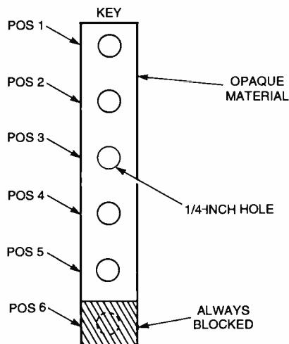
*Fig. 6. One way you can arrange the IR LEDs and phototransistors is to create a slot for the key. As you swipe an opaque card with holes cut in it to match the required pattern of blocked and unblocked pairs, the circuit activates when the patterns match.*
