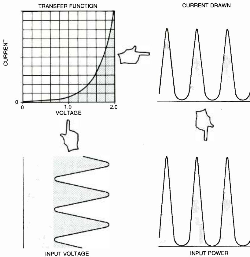
Fig. 1. A transfer function can relate the output to the input of any history-free physical system. In this low frequency hydrogen cell, extreme nonlinearity redistributes the spectral energy.
