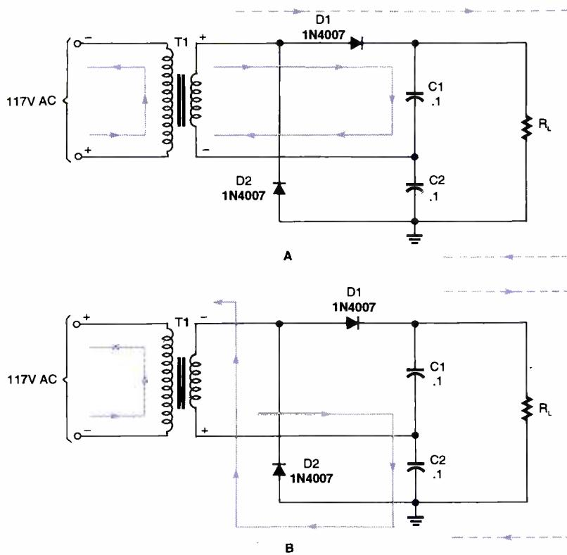
Fig. 3. For the sake of greater clarity, the full-wave voltage doubler illustrated in Fig. 2C can be redrawn as shown here. The full-wave voltage-doubler circuit has better regulation, is easier to filter, and produces nearly double the peak AC voltage of the half-wave version.
