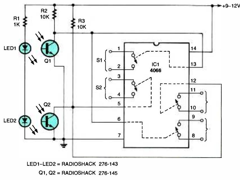
Fig. 1. This simple electronic switch is built around two pairs of infrared LEDs and phototransistors. The CMOS analog switches isolate the phototransistors from whatever load you want to drive.
