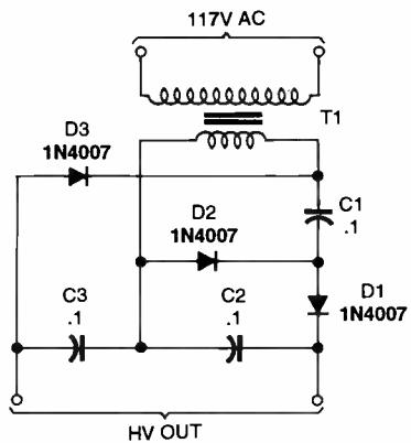
Fig. 4. Here is a voltage-multiplication configuration based on the circuit in Fig. 3 that can be used to generate a DC output voltage three times that of the AC input to the circuit.
