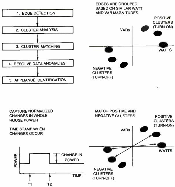
Fig. 3. By analyzing the raw data captured by the recorder, NIALMS can recognize individual appliances by their usage pattern.
