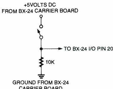
*Fig. 1. Wire the switch so that it connects to the V+ (pin 21, not pin 24) of the BX-24.*
