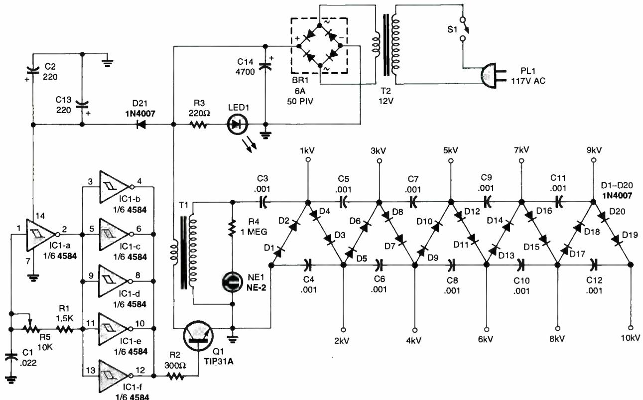
Fig. 9. Generate up to 10 kilovolts with this advanced design.
