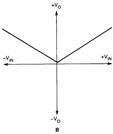
Fig. 7. The fullwave rectifier uses both halves of the input sinewave. Shown in A is the input sinewave and the pulsating DC output of a fullwave rectifier. The characteristic function for the fullwave rectifier is shown in B.
