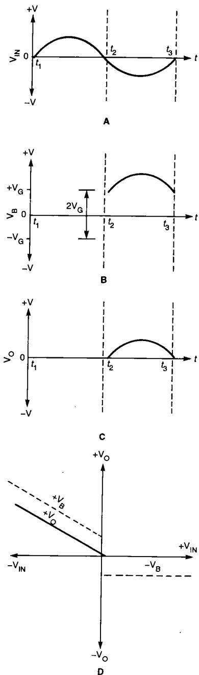
Fig. 4. These waveforms help to illustrate the operation of the precise rectifier. The illustration in A shows the input waveform, B shows the waveform at the output of the op-amp, C shows the circuit's output waveform, and D shows the same situation graphically.
