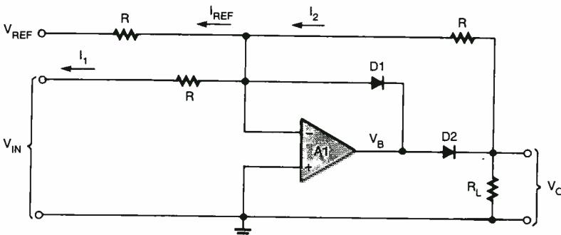
Fig. 9. The zero-bound circuit is one in which there are constraints on the allowable output voltages. The output of a zero-bound circuit indicates when the input signal exceeds a certain threshold and by how much.
