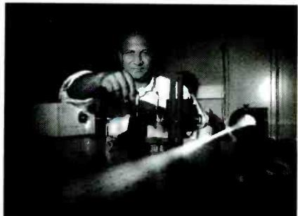
The high-powered laser in Professor Sayeh's lab is a water-cooled device about four feet long. It projects images through a series of lenses and mirrors laid out in a maze-like pattern that allows the laser beam to be repositioned as it sends pages of information to the crystal.
