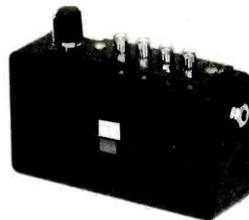
Fig. 7. Several holes need to be located and drilled for mounting the external components of the GameEnhancer. Note the rectangular hole for DISPI and the "speaker-grille" hole pattern.
