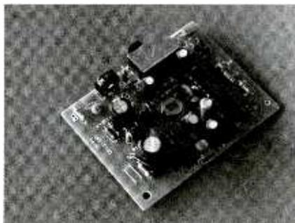
Fig. 5. Here is a hacked PIR detector, showing the DC-operating circuit board.
