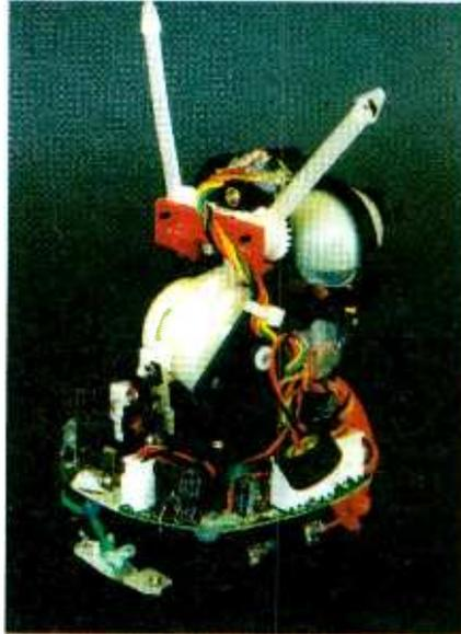
This photo shows just how jam-packed a Furby is inside. A semicircular PC board is located just above the battery compartment, with the mechanical module mounted on top of that. The sound-sensing microphone is hanging on its lead in the foreground.
