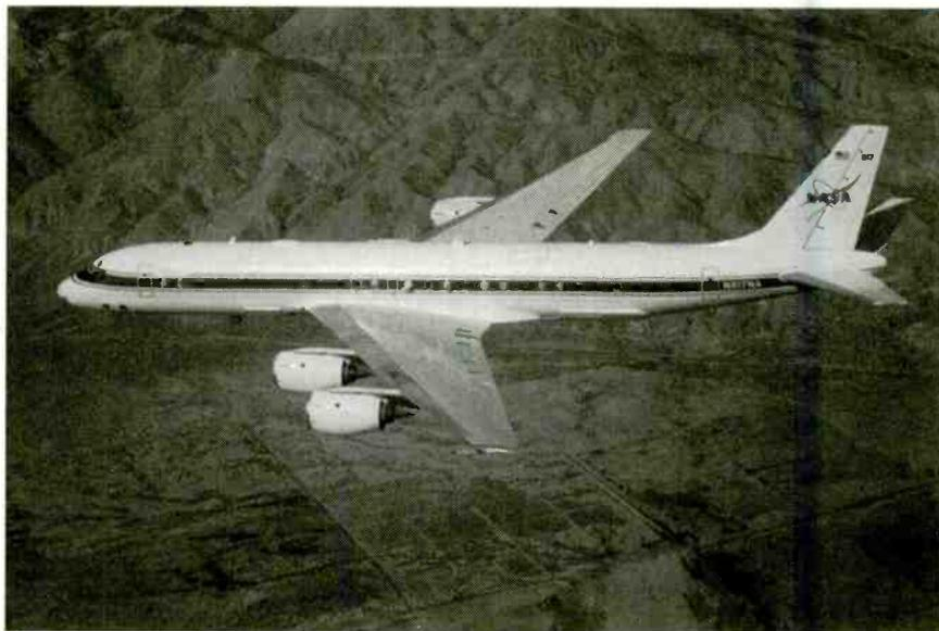
NASA's DC-8 Flying Laboratory is a converted long-range jetliner that is now a world-class airborne scientific laboratory that can carry 30,000 pounds of scientific instruments and equipment along with scientists and experimenters.
