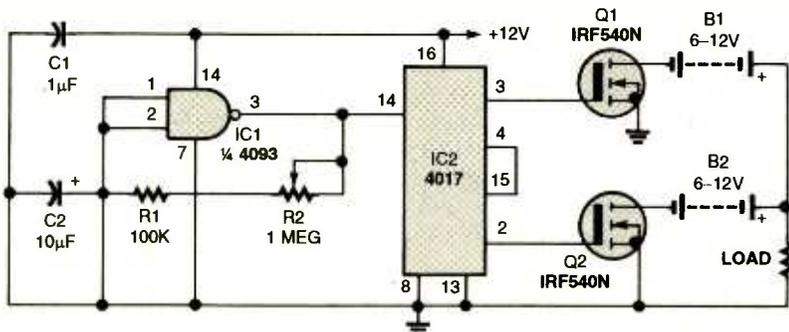
Fig. 3. Two batteries can be life tested at the same time with the circuit shown above. A NAND Schmitt trigger is at the heart of a square-wave circuit that controls the tester.
