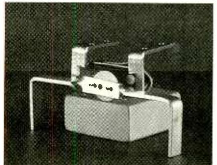
The center servo is shown here ready to be attached to the body. The center legs and the two L-brackets have been attached to the servo.
