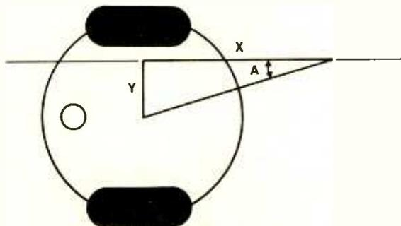
48 Fig. 4. When the robot is not in the middle, a second angle of correction can be calculated.
