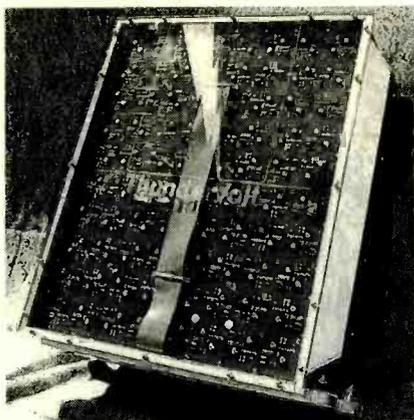
The ThunderPack ultracapacitor unit uses 149 Maxwell PowerCache ultracapacitors. A dual pack can meet the most demanding acceleration and peak power needs of large HE transit buses and trucks.
