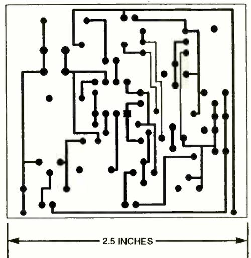
Fig. 8. Here is the solder-side foil pattern for the main PCB module.
