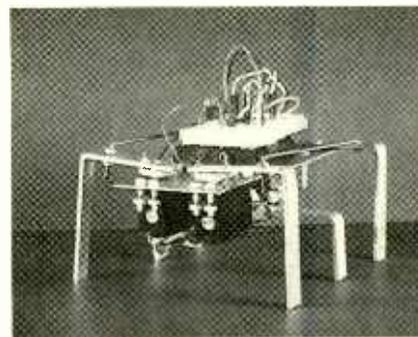
Here is the completed hexapod. A breadboard containing the circuit is mounted to the top of the body. The robot is controlled by a PIC16F84.
