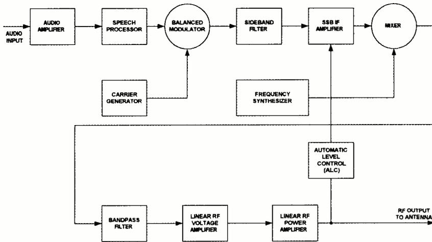
FIG. 1. BLOCK DIAGRAM SSB TRANSMITTER USING FILTER METHOD
