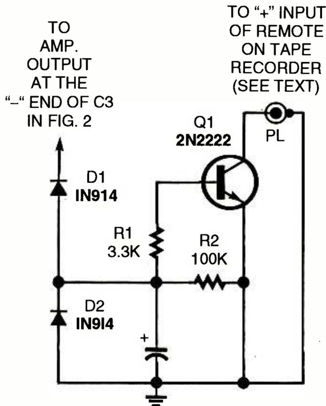
Fig. 5. The amplified audio from the hammering is rectified and fed to the base of Q1. The collector of Q1 connects to the positive input of a cassette recorder's remote input and the negative input to circuit ground. The sound turns Q1 on, starting up the recorder.
