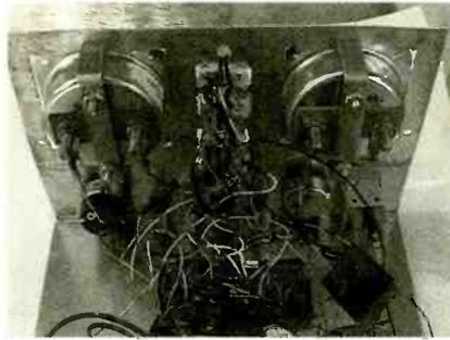
*The variable power supply features two independent outputs, which are adjustable from 0 to 20 V<sub>DC</sub>. Two lead-acid batteries provide power; therefore, the device is completely portable.*
