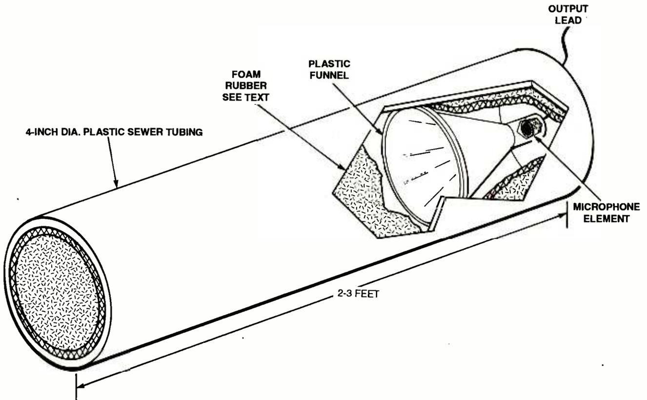
Fig. 4. A drawing for a tube pick-up suitable for gathering bird songs is shown above. A 2- to 3-foot length of light-duty, 4-inch diameter, plastic sewer tubing serves as the sound director and housing for the pick-up.
