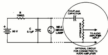
Fig. 3. A neon lamp relaxation oscillator was a favorite project for budding electronics hobbyists and could operate for nearly the shelf life of the battery.
