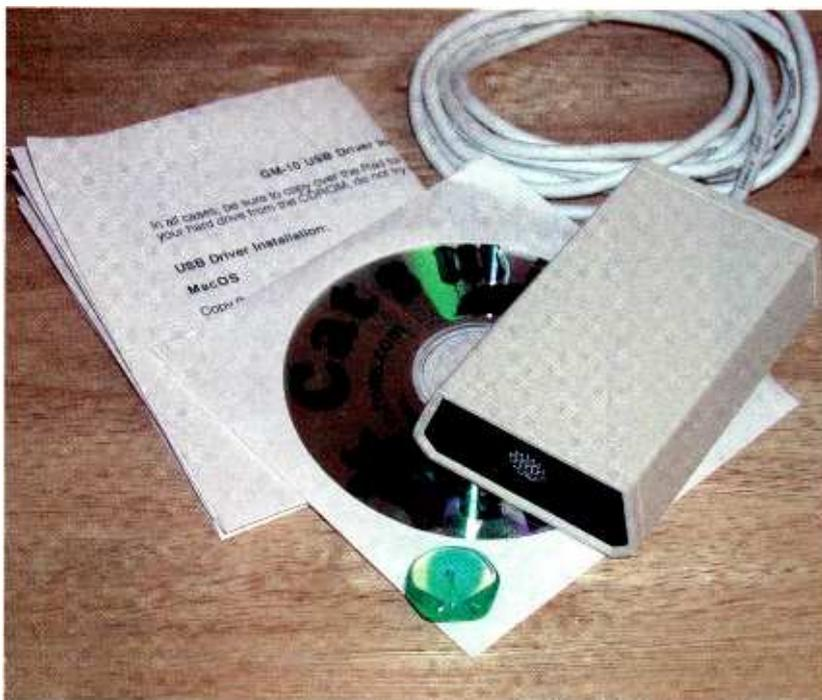
CPM, the higher the radiation level. The GM-10 contains a Geiger-Müller tube capable of detecting alpha, beta, gamma, and X-ray radiation.
