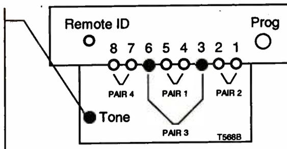
Fig. 6. In tone mode, the remote unit transmits a tone down a selected pair of wires.
