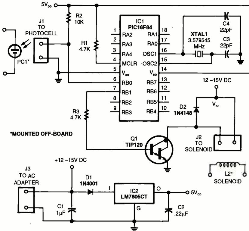
Fig. 1. Here is the schematic diagram of the light-activated circuit, which uses a 16F84 PIC microcontroller. Pin RB0 acts as an input that monitors the voltage developed across a Cadmium-Sulfide (CdS) photocell.
