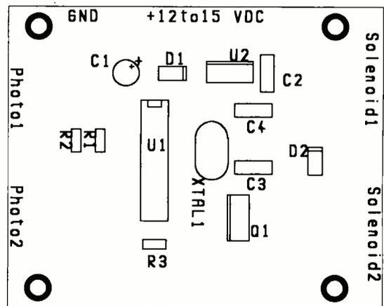
Fig. 3. Use this parts-placement guide as a reference when you construct your board. Be sure to use the 18-pin DIP socket for the PIC no matter what construction method you choose.
