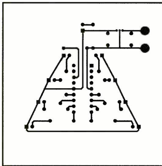
Fig. 2. This is the foil pattern for the Merry Christmas Tree. A kit that comes complete with a printed circuit board is available from Futurlec (see Parts List).
