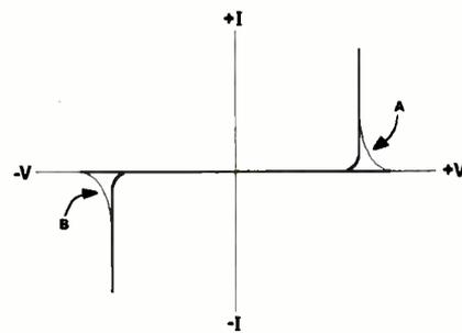
Fig. 1. This current vs. voltage graph of a diac is similar to that produced by a transistor curve tracer and shows the similarity of the device to a neon lamp.
