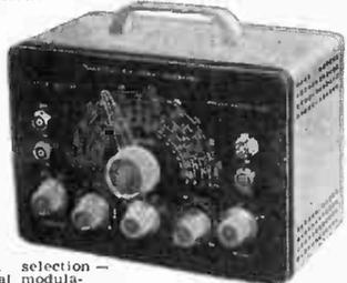
Output selection — interval modulation, pure r.f., or audio output.
