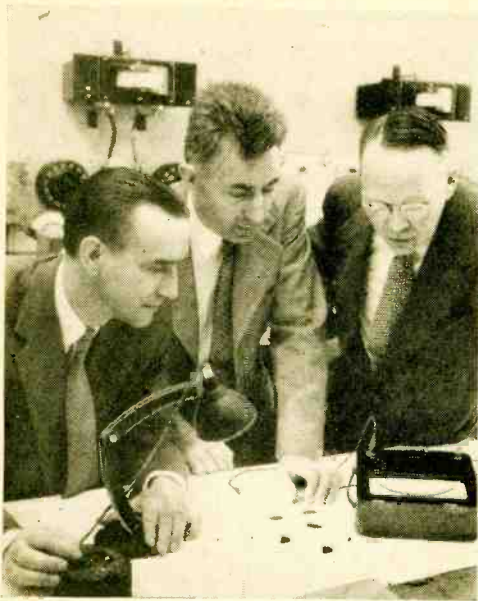
G. L. Pearson, D. M. Chapin, and C. S. Fuller of Bell Labs checking sample devices for amount of electricity derived from "sunlight" (lamps).
