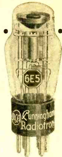
Fig. 3. The electron-ray tube, in many applications, replaces a more delicate meter.
