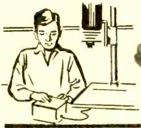
Fig. 1. The timer, shown here controlling an enlarger, can be used to time "on" or "off" intervals of other equipment drawing as much as five amperes.
