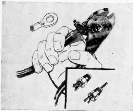
by a recent design change which now enables it to install solderless terminals. In addition, it still performs its original functions as an all-purpose tool for the cutting, stripping and twisting of solid or stranded wire and the installing of the nylon-insulated Buck "Nycaps" on pigtail splices.
