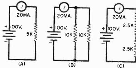
When a resistor of the required wattage rating is not available, it is sometimes convenient to split the wattage by using two or more resistors whose total value is equal to that of the required resistor. As shown in Fig. A, a 5000  $\Omega$  resistor connected to a 100 volt source will draw 20 ma. of current. The wattage dissipated in this resistor will therefore be:
