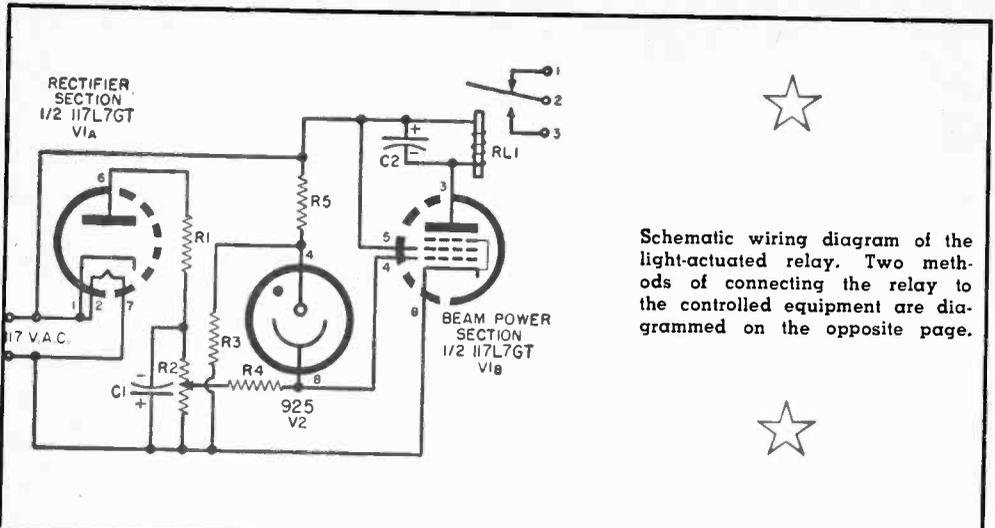
Schematic wiring diagram of the light-actuated relay. Two methods of connecting the relay to the controlled equipment are diagrammed on the opposite page.
