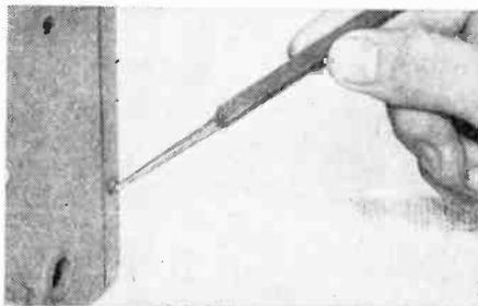
emergency to loosen Phillips type screws if the proper screw driver is not available.
