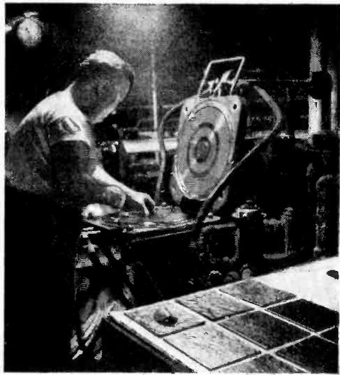
**9** The metal stampers, labels, and heated "biscuits" come together in the record press, which resembles a huge waffle iron. Hot steam, followed by cold water, is forced through the press to assure correct formation of the plastic discs.
