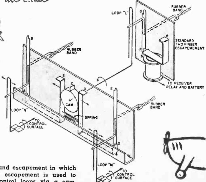
Fig. 1. A type 2 compound escapement in which one standard two-finger escapement is used to actuate two separate control loops via a cam.
