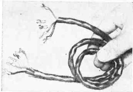
Cable of this type is listed in catalogues for speaker and telephone wiring and is usually number 18 or 22 gauge.
