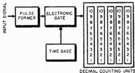
The accompanying figure is a block diagram of one particular EPUT meter. Pulses corresponding to the events, occurring at an unknown rate, are amplified and properly shaped by the input circuit. These pulses are then passed through the electronic gate to the bank of five deci-
