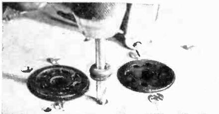
drill bit before you start. Then if the hole breaks through suddenly, the edges will not be scratched by the rapidly descending chuck.
