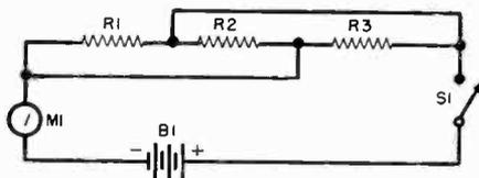
voltage is 3 volts, what will be the total current drain, as indicated by the ammeter, when switch  $S_1$  is closed? The answer is given on page 128.
