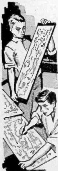
Printed circuits are inspected and retouched wherever needed. Large boards are then cut and punched with holes to receive parts and wiring.
