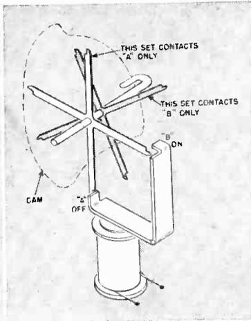
Far left, Fig. 2. Back view of an ECCO compound escapement which uses two four-finger units and two cam wheels to actuate two "Y" yokes, each with its own shaft. This allows two control functions. Left, Fig. 3. Simplified drawing of the ECCO compound escapement showing how the four-finger units operate separately with a single solenoid.
