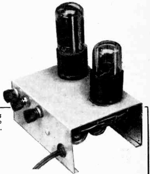
The completed photo relay; binding posts shown are connected to the circuit which is to be controlled.
