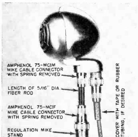
connector, and slip a 2½" length of 5/16" diameter fiber rod into the connectors and tighten the set-screws. The female connector fits the top of the stand, and the male con-
