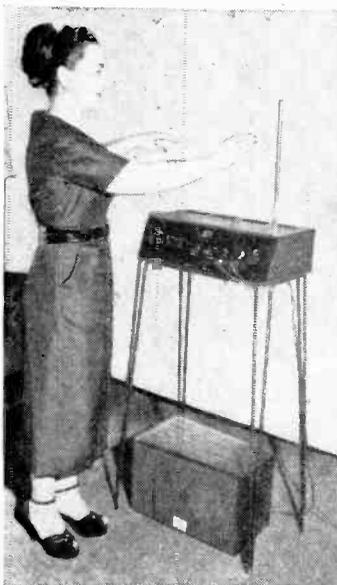
**M**OVING her hands around the antenna, the young lady at the left is playing music on the Theremin, an electronic musical instrument. The volume and pitch are controlled by hand movements; the performer never touches any buttons or keys. Top unit contains oscillator and control circuits; lower unit is amplifier and loudspeaker. This model is made by the *R. A. Moog Company*.
