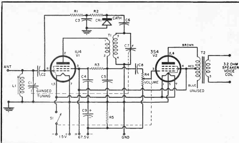
In the circuit shown in the schematic diagram above, V<sub>1</sub> acts as both radio-frequency and audio-frequency amplifier. See the text for an explanation of how this is accomplished.
