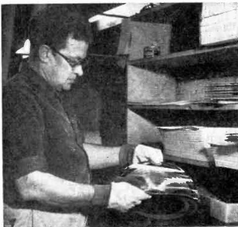
**6** The lacquer master disc is separated from its plated metallic coating, which is a perfect negative impression of the record grooves. This coating, known as a "metal master," may be reinforced and used to stamp records, or it may be plated again to provide a positive metal mold known as a "mother." The "mother," in turn, is electroplated to form a "stamper" which is used to make the actual records we hear.
