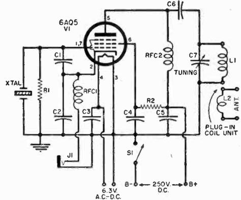
When wiring the transmitter follow both schematic and pictorial diagrams closely.
