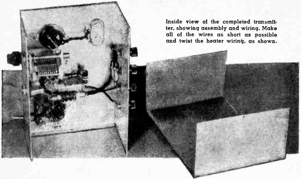
Inside view of the completed transmitter, showing assembly and wiring. Make all of the wires as short as possible and twist the heater wiring, as shown.
