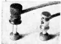
To make these tip-posts, solder the threaded shanks on binding posts into the sleeves of phone-tips. Binding posts with non-removable tops (left post in photo)
