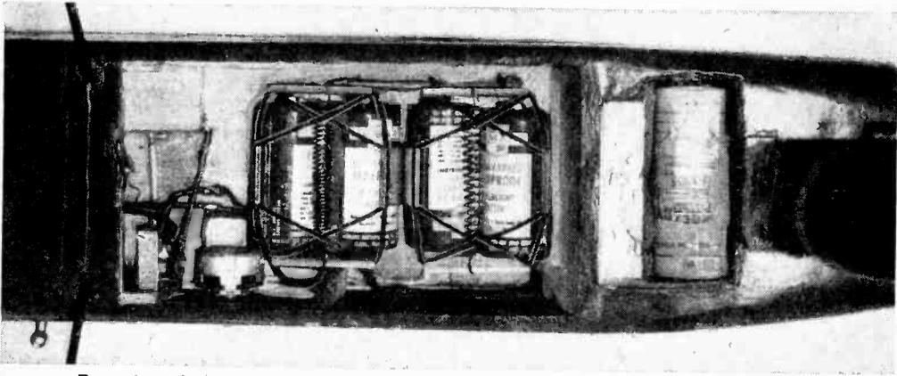
Example of battery installation in the belly of an airplane under the hardwood floor. The forward box contains a hearing-aid "B" battery, the rear compartment contains the batteries for the receiver filaments (1½ volts) and the escapement requiring 3 volts.
