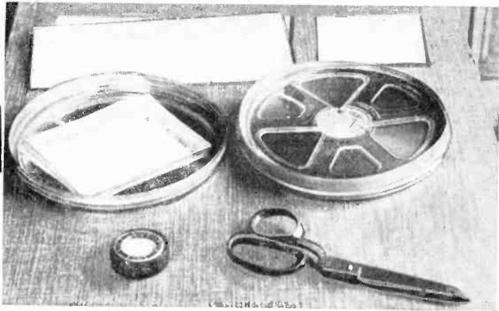
For proper archival storage of tape in can, dried blotting paper must be cut to fit inside the can on top and bottom.
