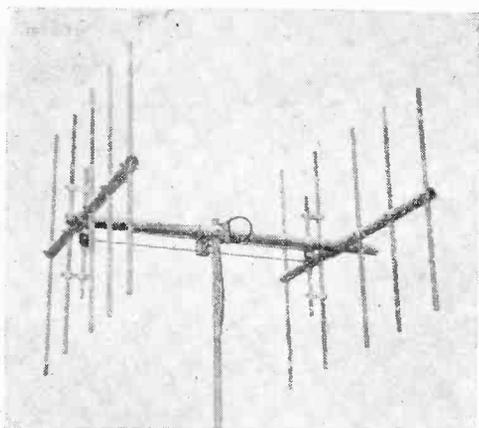
Telrex two-meter beam antenna is representative of a type used by many "hams."
