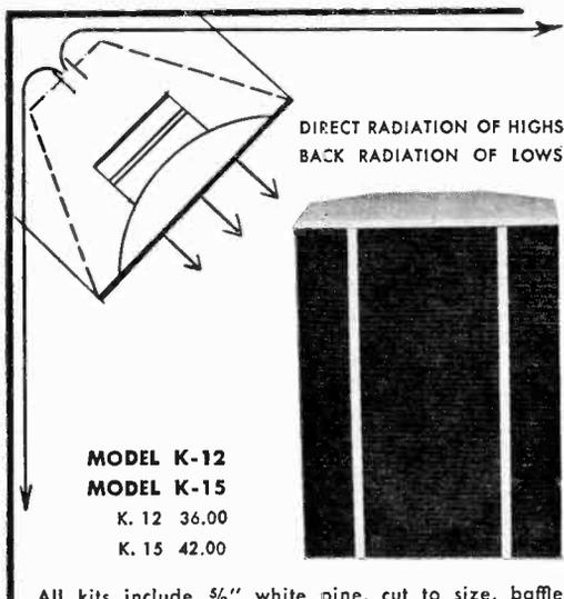
All kits include 5/8" white pine, cut to size, baffle pre-cut for 12" or 15" speaker, Saran plastic acousti-cloth, Kimsul acoustic insulation, assembly and finishing instructions, hardware, plastic wood, sandpaper and glue. Write for complete catalogs and nearest Cabinart kit dealer.
