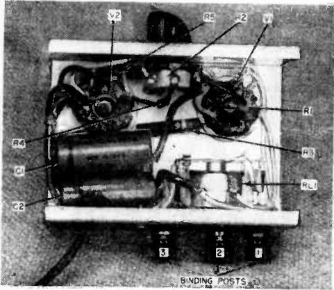
Bottom view of chassis showing placement of major parts.
