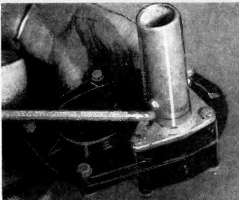
A short piece of pipe is welded onto the bottom or output shaft of the gear box and becomes part of the revolving crank as shown.
